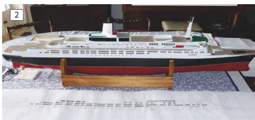
Photo 2. Arrangement drawing of the windows & port lights and the finished model. You can see that the self-adhesive windows already applied match the drawing.
