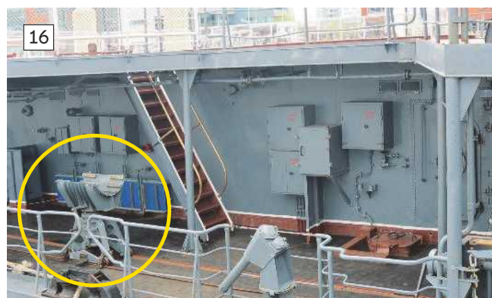
Photo 16. Dropping down from the flight deck to the main deck level aft, there is a dolly (ringed in yellow) for moving mines or torpedoes.
