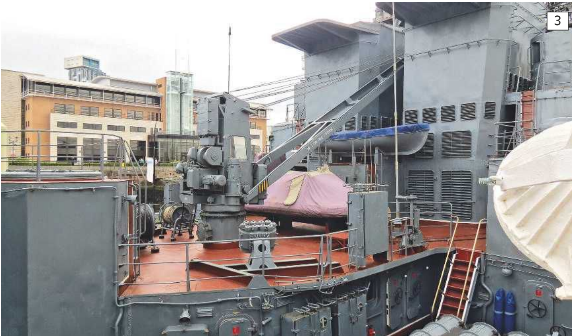
Photo 3. The crane and how it is sited on O1 deck.
