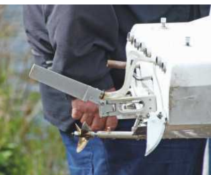
ABOVE: Note the horizontal rudder. It flipped back when this boat hit a buoy and the lower retaining bolt shearing off as designed to do to prevent major hull damage.
