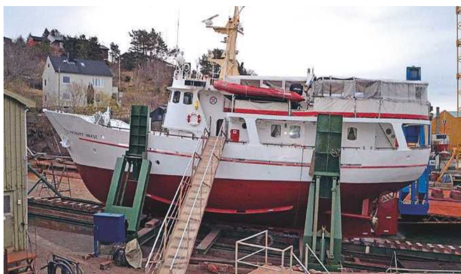
ABOVE: The hull below the waterline is fairly voluminous with deep bilges.
