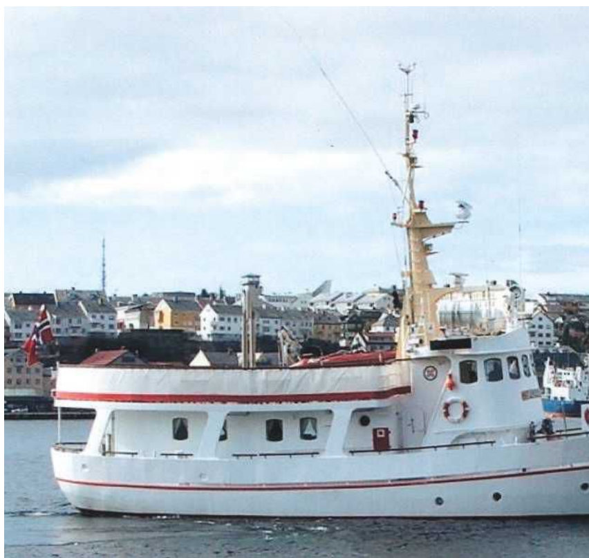
RIGHT: Profile view, which also shows the wooden hand grip rails fitted on top of the steel bulwarks.
