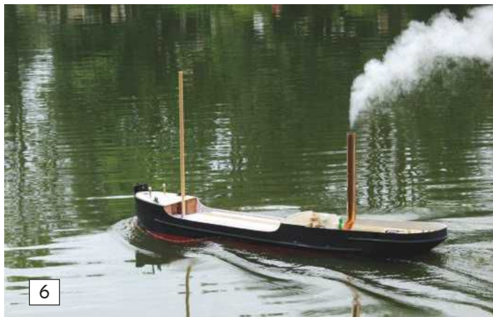
Photo 6. Starting to fit the decks makes the operation more realistic. In this case the foredeck is on enabling access into only the other compartments to be evaluated.
