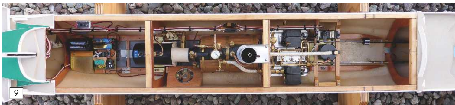
Photo 9. Final arrangement of propulsion machinery and controls inside the QE2 model.
