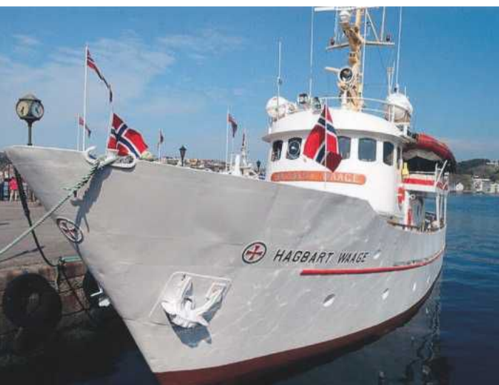
ABOVE: The traditional Norwegian Rescue Service badge is retained on the bow and note the protective additional plating for hull protection from the anchor when it is housed.
