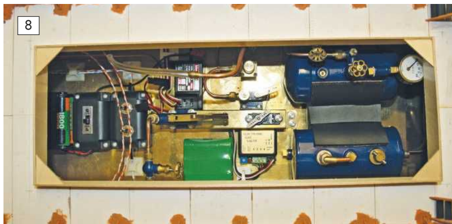
Photo 8. What may have seemed a large opening in the deck suddenly becomes a lot smaller when you are trying to get to all the bits and pieces in the hull. Keeping things that need to be operated regularly are best placed in the centre as with the water pump on this installation, which is on a raised mounting in the middle of the opening.
