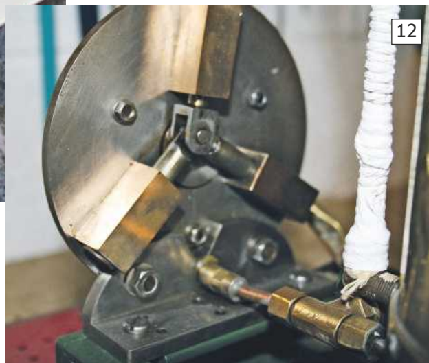
Photo 11. The three cylinder oscillating radial engine came complete as a plant but I have only ever run the engine on compressed air. It would be interesting to know just who built it and whether it was from a purchased design or a homemade design. Either way, it is fascinating to watch in operation.
