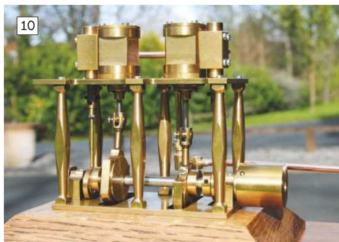
Photo 10. You can quite clearly see in this photo that the Hansen engine does not have a crankshaft. The piston rods and piston valve rods are all operated by eccentrics locked to a straight shaft. Simple, ingenious and a lot easier to manufacture than a conventional crankshaft.
