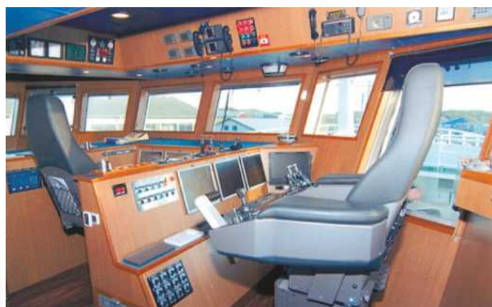
RIGHT: Starboard conning position in wheelhouse, with extended window depth to allow sight of net hauling operations. Photo courtesy of builder
