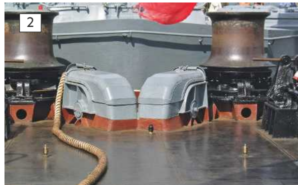
Photo 2. The cable holders and bonnets.
