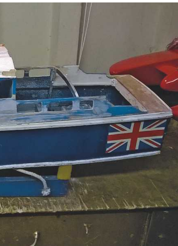
Photo 21. Thin strips of wood were glued and inserted into these gaps to overcome that problem. However, the inner surface of this starboard side had suffered some separation like the port side had to its outer face.
