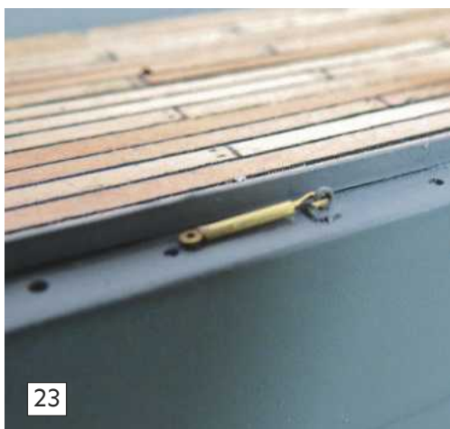
Photo 23. A bottle screw hooked to the eye plate ready to accept the thimble of the shroud.
