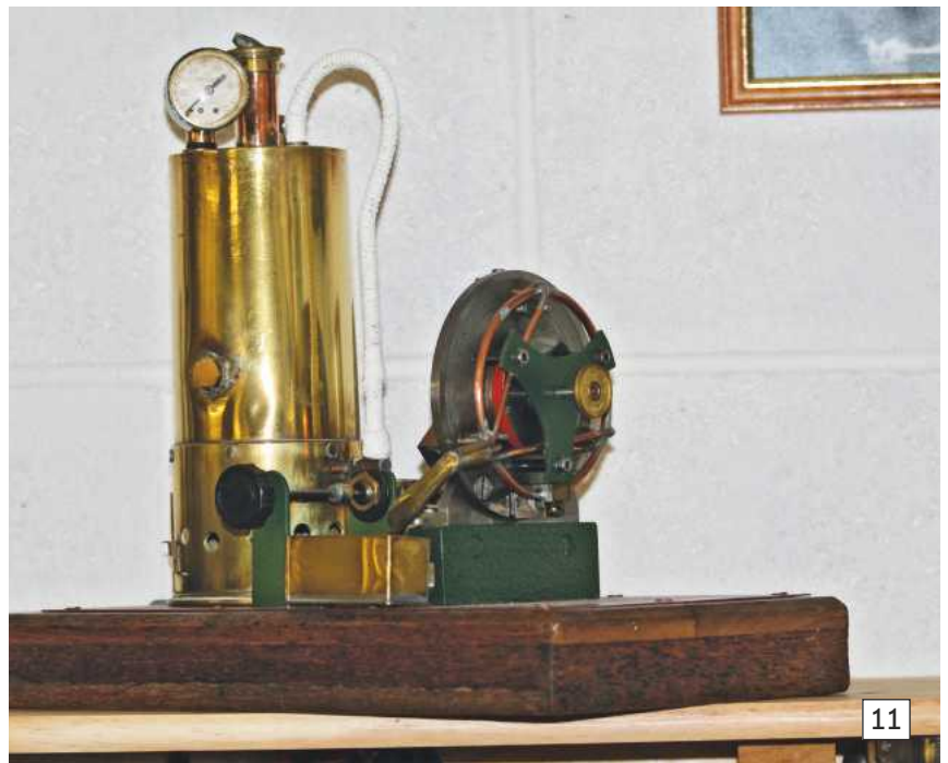
Photo 11. The three cylinder oscillating radial engine came complete as a plant but I have only ever run the engine on compressed air. It would be interesting to know just who built it and whether it was from a purchased design or a homemade design. Either way, it is fascinating to watch in operation.
