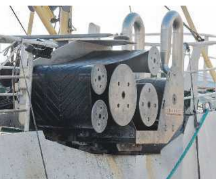
BELOW: View of net hauling winch in fore and aft position. Photo from author's collection
