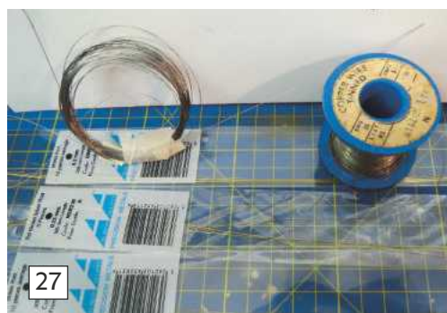
Photo 27. A selection of brass and nickel silver wire that can be used as the rail between the stanchions. If in doubt, always go thinner as at small scales the paint will (if brushed) add enormously to the scale thickness.
