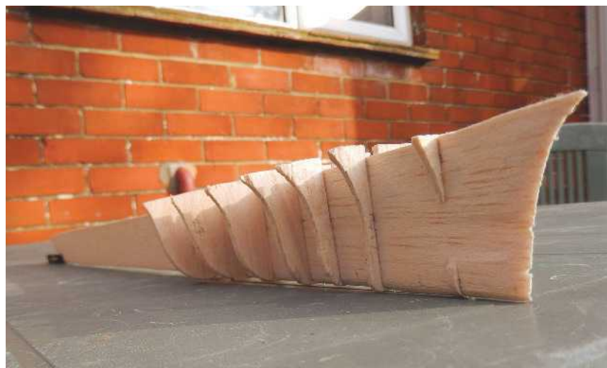
BELOW: The basic hull framework is of balsawood.
