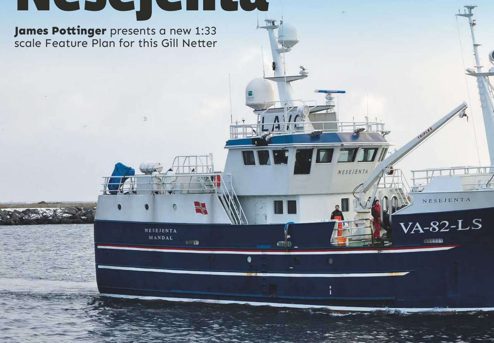
ABOVE: Starboard side, with the deck crane extended. Note the satnav dome on aft side of the after mast. Photo courtesy Frode Adofsen
