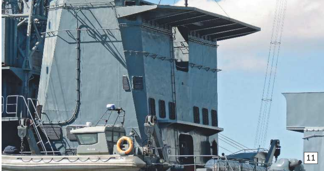
Photo 11 A view of the fore funnel uptake with its rear extension at the top.
