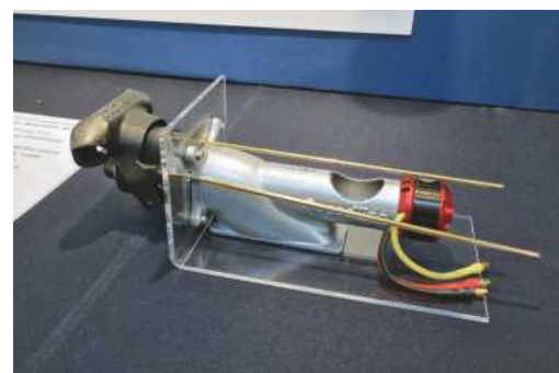
BELOW: Speedline Models will be introducing a brushless powered jet unit for their new Shannon lifeboat kits.
