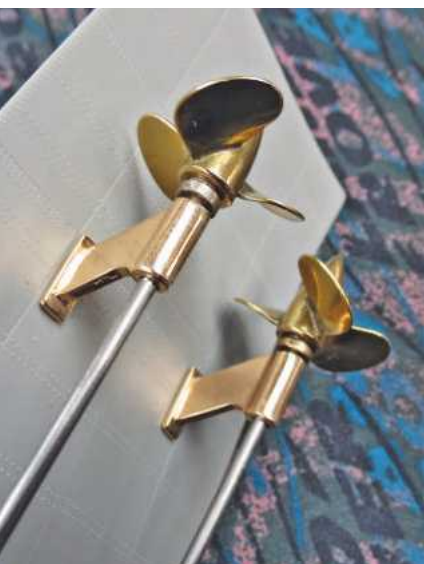
BELOW: The next step in 3D printing are metal fittings such as these propshaft supports.
