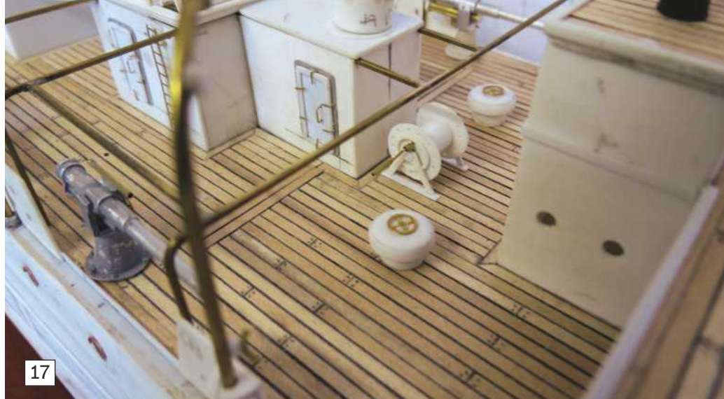
Photo 17. Temporarily positioned are the unpainted cordage reel and two large mushroom vents.
