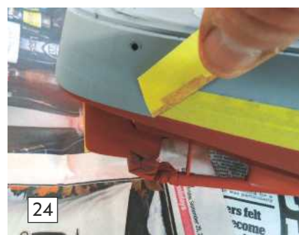
Photo 24. It is best to remove the low tack masking tape gently and at a slight angle to ensure a good clean edge.
