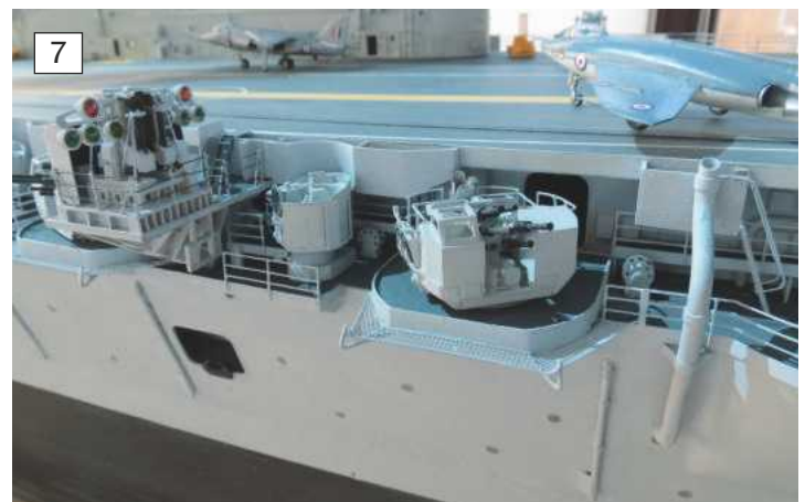
Photo 7. The Bofors Mk VI with its external director. Also in the picture is the deck landing aid, a British invention..
