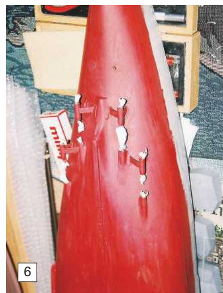
Photo 6. It is essential to get the four propshafts and accompanying A Frames all parallel. The paint helps highlight any hull blemishes that may need rectification.
