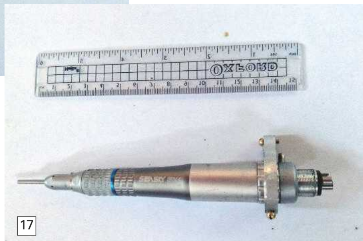
Photo 17: An overall view of a dental air motor, partly adapted for HMS Dreadnought. This is all very much an experimental project, but these motors are easily available from about £20 each, an unbelievable price bearing in mind the high quality engineering involved. These are NOT the high-pitched motors that are often associated with a trip to the dentist, but bench tests have been most encouraging as to the power output of these units which are 6 inches (15cm) long.
