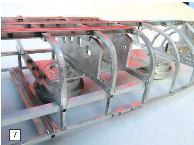
Photo 5: Looking aft and this is the pre-drilled plate for mounting the four miniature steam turbines.
