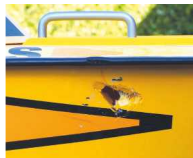
ABOVE: This two inch hole in the side of the Crusader was above the waterline so the boat still able to race, but it needed repairing for the next season.
