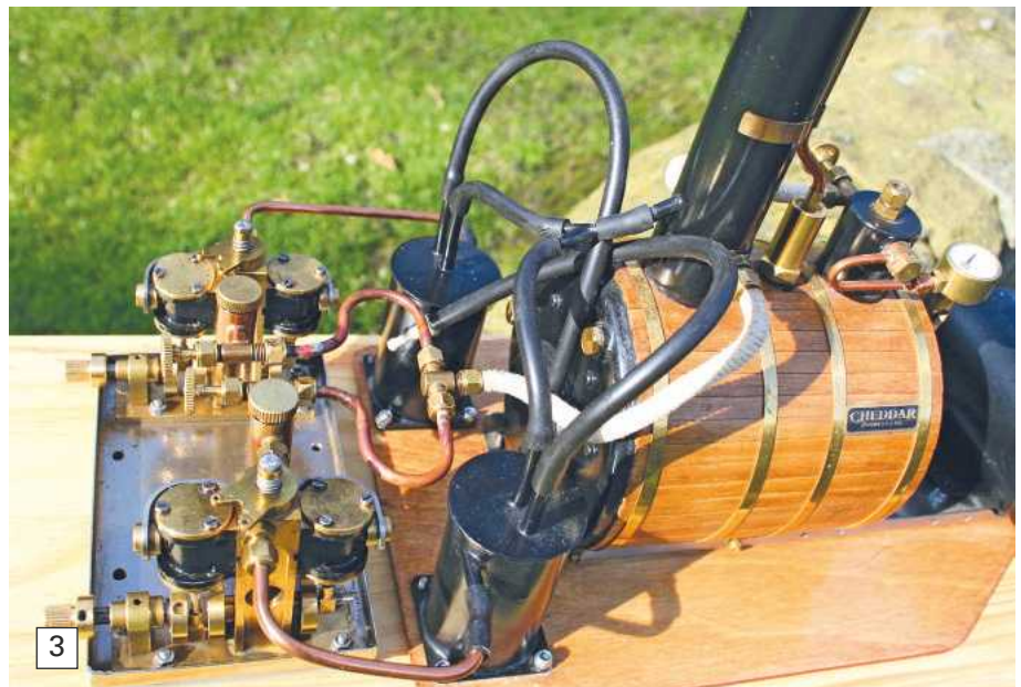
Photo 1. A Wilescot boiler, very similar in construction and capacity to a Mamod item or a Tony Green USE type of boiler. This one does have a safety valve and a sight glass, but no pressure gauge.
