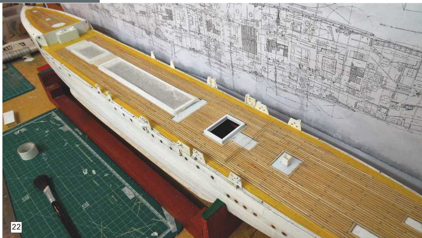
Photo 22. Masking the wood planked deck edge with Tamiya low tack tape in preparation for general masking of the entire planked area.
