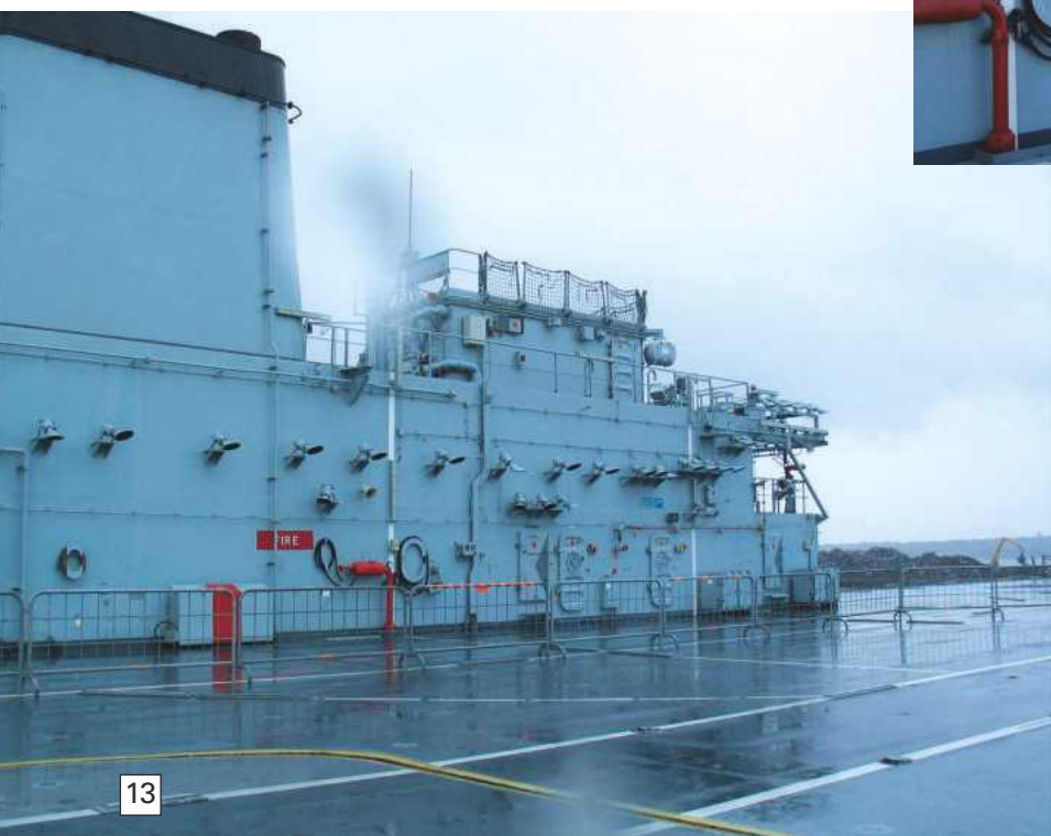
Photo 10. The island superstructure is quite large and causes airflow problems over the flight deck.
