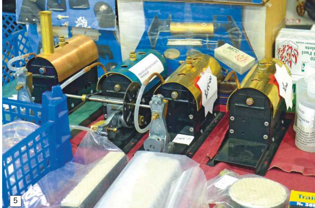
Photo 5. The Tony Green type of Simple Small Boilers. These are fired by solid fuel in the form of Tea Light candles and are particularly interesting in so far as they pivot up for easy, safe and convenient ignition.
