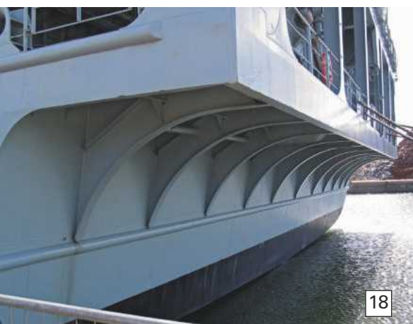
Photo 18. The structural arrangement beneath the stern flight deck overhang.
