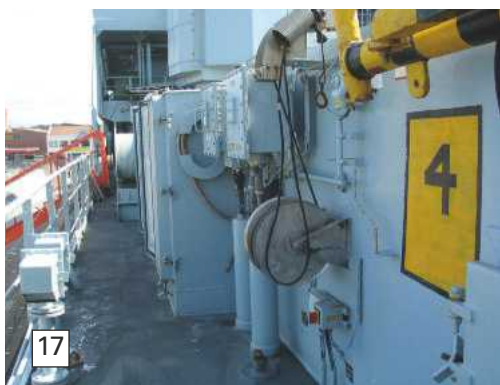
Photo 16. Part of the pipework for aviation fuel delivery.
