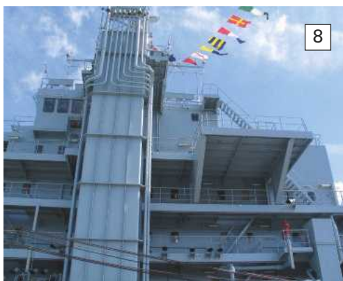
Photo 8. The hangar and air conditioning venting pipework is trunked to the top of the main superstructure.
