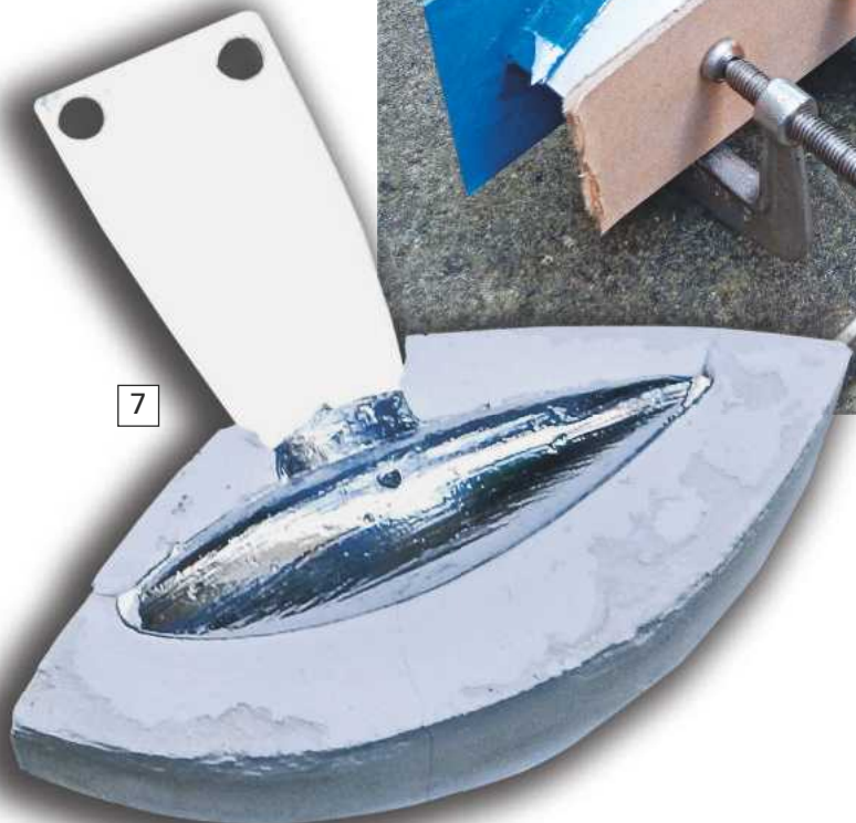
Photo 7. The new lead keel weight, cast around the aluminium plate, with the top half of the plaster mould removed.
