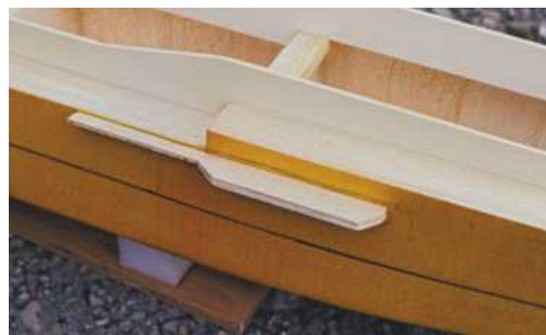
With a fresh felt tip pen, a crisp line can be scribed.
