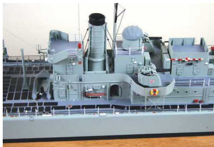
ABOVE: The aft deckhouse with the two twin 40mm Bofors guns.
