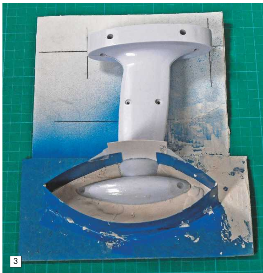
Photo 3. The plastic fin and bulb positioned in the mould box with its lower half filled with plaster.
