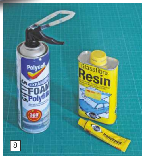
Photo 8. Right: Glassfibre resin and hardener was used to secure the weight and plate to the plastic fin and to seal the fin join on its inside edges. Left: Builder's expanding foam was used to fill the whole of the re-assembled fin.
