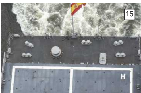
Photo 16. The transom has no large opening for a towed variable depth sonar system. The reason for the three horizontal rows of eye plates is not obvious.
