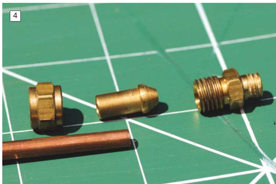
Photo 4. It sounds daft, but laying everything out before you start bending is a good idea. You can see where you want the fittings to end up, allow for their length, as well as see much they may affect the bend positions.
