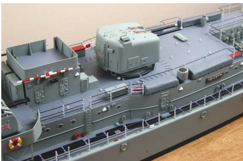
BELOW: The aft 4.5 inch turret. The grey covered objects on the upper deck edges by the railings have liferafts within them.
