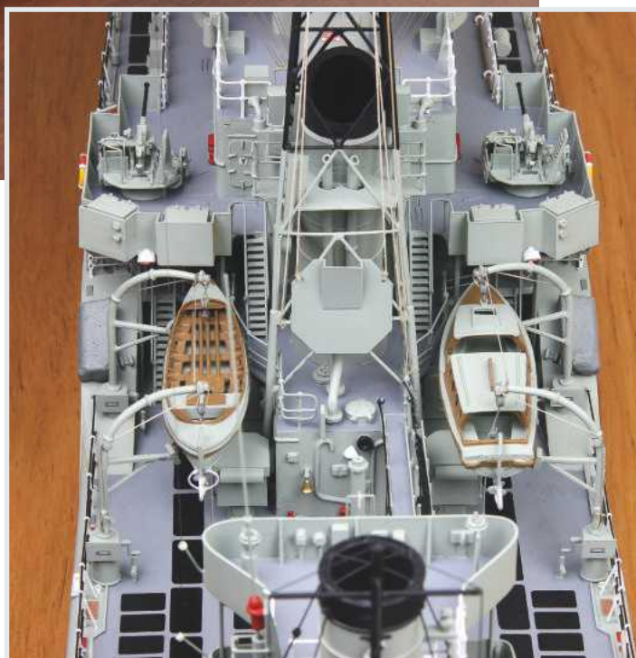
BELOW: The aft 4.5 inch turret. The grey covered objects on the upper deck edges by the railings have liferafts within them.
