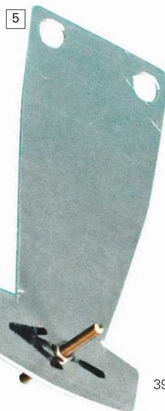
Photo 5. The aluminium plate with brass studding and nuts to ensure it will remain central in the plaster mould when the molten lead is poured.
