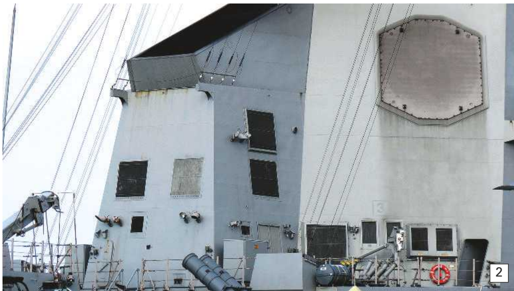
Photo 2. The forward exhaust casing is attached to the forward superstructure block housing the Aegis system.
