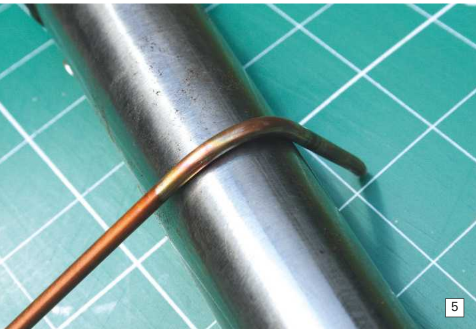
Photo 5. Never underestimate a lump of bar stock as a bending tool. Anything can be used as you will normally be bending the pipe 'cold'.
