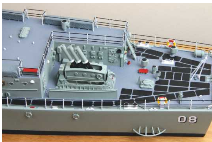
ABOVE: HMAS Vendetta had an anti-submarine role with the Limbo mortar mounted aft.
