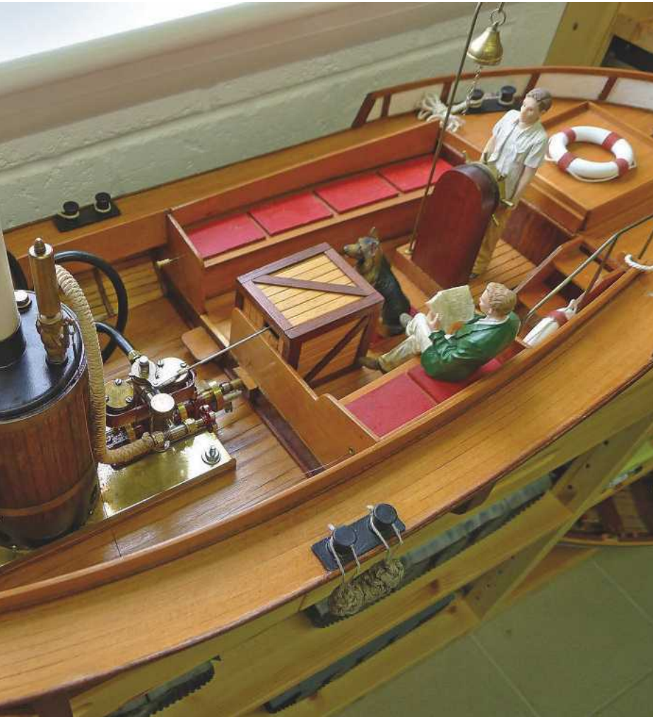
Photo 1. The starting point, a model with any suspicion of scale or sludge in the boiler needs an internal cleaning and a blocked sight glass is just that.
