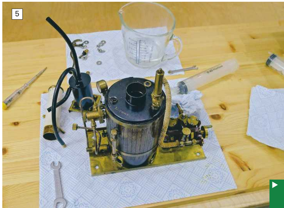
Photo 5. A little bit of care will ensure that you do not splash a single drop and you can fill the boiler right up to its brim, ensuring every internal part gets cleaned.
