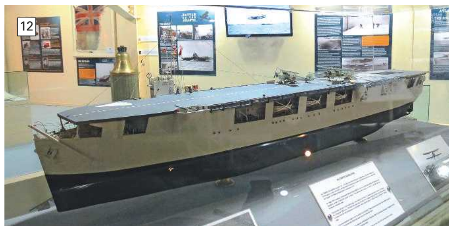
Photo 12. As there was a lack of purpose built escort carriers to protect the convoys during the early part of the Battle of the Atlantic in WW2, the solution was to convert merchant ships with a flight deck running the length of their hulls, as seen on this model.
