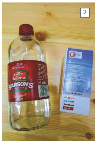
Photo 2. The two likely candidates for the pickling liquid. Vinegar is of an unknown strength, but the descaling tablets are designed for the job and worth that little bit of extra expense.
