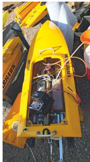
ABOVE: Andy Rennie's CMB 21 powered Challenger – note the large fuel tank amidships.
