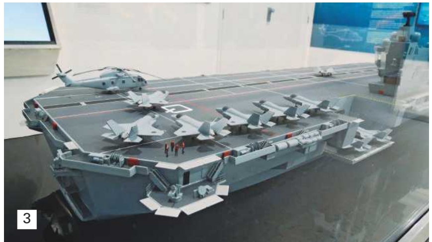
Photo 2. The new aircraft carriers retain a ski jump to assist the STOL capability of the F35B Lightning 2.
