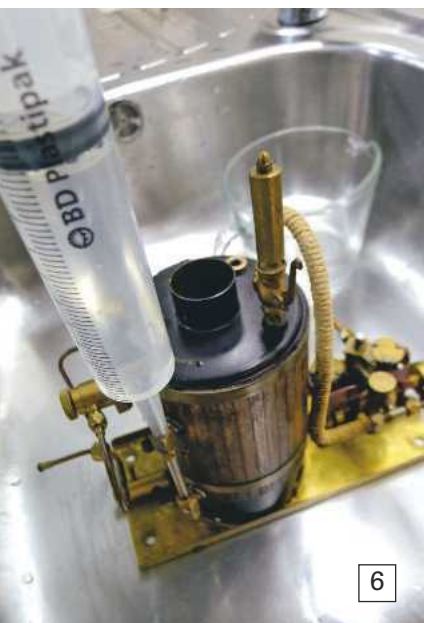
Photo 6. After a thorough flushing, the final process is to also give the sight glass a good flushing through as well, with as much pressure as you can generate at the syringe. This should ensure that the connections are nice and clear and you are going to get a reliable reading from the sight glass.
