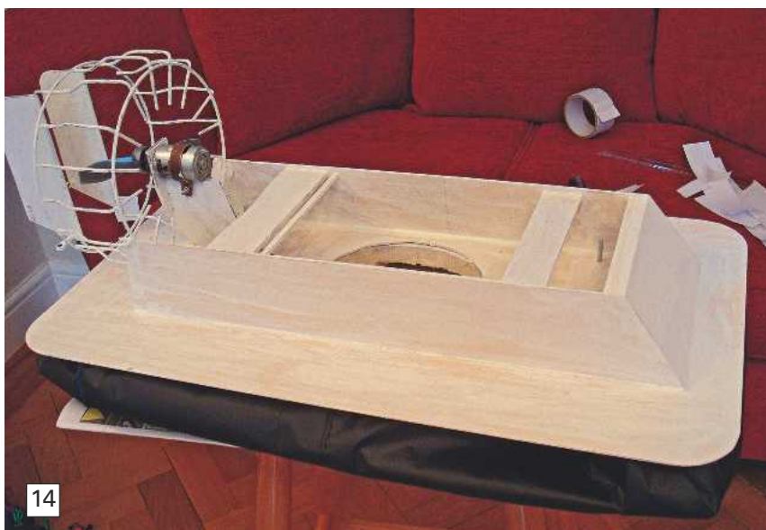
Photo 12: Securing the skirt to the top of the lift duct
