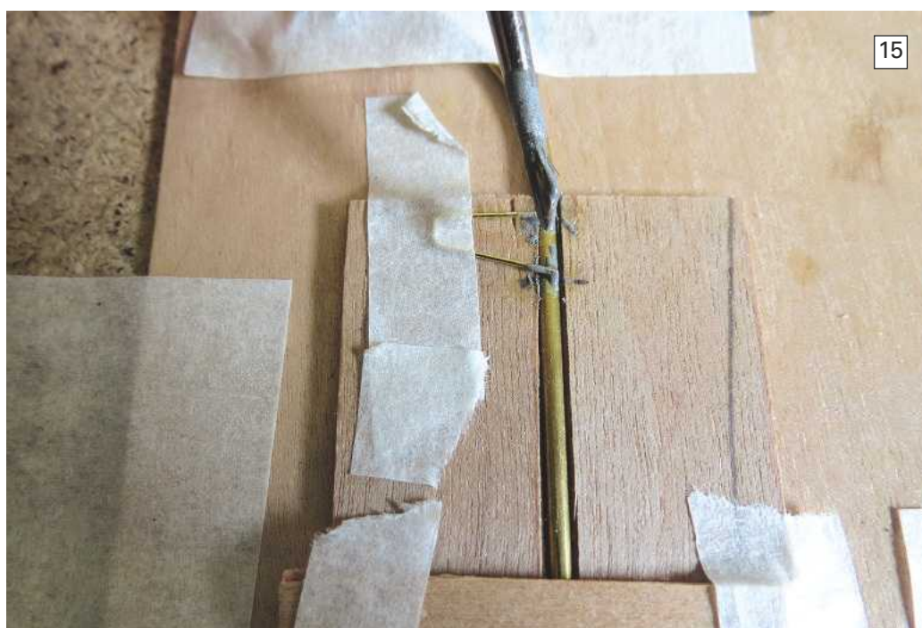
Photo 14. Making use of a simple timber jig to hold all the parts in place ready for soldering.
