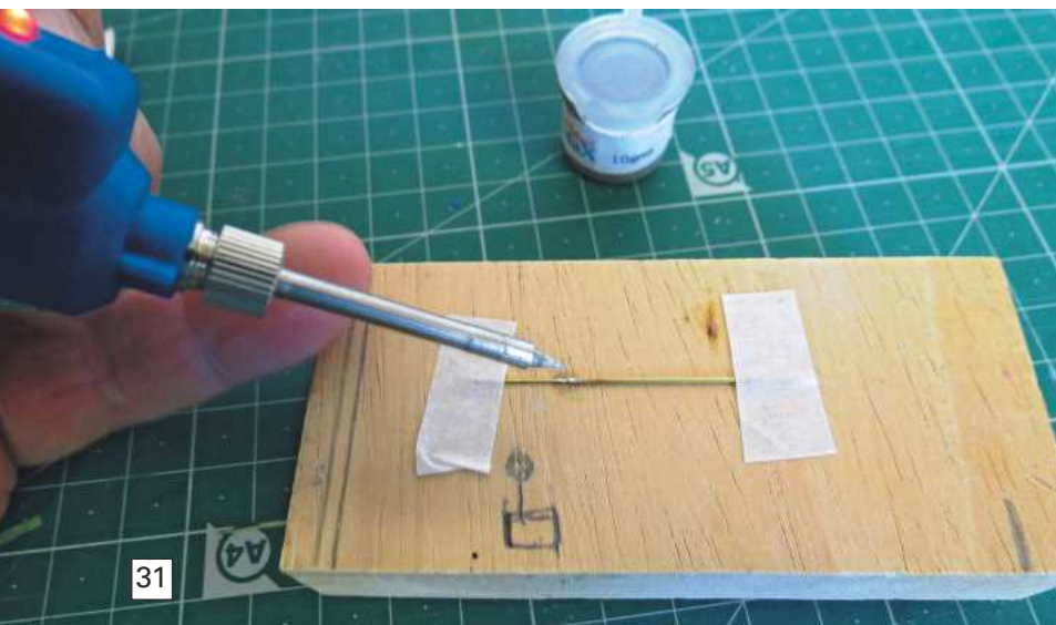
Photo 30. An 8 Watt battery powered soldering iron, whilst limited in capability, does have its uses, especially in fine soldering work such as with photo etched components.
