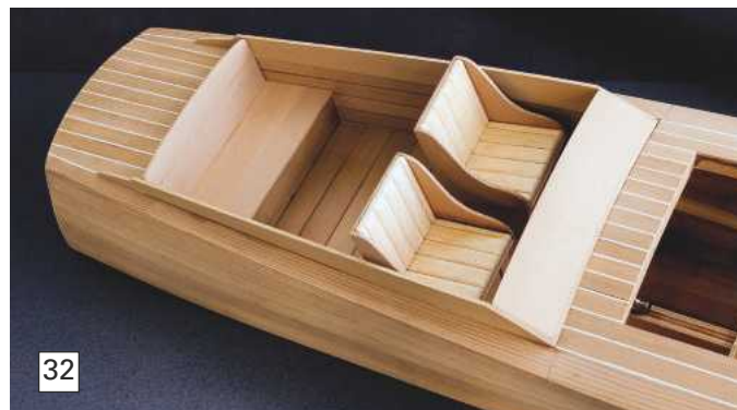
Photo 29: Fitting of the cockpit lining panels, each held with a single screw.
