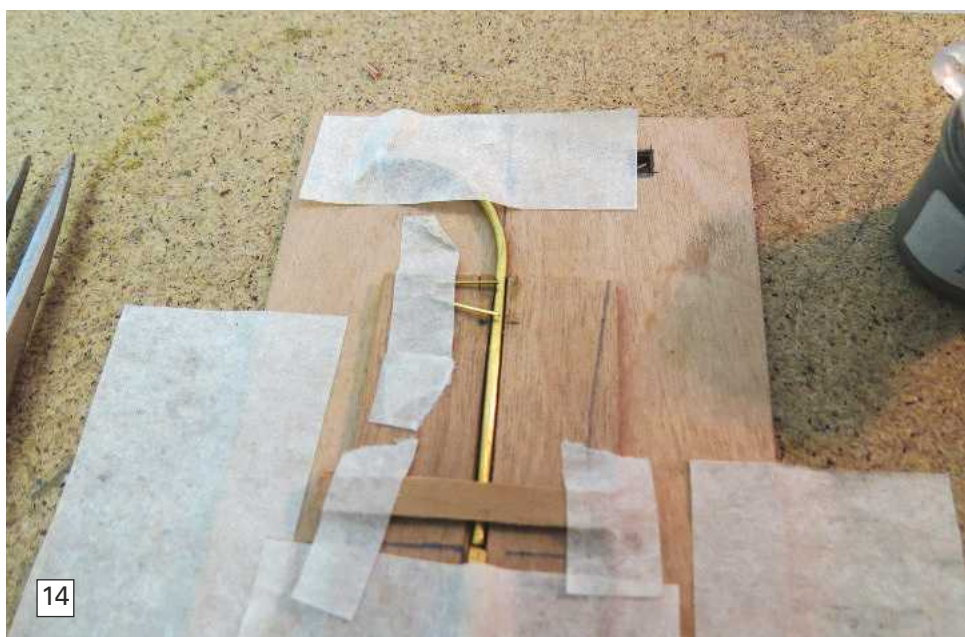
Photo 14. Making use of a simple timber jig to hold all the parts in place ready for soldering.
