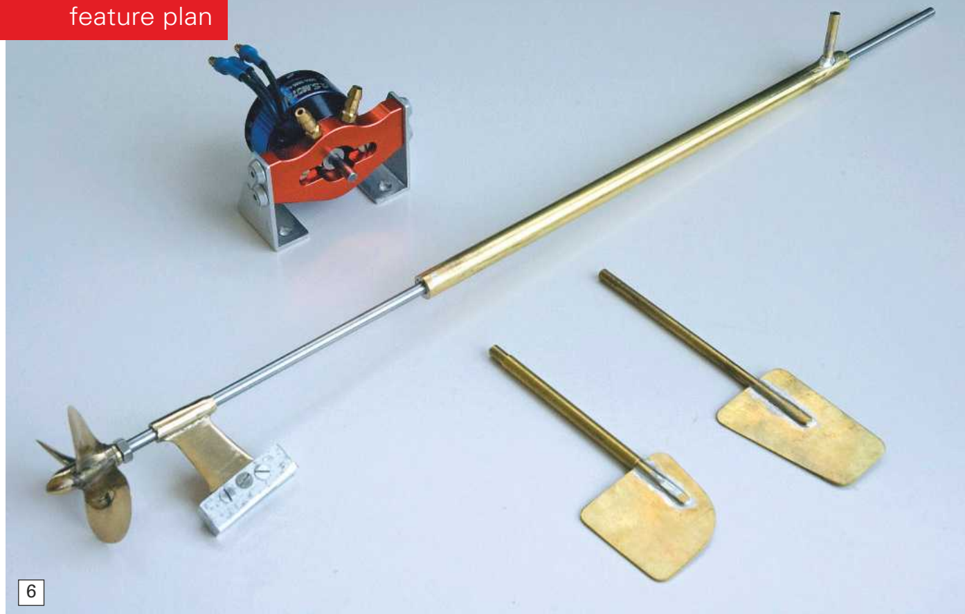
Photo 6: Running gear: Motor, exposed propshaft and alternative rudders.
