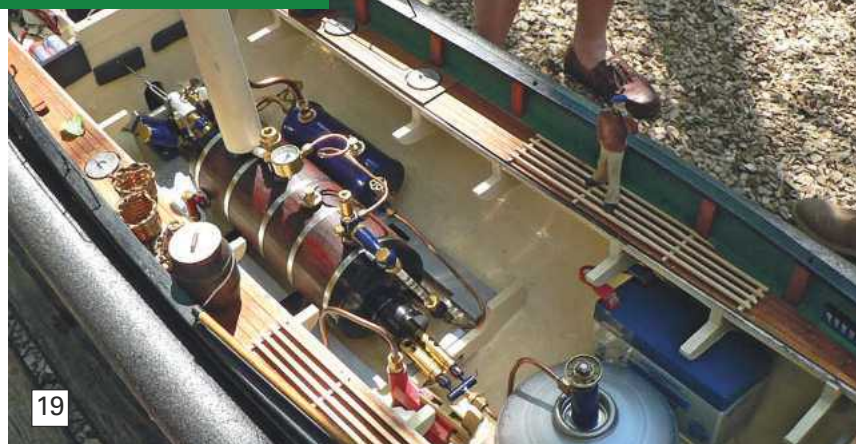
Photo 19. A complete assembly of a Hemmens steam plant in a Hemmens model boat. The hull has plenty of room to work in, and allows for a relatively straightforward assembly process.
