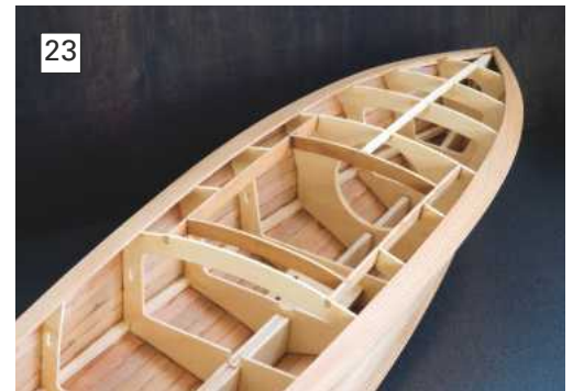
Photo 19: Completion of hull planking – prior to cleanup of sides.
