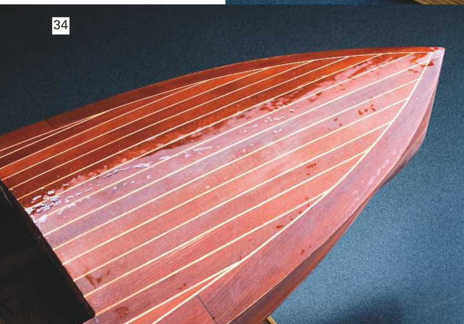
Photo 34: Sanding progress with starboard side still showing a few low spots.
