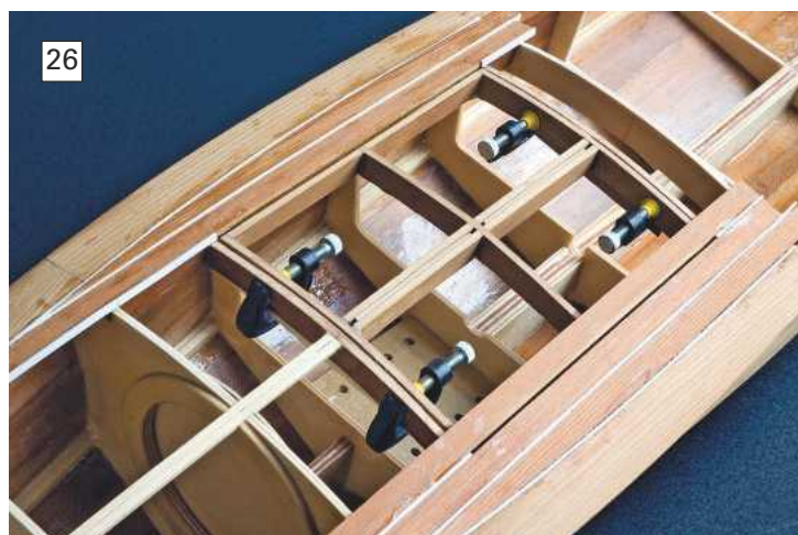
Photo 26: Interior sealed and deck planking underway.
