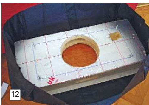
Photo 11: Securing the skirt to the baseplate
