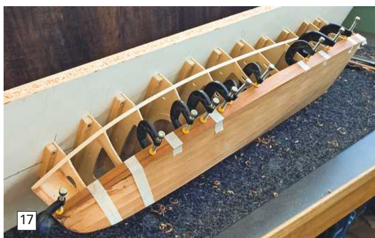
Photo 15: Commencement of planking at the keel.
