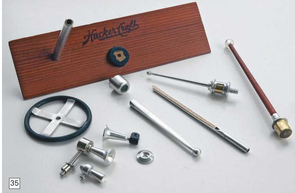
Photo 35: Fittings, including a section of filed rubbing rail and a sample control horn used in making the jackstays and a horn for the deck.
