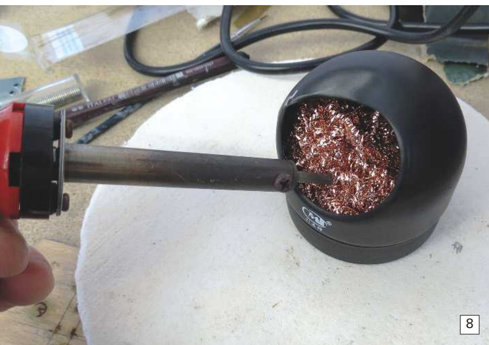
Photo 6. Tip maintenance is an essential task and 'tinning' it with a layer of solder ensures a better transfer of its heat to the job.
