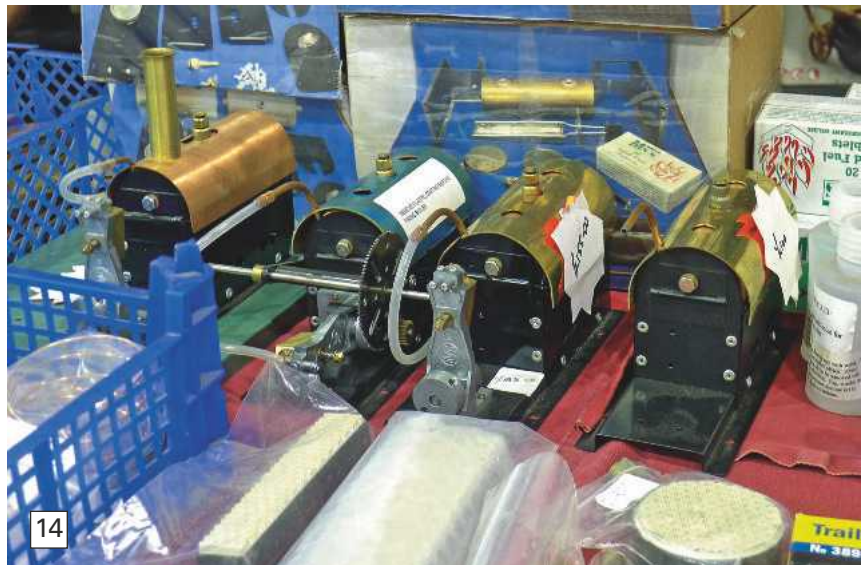
Photo 14. Despite being solid fuelled boilers, the Tony Green range all hinge open so they can be lit in place, making them a lot safer than some others of a similar capacity.
