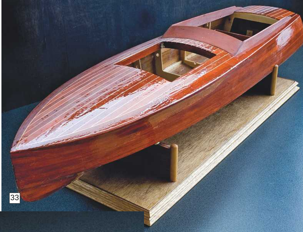
Photo 33: Hull is stained and epoxy coat applied, prior to wet sanding.
