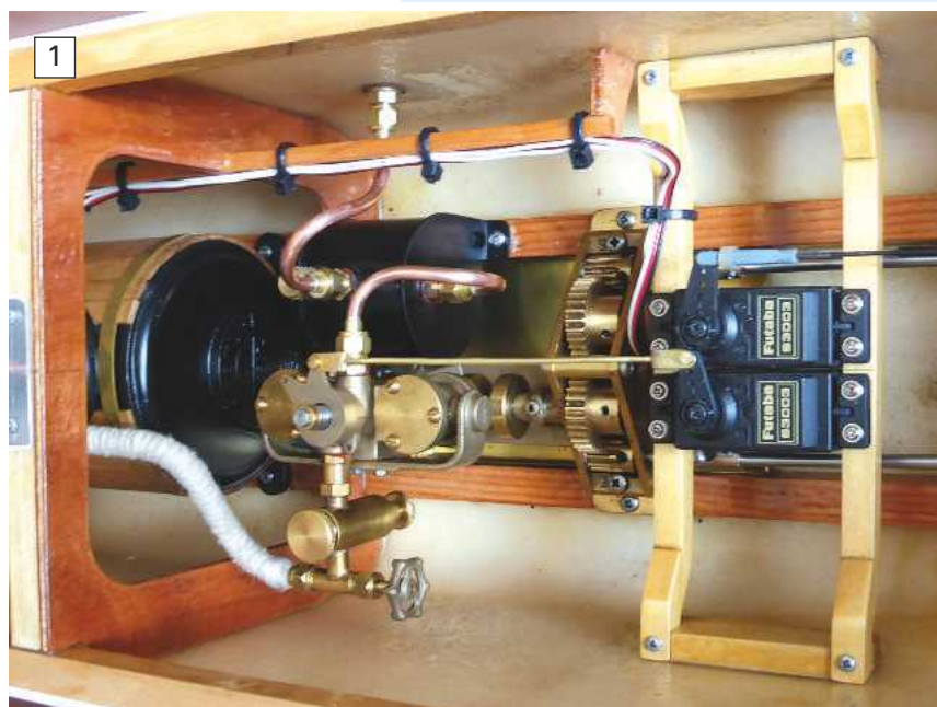
Photo 1. The original Clyde oscillator engine propulsion machinery. Only one servo is needed for engine control.
