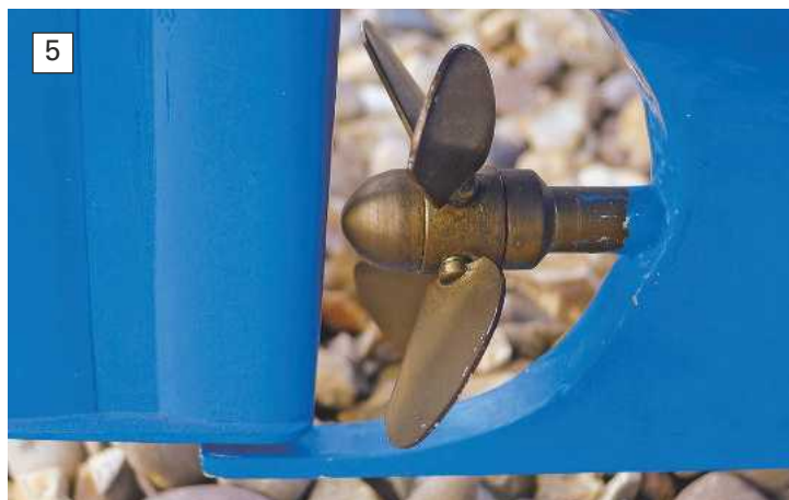
Photo 6. With the mechanism fully over in the opposite position, the blades are now in the full-ahead position. If you compare the angle of the blade to the perpendicular you will see in both cases that the blades are a similar angle on either side of it.
