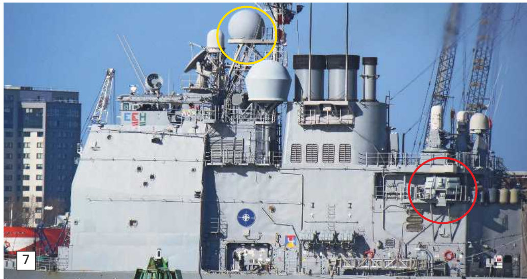
Photo 7. Viewing the port side of the bridge, it's worth noting the absence of the SPY-1 panel. That particular panel is aft on the port side of the hangar.
