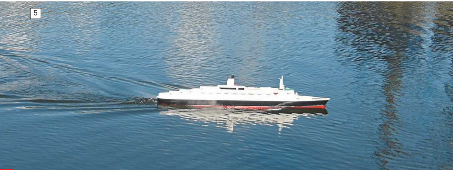
Photo 5. The QE2 model now runs at 2.2 knots, which is equivalent to 31.2 knots for the full-size ship and notably its wake also now looks so much better and truly realistic.
