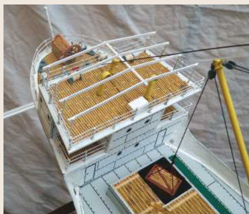
ABOVE: The quarterdeck awning framework was all created using the milling machine.
