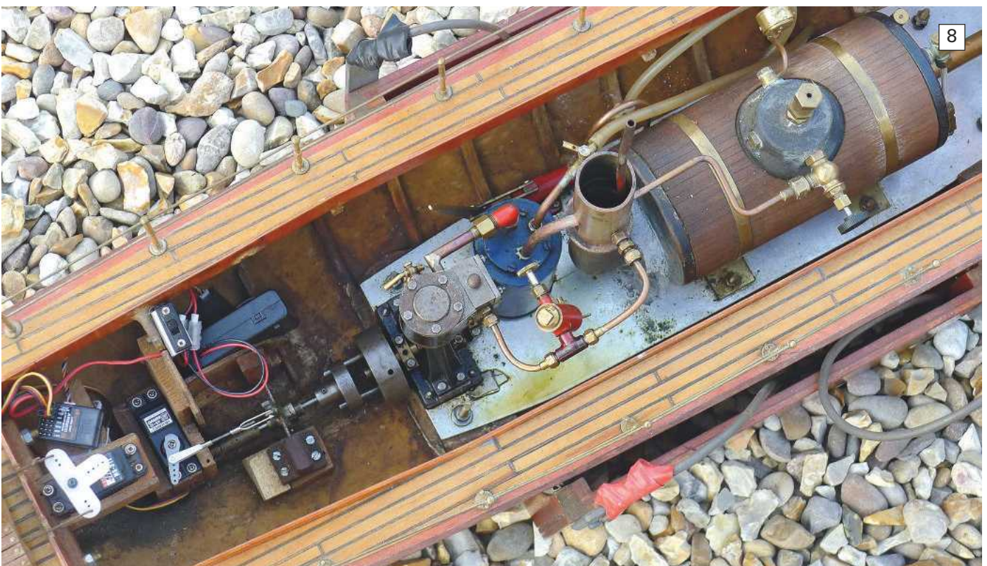
Photo 8. The complete internal layout showing the boiler, engine and controllable pitch mechanism. It is quite obvious here than a twin cylinder engine of a similar size would be a very tight fit as well as being unnecessary, but there is adequate room for the required control modifications.
