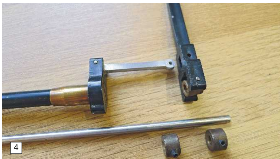
Photo 4. At the control end the operating arm pivots about the end of the aluminium arm and the bronze bush at the bottom pushes against the bronze bushes attached to the shaft. This enables the propshaft to be either pushed into the tube or pulled out of the tube.
