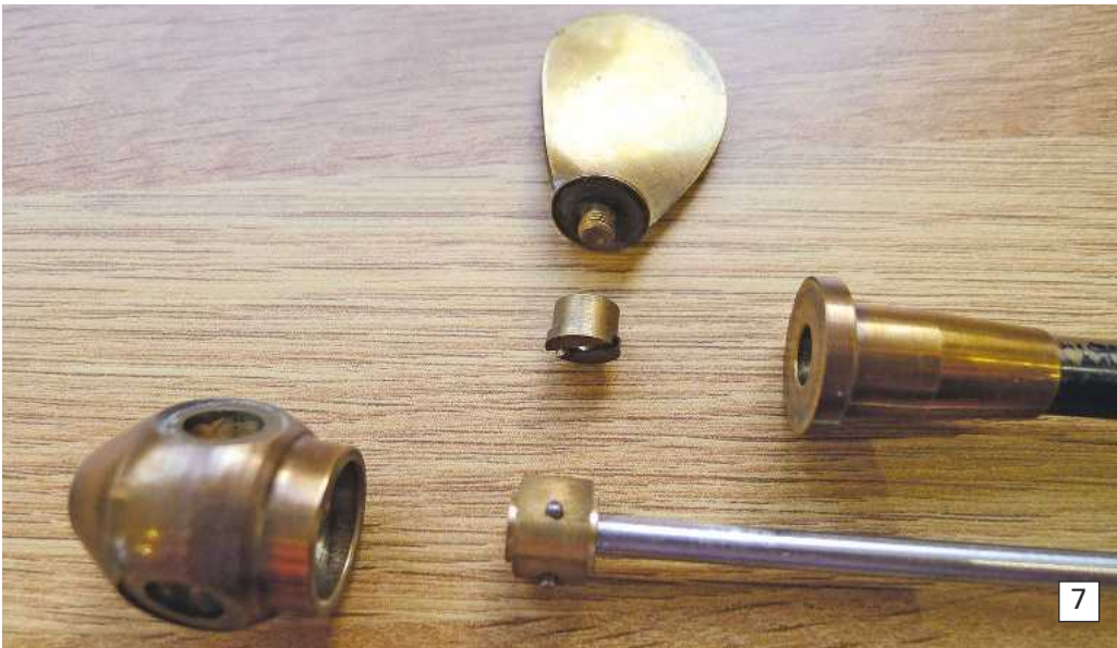
Photo 7. At the 'business' end you can see the brass block on the end of the shaft fitted with the pins on the flat faces offset to the centre line. These locate in the slot in the brass bush with the blade screwed into the top of it. As the pin moves backwards and forwards, it moves along the slot and so the blade's angle of attack (pitch) changes.
