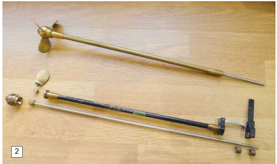
Photo 2. Two similar brass controllable pitch propeller units in their respective tubes. The top one is assembled, but without the operating arm and the lower one completely dismantled to show the internals and their relationships with each other.
