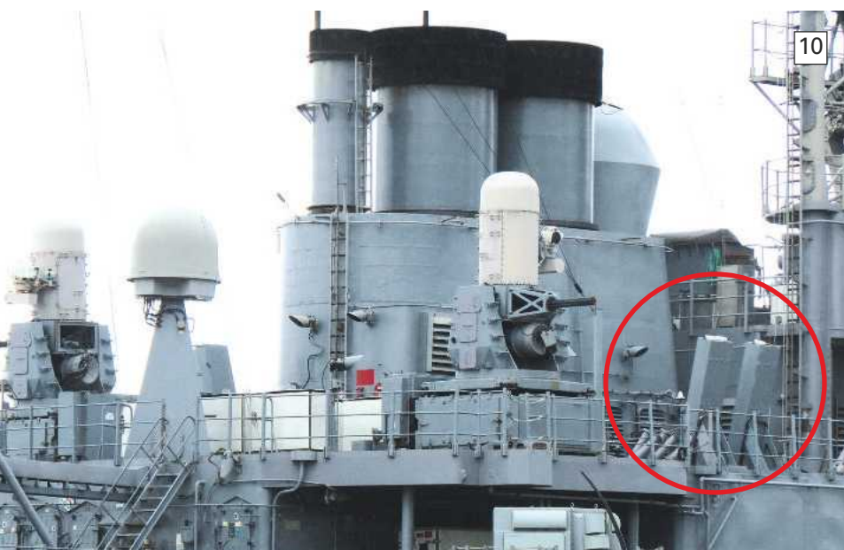
Photo 10. Two Mk. 15 Phalanx CIWS with the Nulka launch boxes circled in red - please see text.
