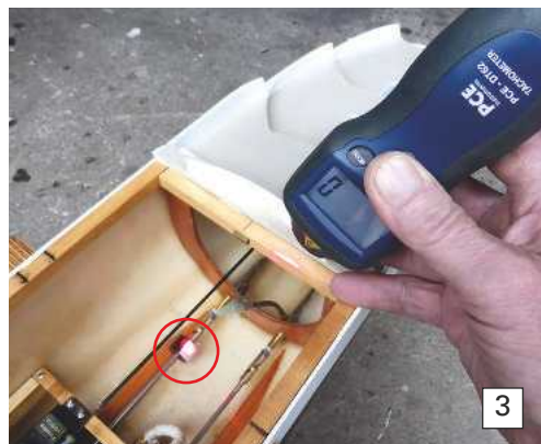
Photo 2. An 18mm diameter black painted aluminium cylinder with 12 x 12mm self-adhesive reflective tape, has been fitted to the starboard propshaft.
