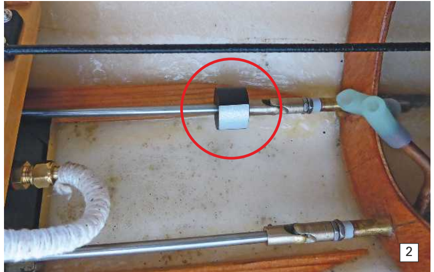
Photo 2. An 18mm diameter black painted aluminium cylinder with 12 x 12mm self-adhesive reflective tape, has been fitted to the starboard propshaft.
