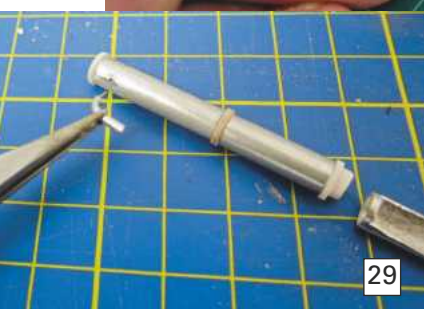
Photo 29. Using 1.8mm o.d. tube for the firing valve housing which is added to the breech end of the tube.
