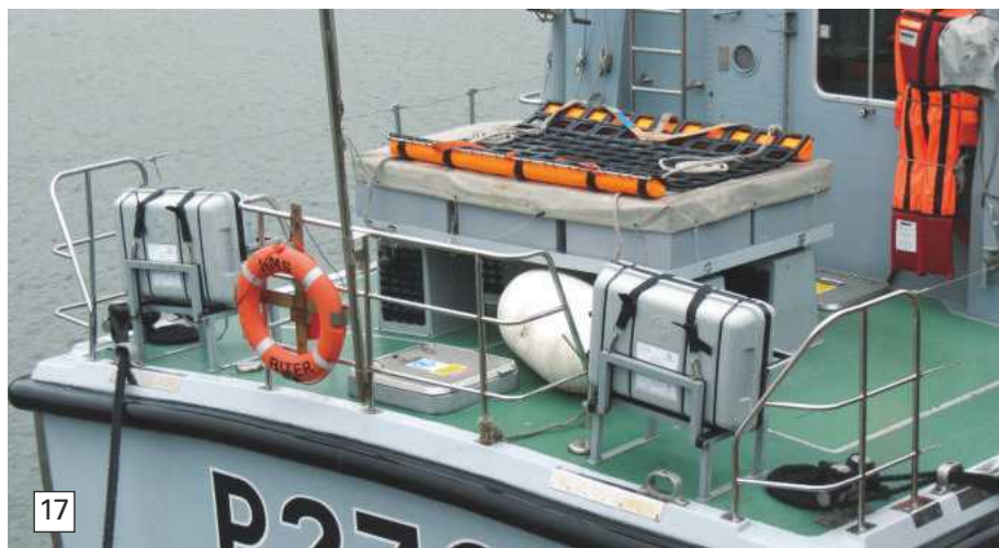
Photo 17. Viewing the quarterdeck and it's worth noting the camber on it and that all the handrails are of stainless steel.
