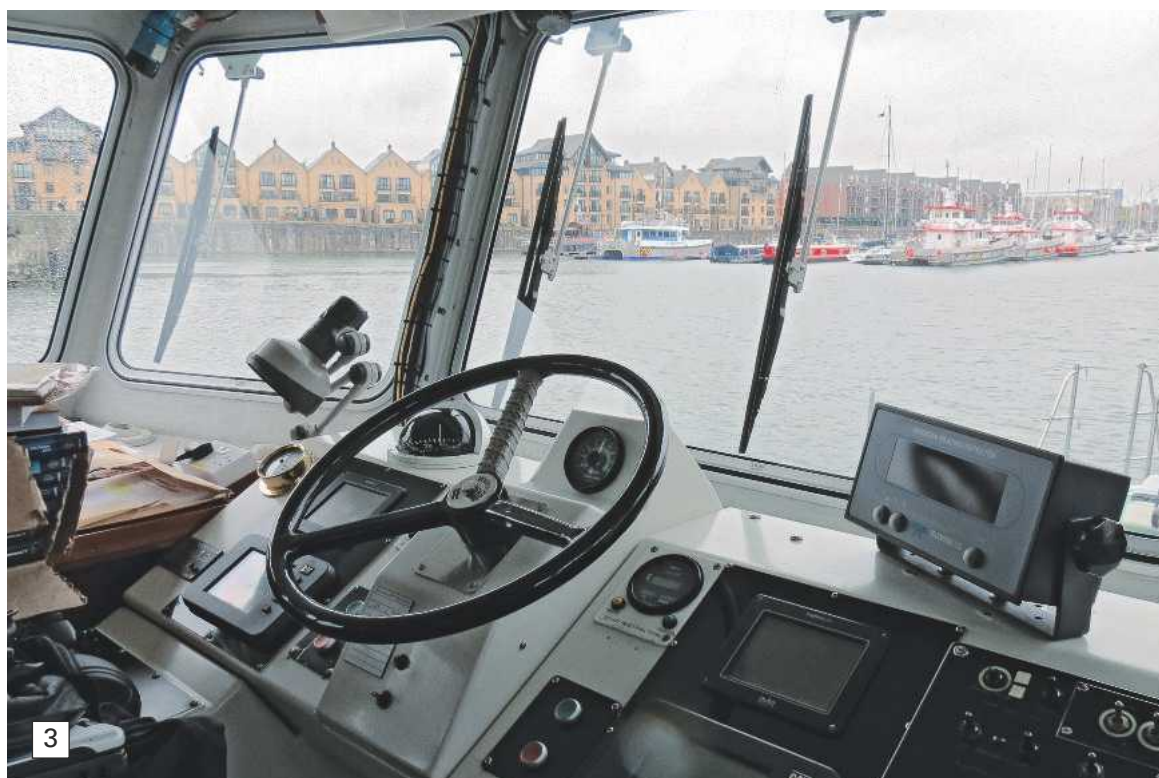
Photo 3. Inside the internal navigating position, it's interesting to note that the helm is a conventional steering wheel rather than the smaller half-wheels of those aboard such vessels as the larger RN River class.
