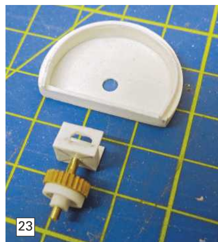
Photo 19. The three basic parts for the semi-circular turntable torpedo tube mounting.
