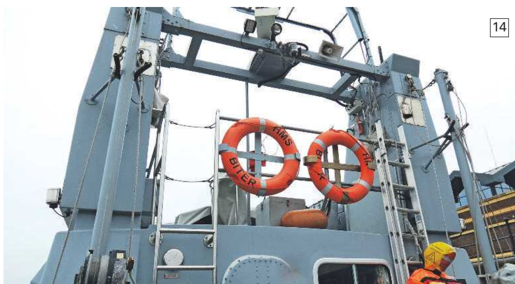
Photo 14. There are identical lifting posts, port and starboard, and you can also see the design of the cross bars at the base of the mast.
