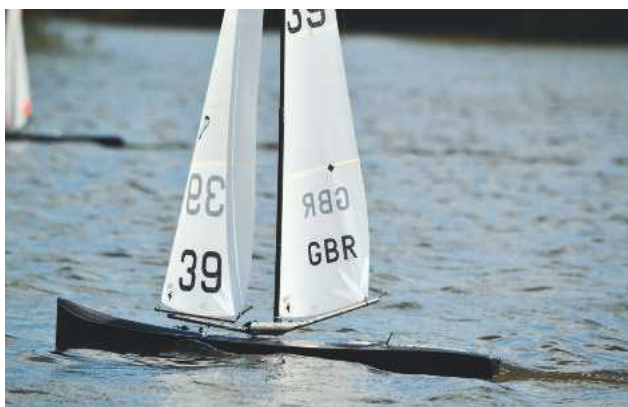
BELOW: Peter Stollery's INSIDE EDGE has an offset pivot swing rig. (Photo courtesy of Sue Brown)
