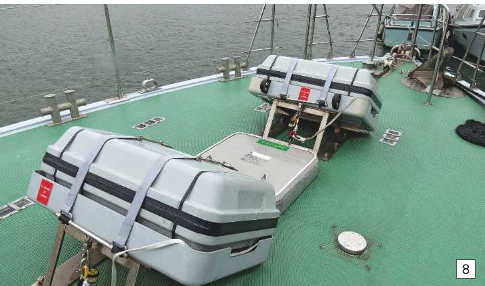
Photo 8. Two box type liferaft containers are mounted forward.
