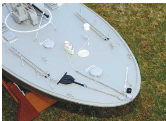
ABOVE: Foredeck detail: The anchor is principally from 1/16 inch plywood.
