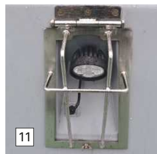
Photo 11. On the lower half of the superstructure front are two waterproof deck lights in protective coverings.
