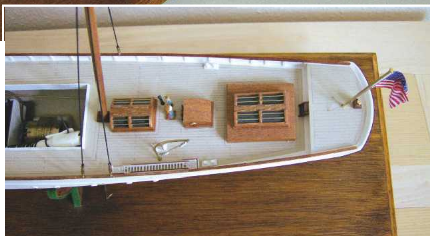
ABOVE: The skylights and companionway are built around balsawood formers.
