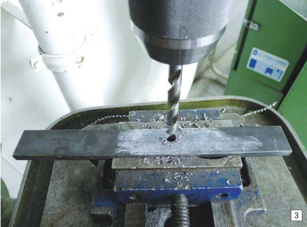
Photo 3. Ideally, whatever you drill your hole with, can then be used to hold the tap, be it either a drill press, milling machine or lathe. Always use the correct size drill for the thread you are cutting to prevent broken taps or sloppy threads.
