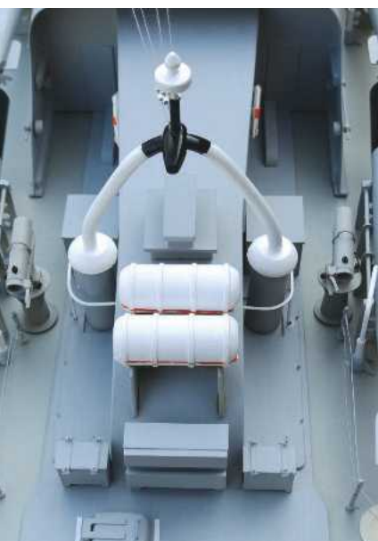
BELOW: The liferafts have been created from rounded off lengths of 3/4 inch (18mm) dowel with thin card strips added before painting. The mast is of copper tube with car washer tubing forced over it to increase the tube's girth.
