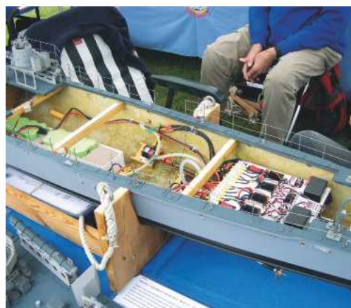
RIGHT: The interior of Hilary Breeze's revamped MTB 777, now with brushless motors, and boy, does it go!
