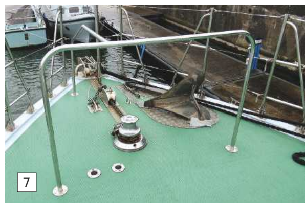
Photo 6. Although only 54 tons and 20.8m in length, the anchor handling arrangements still require a cable stopper and Blake Slip.
