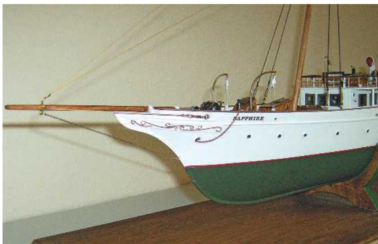
BELOW LEFT: The planking is actually coloured Fablon self-adhesive covering material, cut to shape and carefully marked in pencil.
