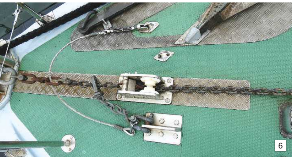
Photo 6. Although only 54 tons and 20.8m in length, the anchor handling arrangements still require a cable stopper and Blake Slip.
