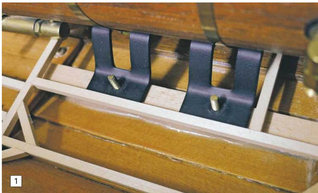
Photo 1. This captive nut process allows us to use mechanical fastenings thus enabling us to dismantle parts of the model for servicing. Sometimes a bespoke threaded component may be required which you might want to tap yourself.
