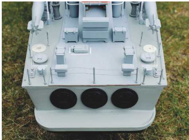
ABOVE LEFT: The three large exhaust outlets have been made up from timber discs with hinge detail added. The railings are dowel posts drilled for thin wire to pass through.
