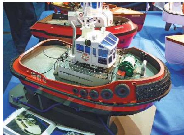
ABOVE: Numas Warrior, an unusual tug by Alan Wyatt of Kirklees MBC and which includes a pair of completely home built Schottel drives.
