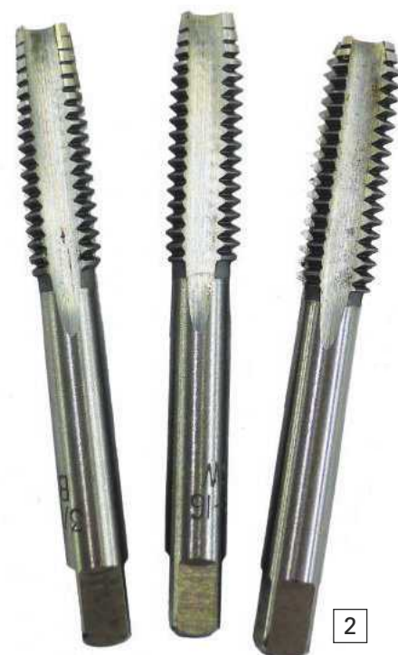
Photo 2. Although many taps now come just in pairs, traditionally a full set of taps would include three taps with from left to right: The Taper; The Second (or Plug) and the Bottoming Tap.
