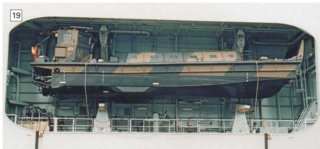
Photo 17. The mast is designed to fold down aft, so as to clear the davit.
