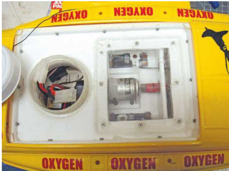
The completed internal watertight box with lid. The batteries are under the round access cap.
