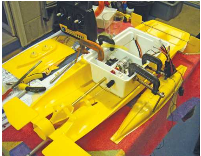
The internal watertight box under construction.
