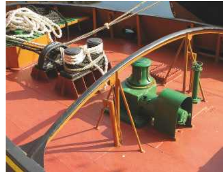
ABOVE: The aft deck of the preserved tug Brocklebank in Albert Dock, Liverpool. Again, this is very much shows the aft arrangement of an electrically driven capstan, bollards and eye plate. The notable point being that traditional tug deck fittings changed little over the years.
