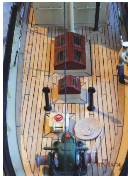
ABOVE: Foredeck detail - note the superb deck planking and neatly joggling around the edges.
