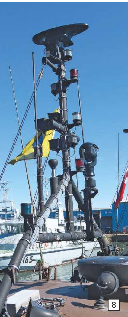
Photo 8. There is a short mast that supports the navigation lighting and radar.
