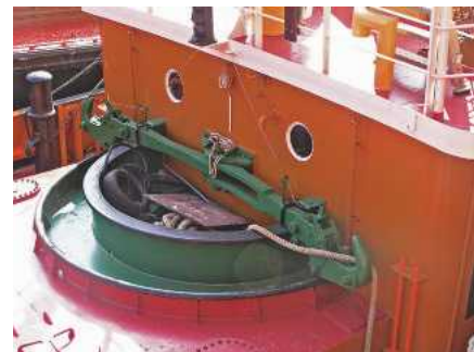
ABOVE: A close-up of twin tow hooks on Brocklebank mounted on a common pivot and support rail. Note the emergency trip wires which lead to the helmsman, in order to release the tow in an emergency.
