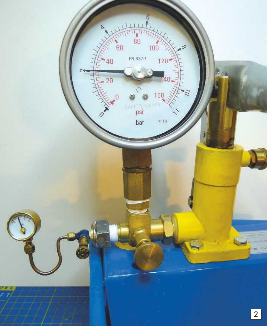
Photo 2. A typical club test rig to be used for boiler pressure tests and to check the calibration of the model Pressure Gauge. The rig's gauge is sent away for calibration and re-certification every two years and the certificate kept available.
