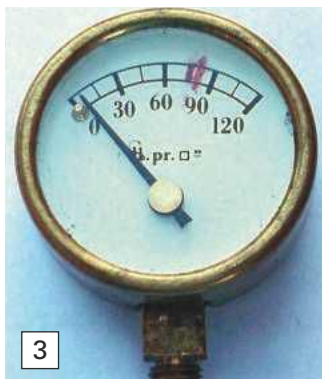
Photo 3. Challenges with the marking on the glass are: A) The glass can come loose and rotate; B) The red mark can be eroded away; C) Parallax error can be quite significant with a relatively big difference compared to the small scale.
