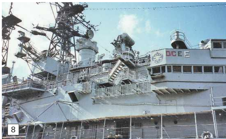
Photo 10. The 6 inch gunfire control director forward of the foremast.
