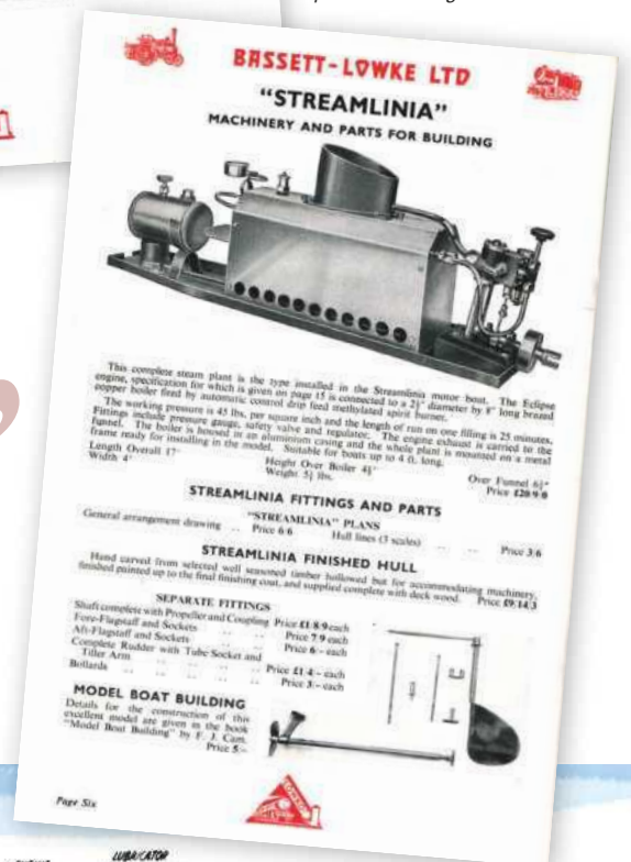
BELOW: Streamlinia's power plant and fittings details.
