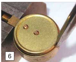
Photo 6. Then you should find that the bezel on the opposite side to the mounting is a lot easier to push down with the same screwdriver. Obviously take care not to scratch the housing, but also take great care that the mounting does not slip down in the vice. You might find it easier to hold the mount at 90 degrees so you are actually pushing against the vice jaws and not relying on the grip.
