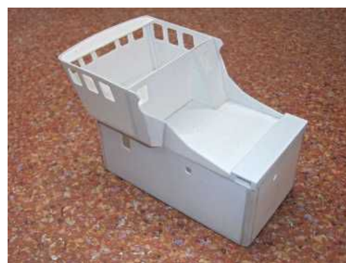
ABOVE: The main superstructure block and wheelhouse is assembled from styrene sheet.
