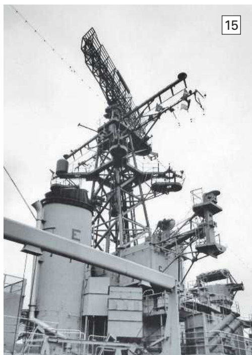
Photo 17. An early version of Chaff launcher having a similar purpose to that of the RN Corvus device. These were (and are) a defence against anti-ship missiles and hope to confuse their homing devices.
