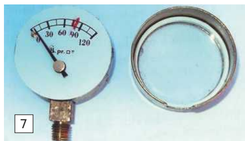
Photo 7. With the bezel off, you can mark a nice neat red line on the scale. If you are particular you could use a paint pen or even a thin strip of modelling decal or red tape and then seal it in with a coat of clear varnish.
