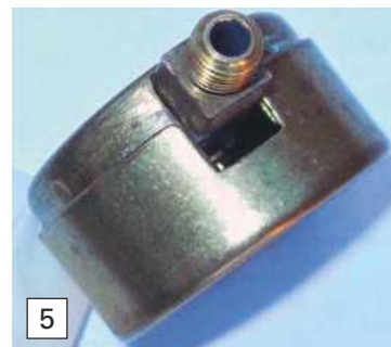
Photo 5. Once the bezel has started to move it should be noticeably clear at the base and now no longer sat on the housing square.
