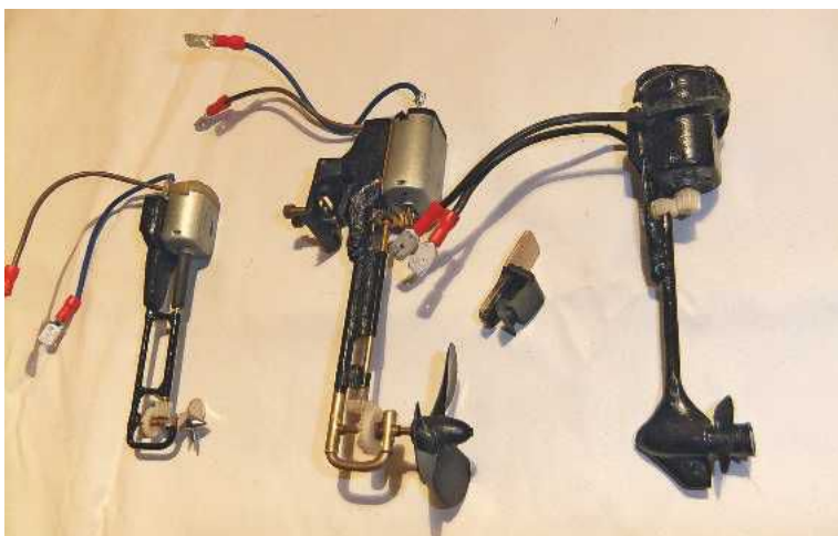
Photo 12. These are examples of contrate geared electric outboard drives, made (as they say) somewhat earlier.
