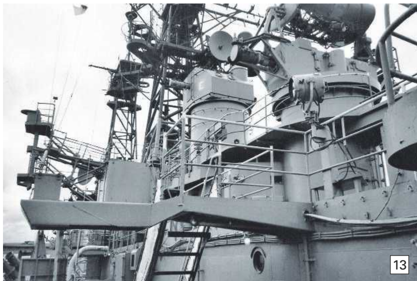
Photo 13. An excellent picture on the starboard side on 01 deck. The Mk. 35 director with the letter E on the side is, apart from the radar, vintage WW2.
