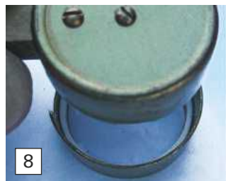
Photo 8. Place the bezel face down on a flat surface and then drop the housing into it, taking care to align the slot in the bezel and the mounting.
