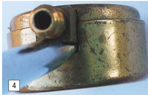
Photo 4. A small fine-bladed screwdriver will work perfectly to lever the bezel away at the base where you can push against the substantial mounting fitting.
