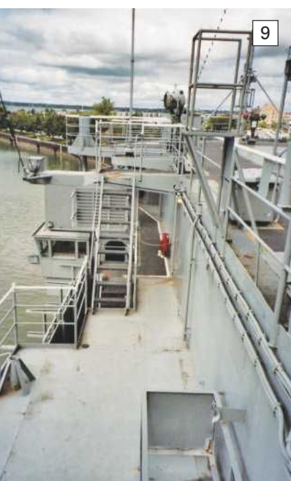
Photo 8. The gunfire control directors were retained, but the original pole masts were replaced by lattice versions.
