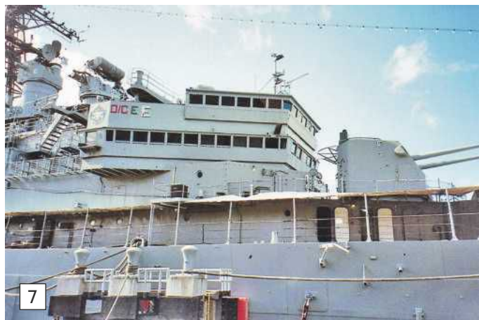
Photo 7. The bridge on USS Little Rock was extensively rebuilt during the conversion.
