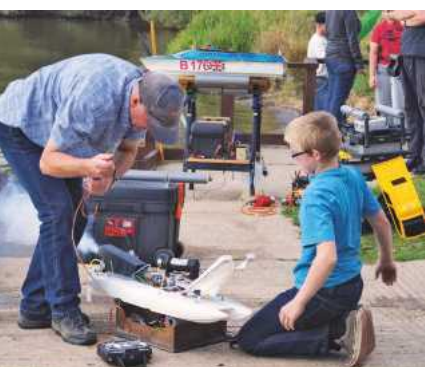
ABOVE: Harry Stuart firing up his OPS 45 powered catamaran. Note the leather cord used instead of an electric starter.
