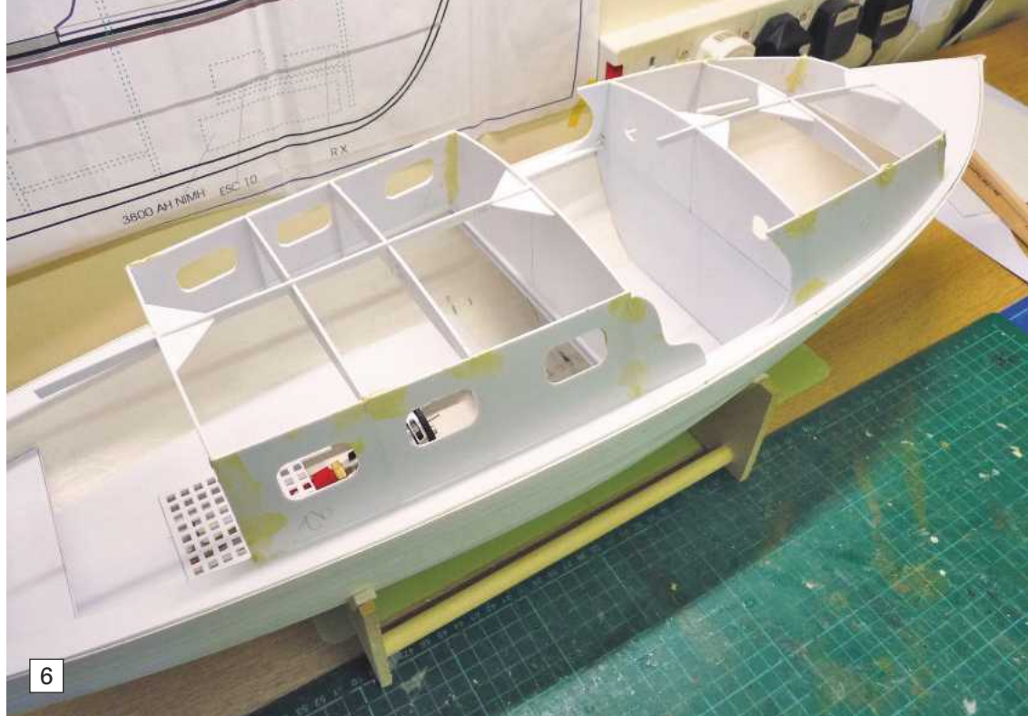
Photo 6. The cabins being constructed without their roofs. Tamiya masking tape is very useful for holding everything together before applying the liquid polystyrene glue.
