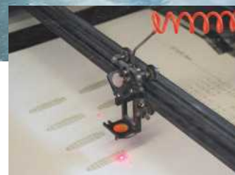
RIGHT: The laser cutter in action on the new St. Olaf hospital ship kit's lifeboats.
