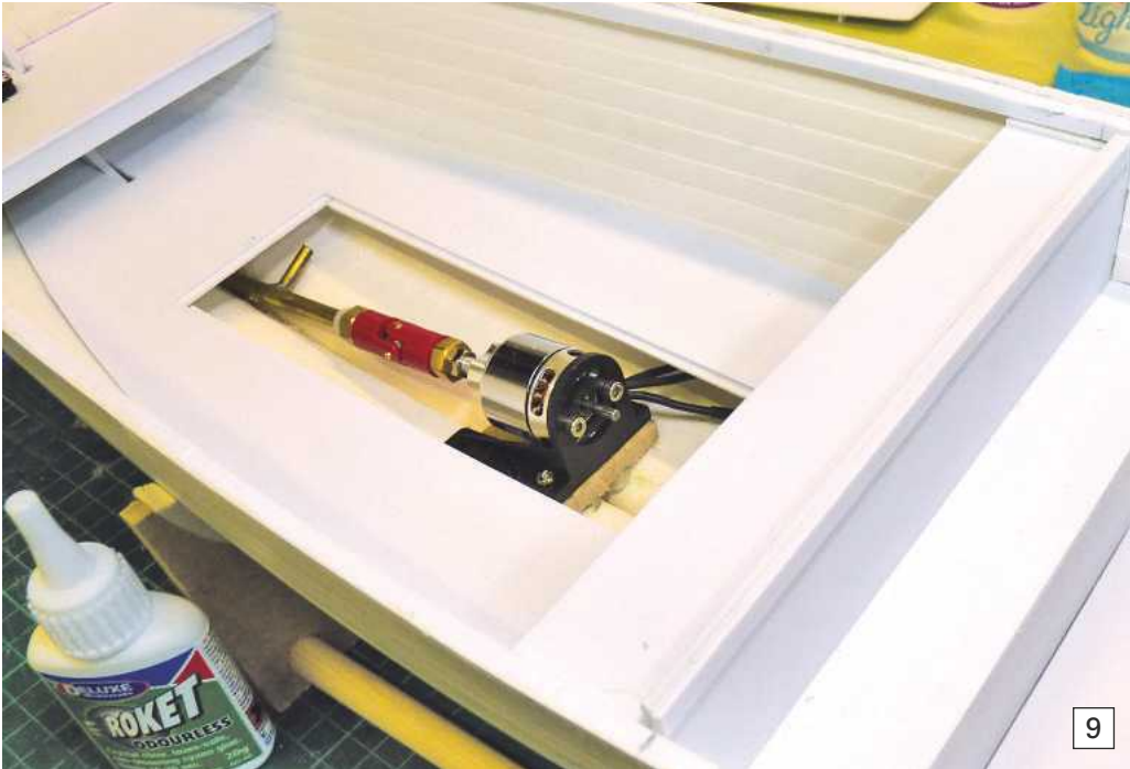
Photo 9. The simulated internal planking aft of the second bulkhead.
