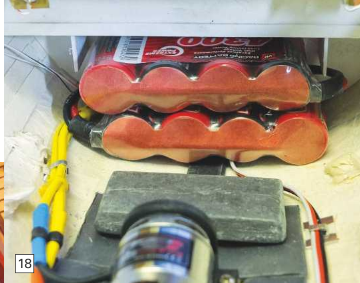
Photo 19. There is plenty of room for the receiver, esc and battery monitoring device.
