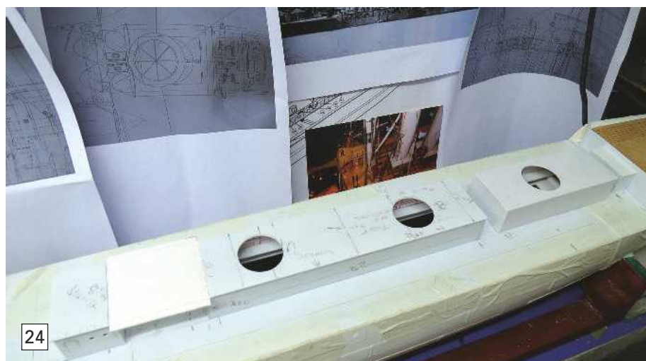
Photo 24. There is a bridging section between No's 2 and 3 housings and once complete, this slots into place.
