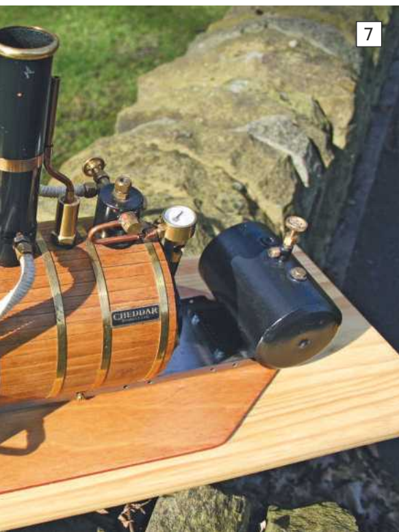
Photo 7. Just to give you an idea, these two Cheddar Puffin engines are going to have quite a demand for steam so are supplied by a pretty large boiler. Being a tug set-up though, we do need the fast response and manoeuvrability.
