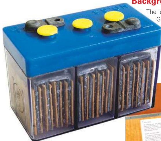
ABOVE: This model wet-cell battery shares the same basic internal construction as its full-size counterpart.
