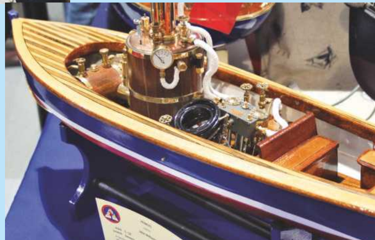
BELOW: Pebbles, an exquisite steam launch built by John Williams of the Manx MBC and fitted with a Marten, Howes & Baylis steam engine and Maccsteam boiler.
