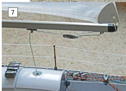
Photo 7: Adjustment was provided for the main sheet with an additional metal loop fitting, glued into the boom end, and a plastic bowsie. The jib boom has been similarly equipped.
