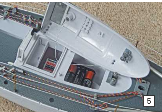
Photo 5: The deck is loosely re-fitted and the cabin top tilted to show the access holes in the main deck. The sheets have not been threaded.
