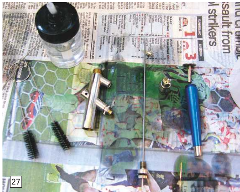
Photo 28. Liquid Reamer is formulated to remove even the more stubborn paint deposits from within an airbrush's body.
