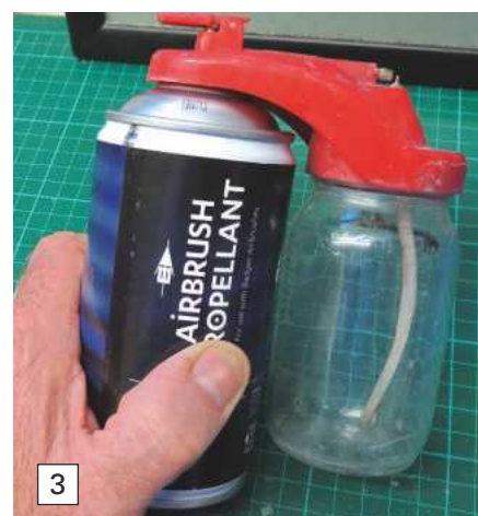
Photo 3. Another basic siphon type airbrush using a detachable can of pressurised air, is external mix but has a large paint capacity.
