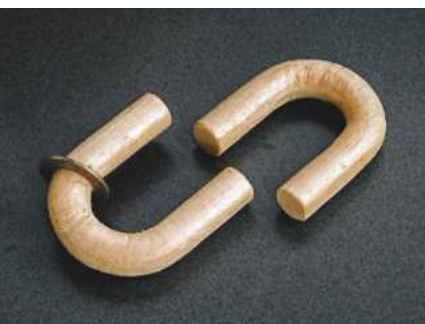
ABOVE: Carving the balsawood liferaft, second stage, rounding the separated sections with a sharp-holed washer.
