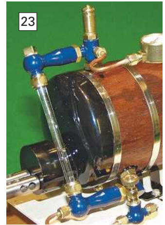
Photo 23: A common gauge glass on a Hemmens Ribbersdale boiler. Attaching the mountings to the circumference of the shell gives an excellent picture over a wide range of exactly what is in the boiler, but it does make the glass long and susceptible to breakage.
