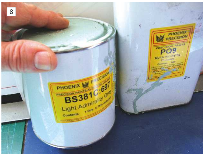
Photo 8. Phoenix Precision Paints are blended to a BS standard for the model maker and can be supplied with an appropriate grade of thinners.
