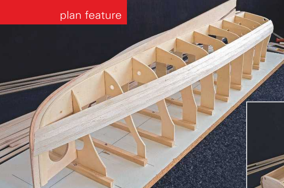
ABOVE: Bow planks meeting the keel at the bow doublers.
