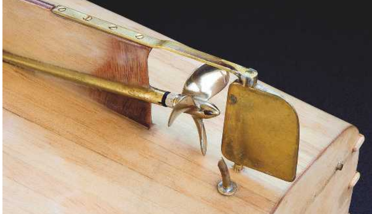
ABOVE: Propeller, skeg, rudder and cooling intake detail.
