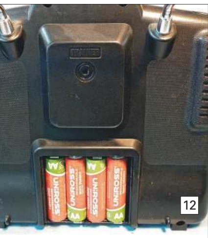
ABOVE: Back of Planet T5 transmitter showing rechargeable NiMH cells fitted and trainer socket.
