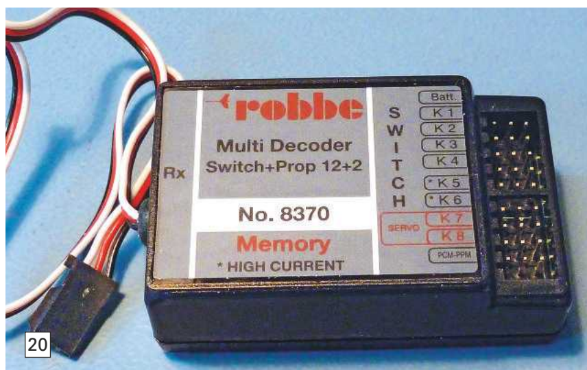
ABOVE: Robbe Multi Decoder Switch+Prop 12+2 module fits in model and connects to receiver.
