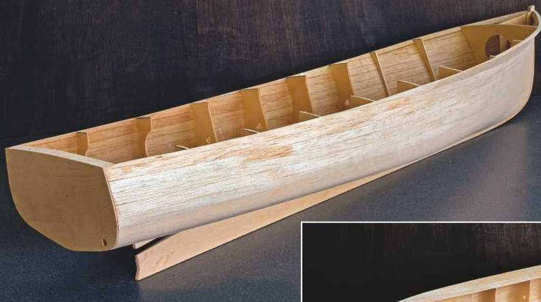
LEFT: Overall view of hull with its planking sanded and the plywood transom fitted.
