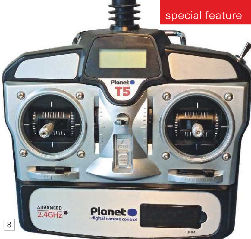
ABOVE: Planet T5 5-channel 2.4GHz transmitter.
