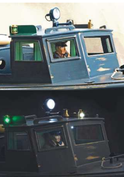
ABOVE: A total of six LED's were used for the lighting system; cabin light, forward light, searchlight, two running lights and mast light.
