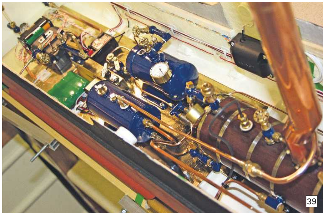
Photo 39. Neat straight pipe runs always look so much tidier than either twisted bent pieces of copper pipe (or silicone tubing), whether they are polished or insulated.
