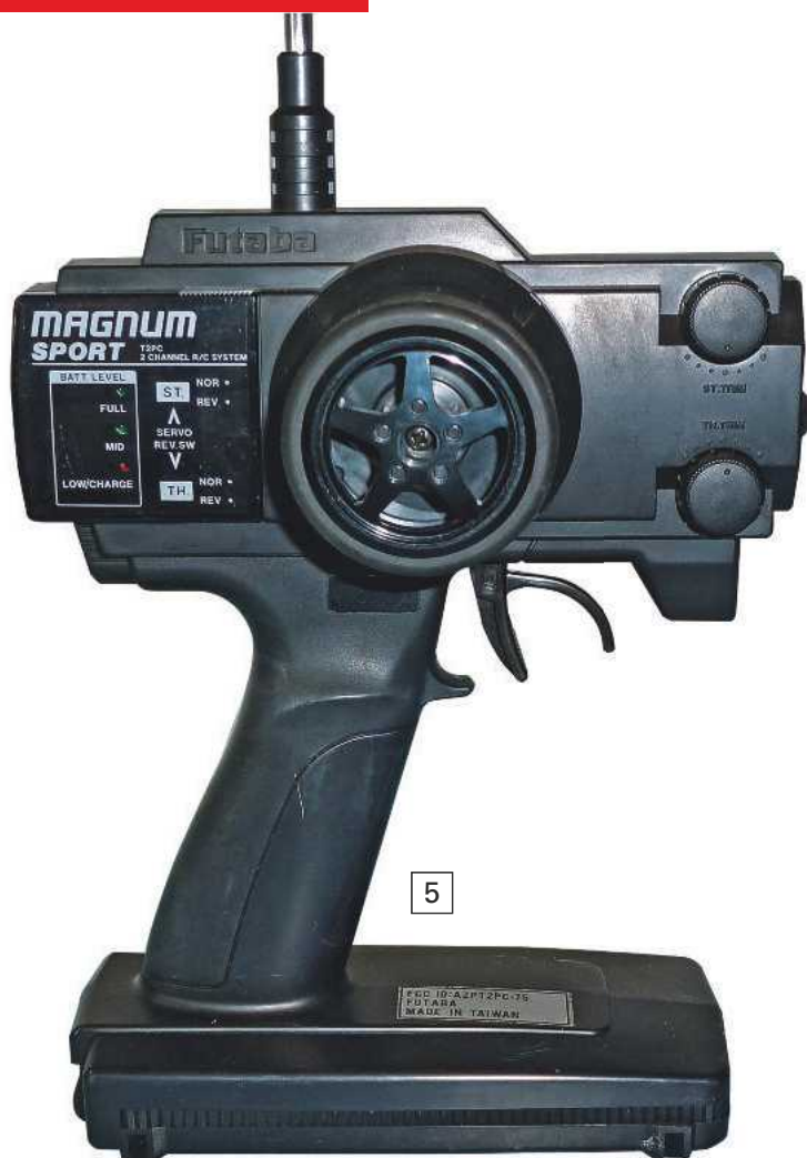
ABOVE: Futaba Magnum 2-channel 27MHz AM steerwheel style transmitter.
