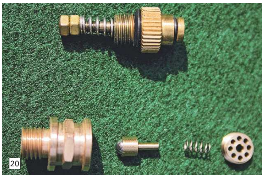
Photo 20. Two typical boiler safety valves. The Cheddar type at the top requires removal for adjustment, but the more modern unit at the bottom can be adjusted externally.
