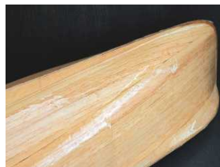
ABOVE: A closer view of the sheathing showing where a cut was required in the glass cloth.
