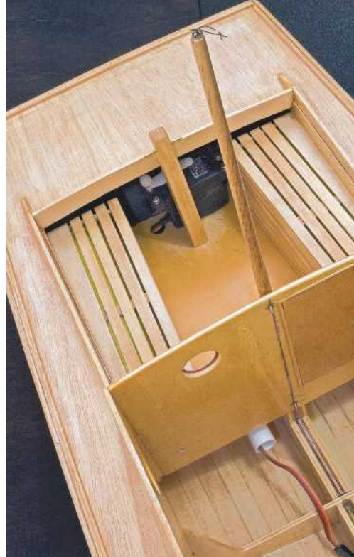
ABOVE: Stern area with rudder servo, also showing mast fitted later with internal wiring for light.
