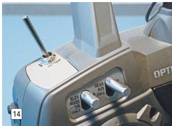
LEFT: Switches on left hand side of Optic 6 transmitter.
