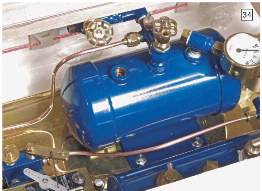
Photo 34. The onboard gas tank. On top is a pressure gauge and a manifold to allow the raising of pressure from an external tank on the bank as well as the normal outlet. The final connection is the filling Schrader valve.
