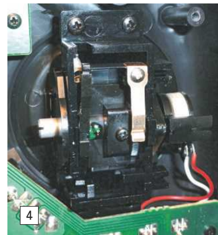
ABOVE: Centring spring disconnected and ratchet arm fitted instead.
