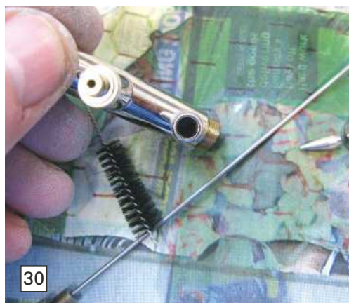
Photo 30. The final stage involves cleaning orifices with specialist brushes as some paint deposits may have dissolved but remain within the airbrush body.
