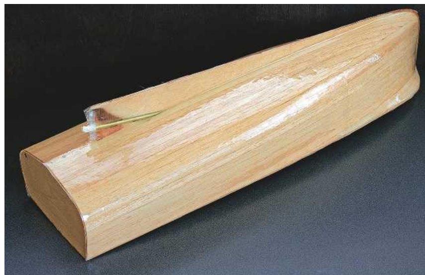
ABOVE: Epoxy fibreglass sheathing of the hull.
