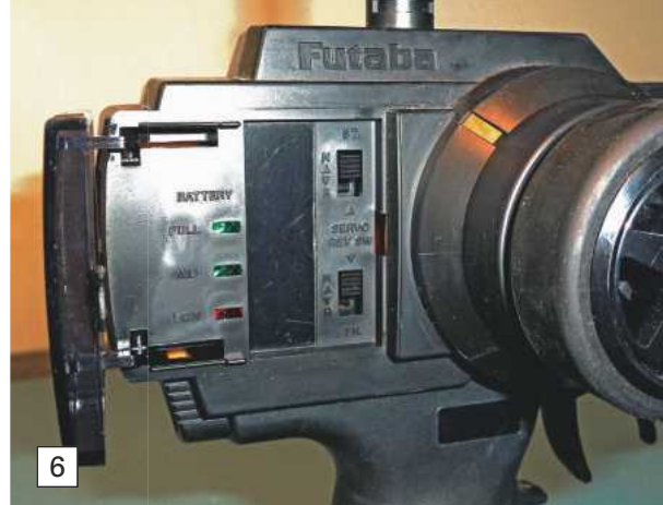
ABOVE: Servo reversing switches and battery indicator LED's.
