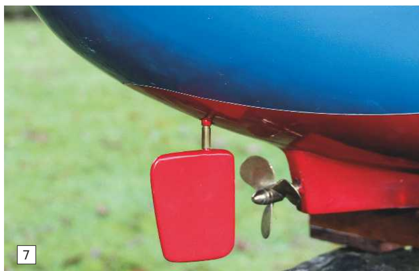
Photo 7. A comparatively slender hull of a launch will require a bit more speed and so a smaller propeller with a reduced pitch and probably only three blades operating at a faster speed will be more appropriate. This propeller is 60mm diameter.
