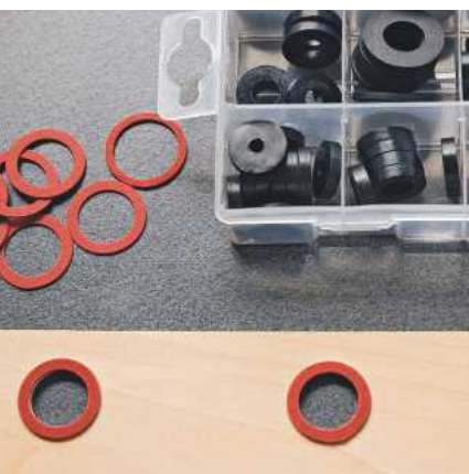
ABOVE: Sorting and fitting fibre plumbing washers for the porthole surrounds.
