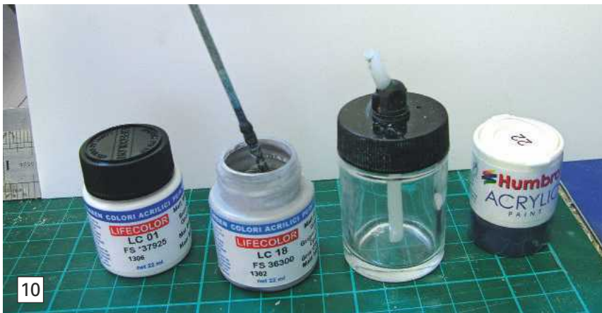
Photo 10. The mechanical pre-mixing and blending of paints is highly recommended before their use, whatever the means of delivery to the object being painted.
