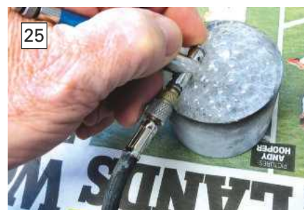
Photo 25. Immediately after use, the first stage of cleaning is to immerse the airbrush in a cleaning agent and allow both air and the cleanser to circulate.
