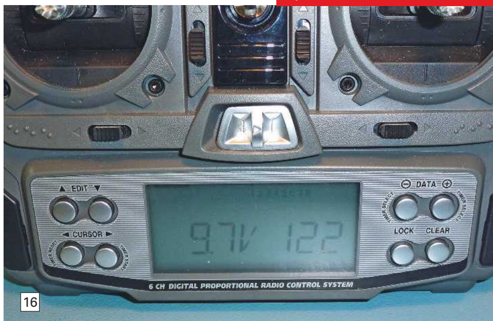
ABOVE: LCD display and programming buttons.
