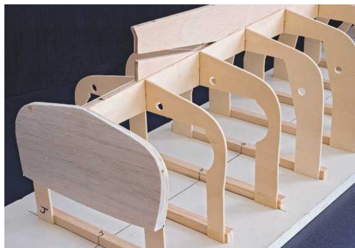
BELOW: On the building board, showing balsa transom filler piece.
