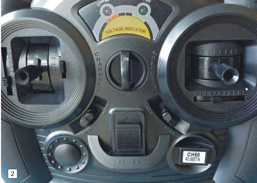
LEFT: Close-up of two channel Tx showing sticks, trim levers, servo reverse switches and throttle neutral adjustment lever. Battery indication via two LED's.
