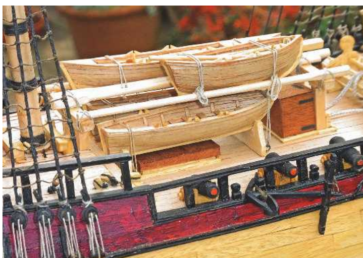
ABOVE: One of the ship's four boats coming out of its plug. The wooden plug was first coated with cling film, then brown parcel paper, followed by the external planks, keel etc.
