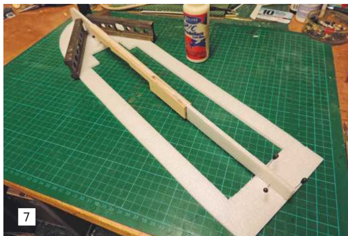
BELOW: Using pins and some 90 degree weights, glue the assembled keel on the centre line of the chine deck and leave to dry.
