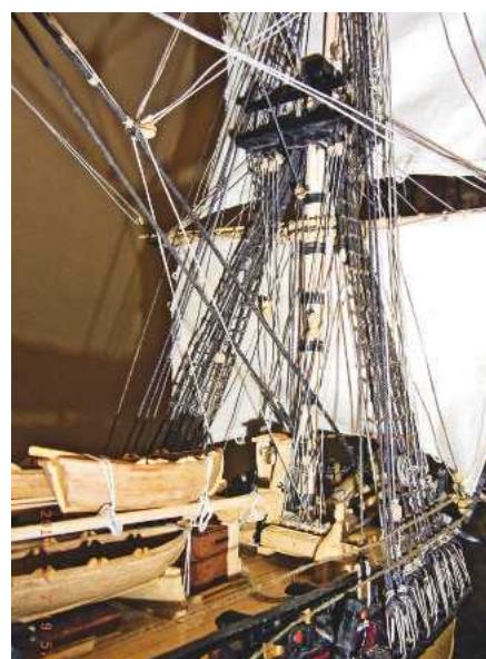
ABOVE: The rigging to the foremast. All the blocks, deadeyes and ropes are to the correct scale sizes and colours. The rigging lines are belayed in their correct manner, but the ones used for actually sailing the model are made to run through to enable the sails to be set for each tack.
