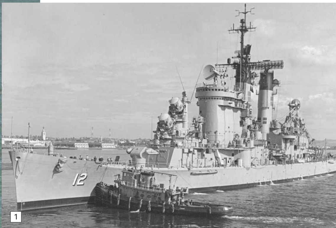
Photo 1. USS Columbus as rebuilt into a guided missile cruiser. Note the very high superstructure and bridge and the two combined funnels and masts (MACK's).
