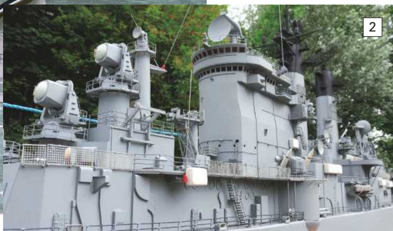
Photo 1. USS Columbus as rebuilt into a guided missile cruiser. Note the very high superstructure and bridge and the two combined funnels and masts (MACK's).
