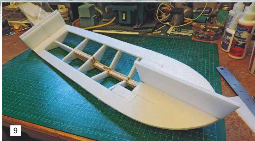
9 ABOVE: Glue the transom assembly and the front deck support on the centre line. Ensure they are at 90 degrees, although the side formers, if they are cut accurately, will ensure the correct angles.
