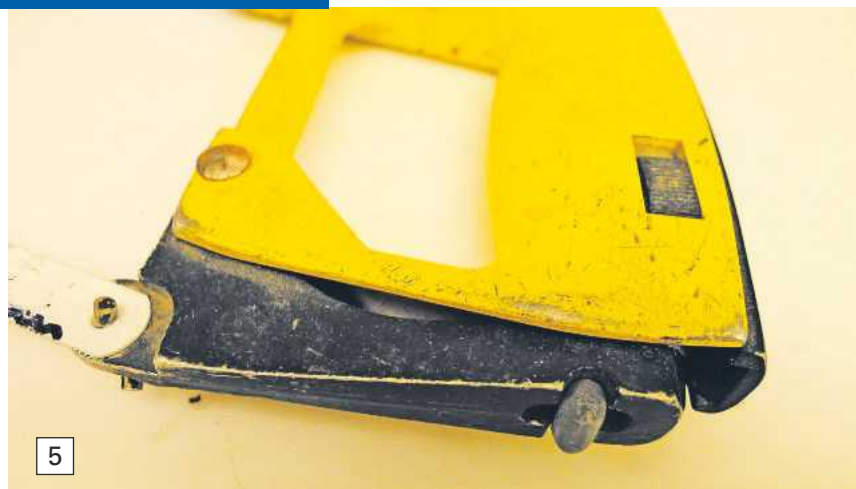
ABOVE: Hacksaws have many varied types of arrangement for tensioning the blade, but they all have the same considerations. If the set-up is worn and the blade is allowed to become out of alignment, the saw should not be used.
