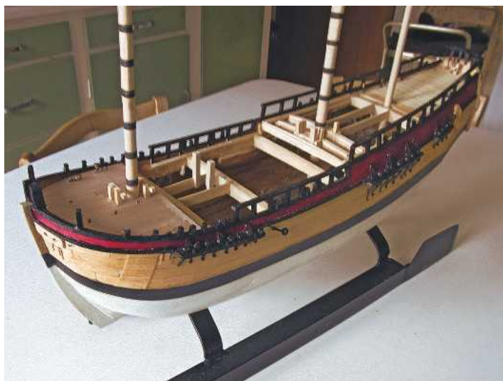
ABOVE: The external planking is complete, stem, sternpost and keel fitted and the decks are half-complete. The decks are in two layers, the first being plywood sheet across all the deck, followed by planks to scale. Attachments for blocks are fitted at this stage.
