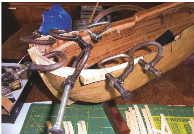
ABOVE: The veneers have been coated with brown parcel paper, deck supports fitted to make the hull rigid and the first external planks of 0.9 mm Obechi are being laid, clamped in place until the PVA glue has set.
