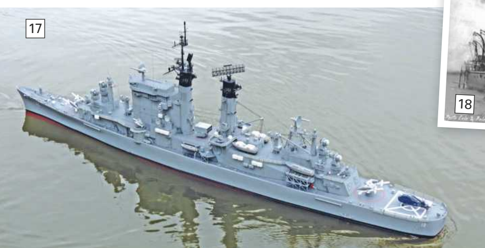
Photos 16 and 17. USS Columbus underway with no stability problems because of the hidden keel weight.
