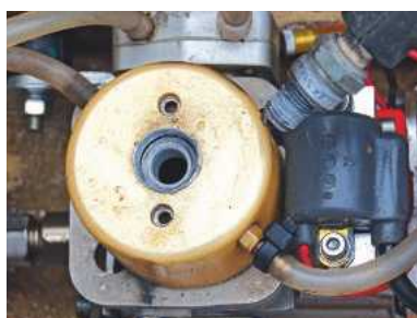
ABOVE: The somewhat overheated engine of Mike Barnes' winning D4 Patriot. Note the threads of the spark plug (top right) containing the cylinder head alloy that melted causing the plug to blow out!
