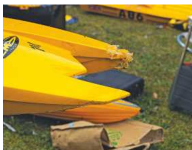
BELOW: The damaged front sponson of Malcolm Pratt's Catamaran.
