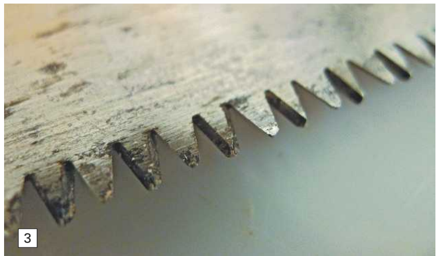
ABOVE: A close up of the wood saw teeth shows clearly the cutting face on the forward edge of the tooth. This is exactly the same arrangement with metal cutting saws, but in a smaller size.
