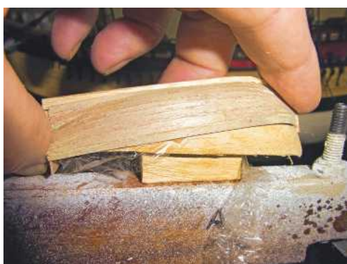
ABOVE: One of the ship's four boats coming out of its plug. The wooden plug was first coated with cling film, then brown parcel paper, followed by the external planks, keel etc.
