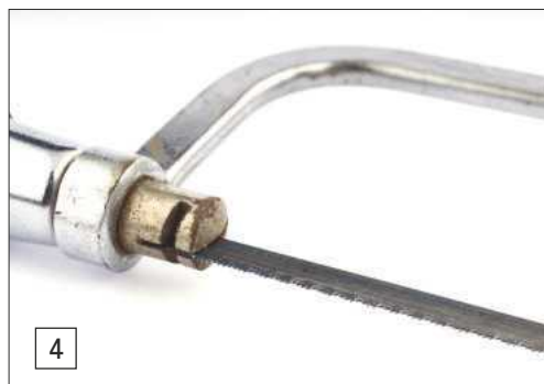
LEFT: The much finer teeth of a typical metal cutting hacksaw blade. Despite being a disposable blade, it is still designed to cut on the forward stroke and the teeth are offset just like a wood cutting saw.
