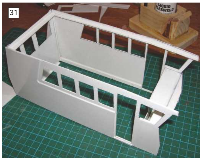
PHOTO 31. This is the starboard side cabin outer skin in place. You can also see the strip inside the cabin sides' top edges to support the roof.
