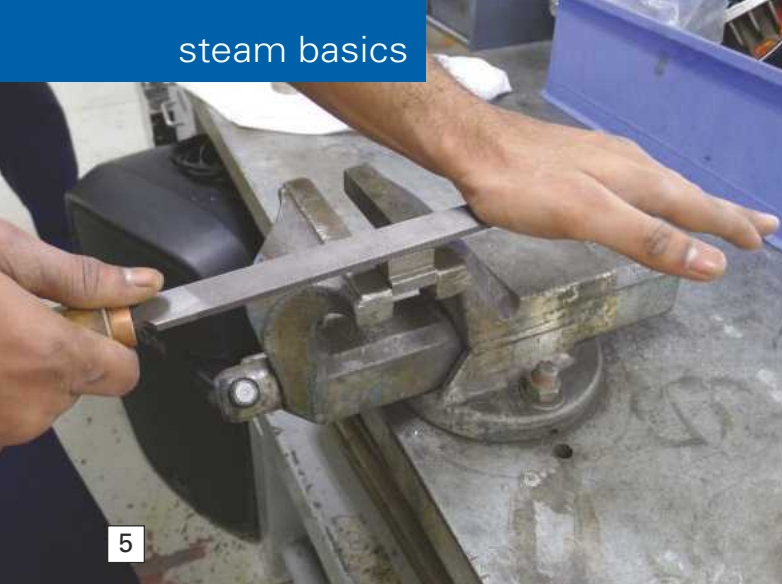
PHOTO 5. Heavy cross-filing with good pressure provided by the heel of the hand on the forward strokes.
