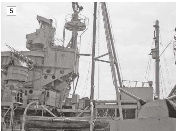
PHOTO 5. As part of the refit at the Boston Navy Yard, an extension was made aft of the bridge to accommodate the raised platform for the Type 277 radar.
