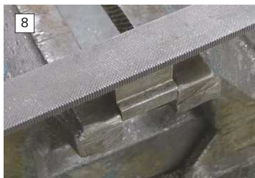
PHOTO 5. Heavy cross-filing with good pressure provided by the heel of the hand on the forward strokes.
