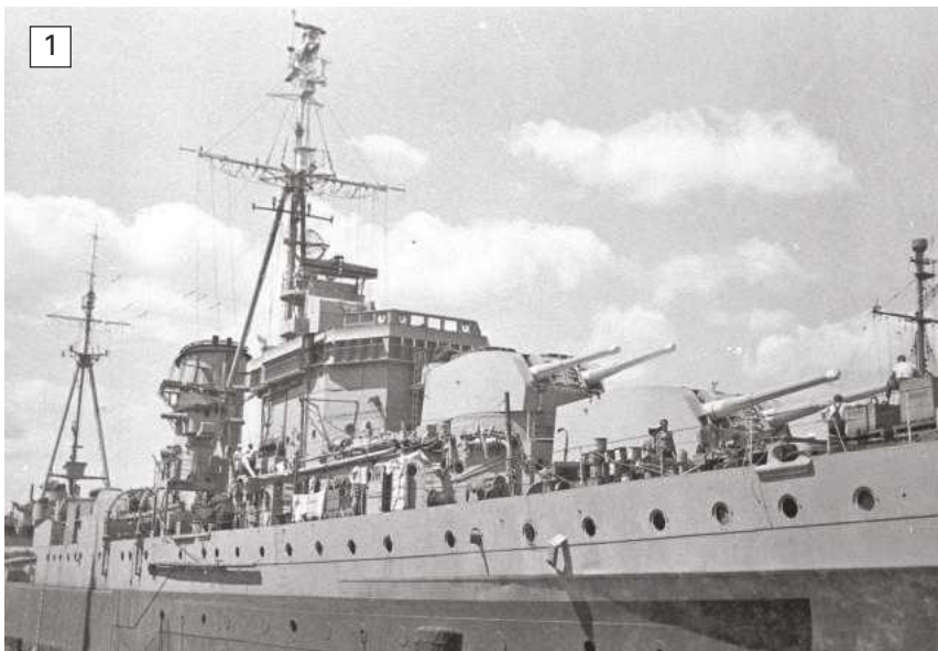
PHOTO 1. An excellent starboard side view of the hull where extensive use was made of welding.
