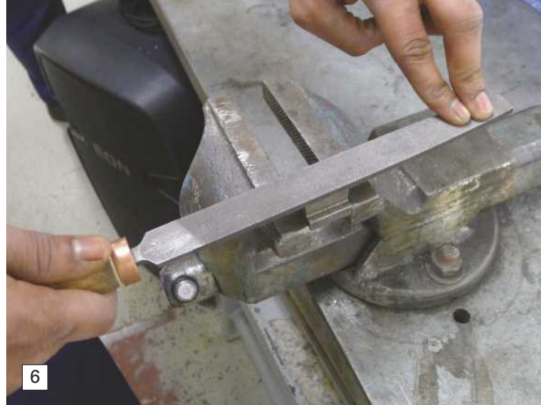
PHOTO 6. Lighter cross-filing should be done with a couple of fingers to reduce the pressure while maintaining good control and releasing the pressure on the back stroke.
