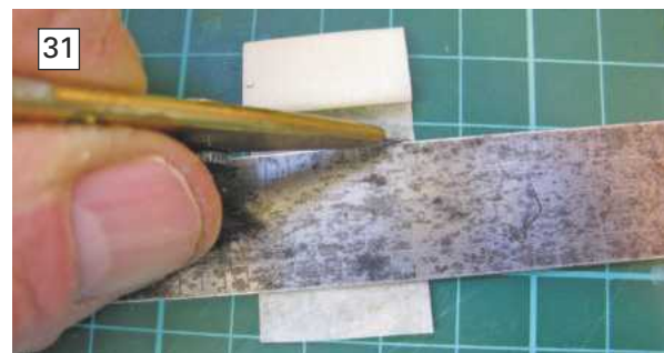
PHOTO 31. Ordinary masking tape was used to form the shape of the self-righting bag.
