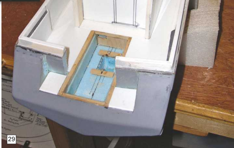
PHOTO 29. The cabin must be a decent 'tightish' fit over the coaming.
