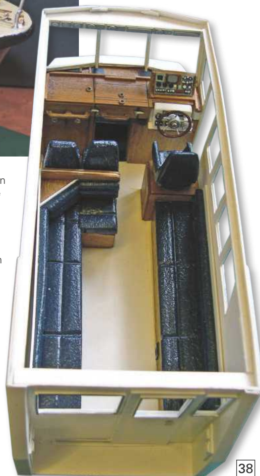
PHOTO 36. The rear part of the cabin interior is all built on a removable floor.
