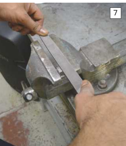
PHOTO 7. Draw-filing is tricky as there is very little length of file to control, but it should be only for finishing cuts anyway and not to remove large amounts of metal.
