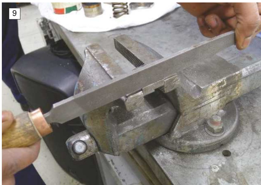
PHOTO 9. Delicate filing is always best done with fingers rather than the heel of the hand, particularly when finishing off a corner.
