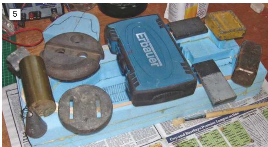
PHOTO 5. Gluing together the hull blocks. The centre lines together with locating cocktail sticks are essential to ensure everything is in alignment.
