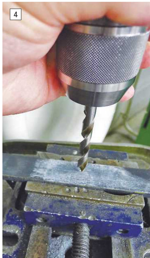
PHOTO 4. To get the drill bit in the perfect position rotate the chuck by hand while applying very gentle pressure. You should see an evenly marked centre punch mark when you lift the drill bit again. When you have the position perfect, lock the vice and lock the table before a final check.
