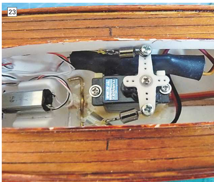
PHOTO 21. The rudder shaft has to be bent to form the tiller. The fishing line linkages from the rudder servo attach to the end of the tiller.
