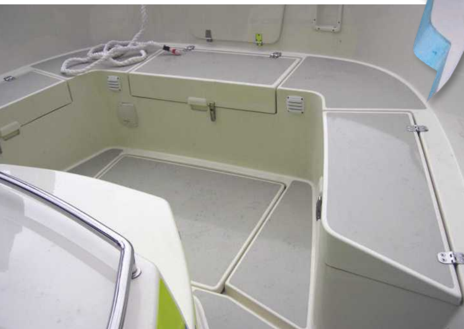
ABOVE. A photo of the bow area of the full sized boat showing the seats/storage lockers.
