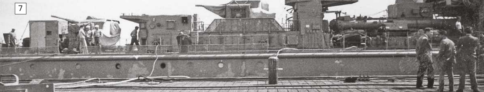
PHOTO 7. This general picture helps in assessing the position of the various fittings, gun mountings fits and the aft torpedo tube arrangement.
