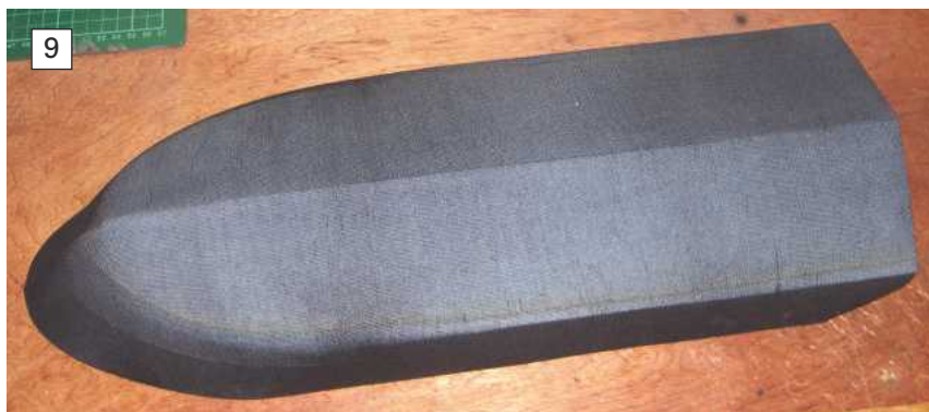
PHOTO 9. Push the shaped hull block into a leg of a pair of tights or a single stocking. 30 denier (thicker than usual) was used on this prototype Targa model.
