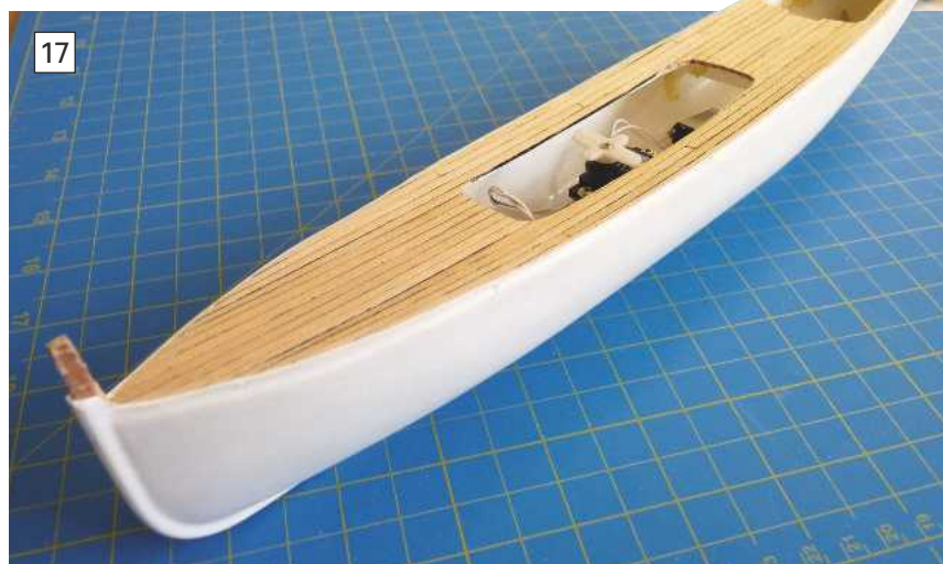
PHOTO 12. Caulking the edges of the planks. The optional supplied caulking is wonderful stuff!
