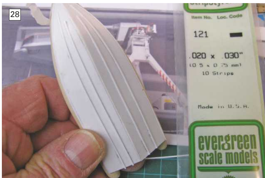
PHOTO 26. The spray rail positions were marked and styrene strips glued in place to represent them.
