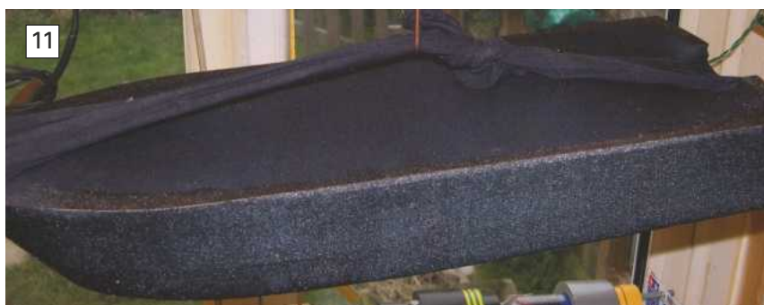
PHOTO 11. It is a good idea to hang the hull, whilst the resin is curing, This is best done by making a bespoke 'hanging device' before commencing the resin application.
