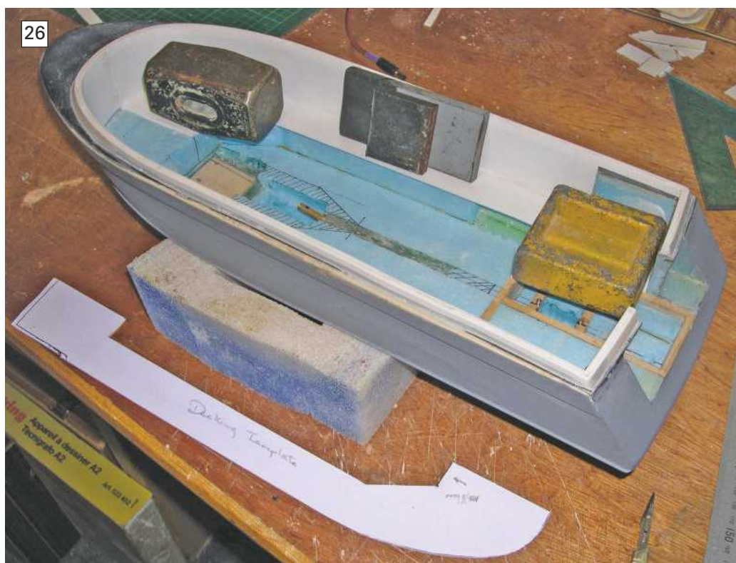
PHOTO 26. Using the centre foam block cutout to help achieve the right shape, cut and trim 0.5mm styrene sheet to size, glue and weight down.
