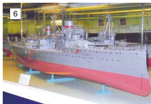
PHOTO 6. The builder's model of HMS Colossus at 1:48 scale. Note the fore funnel is in front of the fighting top, thus filling it with smoke when the ship was at full power.
