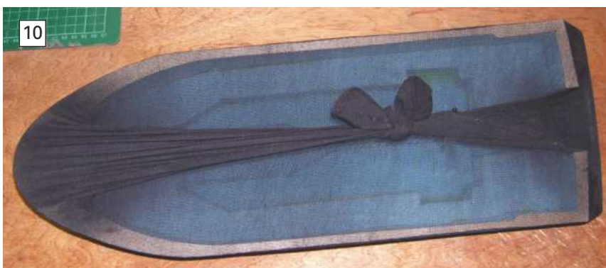
PHOTO 10. Tie together over where deck will be, smooth out all wrinkles and make sure no ladders or seams are over the hull's outer surfaces. Two coats of twin pack epoxy finishing resin were then applied. Leave each coat to dry and don't 'squeeze' it all too much as nylon tights/stockings will move about when wet.
