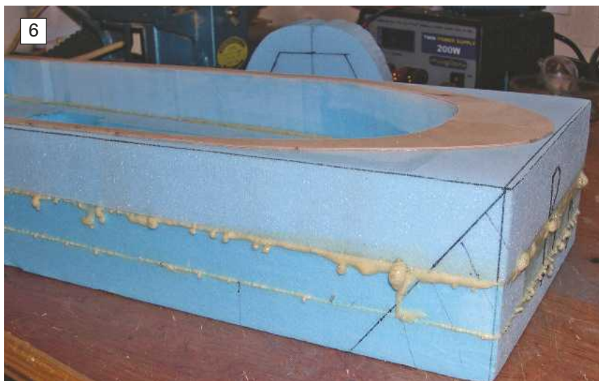
PHOTO 6. Mark out the bow angle of 60 degrees from the bottom and cut the waste away.
