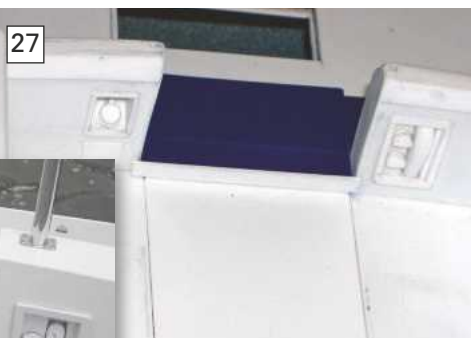
LEFT. Detail from the real boat showing power socket, shower controls, and the transom gate.
