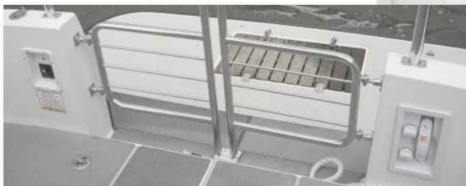
PHOTO 27. This is the sort of detail one can include in this sort of model, namely a power socket and a caravan style shower unit in the stern panels either side of the transom gate.
