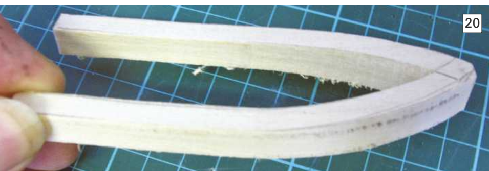
PHOTO 20. Now that the basic collar is prepared, sanding the rounded shape can begin. This part of the job actually took no more than 20 minutes or so of dusty work!
