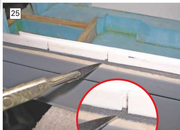
PHOTO 25. The coaming top edge which supports the handrails is now created by laminating the styrene, with the middle parts being spaced with gaps, which in due course will accept the handrail supports. Mark from the plans and glue first one piece to the extended walkway sides, followed by the other 'spacers'. Finish by a further complete strip around the outside. Lightly fill in where the coaming meets the deck to get a nice slope at the bows and sand as need be.
