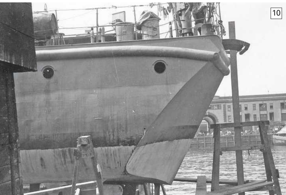
PHOTO 9. The stern part of the vessel. It's worth noting the two small cranes mounted on the transom for deploying the minesweeping equipment.
