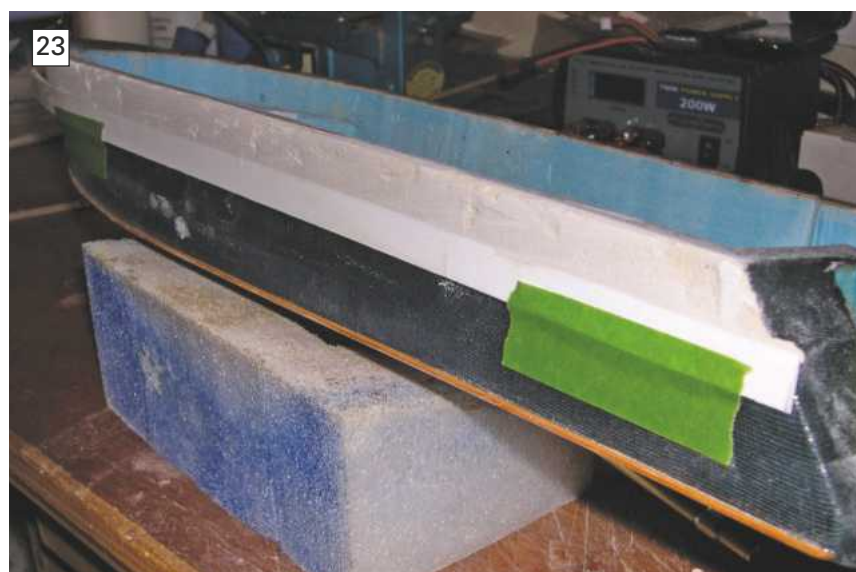
PHOTO 23. At the top of the hull sides is a flange. This could be made from 1.5mm styrene or plywood just stuck to the hull's sides, but here the bottom edge was created by using a narrow flexible strip to give the flange's depth and then lightweight car body filler was applied and later sanded to shape.
