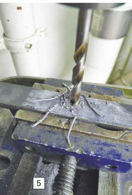
PHOTO 5. Just the right amount of pressure should generate the same swarf from both cutting faces without generating too much heat at the bit. Steady and consistent pressure will help to ensure a neatly drilled hole.
