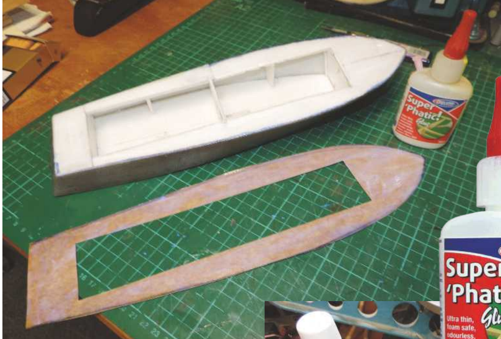
LEFT: Super Phatic for gluing veneer to Depron.
