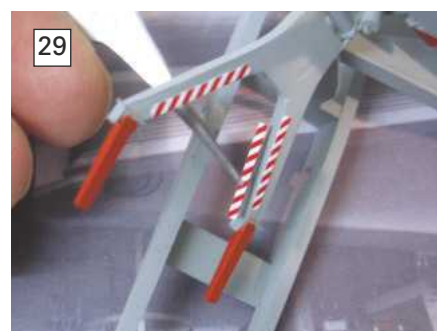
PHOTO 28. Each chevron was cut to size and fixed to the hoist arms.
