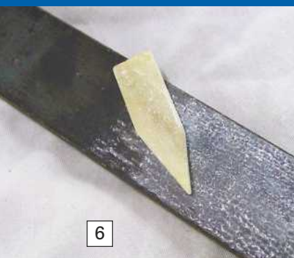
PHOTO 6. Engineer's chalk is quick and easy for marking-out purposes and is readily available. It is actually quite handy for writing on bits of metal as well.
