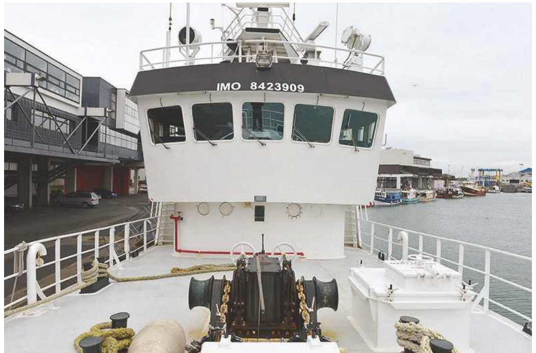
ABOVE: Forward end of the wheelhouse looking to port, with twin helmsman seats and the central console and instrumentation displays. ABOVE RIGHT: Central console in the wheelhouse and no traditional steering wheel can be seen anywhere! BELOW: Bridge front: This view shows the windlass and the large hatch to port incorporating a smaller escape hatch with central unlocking hand wheel.
