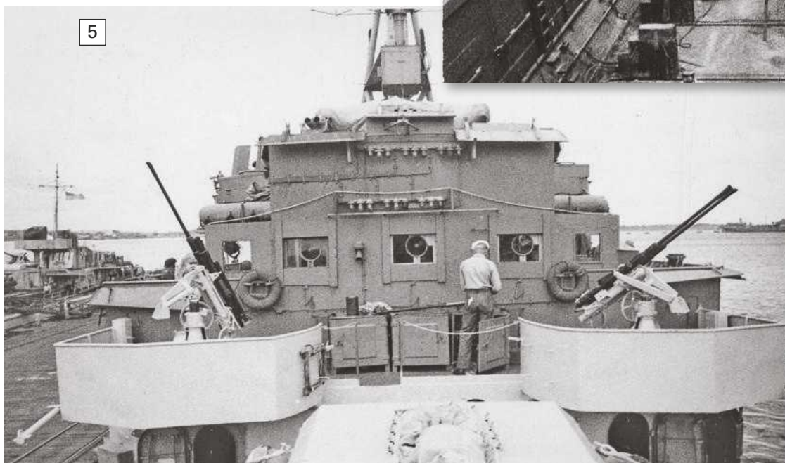
PHOTO 2. Unlike the earlier torpedo boats (T1 to T21), T35 does not have a knuckle forward towards the bow and was fitted with two exhaust uptakes.
