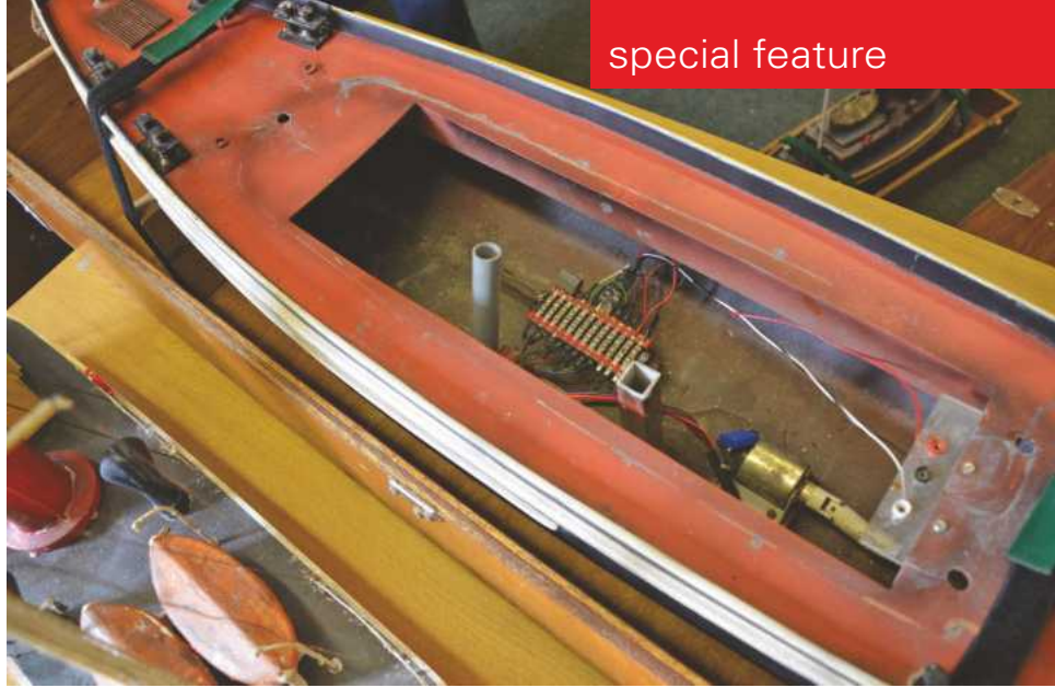
ABOVE: The inside of Hercules . The grey pipe allows another pipe to be inserted through it to feed 'smoke' up through the stack (funnel) for filming.
