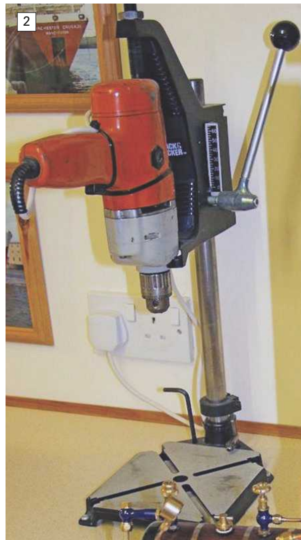
PHOTO 2. Although limited in many ways, a simple drill stand such as this accessory for a hand-held pistol drill is a huge improvement over not having anything! The job is clamped, the drill is clamped and vertical movement controlled. The whole operation is safer and infinitely more accurate.
