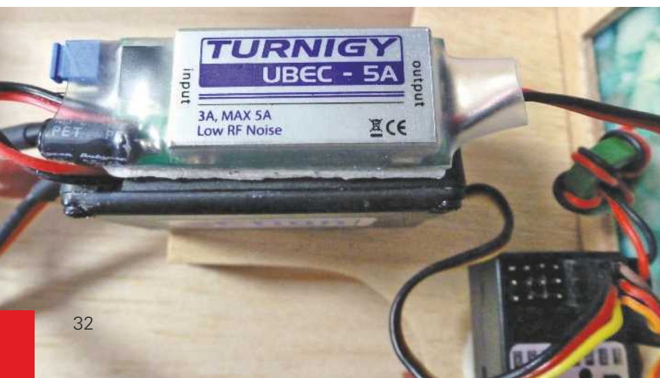
BELOW: A Turnigy UBEC device fitted to the speed controller in the author's Vic Smeed designed Moonsong.
