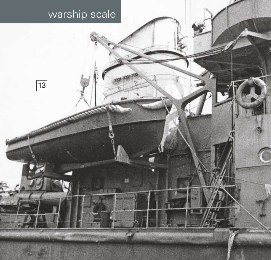
PHOTO 13. Another view of the starboard side boat stowage. T35 carried three boats in all, including a dinghy.
