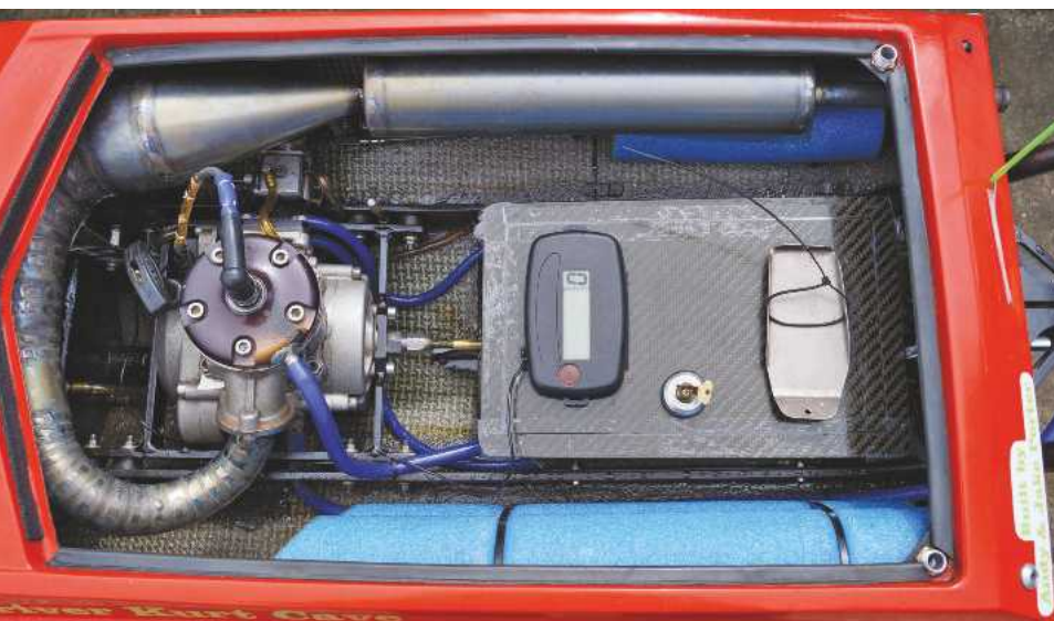
BELOW: Inside of Kurt Cave's huge Apache Chief and please note the titanium tuned exhaust system.
