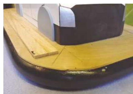
TOP: Platform and body being glued to the Armaflex skirt.
