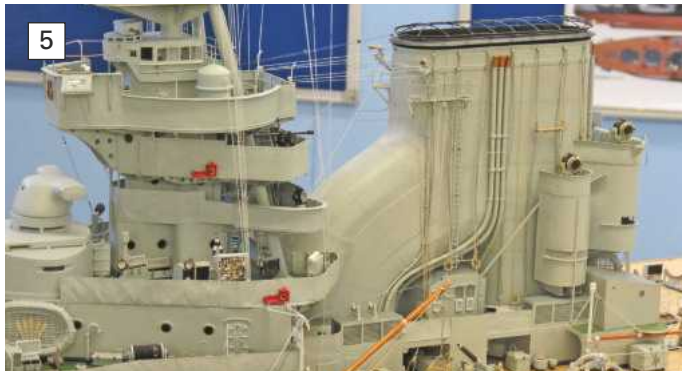
PHOTO 5. In the 1926 refit the foremast was re-built and the original two funnels trunked into one. David Brown's model demonstrates this reconstruction really well.
