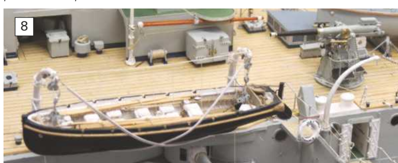
PHOTO 8. This picture shows a wealth of detail and includes one of the two 3-inch anti-aircraft guns and the Robinson Davit Disengaging Gear on the 32ft cutter, and still all to 1:96 scale in case you had forgotten!
