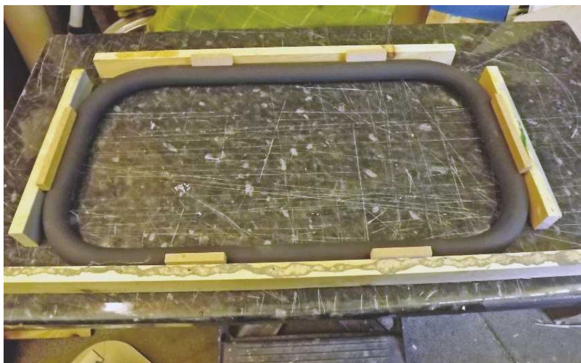
RIGHT: The Armaflex skirt in the jig, ready to be fixed to the main platform.
