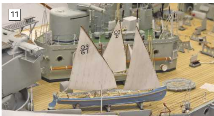
PHOTO 11. A superbly made 30ft gig, (barely 4 inches long) demonstrating the dipping lugger style of rig.
