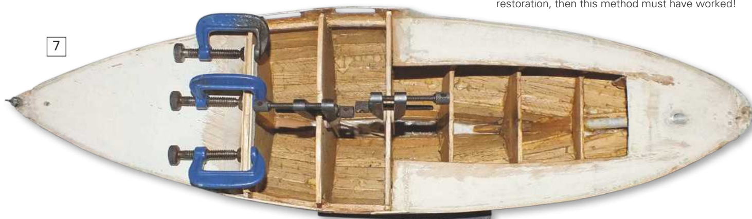
PHOTO 7. The hull was flooded internally with thinned glue to penetrate the wood. Strengtheners were also added to the frames.
