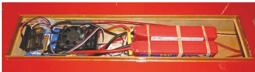
ABOVE: The ex-USS Independence electrics are a snug fit underneath the hatch - note the esc cooling fan.
