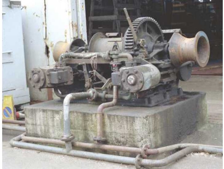
ABOVE LEFT: An electric trawl winch, basically same layout as the steam winch on Ben Idris , with brakes, end warping drums and warp guiding-on gear to the barrels and note the vertical slotted pillar(s) on the deck to take the wooden pound boards. ABOVE RIGHT: This is a steam winch used to haul the carriage on Herd & MacKenzie's slipway at Buckie. Whilst of different layout to the trawl winch on the trawler it shows the arrangement of steam cylinders and connecting rods etc.
