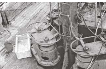
ABOVE: Centre rollers, sometimes known as centre bollards. Here we can see warp from the aft starboard gallows passing around a single roller, next around the centre roller and then leading aft to trawl winch. The port centre roller handles the warp from the forward gallows.
