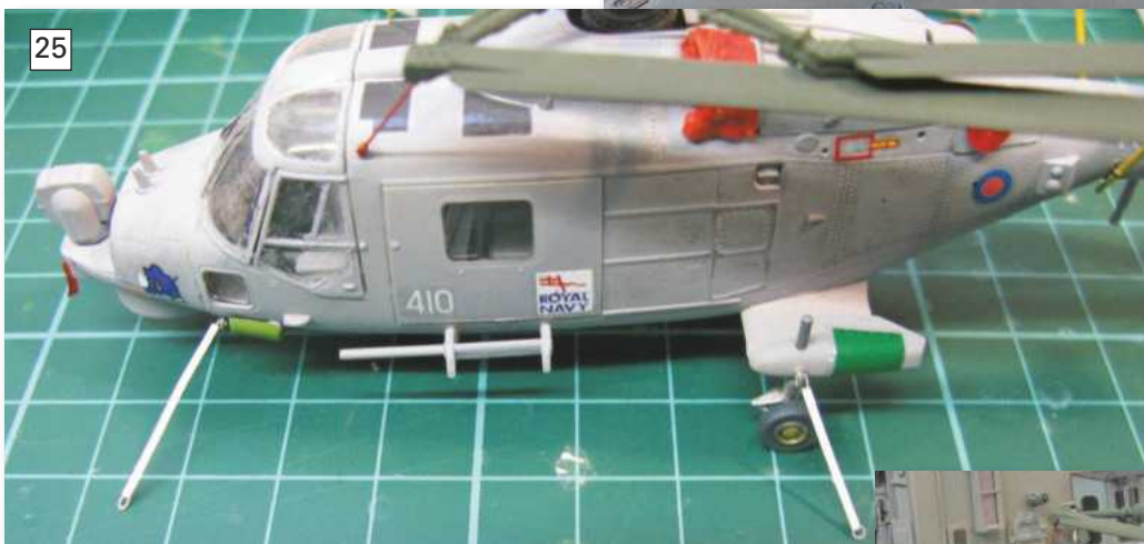
PHOTO 25. Litho plate is a good material for making the tie-down straps.
