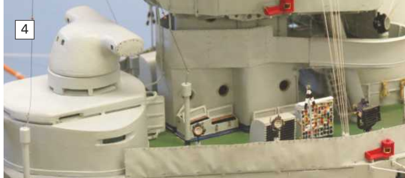
PHOTO 4. Just aft of the main director at the base of the foremast is the signalling position.
