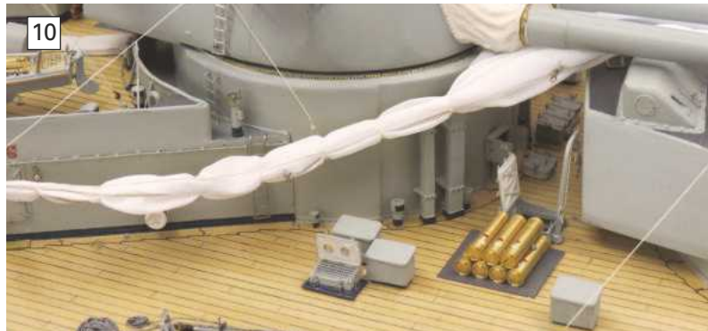
PHOTO 10. Immediately beneath the barrels of X Turret are brass cordite cases ready to be hoisted below and please note the small davit for just that purpose.
