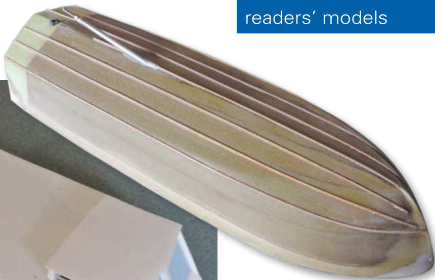
ABOVE: Here the hull has been coated, rubbed down to a smooth finish and the spray rails added, before coating again with epoxy finishing resin.
