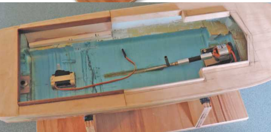
Where's the motor? Remember this hull is only 20 inches long and the 2830 brushless motor is far smaller, but also much more powerful, than a 380 brushed motor which used to be the standard.
