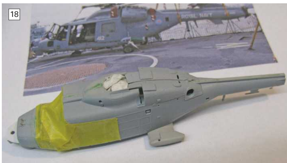
PHOTO 18. Masking over the completed interior ready for airbrushing the fuselage exterior.
