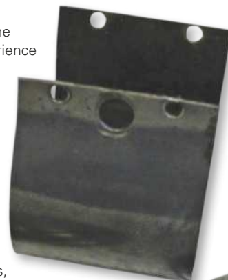
ABOVE: This base from the Stuart 10V has been hand painted with a two part epoxy paint. It is probably the hardest finish to apply to an engine and the colours are limited and application is very tricky. Note all the mating and running surfaces have been masked-off to keep them free of the paint.
