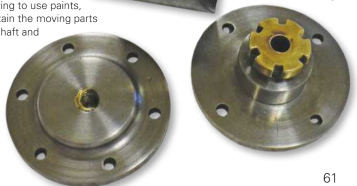
Although all of ferrous metal, these items have only been cleaned, avoiding a high polish that may spoil the authenticity of the engine. The cylinder cover is 'blued', which is another form of protective coating beyond the usual capabilities of the home hobbyist but is very similar to acid based blackening.
