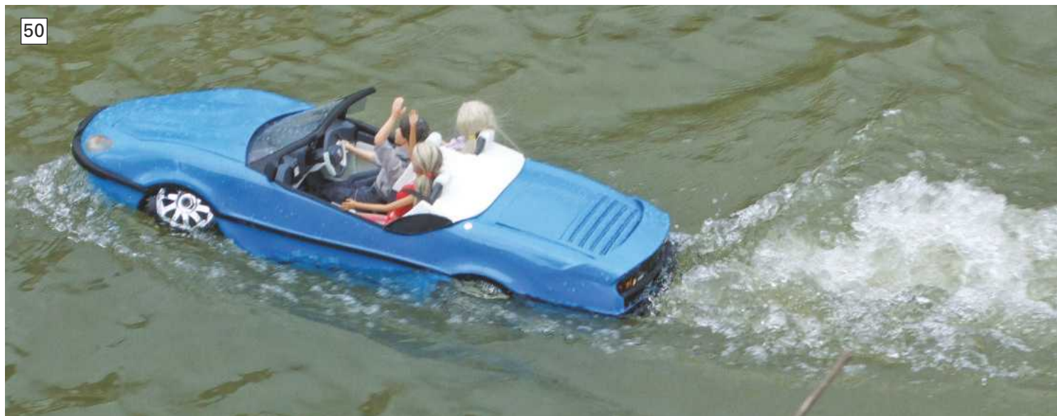
PHOTO 51. A high speed run, showing the planing angle it runs at and the extensive wash.
