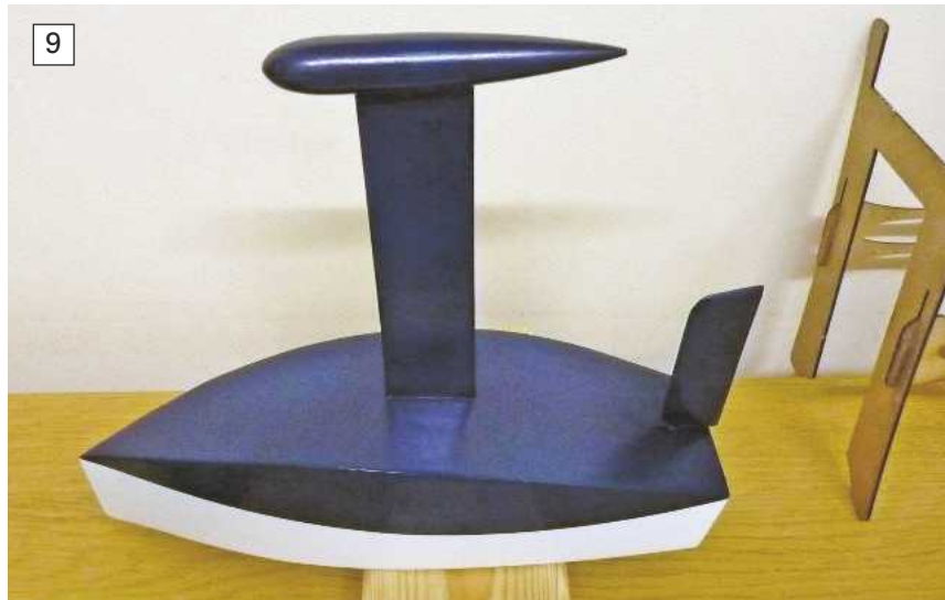
PHOTO 9. The ballast weight is supplied readymade, but it has to be 'fettled' and glued to the wooden keel piece.
