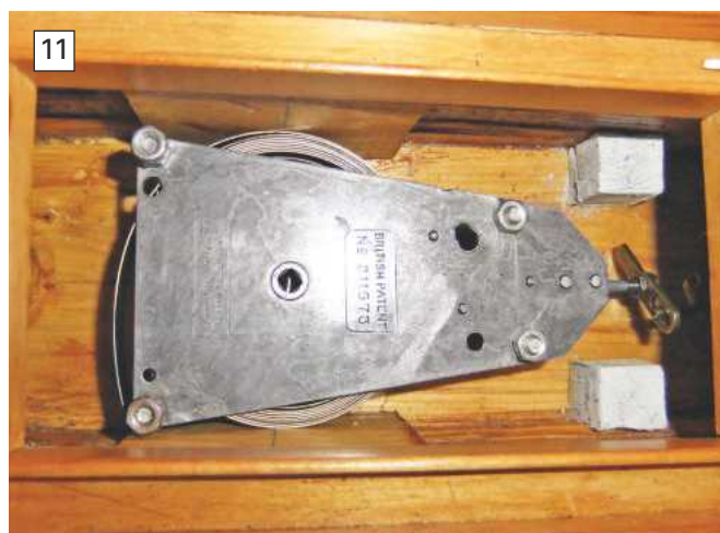
PHOTO 11. Note the spring centering blocks, which keep the model balanced as the spring unwinds.
