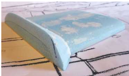
The stubby wings are foam over a plywood base for strength.
