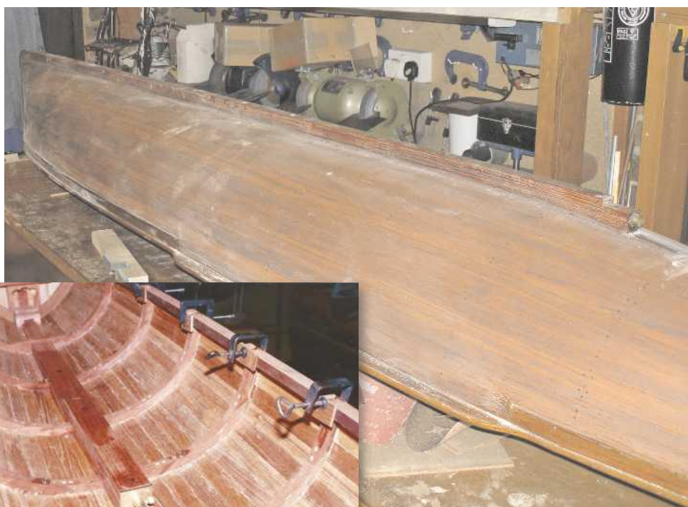
INSET: Detail of the planking as seen from inside of hull.
