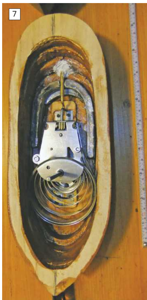
PHOTO 4. The Bassett-Lowke motor now with a standard spring.
