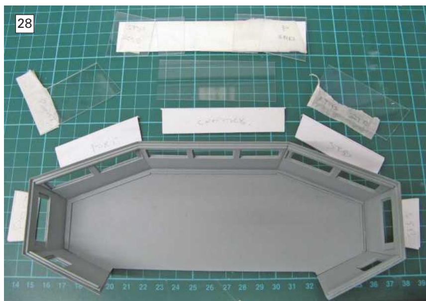
PHOTO 26. Fixing the partitioned bulwark amidships.
