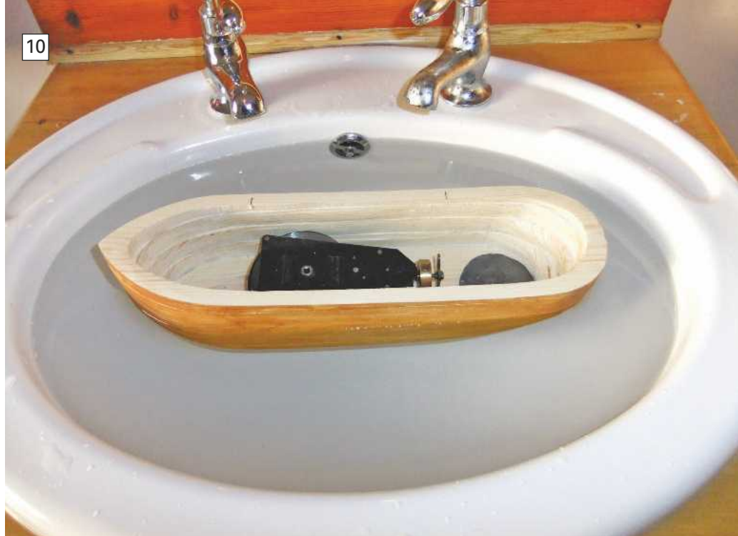
PHOTO 10. This semi-scale steam propelled puffer type of vessel, is built in a conventional bread and butter construction method. Here, it is being tested in the bathroom sink, to get the motor position correct!
