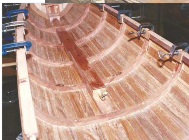
INSET: Detail of the planking as seen from inside of hull.
