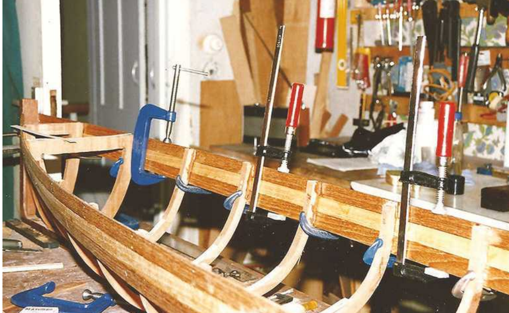
LEFT: Teak is a very difficult wood to work with as it blunts tools quickly. Here are lots of clamps to hold the planks to the hull framework. The glue was a special Ciba Geigy adhesive.
