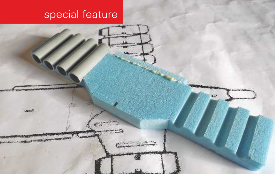
ABOVE: The eight jet engines are replicated by 19mm styrene tube. BELOW: The completed engine unit.
