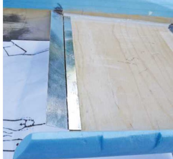
Aluminium flaps that could be bent, were tried to get the model to 'fly' correctly.
