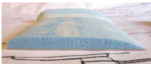
The stubby wings are foam over a plywood base for strength.
