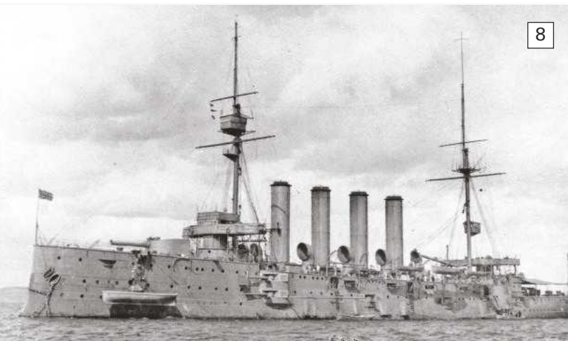
PHOTO 8. HMS Hogue was one of six armoured cruisers that formed the Cressy class. They were fitted with two 9.2 inch main armament guns and 6 inch guns mounted in casemates. 12pdr guns are visible along the upper sides of the hull.
