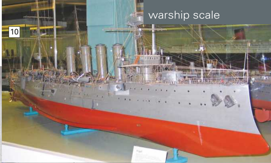
PHOTO 10. The First Class armoured cruiser HMS Argyll was built by Scott's of Greenock and differed from the preceding Cressy class in having four 7.5 inch guns for her main armament.
