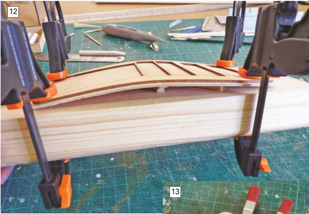
PHOTO 12. Rear hatch cover, clamped to achieve the same profile as the deck.
