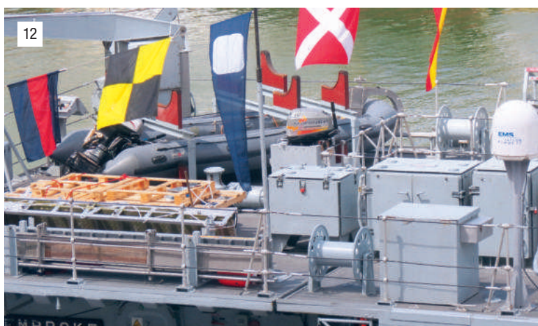
Photo 12. A busy after section of 01 deck with the tiered stowage arrangement for the two Avon mine clearance workboats.
