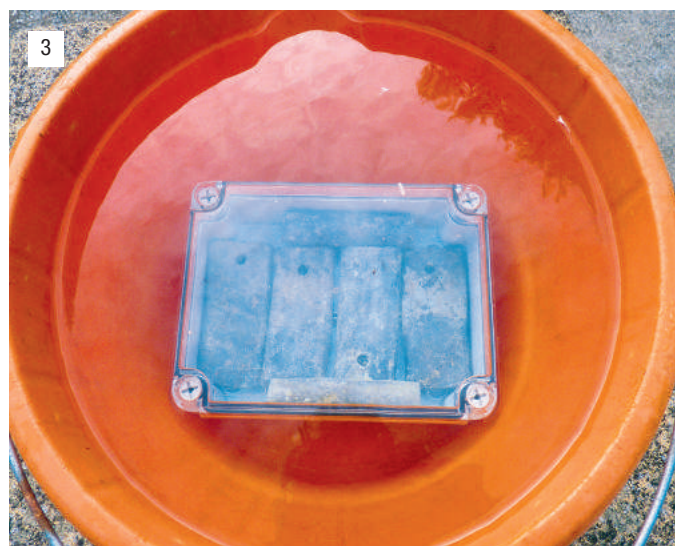
Photo 3. Waterproof test of the power unit.
