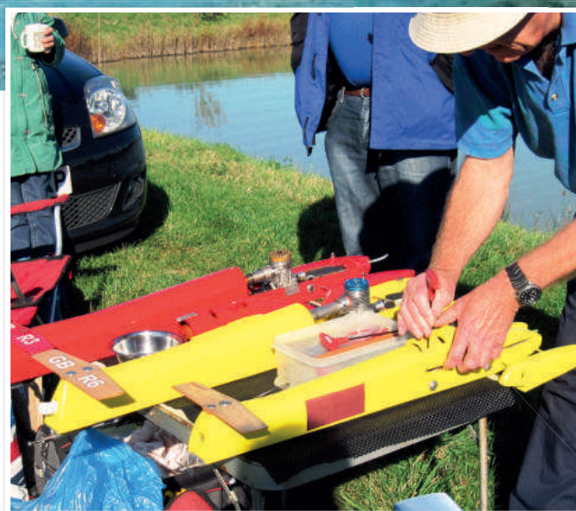
This picture is of the three red and yellow three point hydroplanes by Lynn and Hugh Blowers of the Retro Racing Club. Their models are fitted with 5 and 10cc glow motors. Popular engine brands are CMB, Picco and OPS, much the same as in r/c multi-racing boats.
