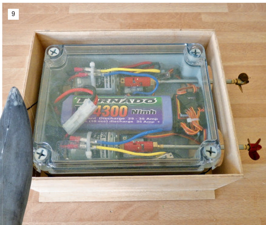
Photo 9. The power unit inside its box.
