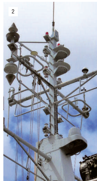
Photo 2. The head of the mast showing the various navigation lights.
