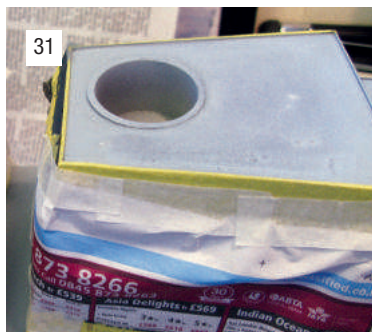
Photo 31. Preparing the fore funnel exhaust casing and the surrounding deck area. The inner part of the top of the funnel will be added later.
