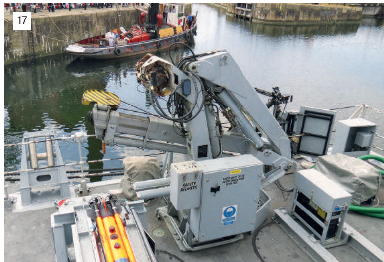
Photo 15. At the extreme stern end to port on 01 deck is a crane for the two mine clearance boats. In the foreground is the (covered) crane operator control panel on its pedestal.
