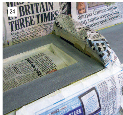
Photo 24. Cover everything! Sprayed paint has an annoying habit of going where you least expect it.
