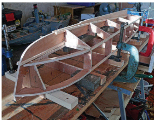
Above left: The basic hull construction of Paul Thomason's design as constructed by Bob Abell. Above right: Bob Abell's 'Ellie' in an advanced state of completion.
