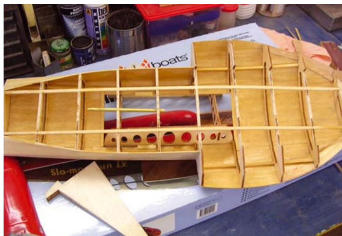
Hull of the Billings Slo Mo Shun under construction (see text)
