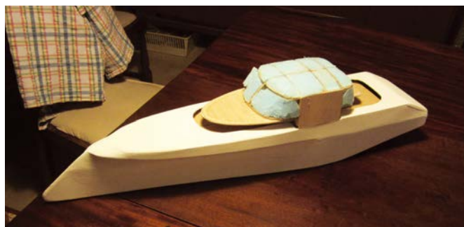
Foam infill to deck house
