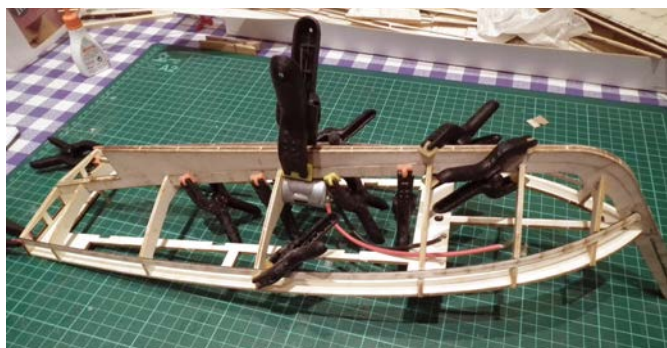
Keel fitted to the bulkheads
