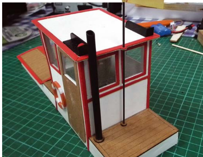
Exhaust and flag pole fitted
