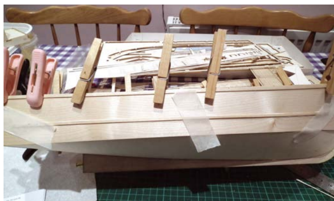
Handrail around the deck edge and rubbing strakes being fitted
