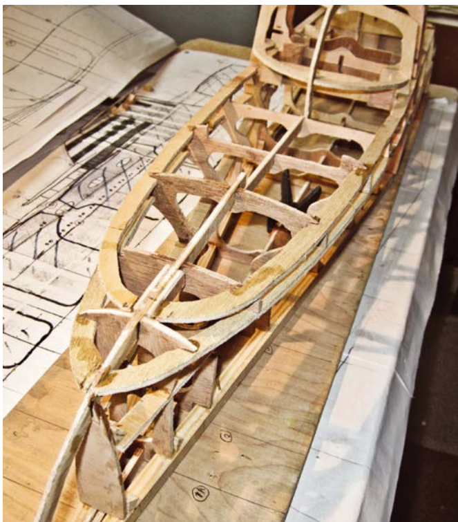
Forward of hull framework
