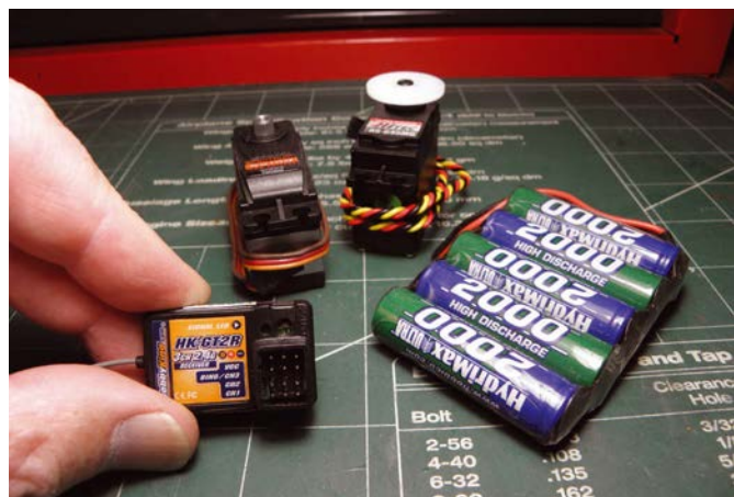
Removing a hull's entire control package may be necessary to determine the cause of a glitch especially one that doesn't easily show itself
