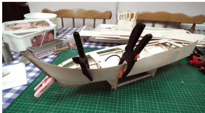
The upper skins clamped in position
