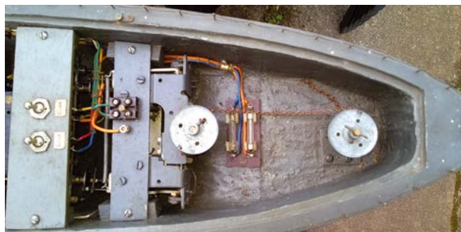
The rudder linkage has a broken chain
