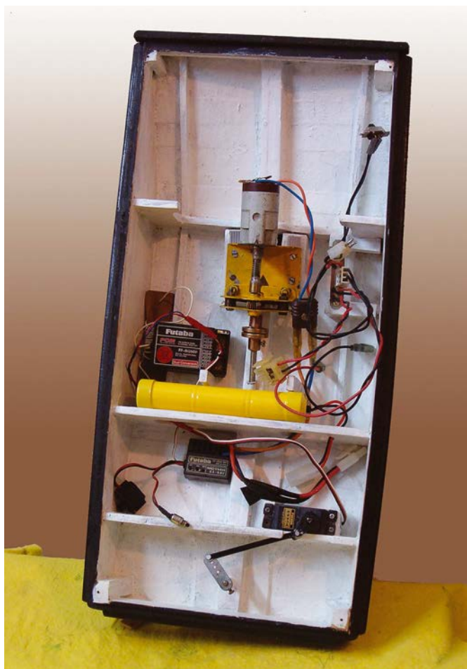
Internal view of radio and drive components
