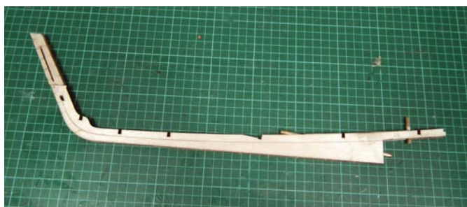
First job is to assemble the keel
