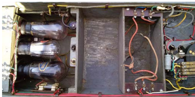
Spaces for all the different batteries required
