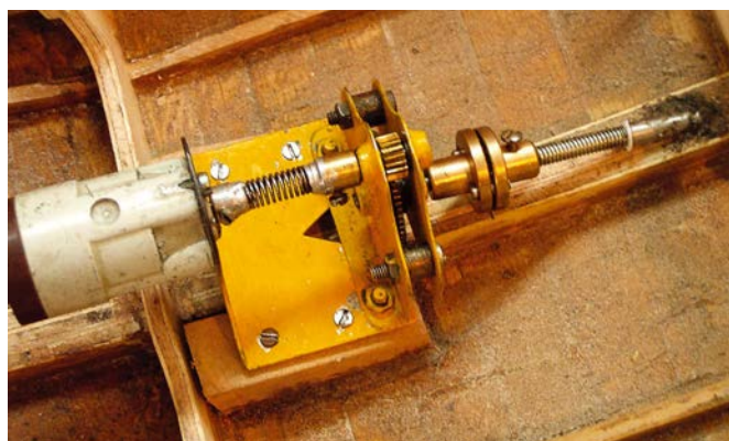
The motor and gearbox
