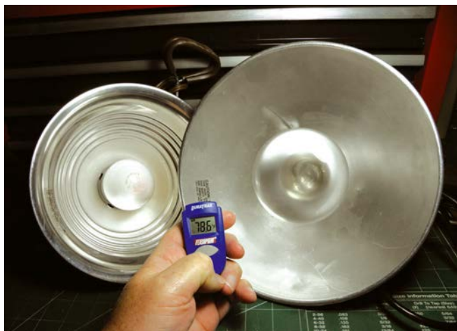
Using two regular heat lamps and a digital temp gauge our boater was able to induce the faulty rudder servo's heat problem
