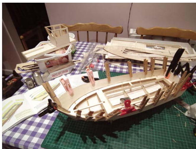
The upper skins are doubled up and need plenty of pegs and clamps!
