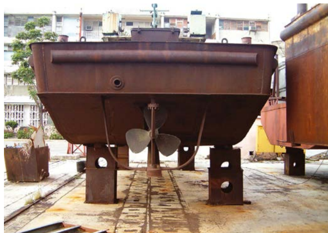
View of the stern and the propeller of a pusher (full size). These pictures were taken as a reference to make the model
