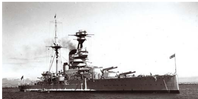
HMS Resolution in 1939 retains the original pole mast
