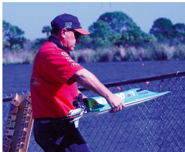
When launching any IC boat be aware it's possible to start its power plant in reverse, which could produce a strange reaction when the hull hits the water
