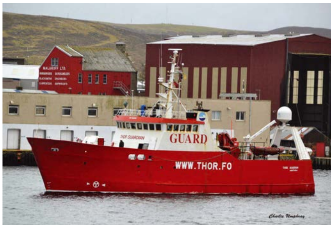
Port side view, this shows the RIB inflatable dinghy and davit, with SatNav beacon mounted on the stern gantry (pic Charlie Umphray)
