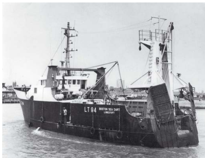
As stern trawler Boston Sea Dart, this and next, shows the extent of the rebuilding carried out for her new role (pic author's collection)
