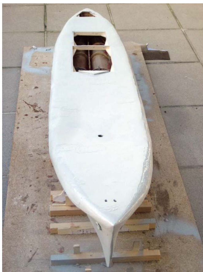
Reinforced by GRP, filled and sanded, the hull awaits its paint job
