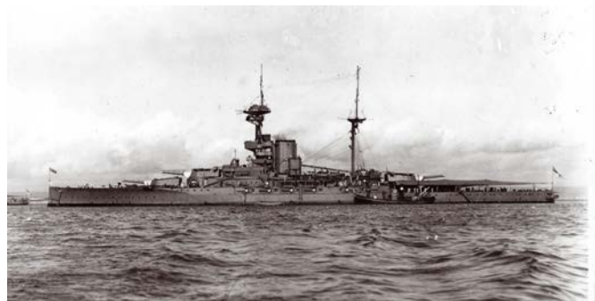
HMS Revenge 1927 with flying off platforms and uniquely the stern walk
