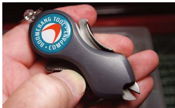
Made to cut braided fishing line this Boomerang Line snip is also useful for making clean ends on R/C yacht rigging cords that demand routing through very small sail/mast fittings
