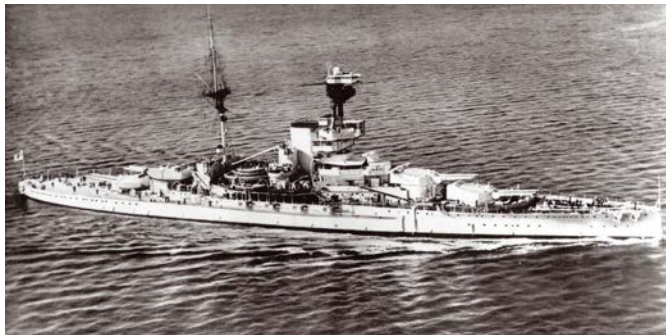
HMS Revenge 1919 with stern walk and long base rangefinders on B and X turrets
