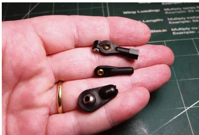
Sporting a free moving metal ball connection point, ball joint ends create a lot of available and freedom of movement points in the average IC boat linkage
