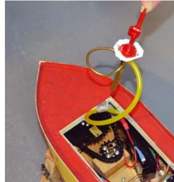
Figure 1. Feed arrangement with coiled tube and hose, and hull drive
