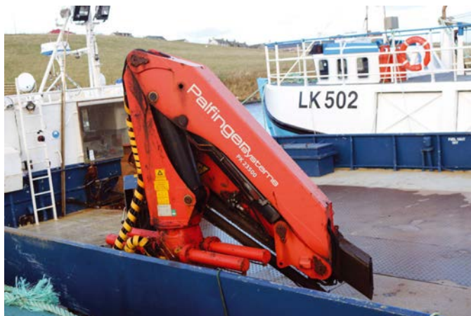
Typical hydraulic crane as mounted on numerous workboats (pic Shipsforsale Sweden)
