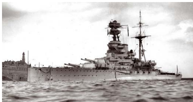
HMS Ramilles in 1939 with a tripod mast for the aft gun director
