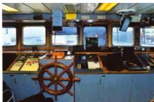
Forward end of wheelhouse with various electronic controls, still retaining a traditional wooden steering wheel, nowadays usually relegated to an ornament (pic Shipsforsale Sweden)
