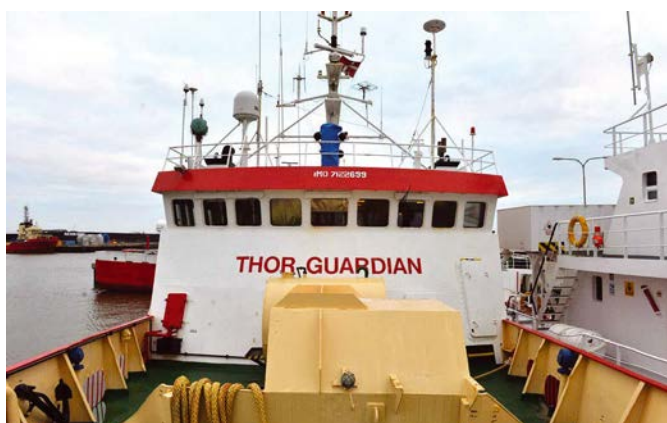
View of foredeck, with companion and breakwater in foreground, this view shows the detail of the bulwark stanchions (pic Shipsforsale Sweden)
