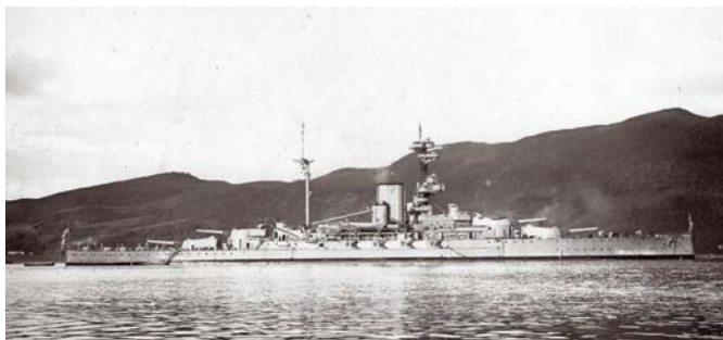
HMS Resolution 1918 with flying off platforms in B and X turrets
