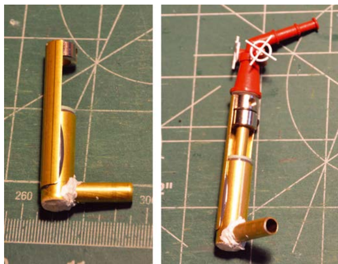
Figure 8. The completed single seal assembly, with fire monitor mounted. When installed the monitor tube must be long enough to fit a drive sprocket
