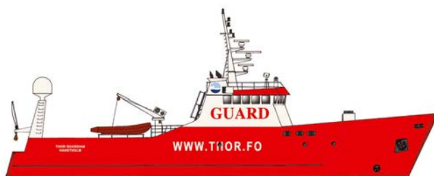
This shows that all deck erection above the main deck has been removed during her conversion (pic author's collection)
