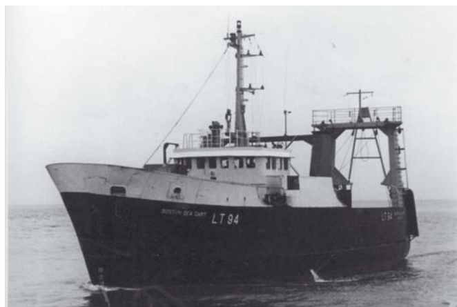
This shows that all deck erection above the main deck has been removed during her conversion (pic author's collection)
