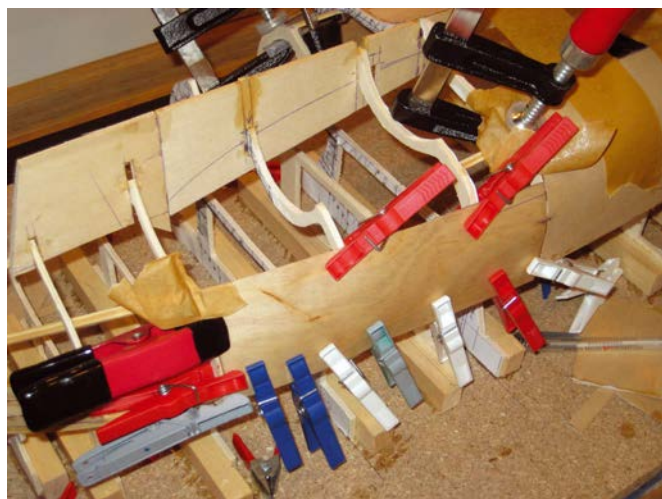
By cooking 0.1 cm spruce in hot water and bending it in shape, the building process is eased
