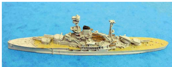
HMS Resolution in 1939 showing the X turret catapult fitted in the 1930s (AR 47)
