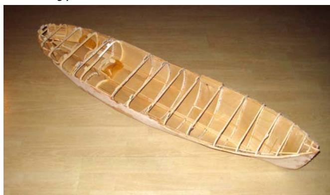
Despite 117 cm in length the hull weighs only a few 100 g (before applying the putty)
