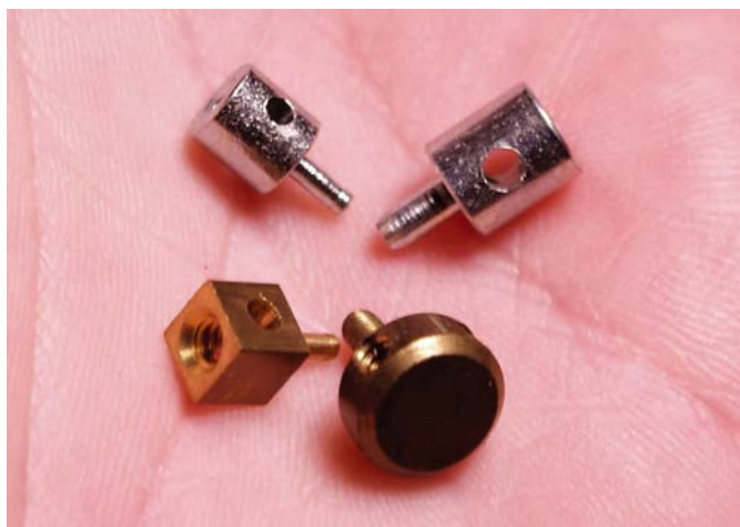
Linkage connectors can receive both metal rod or flexible cable style linkages and are normally joined to a servo, rudder or throttle arm via a small pinch washer
