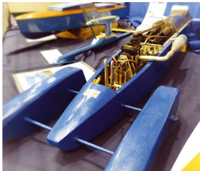
Built by Keith Norfor and now owned and restored by Kevin Fleet of the Victoria MSC, this Flash Steam Hydro (RTP) is capable of over 100 mph!
