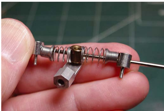
Using small springs to create a simple override function on a throttle linkage this adjustable rod prevents an overstress on your boat's onboard throttle servo motor
