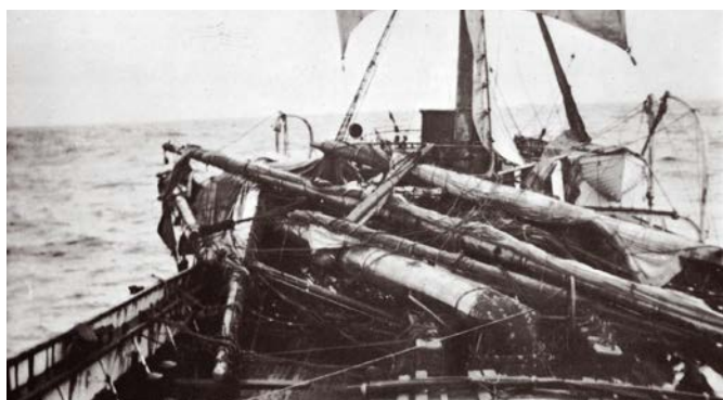
The main deck of 'Pinnas' after the dismantling. Remember this is steel wire rope rigging, and steel spars and masts
