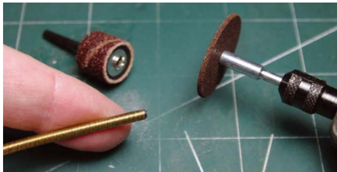
Cut to length with a Dremel tool/cutting disc setup. Multi-strand flex cables can easily connect your hull's power unit to your strut/prop design
