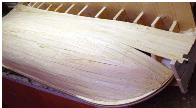
Example of planking at the bow; this model being constructed in two halves
