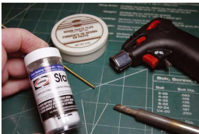
To prevent damage to your drive cable's coupler end, a small torch or high-watt soldering iron is used to flow solder into the cable end to create a solid grip point for the coupler
