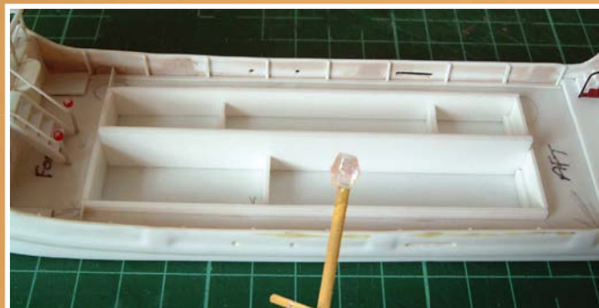
ABOVE: Freeing/wash ports drilled out; interior bulwark surfaces filled and detailed; hatch coaming constructed
