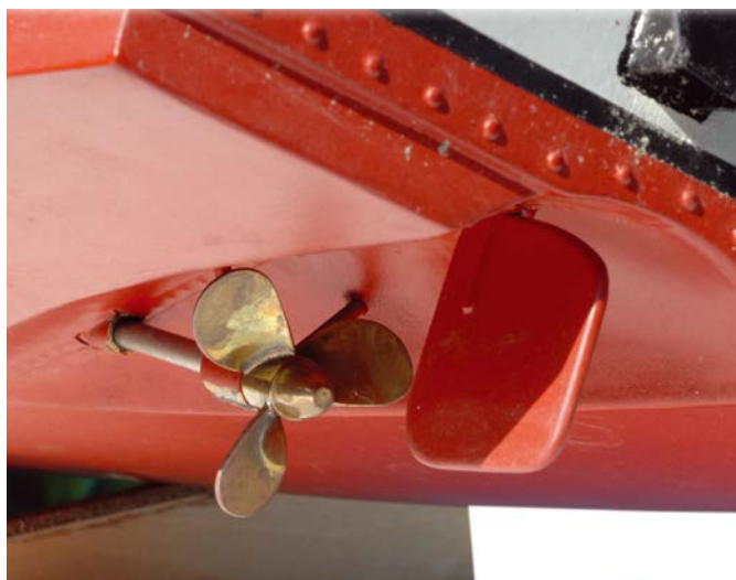
The tunnel is, in this case, rounded, unlike the original configuration that has a rectangular shape
