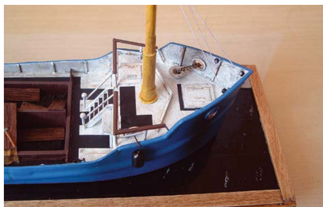
Finished forecastle and deck detailing: showing cargo hold, fender, mast stays, hawsehole with anchor chain and anti-slip walkways
