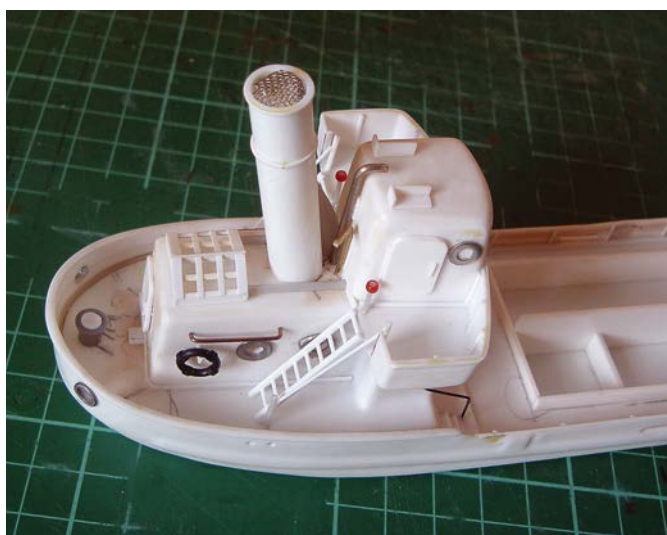
Rear deck/superstructure detailing of wheelhouse and engine room: showing rubbing strips, funnel, life rings, porthole frames, railings etc
