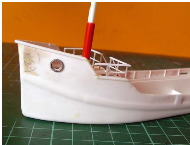
D-section rubbing strips applied; solder wire framing of anchor port; filling of bow sides
