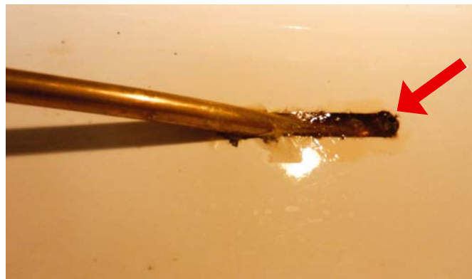
The shaft exit on the Cat. The arrow points to the tiny hole
