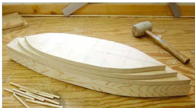
An example of bread and butter construction to waterlines
