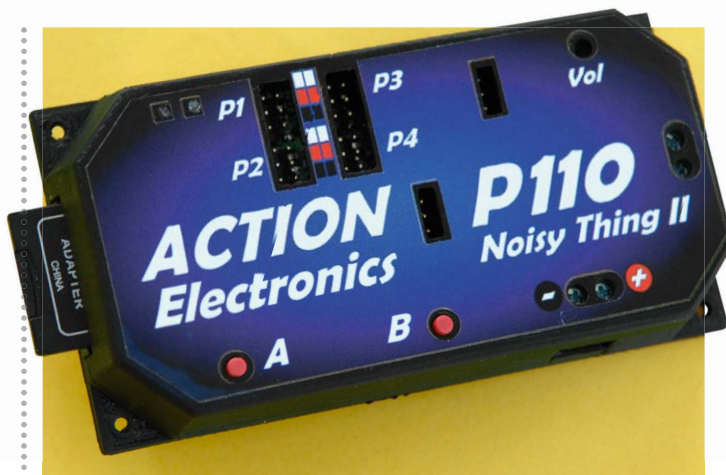
The P110 in all its glory showing the clarity of the printed label. Note the SD Memory Card slid into the left hand side
