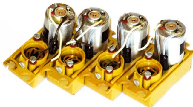
KPS12 motors and pot wipers tested, cleaned and refitted
