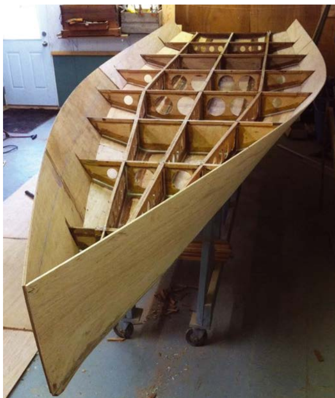
Example of part egg box construction on a full size sailing skiff
