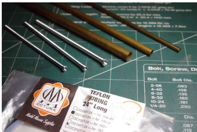
Forming a proper stuffing tube will involve whatever tube bending tool is needed along with a tube liner like the Teflon style sold for powerboat usage
