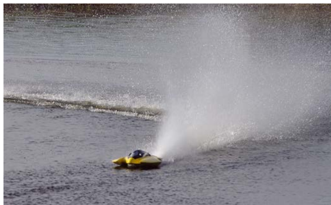
An excessive amount of spray from your hull's propeller could indicate an over-sized blade or a misaligned strut, which, if left in place, could over stress the whole driveline
