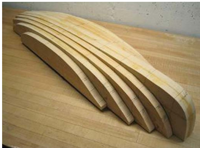
An example of bread and butter done to buttock lines
