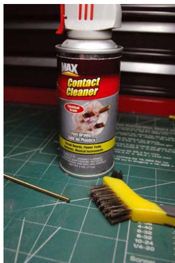
Over time, a flex cable's strands can get clogged with old grease so cleaning it with a fine wire brush followed by a solvent clean up keeps the cable spinning smoothly in the tube
