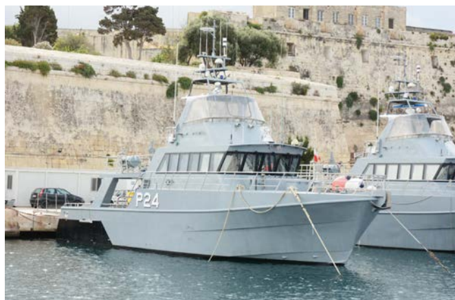
P24 is a 21 m Austal Class Inshore Patrol Vessel built by Australian boat builders Austal and was delivered to Malta in February 2010. It's operated by the Maritime Squadron of the Armed Forces of Malta
