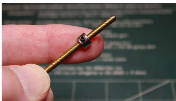
Aircraft-style wheel collars can also prevent cable loss when attached at the engine/stuffing tube gap
