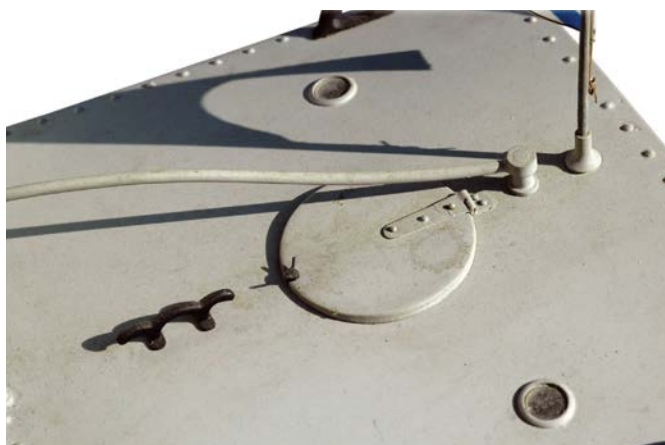
The access to the Stirling engine compartment, and on each side, two small portholes that provide a semblance of light
