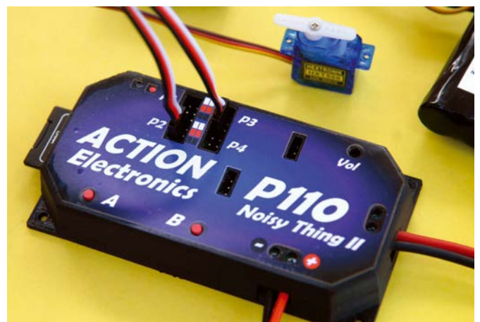
Note the Throttle channel connected to header P2 to trigger engine start, run and stop sounds and a spare channel connected to P3 to trigger individual sounds
