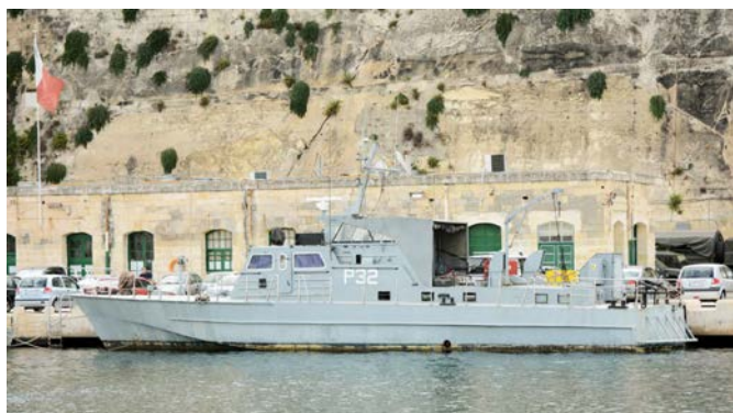
P32 is an East German Bremse Class boat that was decommissioned in 2012 and is seen here moored at Hay Wharf in Malta's Grand Harbour. Note the addition of a fixed cover behind the bridge that replaced an earlier canvas cover
