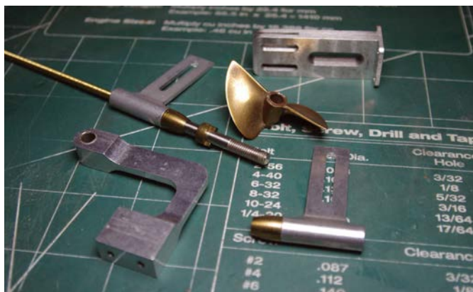
Along with the placement of the engine, the alignment of the strut/bracket and the cable drive dog gaps must be factored in to prevent problems
