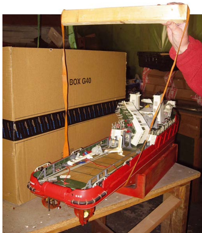
Launching straps that can lead to serious damage to a model if it slips out!
