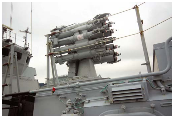
Twelve barrelled RBU-600 anti-submarine warfare rocket system can fire 212 90 ASW rockets or RGB-60 depth charges
