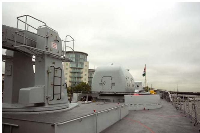
Starboard side looking forward showing the launcher for the SA-N-12 SAM and the AK-190 main gun
