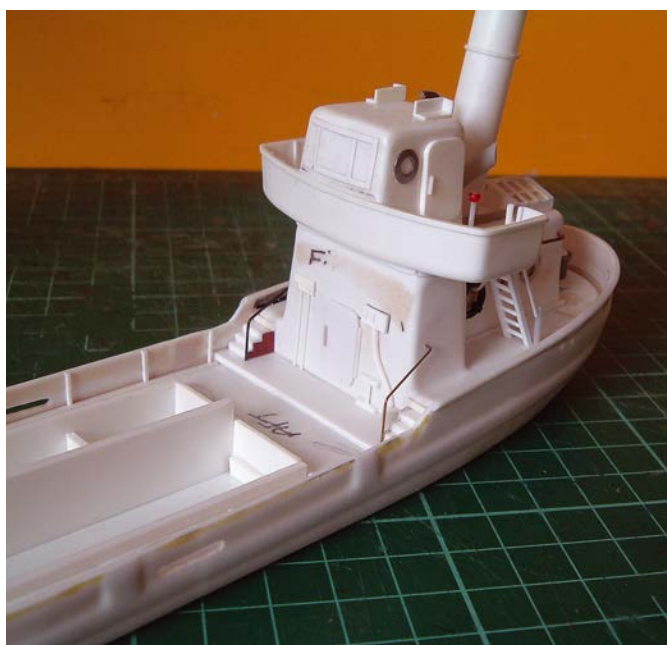
Detailing on bulwarks, wheelhouse and superstructure bulkhead: showing horizontal freeing ports, filled area, window frames, steps and navigation light boards
