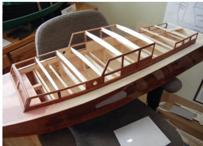
Completed cabin 'skeleton'
