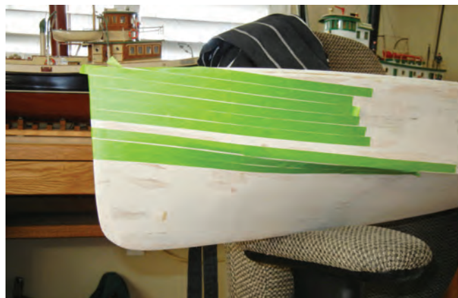
Simulating mahogany planks with masking tape
