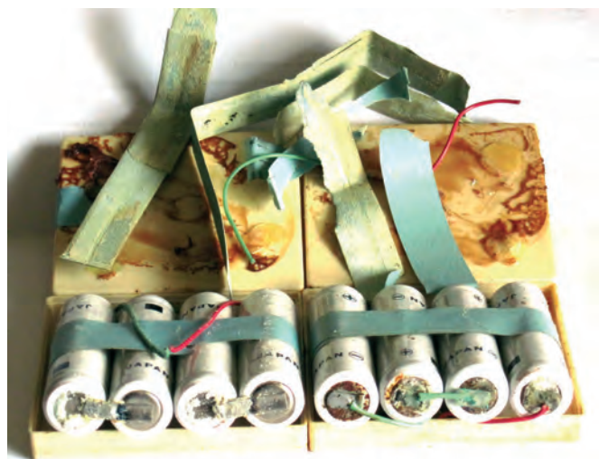
Rotten NiCads are found in all old R/C. Here, 500 mAh AA cells x 8. I've seen worse!
