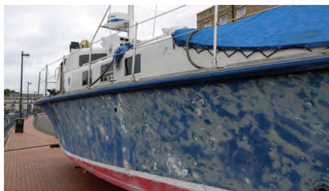
The diagonal planking is clearly seen after the initial rubbing down
