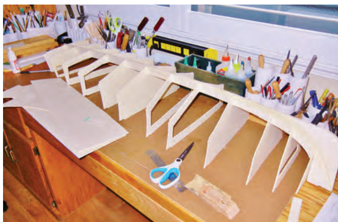
ABOVE & BELOW: Keel and frames being modified
