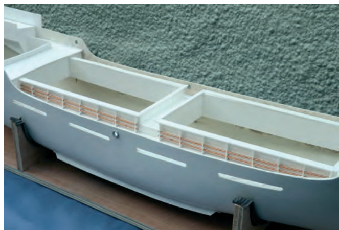
Hatch capping rails fitted
