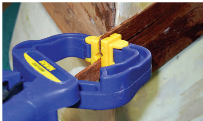
ABOVE & BELOW: Applying and sanding mahogany planking veneer
