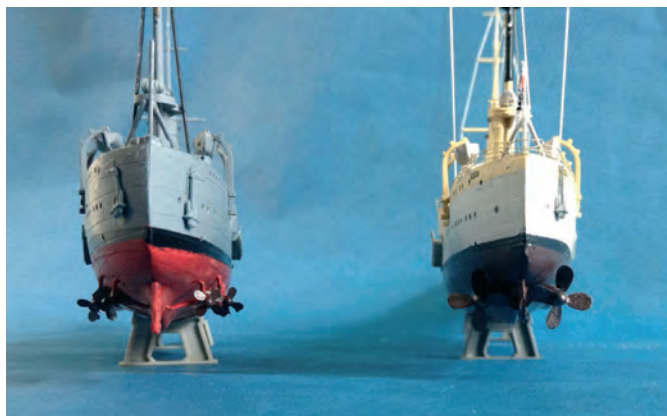
An unusual view of the sterns of the SMS cruisers, Dresden and Emden. Dresden possessed four shafts in comparison to Emden's two
