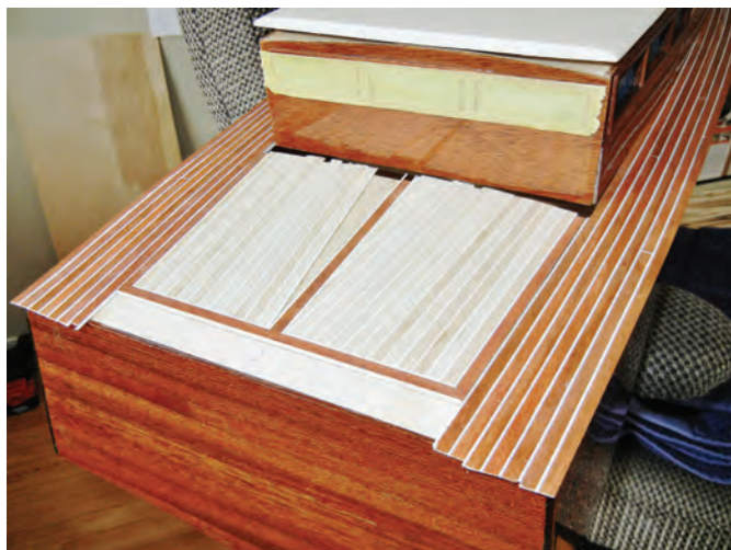
Planking of bridge/stern decking
