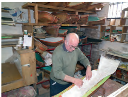
Bryan demonstrating the laying up of a GRP hull
