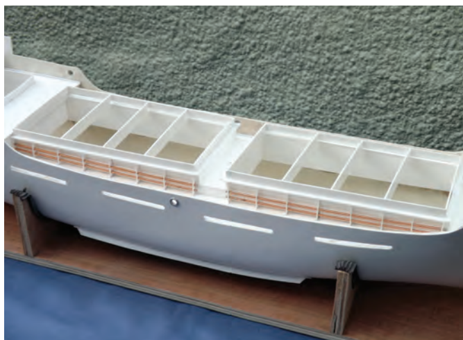
Freeing ports completed
