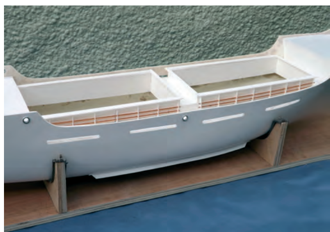
Hatch support and rails fitted
