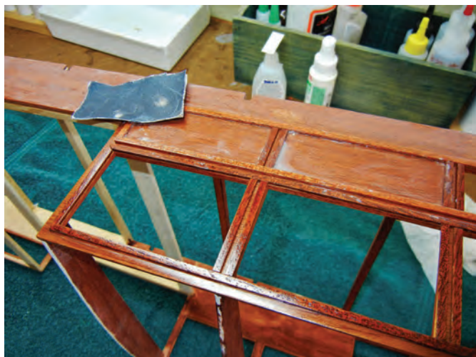
ABOVE & BELOW: Mahogany veneer being positioned and applied
