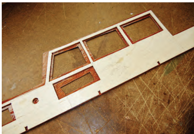
ABOVE & BELOW: Mahogany veneer being positioned and applied
