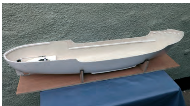
Stringers in place
