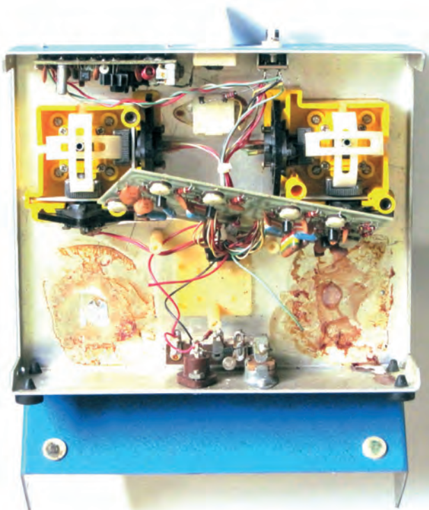
Getting started on transmitter strip down. Marks are old glue from the battery cases
