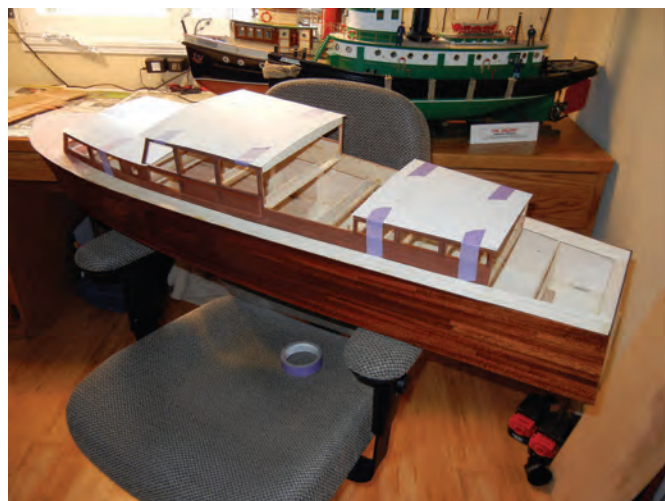
Epoxy reinforced cabin roofs being fitted
