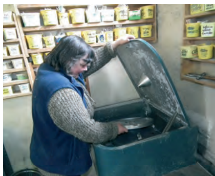
Ann using the white metal casting plant
