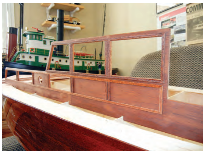
Cutting, sanding, fairing of laminated mahogany cabin sides
