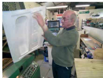
Bryan taking a hull out of the vac form machine
