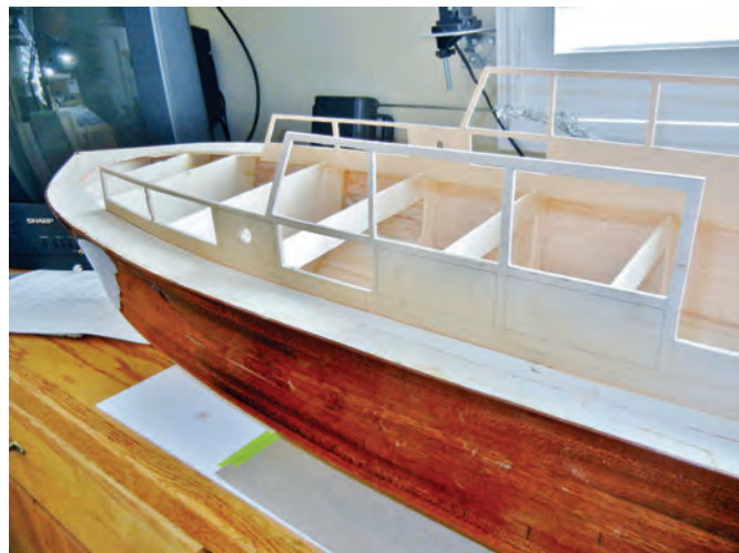
ABOVE & BELOW: Fabricating cabin side structures
