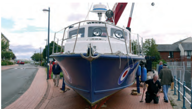
Bow on with the final wedges being hammered into place
