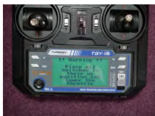
A switch on a warning screen is shown if the switches are not in the up position and the control stick down
