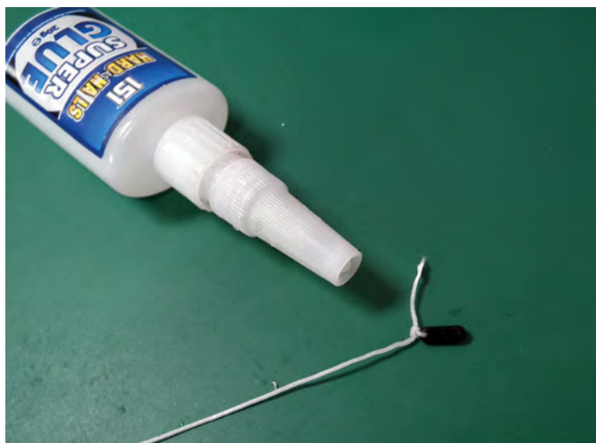
A small drop of superglue will help the knots not to undo but be careful not to block the bowsie holes
