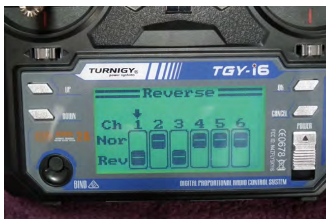
In the set up you can reach the reverse function and set as required
