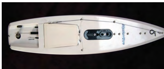
To seal the hatch a single waterproof patch can be used or as shown a piece of plastic can be made and sealed with adhesive tape
