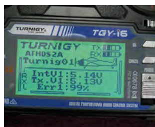
With the Rx switched on the voltage of both Tx and Rx can easily be seen
