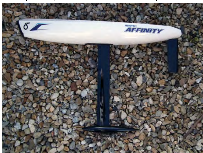
The underwater parts (keel, balance weight and rudder)
