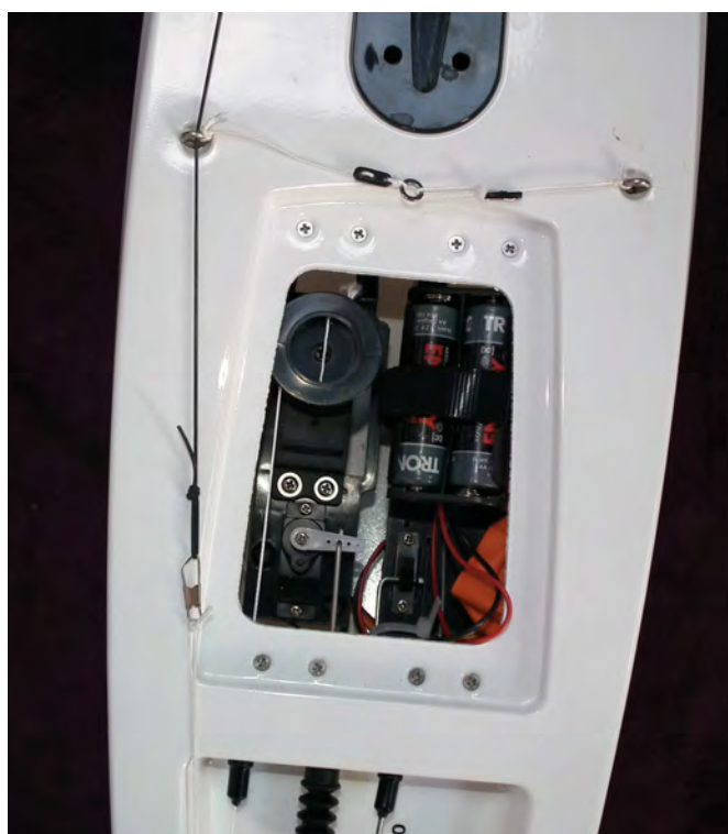
A cosy fit but easy access for the servos, batteries and receiver
