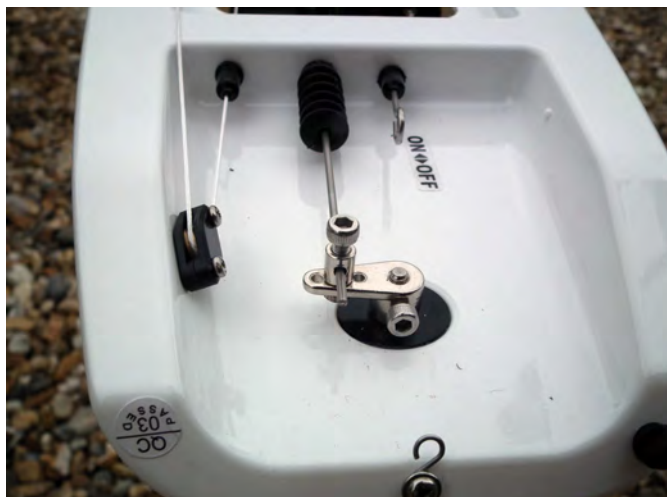
The stern well area with fittings and adjustment for the rudder and push/pull on/off switch
