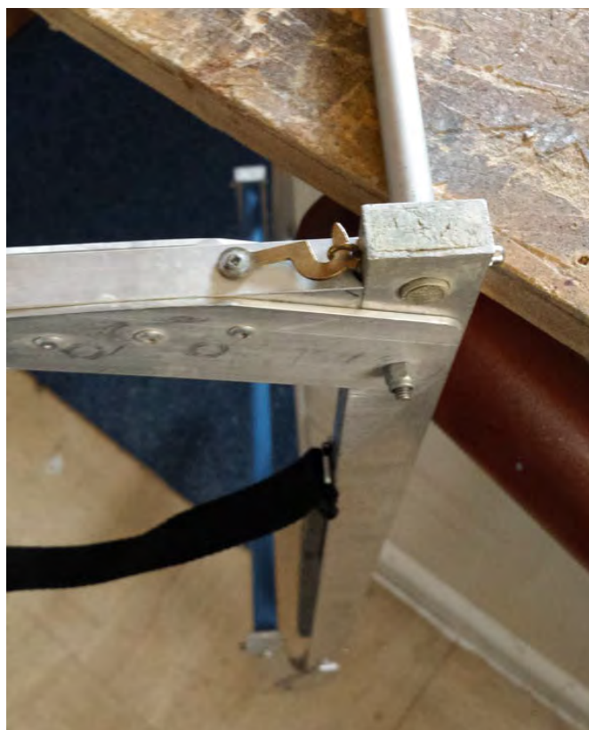
Hook and eye latch to lock into position
