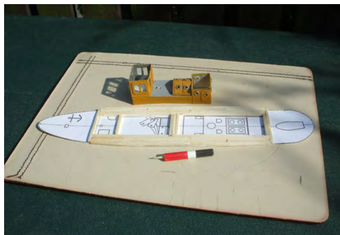
Copy of the plan glued to card and planking being applied
