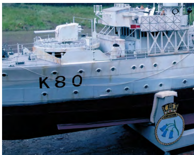
Folded ammo davit near the armour plate side panel. Note oil scum at waterline. When picking up survivors, K80 often wallowed in fuel oil
