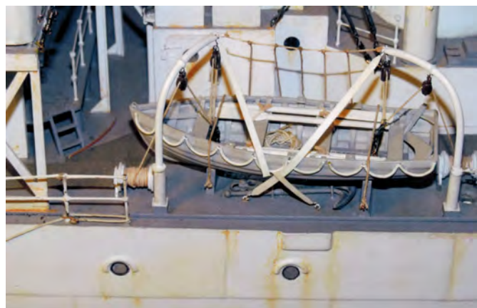
Kedge Anchor shackled to deck under portside whaler
