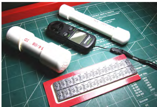
Made up from regular PVC pipe/fittings, a ballast tube (or two) can be secured in your hull using Velcro or nylon ty-wraps
