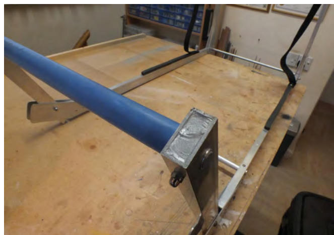
Top tube reinforced with wood block
