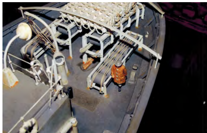
Stern towing arches and wood pallets and degaussing cable
