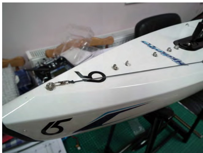
The bow deck area showing deck eyes and winch tension elastic cord
