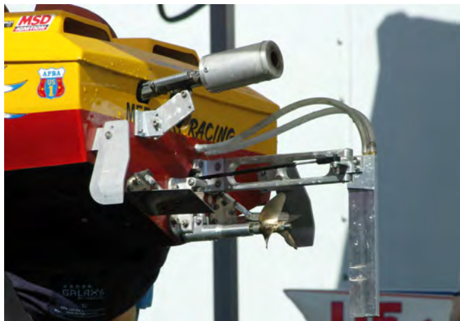
One of the main areas to help combat rough water will be the hull's adjustable transom gear, which can be tweaked for wind/wave actions
