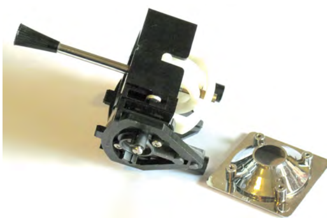
EK Inc's ‘mono ball’ adjustable tension stick
