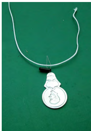
Threading rigging through bowsies can be helped by using a sewing needle threader
