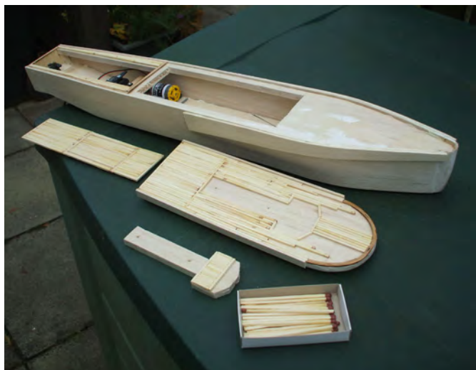
'Planking' the decks (long cook's matches). In front is the small superstructure and the 'footprint' for the wheelhouse
