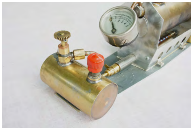
The gas tank
