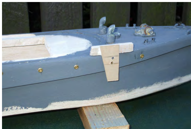
Portholes being installed using a simple jig (also some fittings being temporarily fitted)
