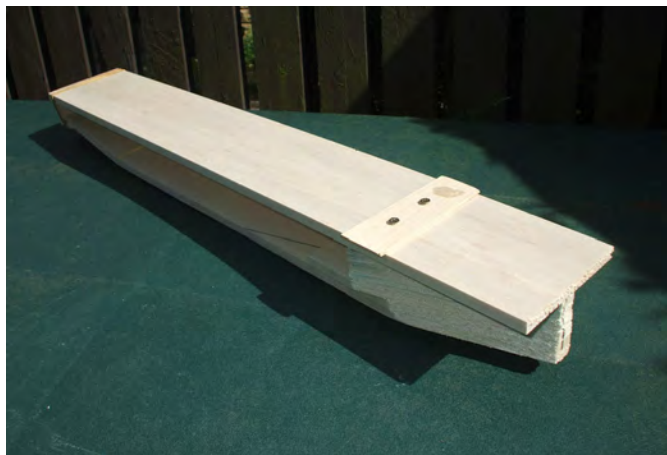
The top deck screwed to the 'b&b' section for cutting, shaping etc
