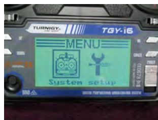
The first menu screen is reached by pressing the OK button then you can go to the system or set up
