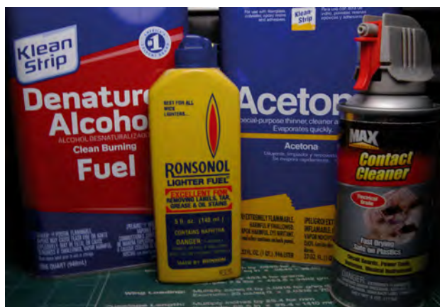
Different chemicals can produce extreme negative reactions to many plastics especially the kind found on many older nitro boats sold in kit form
