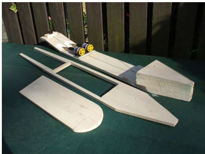
The hull bottom with motors/propshafts installed. The top deck with access opening and upper deck
