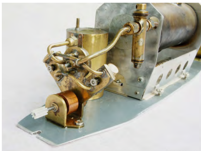
The engine with its output, which will be geared down by 2:1
