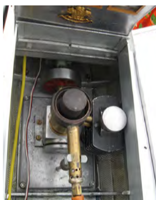
The Sterling hot air engine in John Hanson's Evergreen
