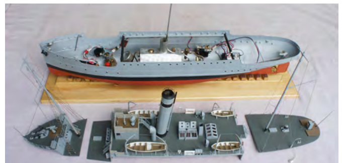
For access to the internal machinery the decking was completely removable
