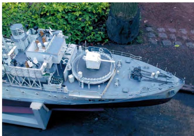
Anchor stopper chains. Bagged ammo at 4" gun. Canvas covers kept salt grime off ammo
