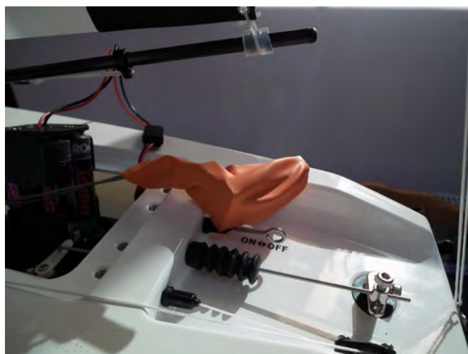
It is a good idea to place the receiver in a rubber balloon to make it waterproof
