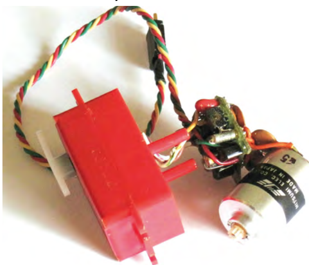
A view inside the tiny EK ‘super-mini’ servo
