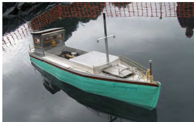
Evergreen, by John Hanson of Margam Park MBC, powered by a Stirling hot air engine and solar panels
