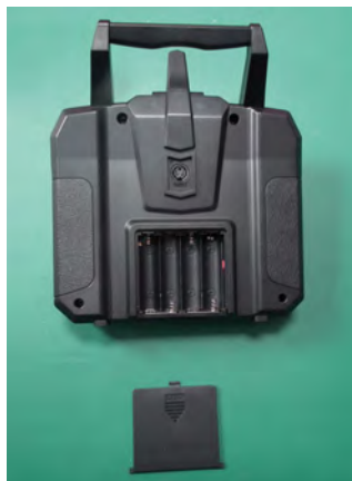
The rear of the Tx showing the battery compartment
