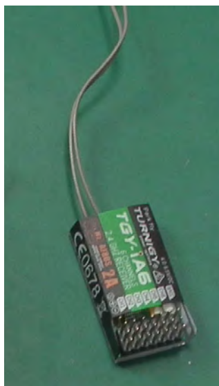
The receiver with the two antennas which should be set 90 degrees apart
