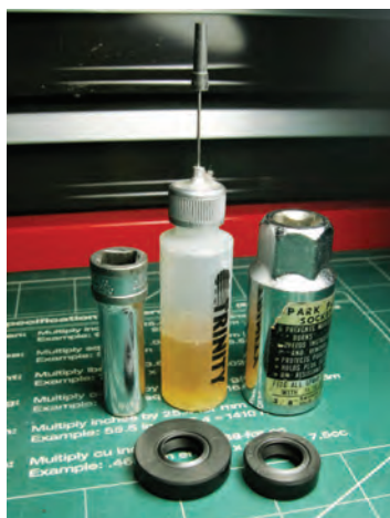
Regular metal sockets can act as both your crankshaft seals and ball race installers and a bit of premix oil will lubricate the parts to help ensure they aren't damaged during the install process
