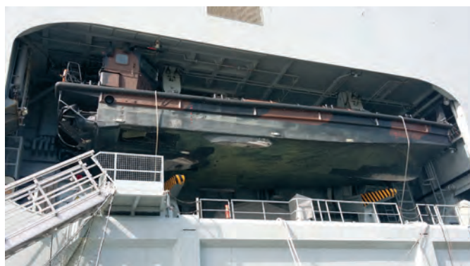
One of HMS Ocean's LCVP Mk5B in her davits on starboard side
