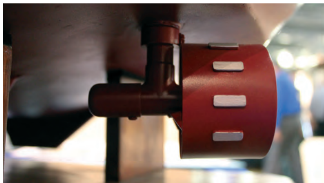
The homemade schottle unit that powers 'Giano'
