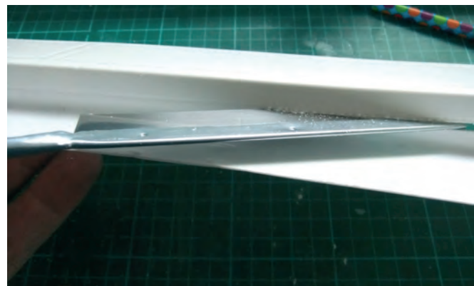
Removing the moulding from the base plastic with a fine-toothed saw
