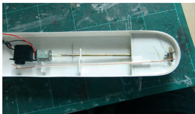
Inside with the motor, propshaft and rudder now fitted
