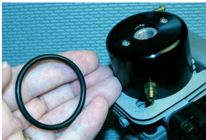
Often over-looked the large rubber O-ring used on the cylinder/water jacket joint should be replaced along with pistons, rings and other internal engine parts as well
