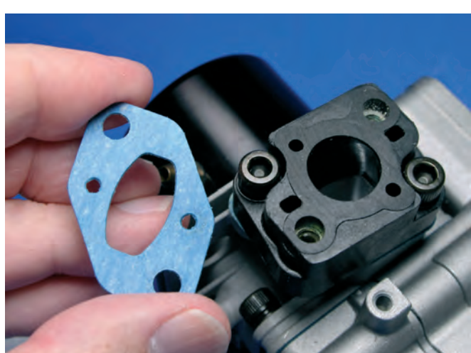
Due to any warpage in a composite manifold block its sealing gaskets must be replaced, as leakage in this spot will upset the engine's total start/run actions
