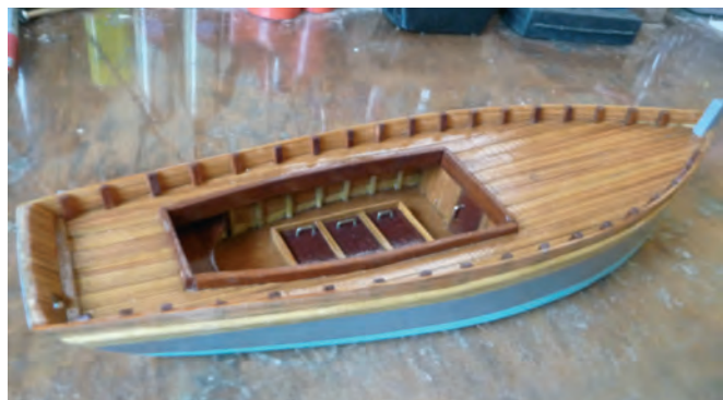
Hull ready for bulwark capping
