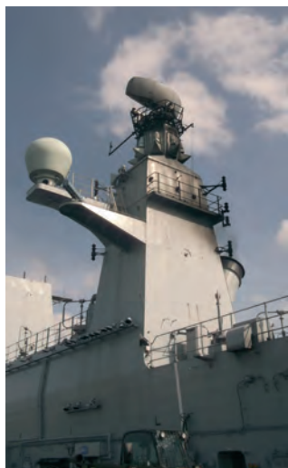
HMS Ocean's aft main mast. Note the radar aerials and satellite communications equipment
