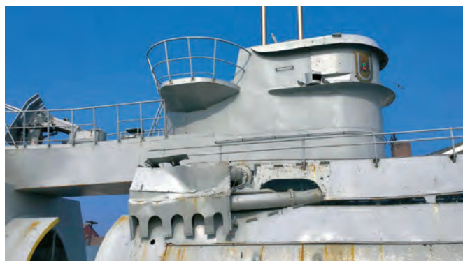
The centre section divided under the conning tower with viewing windows at either end of each section. The gun just visible is the original twin 3.7 cm AA gun
