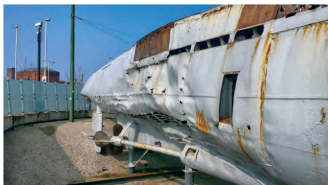
The aft section, showing the damage caused by the depth charge, which exploded under the boat. The open hatch (door missing) is the Pillenwerfer chute, which released a device designed to confuse attacking ships' Asdic by releasing oxygen bubbles when away from the U-boat's hull. The bubbles were generated by a chemical reaction to the seawater
