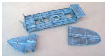
The underside of the decks showing the reinforcements necessary for rigidity
