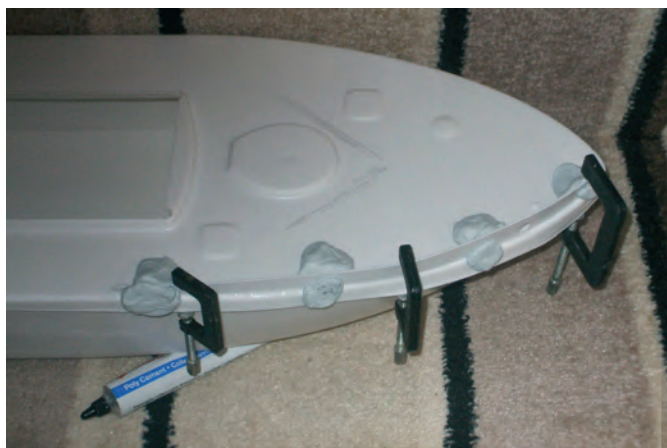
Fitting the low bulwark (spray/kick strips), around the bow
