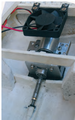
The handcrafted coupling between the engine and the axis of the propeller was made of a spring welded on both ends
