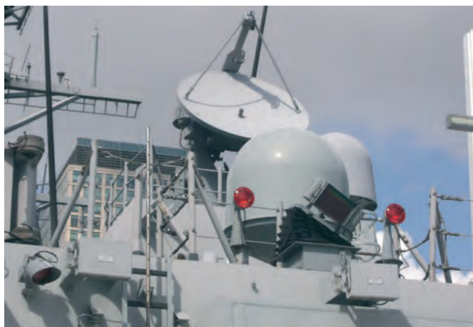
Close up view of radar and antenna on hangar roof
