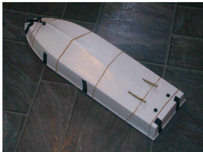
Finally fixing the deck down to the hull, utilising rubber bands and tape, as suggested
