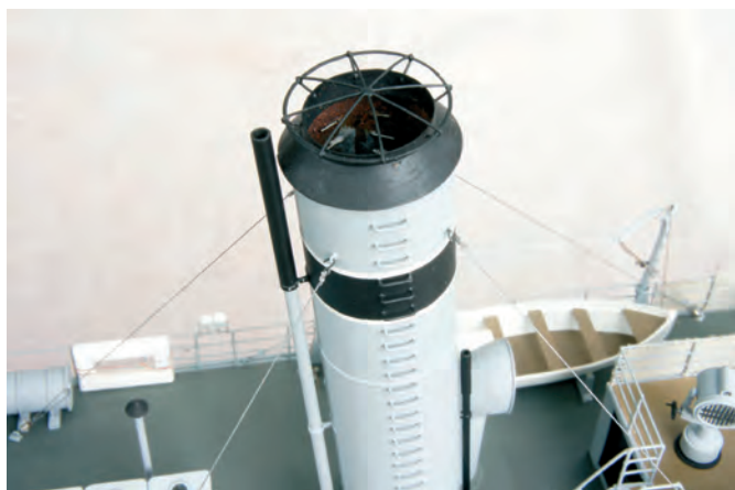
The funnel was made from a curved and soldered sheet of tin
