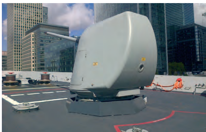
ABOVE & BELOW: The main gun is the American 5 inch/54 Mk45
