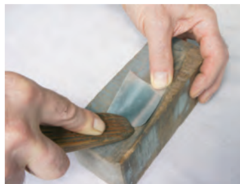
Plating panels are formed using a hard wood pusher by rubbing and pressure in a hard wooden block
