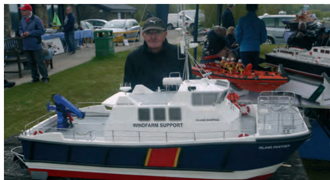
Ken Hawker's Island Panther built on a Models By Design hull and superstructure, and powered by twin Robbie Water Jet Thrusters. The crane was from Max Mouldings
