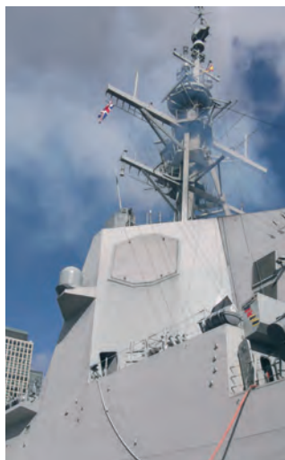
The important Aegis style radar arrays on the stealthy forward mast
