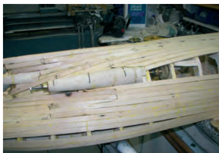
Basswood planking of the rear hull section in progress
