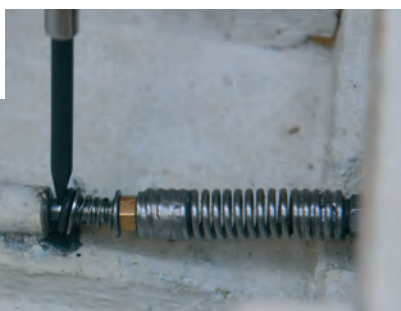
A locknut on the coupling used as a universal joint; another small spring on a metallic washer and a rubber washer prevent water from getting in through the axis of the propeller
