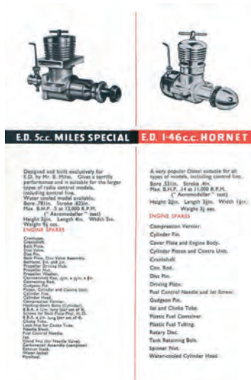
The spec' sheet for the 5 cc E.D./ Miles 'Special'
