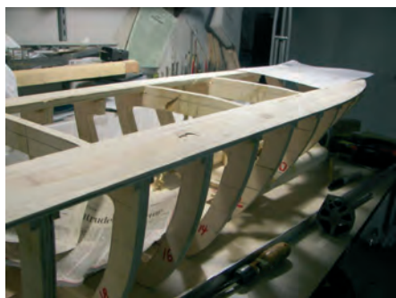
Ready for planking
