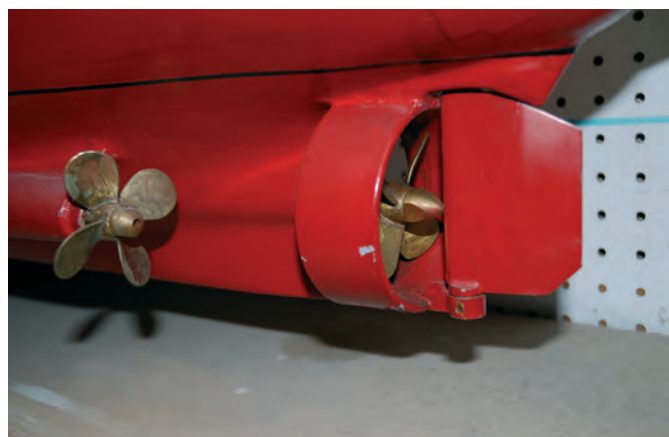
Kort nozzle flanked by two open propellers
