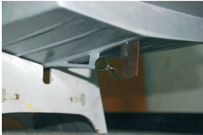
The handcrafted 35 mm two-bladed propeller
