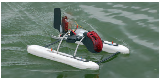
Alexis's 'mosquito', with a cockpit made from a PC mouse, the landing gear from an autogyro fitted with foam floaters and a small electrical plane engine. Notice the electronic elements protected inside a plastic bottle
