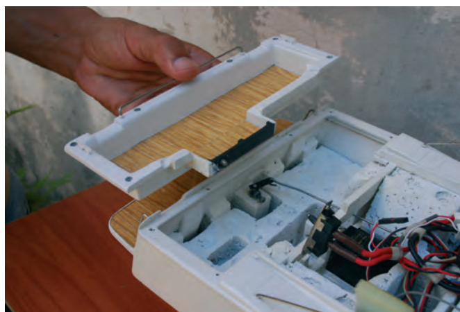
Making the cockpit (a part of the floor in the stern) was another problem, for there was very little room underneath for the servo
