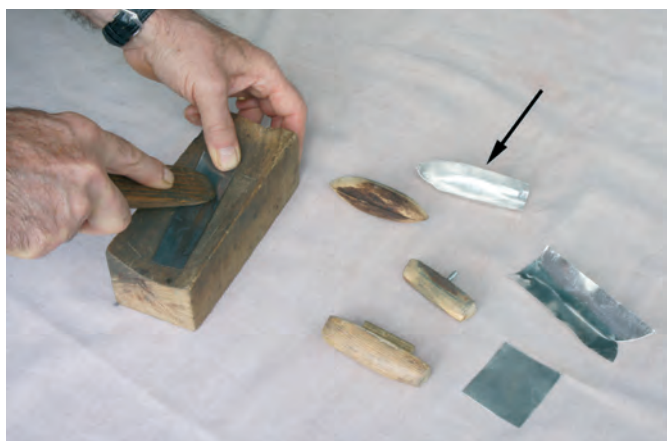
The boats are shaped on hard wooden templates. The arrow shows a first shaping, which with a little patience, will become a beautiful boat
