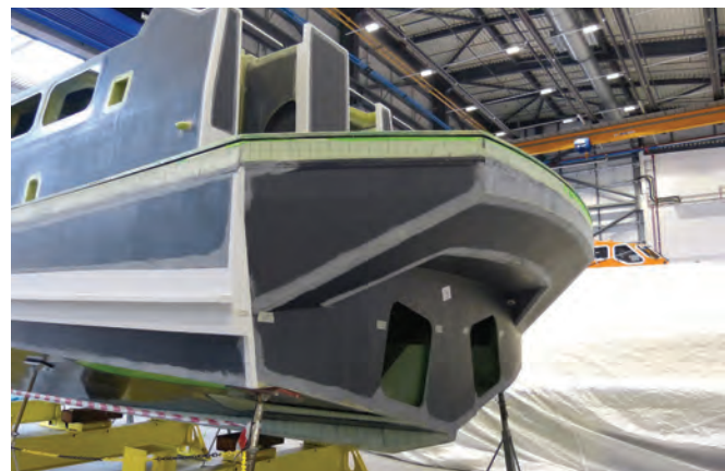
The stern quarters of 13-23, giving vital data for the model builder into the measurements and angles. Note the stainless steel datum marker screwed to the vertical corner – how often do we see that detail on a model?
