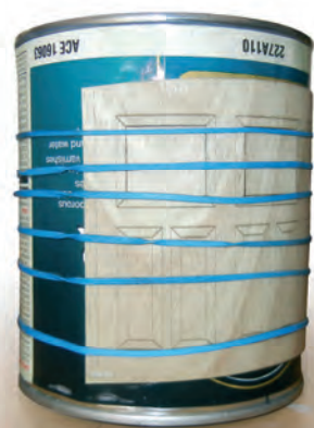
Thin birch plywood wheelhouse front curvature being coaxed with rubber bands, ammonia water spray and a paint can
