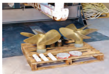
The reconditioned five-bladed Tamar propellers and the old sacrificial anodes waiting refitting
