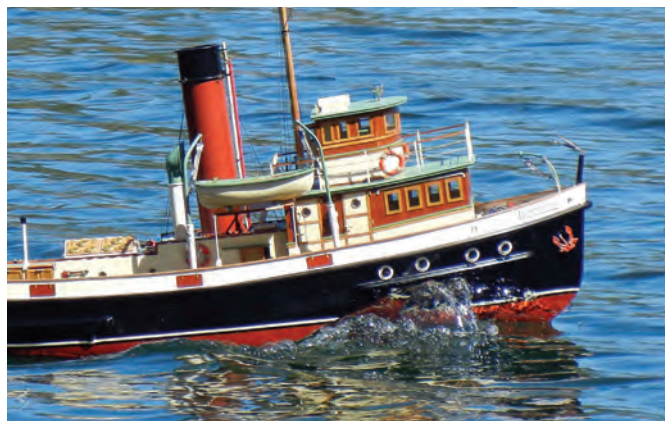
This picture shows how the colour scheme was altered. The 'yacht' look was accomplished with mahogany stained veneers, birch and basswood
