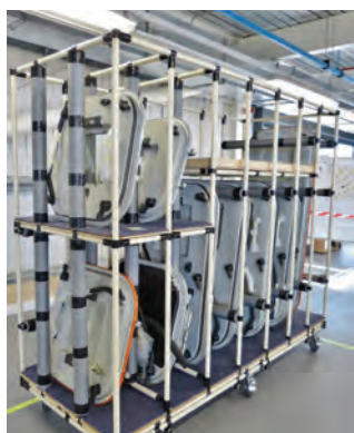
Once the doors and hatches have been given a 'dry' fit to their respective boats they are placed on these trolleys, off the floor, to keep them in pristine condition – awaiting the final fit
