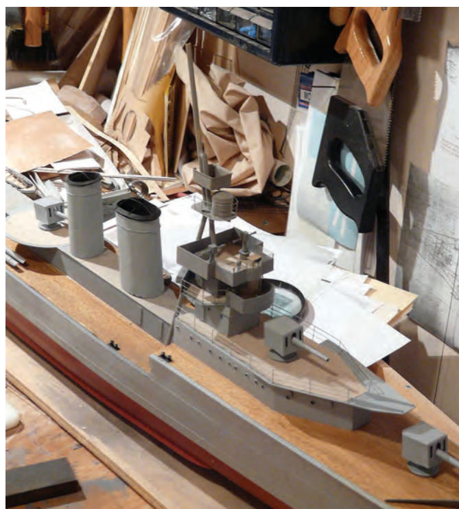
Bridge nearing completion, with guard rails round B turret fitted. The decks are all planked, from 1/32" basswood cut to 3/32" strips
