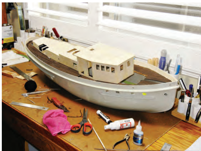
The removable main cabin was fitted to the deck after cabin sides were enlarged
