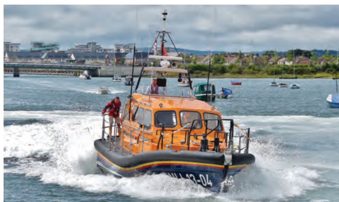
Shannon class lifeboat 13-04 RNLB Storm Rider – named by the younger RNLI members of the Storm Force club – being stopped forcefully by dropping the water jet buckets and creating a forward rush of water!
