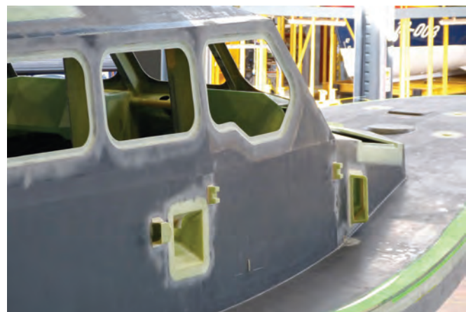
Further detail – the boat hook protection nacelle, engine room breather inlets, survivor cabin outlets, window profiles and the boat's centre of gravity stainless steel datum mark for lifting purposes. They look like they came from Macs Mouldings!
