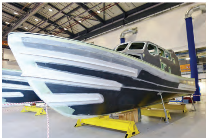
Shannon class 13-22 with its three portside bow spray rails and stern ones fitted. Looks just like one of my lifeboat models in the workshop – all blue and grey!
