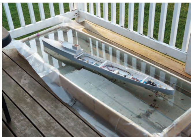
Ballast test. The model was too long for the bath, thus the tank on our deck. Plating completed from thin card before painting
