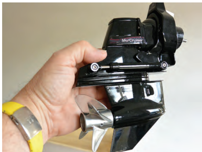
The completed stern drive fitted in position
