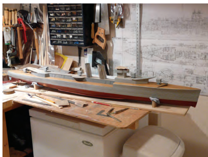
Main superstructure complete. Note much of the structure is ply but the funnels are tin plate
