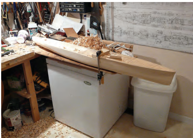
Hollowing the hull is fairly hard going. I had to be very careful not to take too much out, using callipers and simply feel
