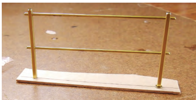
Linear brass stock was used to fabricate stanchions and railings
