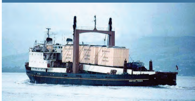
Aberthaw Fisher with two heavy loads on trailers with the lorry attached resting on the roadway, proceeding underway on the Clyde (photo courtesy Paul Stratthdee)
