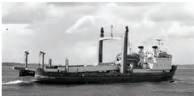
Aberthaw Fisher with a large load positioned on the forward end of the roadway. The roadway, the adjustable roadway after guideposts and ramp hoisting posts are prominent on the after deck (photo courtesy WSSPL)
