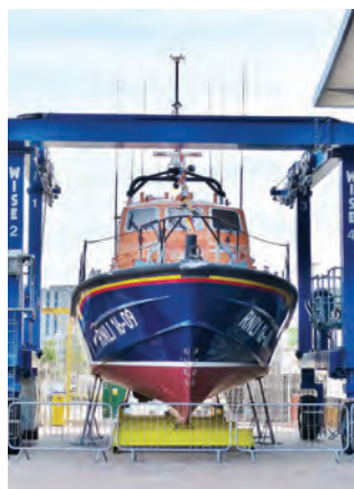
A 16 metre Tamar class lifeboat 'RNLB Baltic Exchange III' 16-09 from Salcombe in Devon on a four post Wise boat hoist
