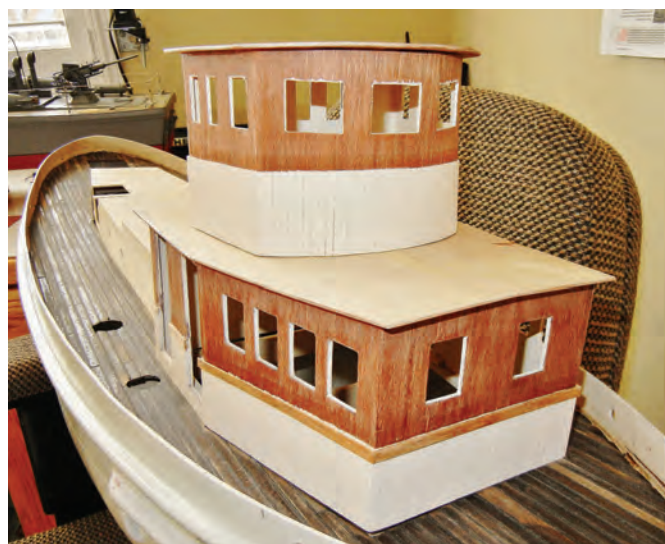
Here can be seen the wanes coating, mahogany veneer and trim being fitted
