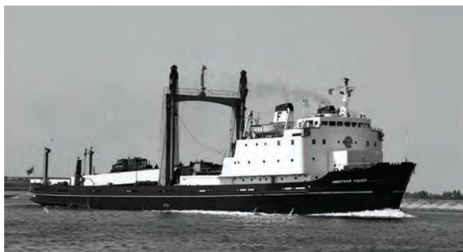
Aberthaw Fisher under way with transporter vehicle on the roadway, the starboard guide post and ramp hoisting posts are evident aft (photo courtesy WSSPL)
