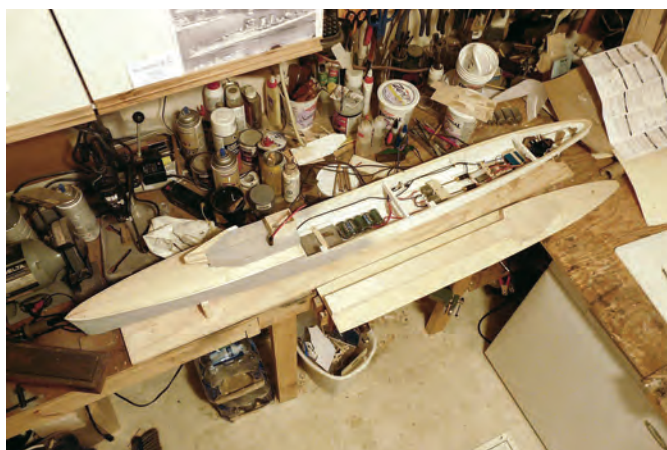
Mechanicals and electrics fitted. Note charging lead plugged into a 'to be' hidden socket (under a removable hatch), and main deck cut and ready for planking
