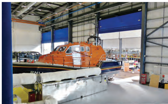
In the second boat bay (AG5) Bembridge's Tamar class lifeboat 16-17 undergoing a forward bulkhead reinforcement build and some stern driveshaft upgrades
