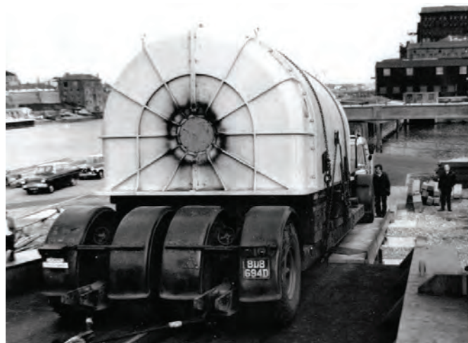
Typical of the indivisible heavy loads handled by Edward Beck & Son Ltd of Stockport. Here seen backing up the ramp and hence on to the roadway, a wire cable from the winch at forward end of the bridge deck assists (photo courtesy Edward Beck)
