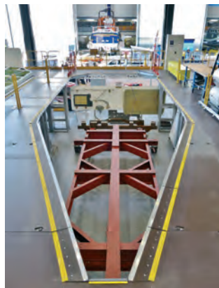
Designated bay BG6 awaits its new Shannon hull for fitting out in this custom built set-up
