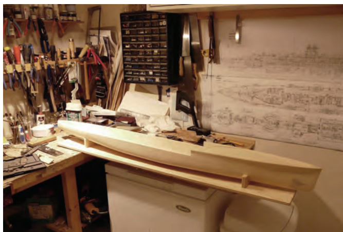
Fully hollowed and ready to fit ply decks, which will be planked later
