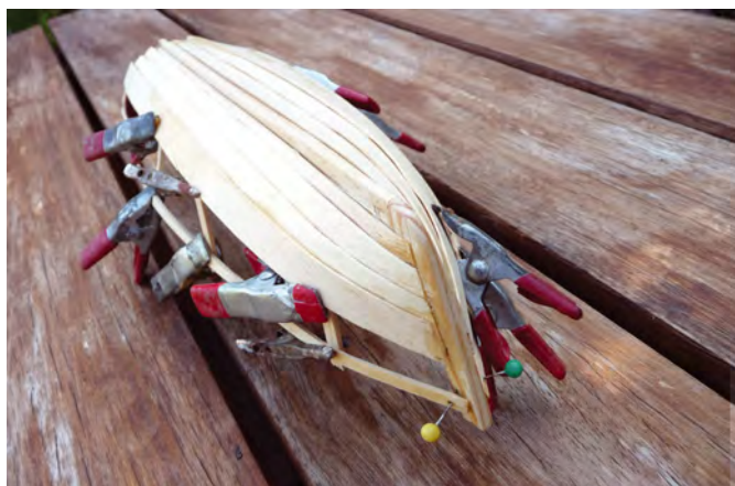
Fitting hull planking
