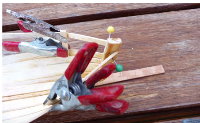
Clamping planks onto stem
