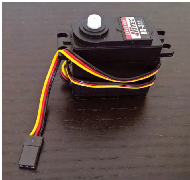
Keep all your servo plugs clean with switch cleaner (see text)
