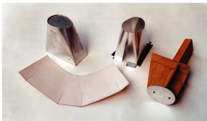
Method of manufacturing of the base of the funnel of the battleship 'Caio Duilio'
