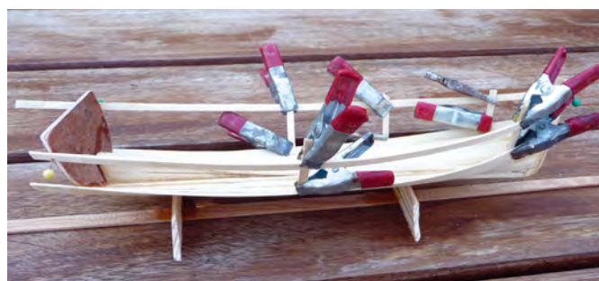
Stringers clamped in place
