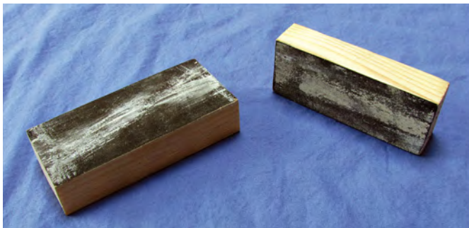
Sanding blocks are always useful. Here we are using simple blocks of wood covered with double-sided adhesive and a thickness of sandpaper
