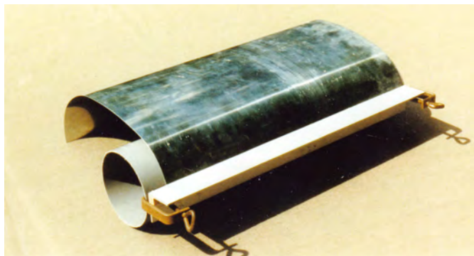
Bending of the central cylindrical part of the submarine UB-4
