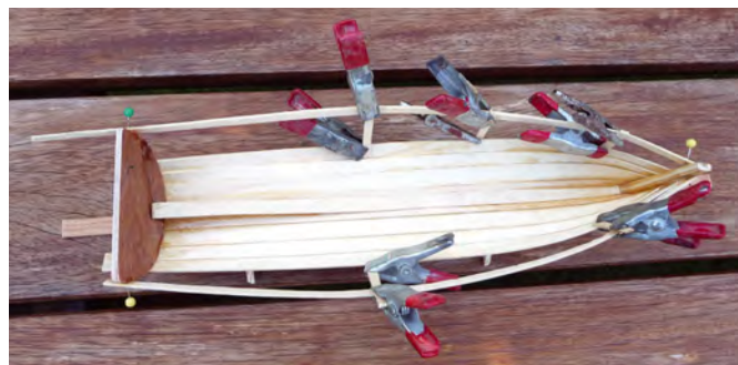
Frame and first planks
