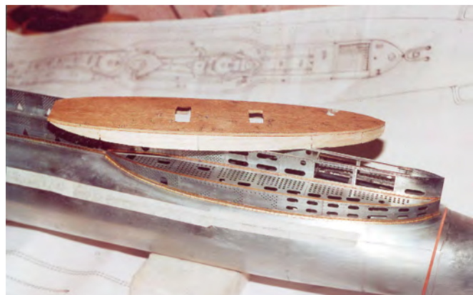
The superstructure of a submarine made using the wooden template
