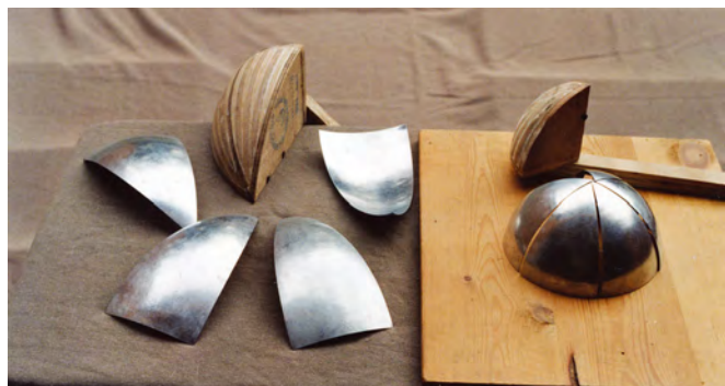
The bow and the stern of the Fulton Nautilus, the pointed cap is made up from six triangular zinc segments, hammered on hardwood jigs to give them the appropriate concave and convex shape. Then it is all soldered together
