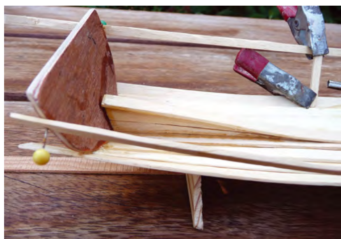
Fitting the transom
