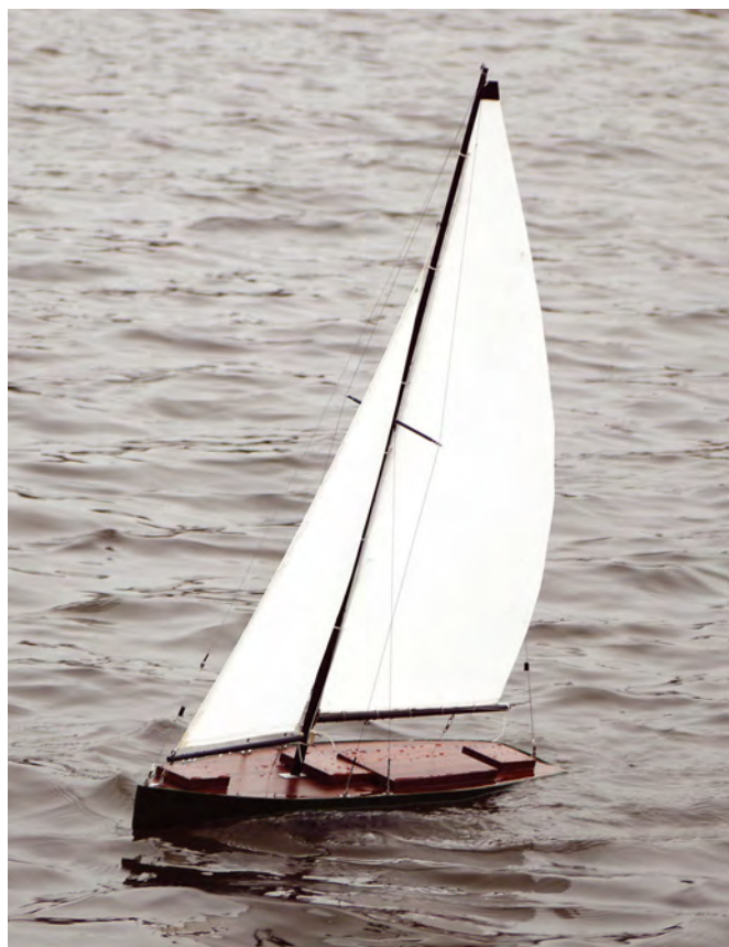
The MMI 'Starlight' built from the plans by John Kingsley of the Cwmbran club. The hull is GRP built from a plug made from the original wooden design. The mast is also shortened to fit into the car
