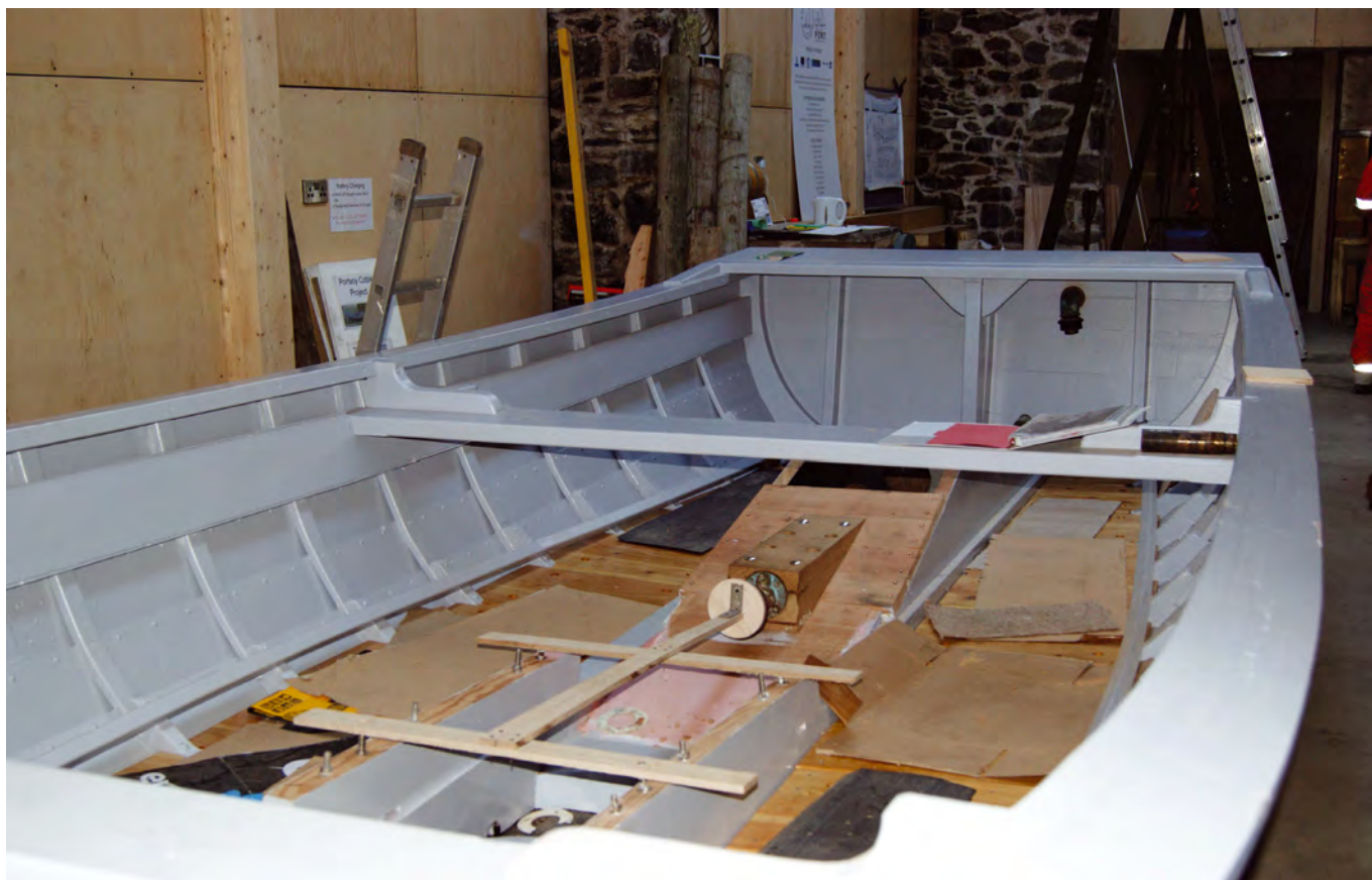
Stern of the new coble, with the engine template in place to check the engine bed heights. The rise of the tunnel is plain to see
