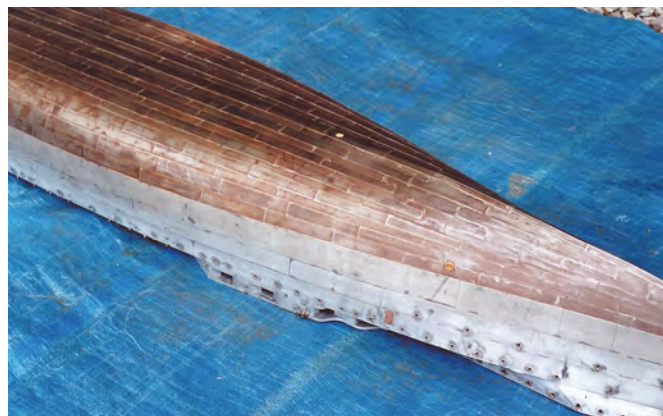
The mixed use of zinc and tin may result in significant rusting if used to construct an operational ship's hull
