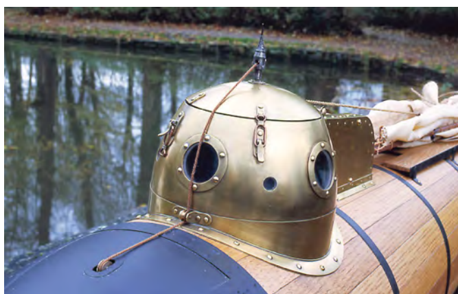
Here is a magnificent achievement in the shaping of metal. The conning tower of Fulton's 'Nautilus' is made in 0.3 mm brass
