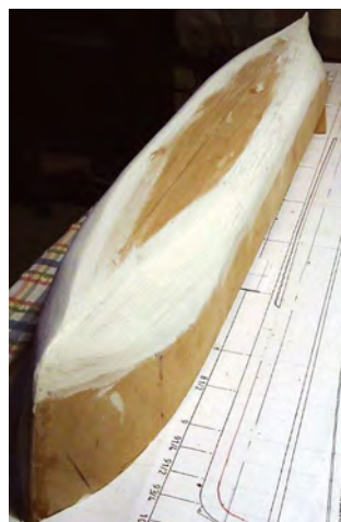
Finishing coat of emulsion
