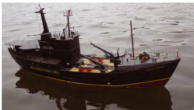
The Farley Mowat owned and rebuilt by Jason Bengie. The hull is an adapted GRP trawler hull with a single screw driven by a hydraulic pump motor
