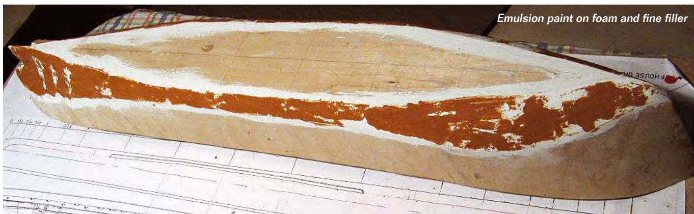
View of foam infill inside hull
