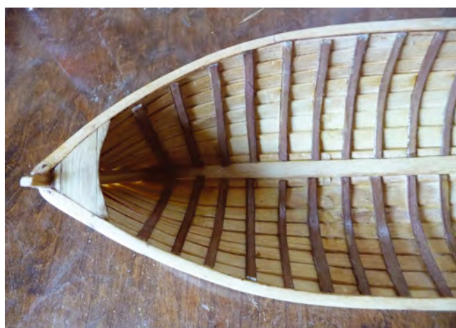
Bow construction showing ribs and hog
