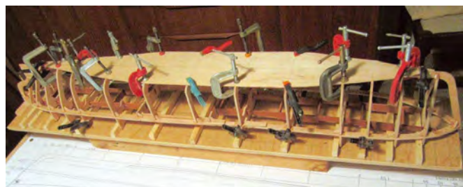
Gluing ply bottom to frames
