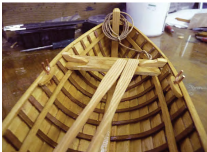
Bow view showing clinker construction
