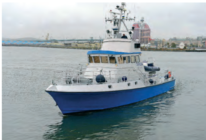
Closer view of port side, the port engine exhaust outlet at the waterline aft, also a distinct break in the chine at the junction of upper and lower shell plates
