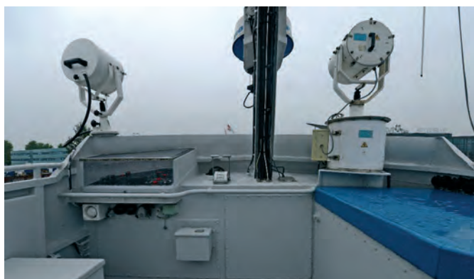
Upper fly bridge with duplicate engine instrumentation under clear shelter panel and dual searchlights
