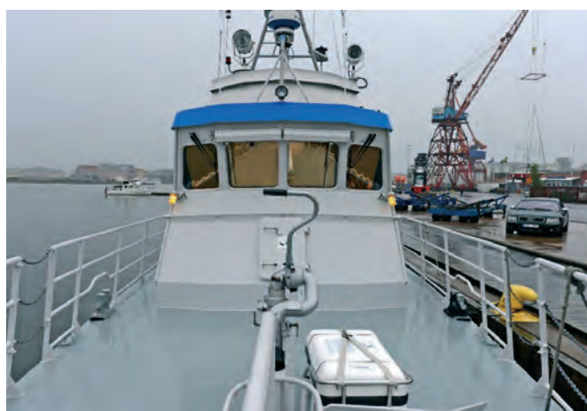
Fore deck and view of wheelhouse front, also a water cannon and life raft
