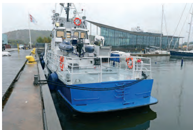
Close-up view of stern, this shows the hatch with low coaming and circular escape hatch on after deck, the large vent intake is shown on the plan
