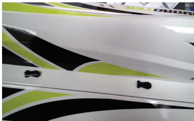
Turn tabs used to seal the hatch with the main hull
