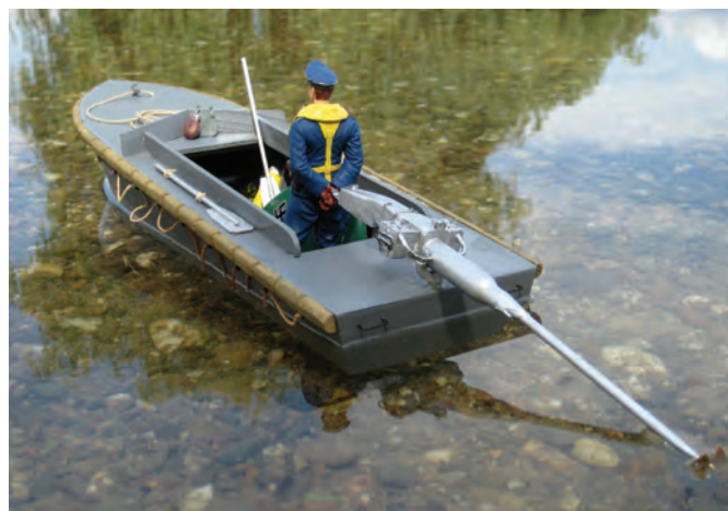
The Kovacs-engine sports a long tail. If you've ever been to Southeast Asia, you realise where the idea of long tail boats stemmed from!
