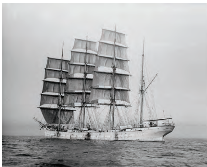
The sheer size of a big Cape Horn is apparent from this picture. The yards are squared, for a fair wind, though there isn't much of it at the moment
