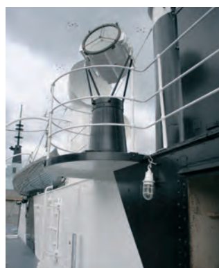
Searchlight which could be moved on rails
