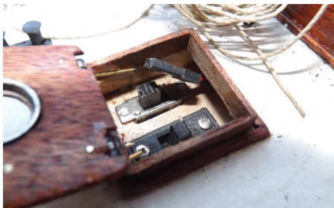
Switches and charging access under forehatch
