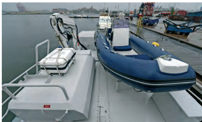
Engine raised casing with RIB stowage, the large casing on starboard side could possibly be a vent
