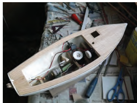
Decked with planking laid
