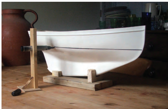
Marking waterline for ballast check. Shows unmodified hull lines
