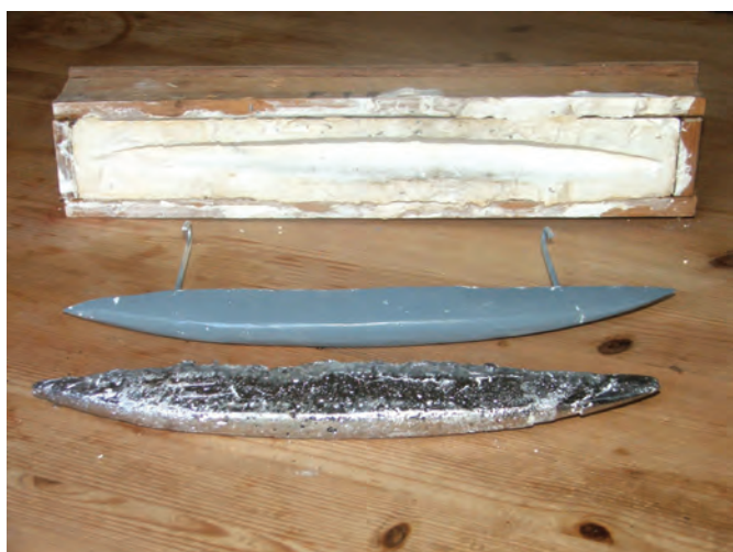
Plug mould and ballast
