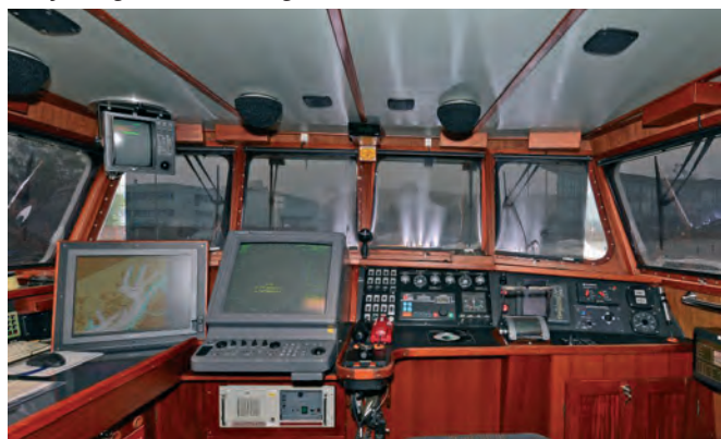
Control station at forward end of wheelhouse
