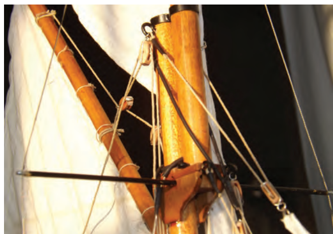
Hounds spreaders, etc. Standing rigging served and parcelled
