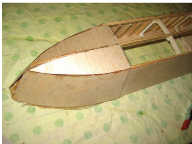
After the hull's sides are added, dummy stringers were glued in place
