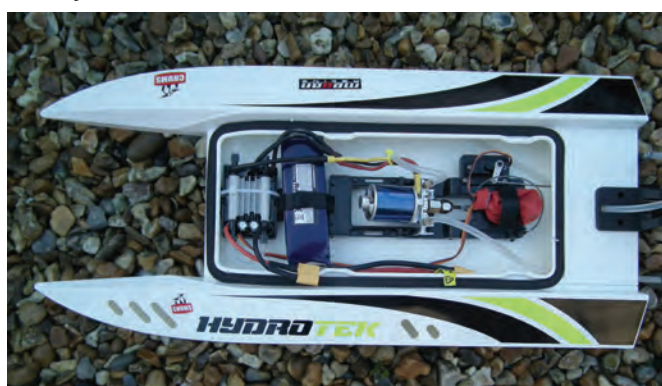
Hatch removed showing the layout of motor, ESC, receiver etc.
