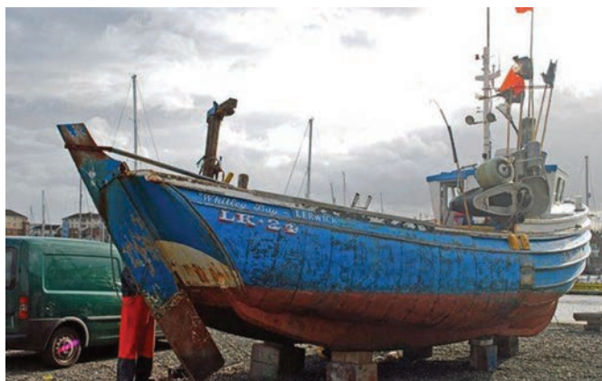
Showing the traditional, long, thin rudder. This is actually a Scottish coble
