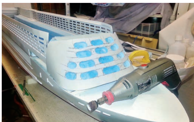
The front of the superstructure now added in polystyrene sheet (formed from a paper template) with the window apertures now removed with a cylinder rotary tool
