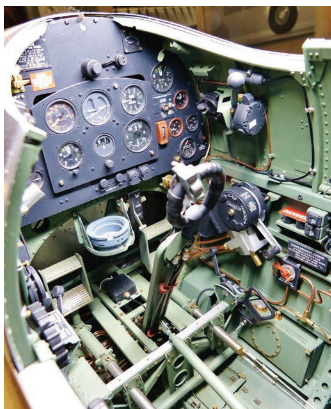
The front dashboard (minus compass) and cockpit area of David Glen's 1/5th scale Mark IX Supermarine Spitfire – a sheer modelling delight to behold
