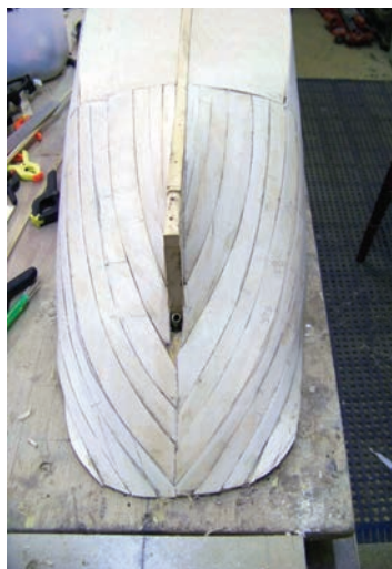
Counter stern planked showing brass rudder tube
