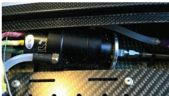
One of the SSS motors 4092, 1400 KV
