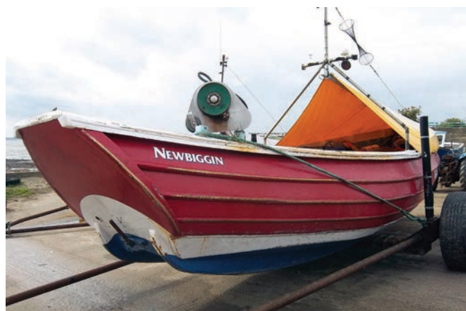
A Newbiggin (Northumberland) Coble showing the traditional transom shape
