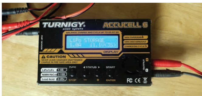
A LiPo charger ready to put a 3S battery into storage condition (half charge)
