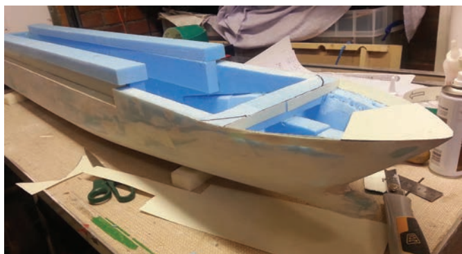
The hull now shaped and with its outer coating of glass-fibre woven cloth and epoxy resin
