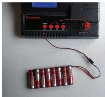
My very reliable but rather old Graupner Ultramat 17 charging a NiMH battery using an adapter lead
