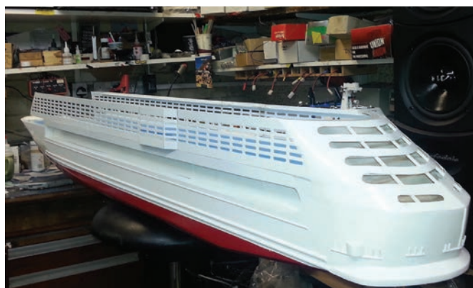
The stern and sides of the superstructure finished, sanded and painted
