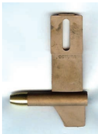
Octura BeCu strut (see text) the little fin can be sawn off for hydro use
