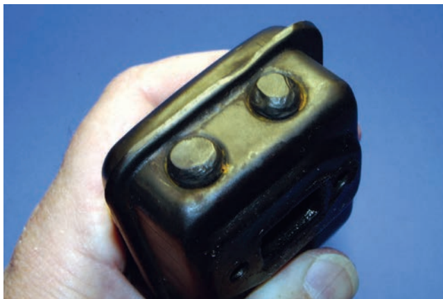
As it came from stock, this can muffler had twin exhaust tubes, but, both were plugged/welded to make it suited to R/C boat usage
