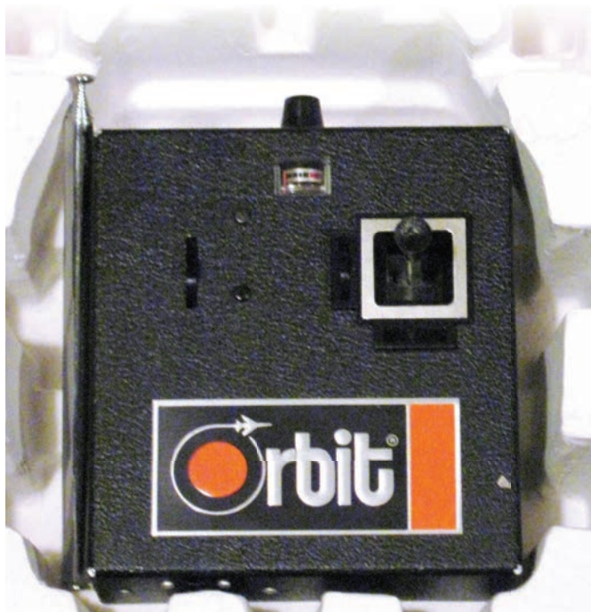
The late 1970s Orbit 'Compact' 3-ch transmitter
