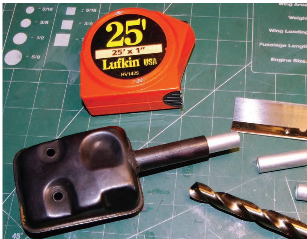
Cut to several different lengths, this 1/2 inch diameter aluminium tube fits inside the muffler exit tube and is used to help the gases exit the boat and/or help the engine's power curve
