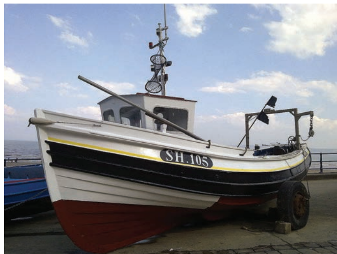
A more modern coble with forward wheelhouse and gantry for line hauler (Photo Nigel Coates)
