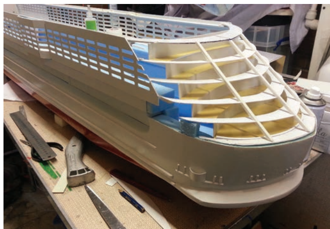
The stern wheelhouse profile being added (again from paper templates) in polystyrene and some hull detail too
