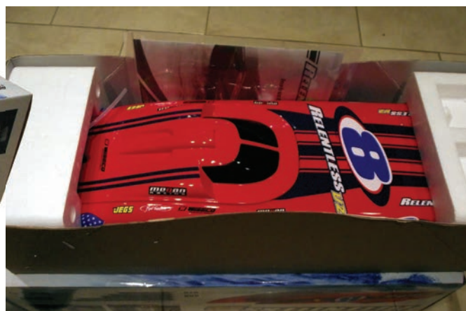
The expanded polystyrene blocks at bow and stern protect the boat and hold stand and other parts
