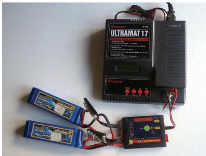
As these 4S LiPos are run as a pair a separate balancer is needed to check all 8 cells during charging
