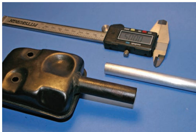
The yard tool engine muffler used on some gas boats can be tweaked to help flow the exhaust gasses by adding a tube extension made on your workbench
