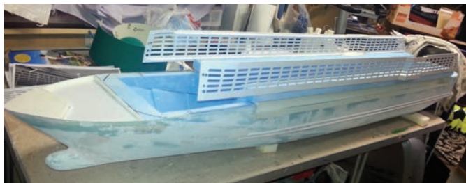
The port and starboard windows added, fabricated from aluminium radiator grilles
