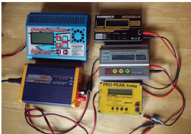
Various chargers capable of charging lead acid, NiCad, NiMH and LiPo batteries
