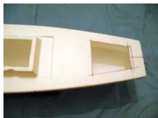
This is the extra hatch cut to gain access to the rudder which is not shown on the boat but I think is necessary
