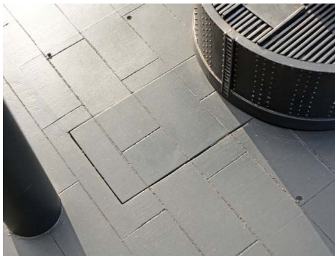
A small hatch above the motor compartment is normally sealed, but can be opened for repairs
