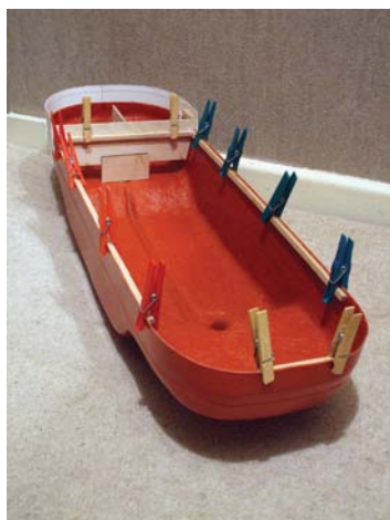
Fo'c'sle bulkhead and deck supports being installed
