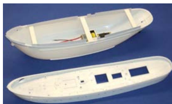
Both sections bracing and strips of plasticard fitted to allow upper section to line up correctly
