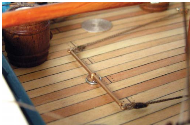
Detailed view of the steering mechanism at the stern. Note the details of the deck planking
