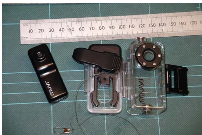
The miniature camera, and its waterproof box. The ruler will give you the scale
