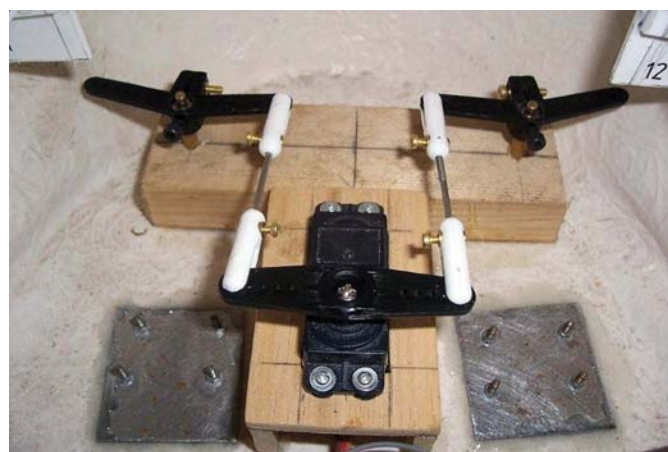
Twin rudder closed loop system. Note the adjustable nylon clevises
