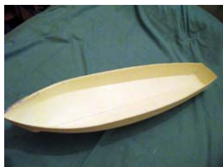
Hull finished and finally sanded to the correct size
