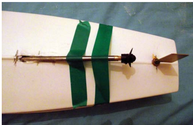
Propeller shaft fitted and glued in place held by tape until dry
