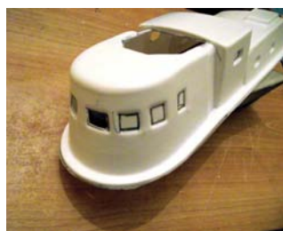
Here the windows have been marked undersize and are cut out roughly to be finished later
