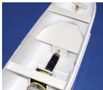
Cover fitted over prop shaft to allow area for servo to be fixed in position
