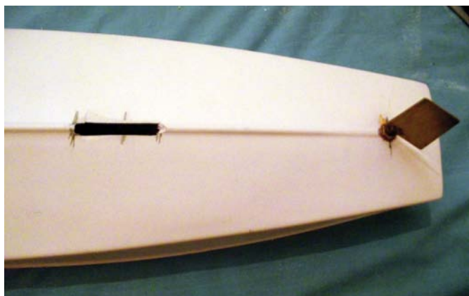
With the rudder fixed the slot was cut for the propeller shaft
