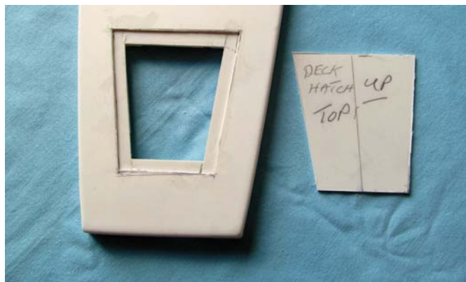
Shown is the aperture cut out and strip fitted underneath and then the filler plate can be fitted
