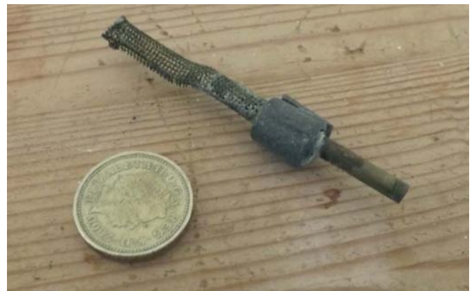
The strum box/water pick up filter
