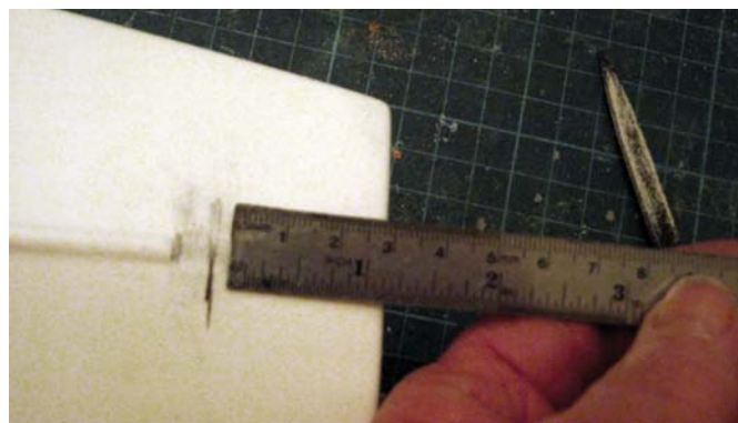
This shows me measuring the position for the rudder
