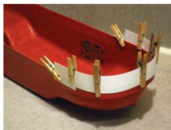
Building up the bow to give an extra deck height
