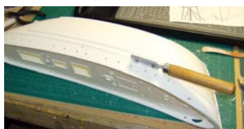
Hull and deck assembled top section being separated with razor saw
