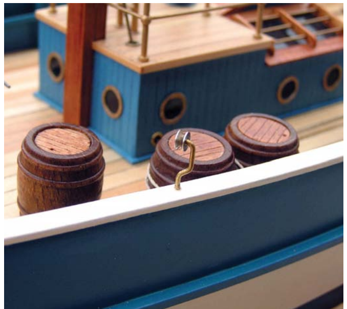
The sheet pulley installed on the bulwark
