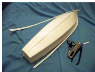
Here we see the hull partially cut and left rough ready when finished ready to sand
