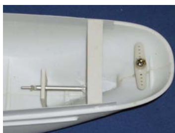
Prop shaft and rudder shaft in place
