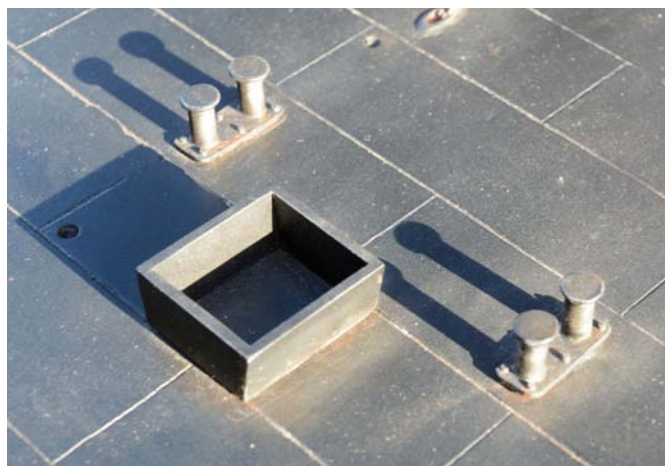
The hatches on the real Monitors were protected by walled structures to prevent water getting into the hull
