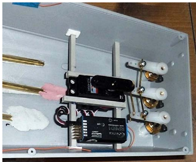
Triple rudder system using 'Z' bends and EZ connectors. Note short pushrods
