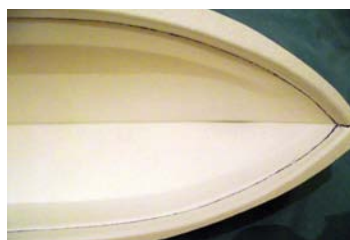
Here I have checked where to cut the hull and marked with a pen to avoid mistakes
