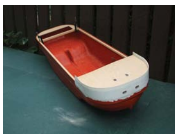
Fo'c'sle deck with anchor hawse pipes and quarterdeck with access to tiller arms
