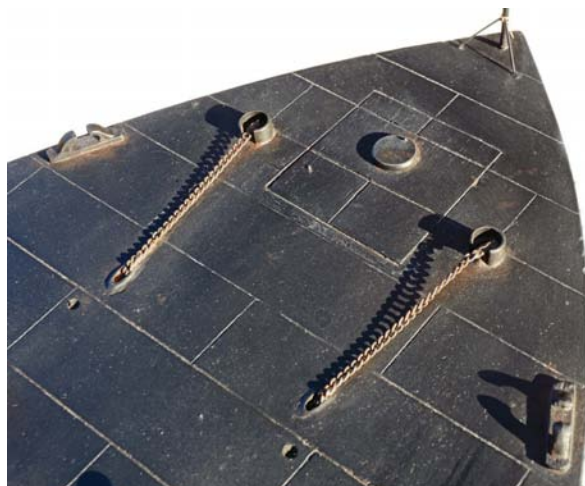
Here we see the small service hatch above the steering arms
