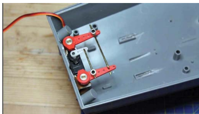
Twin rudder system using a servo with a single arm, using 'Z' bends and EZ connectors. This is a very compact system in a plastic kit
