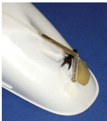
Handmade rudder and strengthening bar fitted
