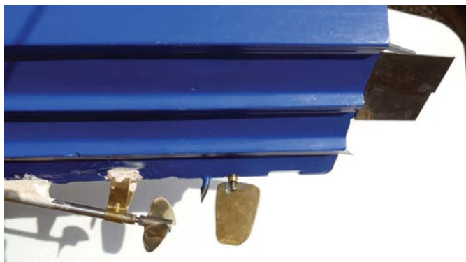
Having done some work on the prop shaft I had failed to notice that the solder joint on the rudder had clearly failed
