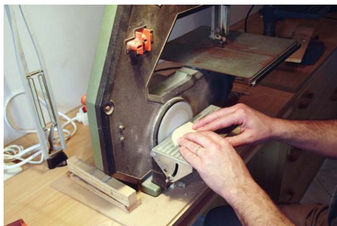
The pieces obtained by sawing are adjusted using a fixed sander
