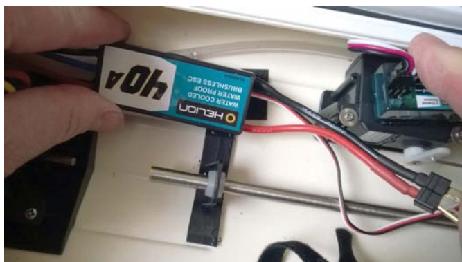
Installing the new ESC
