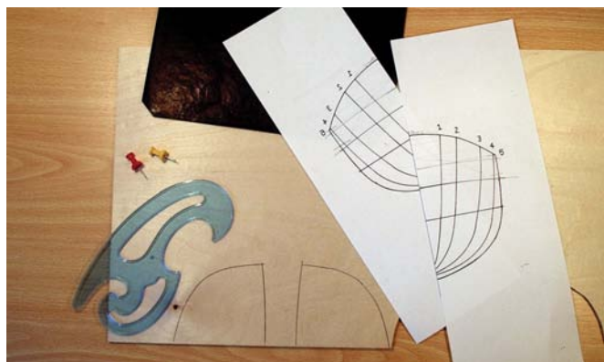
The bulkheads were copied using a sheet of carbon paper. The accuracy of their shapes was ensured by the use of a French curve, a ruler and a sharp pencil
