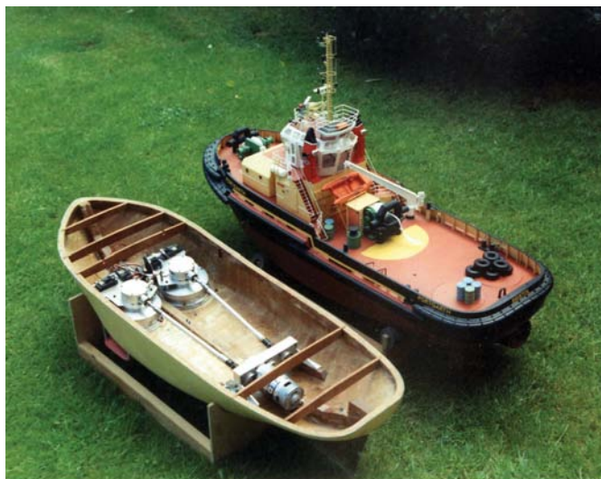
The VSPs fitted in the hull of Kevin's Tees Tractor Tug
