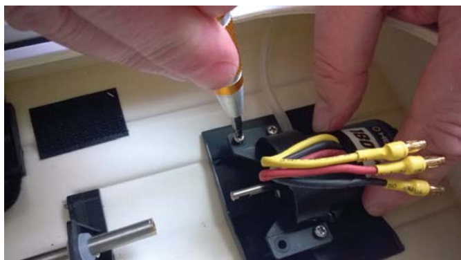
Fitting the new motor (see text)
