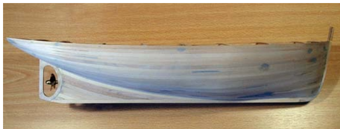
Then the other side of the keel was covered. Because of the thinness of the planks, it was decided not to over sand the hull so the occasional use of mastic was needed. This was a problem as the hull was to be painted
