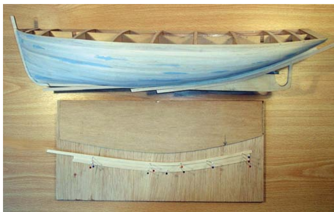
The planks were glued on the keel. Subsequently, the appropriate shape was cut for the installation of the propeller shaft and the bottom of the keel
