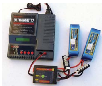
My old reliable Ultramat 17 requires an additional balancer to charge the 8 cells needed for my fast electric. Charging takes place in a fireproof box for safety
