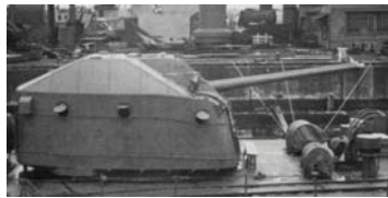
No.4 twin dual-purpose 100 mm gun-house aft onboard Hatsutsuki, revealing the potential to detail these four prominent mounts, through 'opening-up' the three side ventilation ports as shown in this view (IJN Department of Naval Aeronautics)
