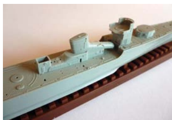
Close-up amidships, the non-slip texturing to the central portion and linoleum strips forward (and aft) is clearly shown on the decks
