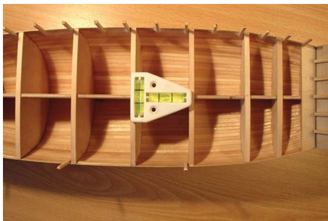
A spirit level was used to accurately align the model before constructing the bulwarks
