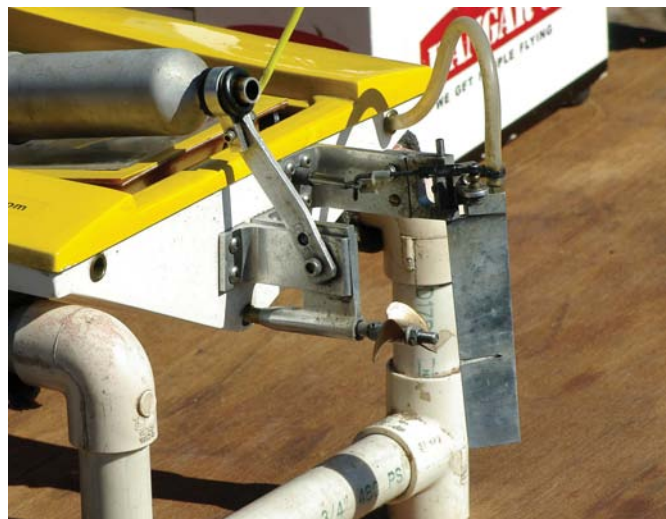
Making your own transom/exhaust hardware components makes it easier to mount them on limited-space transoms, as will using locking fasteners
