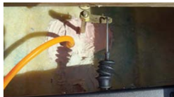
A close inspection of the steering linkage and sealing boot is important
