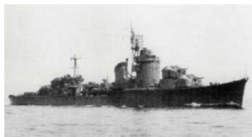
Another class member, Fuyuzuki in May 1944, possessing a Type 21 mattress radar array atop her enlarged foremast and Type 13 aft, along with an enhanced 25 mm battery (IJN Department of Naval Aeronautics)
