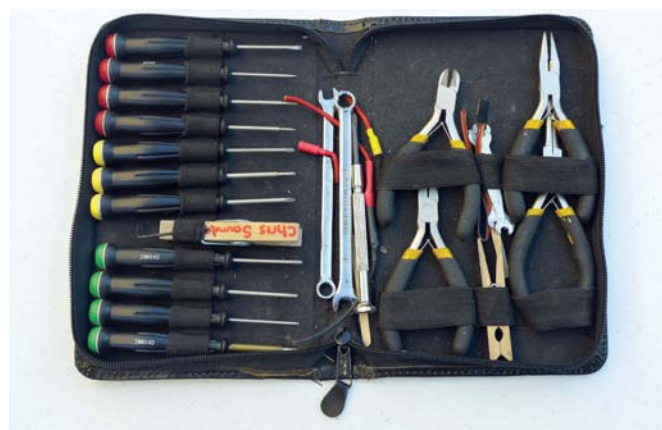
My lake-side toolkit with the very useful 7 mm and 8 mm spanners (for 4M and 5M nuts respectively)
