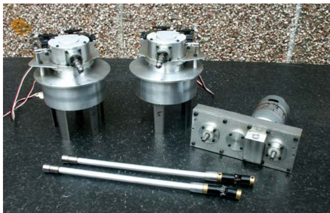
Kevin Fleet's home built VSPs with gearbox and drive shafts
