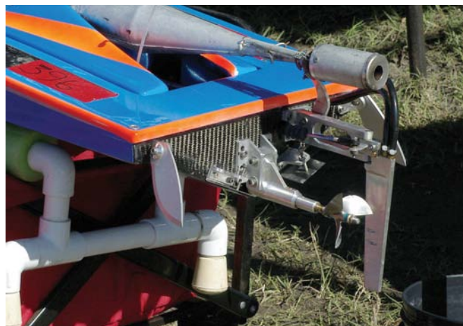
With minimal transom space some extra effort done while mounting the rudder, drive strut, etc. will prevent loose/lost fasteners at the lake
