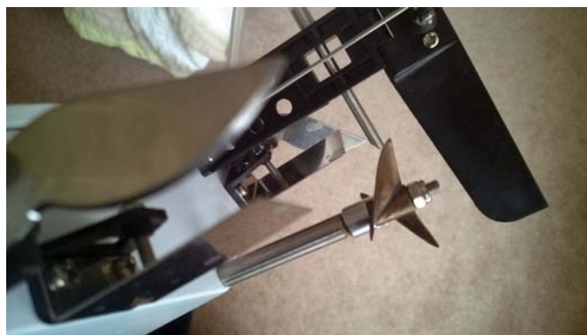
The Octura prop on the boat. This also shows the trim tabs angled up slightly as mentioned in the first part of this review
