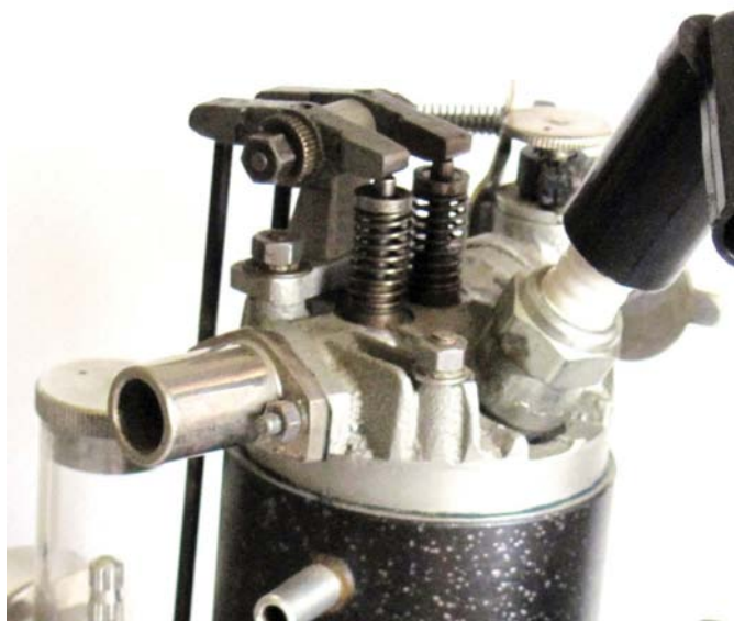
The GAN 'top-end' showing exhaust stub, rockers and needle
