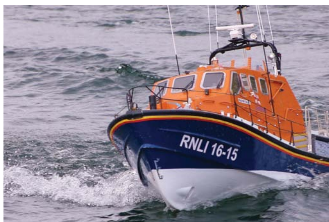
Out on a shout! Mike Gunn's 1/12th scale Tamar class lifeboat 16-15 RNLB Enid Collett, based on the Shoreham Harbour, Sussex lifeboat, exposing her bow thruster. This had great LED deck lighting, just like the real boat
