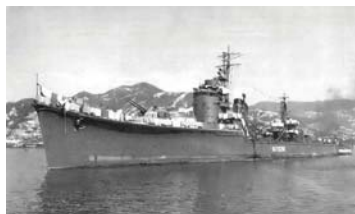
Natsuzuki post-war, of interest here has to be the plated-over hull portholes, the track of her girdling degaussing cable, breastworks outboard of the single 25 mm battery, and Type 13 'ladder' radars to both masts, with Type 22 'horns' atop her bridge (IJN Department of Naval Aeronautics)
