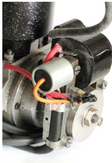
The more expensive magneto Gannet modified for battery ignition
