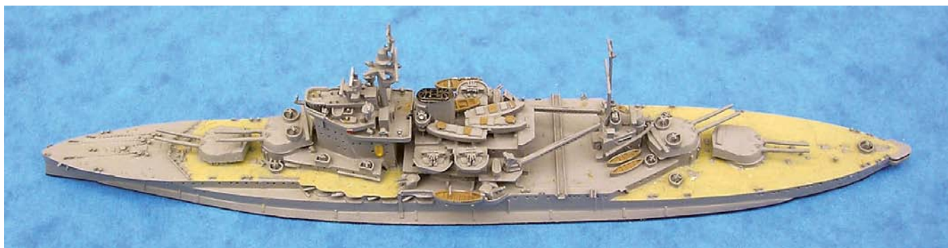
Neptun HMS Warspite with amidships catapault with eight 4" guns and 6" guns
