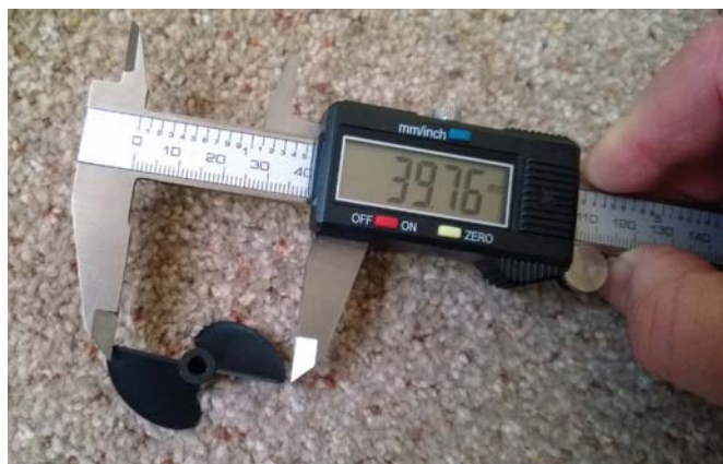
(Almost) 40 mm diameter prop (see text)
