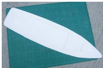
GRP deck prior to cutting out the hatches and cockpit well
