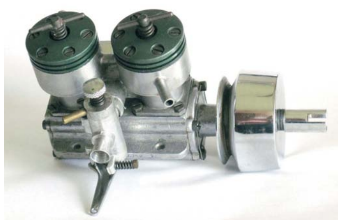
A 1959 Mk.1 Taplin-Twin 'green head' fitted with the first ball coupling
