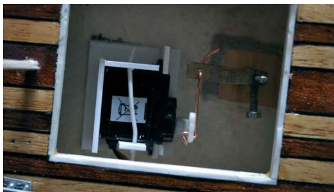
Steering servo with rudder linkage using universal pushrod (2.5 mm copper electrical wire)
