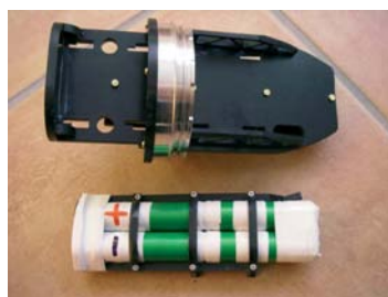
Support for the batteries and the base plate still empty, but fitted with the closure system
