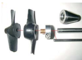
An exploded view of the counter-rotating propellers
