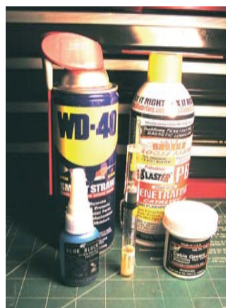
Lubricants in mini oilers, spray and bottle forms are commonplace for I/C toolboxes to service/repair any fastener/rotating component on the marine craft
