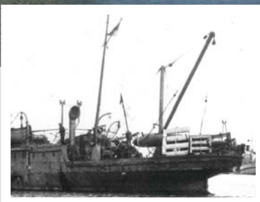
Modeller's detail – minesweeping gear on HMS Medway Queen (PSPS Collection)
