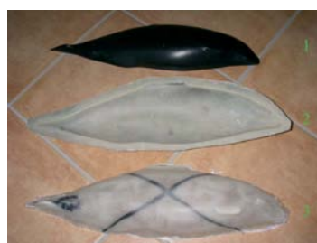
From the top down: half a porpoise in Orinol (1) used to make a negative mould in GRP (2) and the positive part obtained, also in GRP (3). You can see the reinforcing tapes of carbon fibre in (3)
