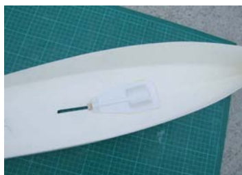
ABS hull with motor mount fitted
