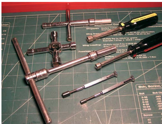
Special jobs can require special tools like forceps for holding fuel lines, T-handles for loosening engine screws and mini drivers to tweak small carb screws or strut brackets
