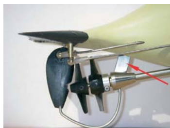
The propulsion and steering. The power of the machine is such that the central axle of the contra-rotating propeller system, broke as a result of vibration; an additional bearing, installed at the furthest point of the propeller tubes, solved the problem, marked with an arrow
