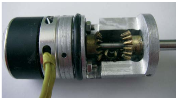
A bevel gear system for contra-rotating the propellers was tried at first, but it overheated too much
