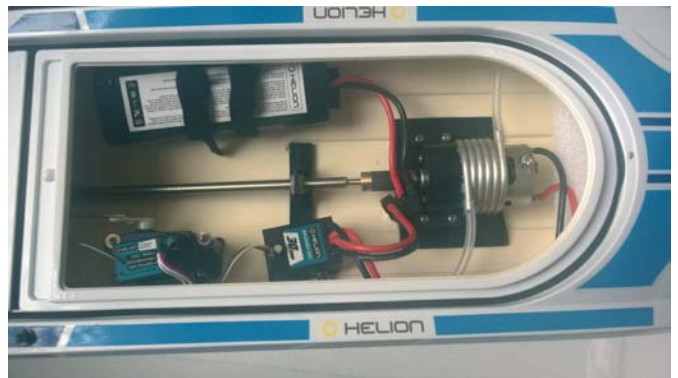
The interior of the boat as supplied, but with the battery fitted
