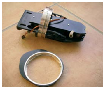
The bayonet locking system
