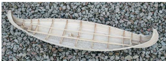
The plank on frame construction can be seen here but the many internal bulkheads might make it tricky to convert to R/C?
