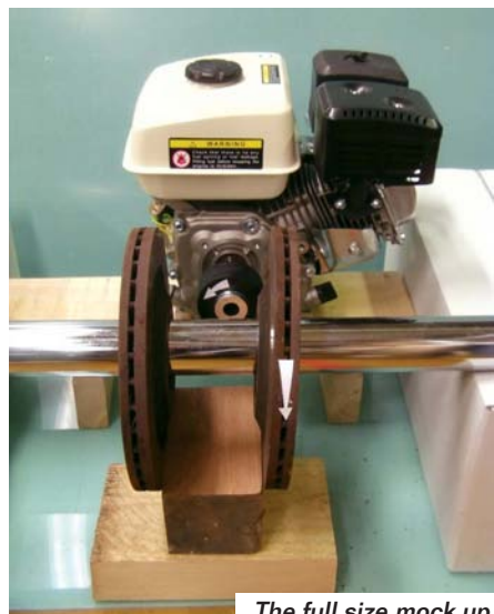
The full size mock up, with arrows indicating the various rotary motions achieved by friction
