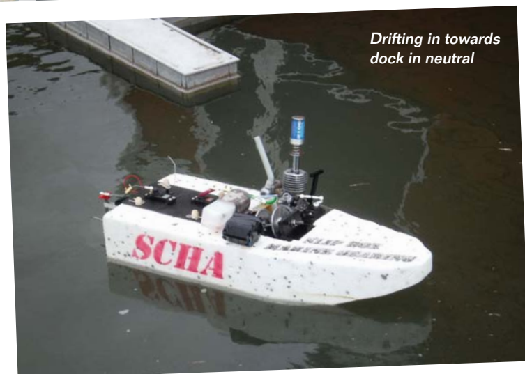
The wash from the prop in astern hits the transom virtually dispersing the thrust. We will have to redesign this
