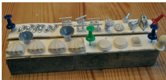
Most of the fittings mounted on a block prior to spraying
