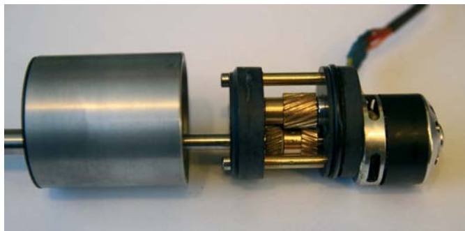
In the end, a set of helical gears were the solution
