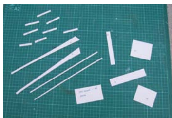
Parts cut out from the pre-printed sheet of plasticard
