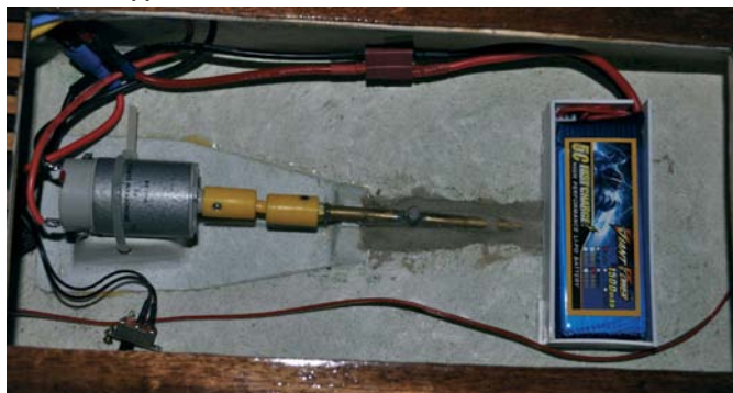
Motor, coupling and battery box now fitted
