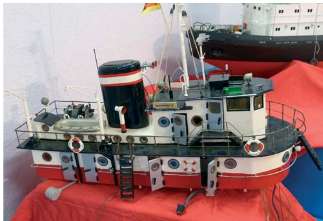
The wheelhouse of tug Hamburg II – note the umbilical wiring leads for its electrics and lighting
