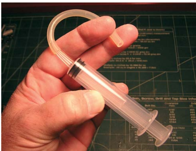
By simply adding a short section of silicone tubing to this syringe you can get into tight spaces with whatever glue you need to bond your hull parts together
