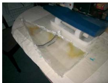
Hull base external mould
