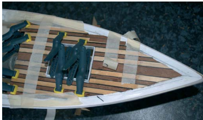
Plenty of clamps and masking tape required for holding the planking in place while the adhesive is setting
