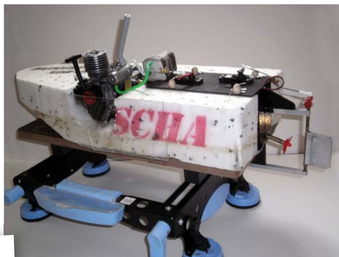
The wash from the prop in astern hits the transom virtually dispersing the thrust. We will have to redesign this
