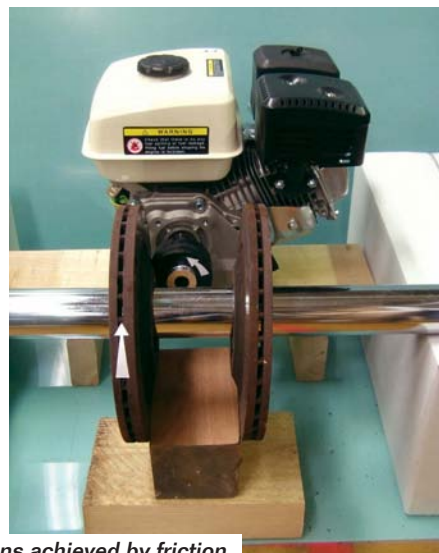
The full size mock up, with arrows indicating the various rotary motions achieved by friction
