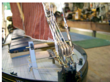
Cleats for downhauls on the bits for the massive anchor winch
