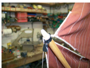
Outer end of sprit. Fitting to take the vangs and topsail outhaul. Mainsail has a loop sewn in that drops over the upper end of sprit
