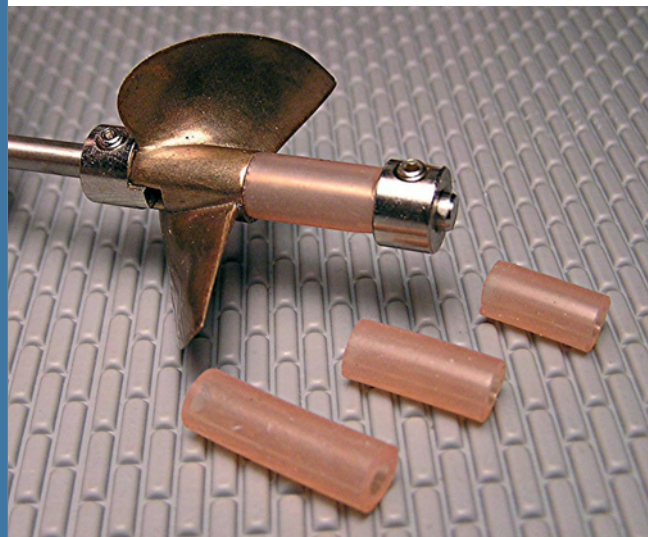
Besides being useful as nitro boat fuel hose regular silicone tubing, cut in small lengths makes an excellent bumper to help the propeller survive any contact with floating debris
