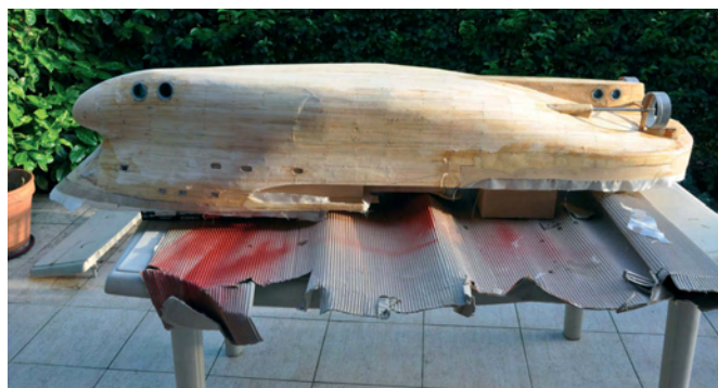
Covering the hull with glass fabric and epoxy resin
