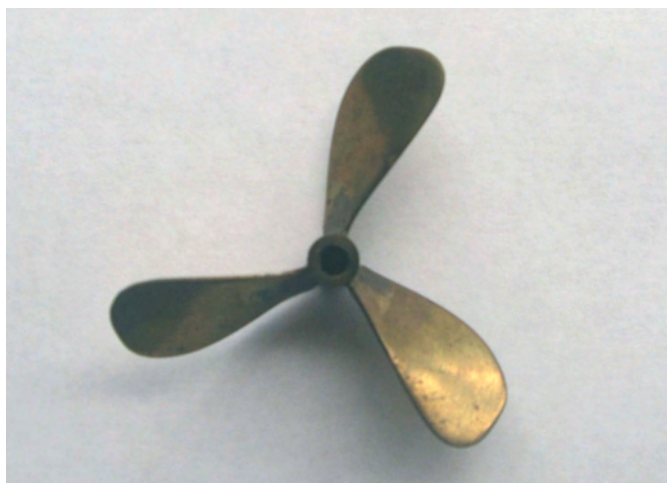
Handmade prop using the method outlined in the text, the blade roots aren't actually as thin as they appear in this photo
