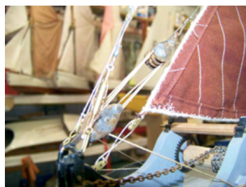
The stemhead was a busy place: the three-part tackle that hoisted the mast up, the jib downhaul, topmast forestay and staysail downhaul
