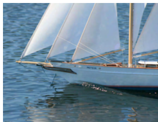
Meteor – Clipper bow with fine entry
