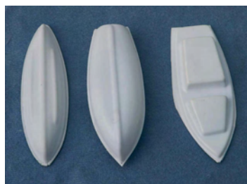
Vac-formed parts to make the ship's boats
