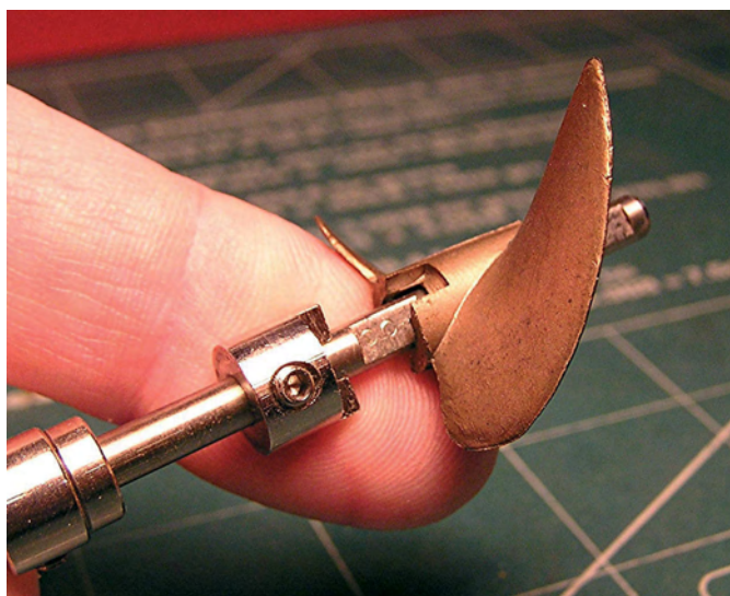
Normally held to the driveshaft by grub screws, the drive dog's dual tabs must solidly lock into your prop's matching slots to prevent any slippage under a strong engine load
