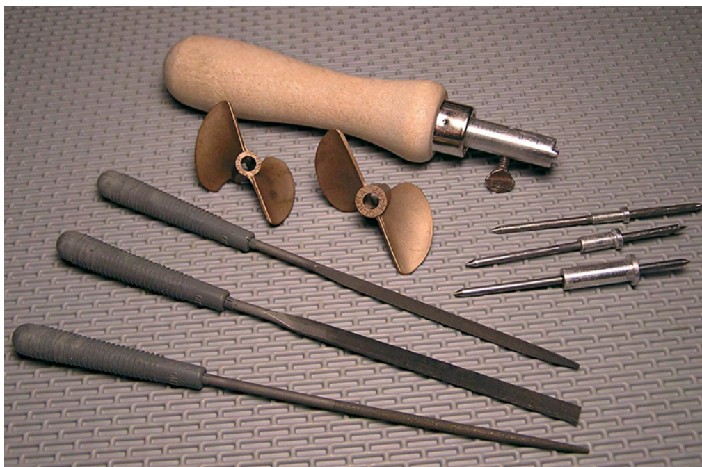
Using only some small files, wet/dry or emery paper and a balancer unit you can alter any metal propeller and add it to your blade collection as needed
