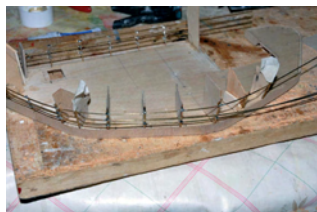
The rail formed using templates
