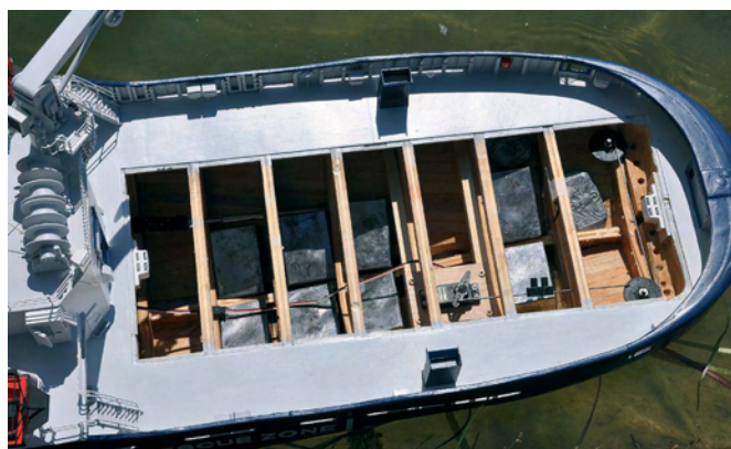
The distribution of ballast, at the rear of the hull
