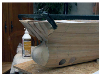
Wooden blocks showing the techniques used to shape the bow
