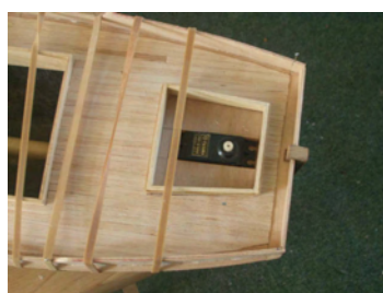
Rudder servo installed
