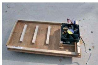
The board made to accommodate four batteries and a variable speed fan from a PC
