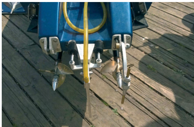
Overhead view of rudder and props. Note how close together they are (see text)
