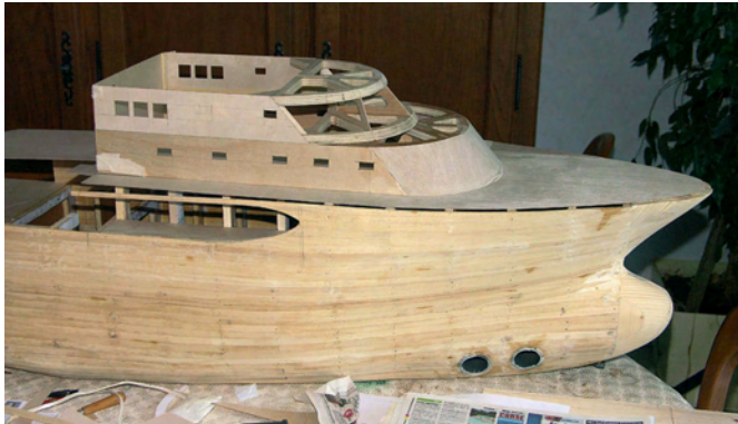
Starting assembly of plywood superstructures
