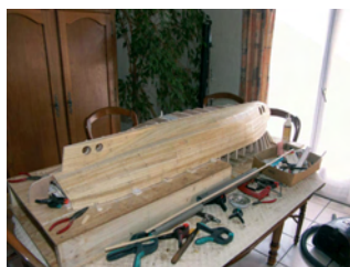
The four holes for the thrusters are made. The model is worked on upside-down
