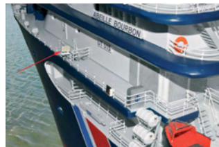
The port side which contains the lateral docking support, marked with an arrow
