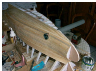
A hole saw, attached to a PVC tube of the same internal diameter as the thruster propellers, was used to cut the thruster holes
