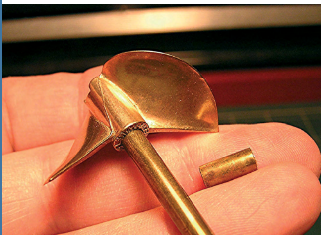
For those instances where you might need to re-size or re-bore a metal prop's centre hub hole a short section of brass tubing can create a tight fit on your boat's shaft end
