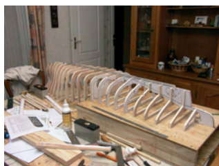
The frames for the hull have already been positioned across the model
