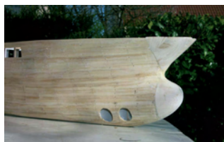
The bow blocks fully shaped
