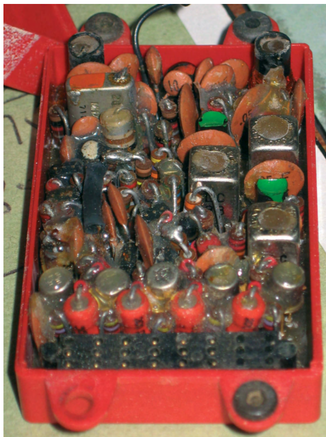
A matching receiver. It's a discrete, single conversion Superhet' with an early SCS (silicone controlled switch) decoder. Note how tightly wedged in the components had to be before I/C's came along
