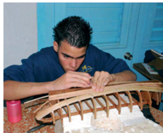
Great concentration was needed while planking the hull
