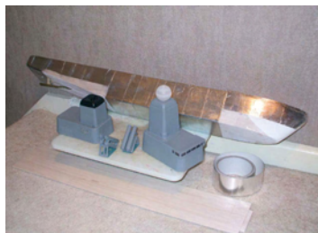
Hull being plated over with aluminium foil (optional); note also the more complicated bridge windows (see plan and text)
