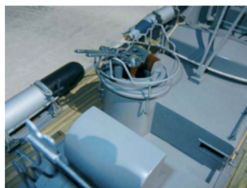
The steel tube 'cages' around the .50 calibre machine gun, depicted here, illustrates how this gun and others cannot be trained on the boat or its sailors
