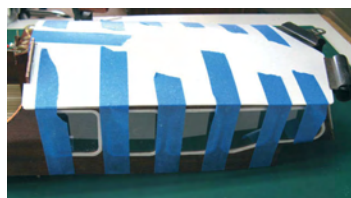
The cabin roof is glued in place
