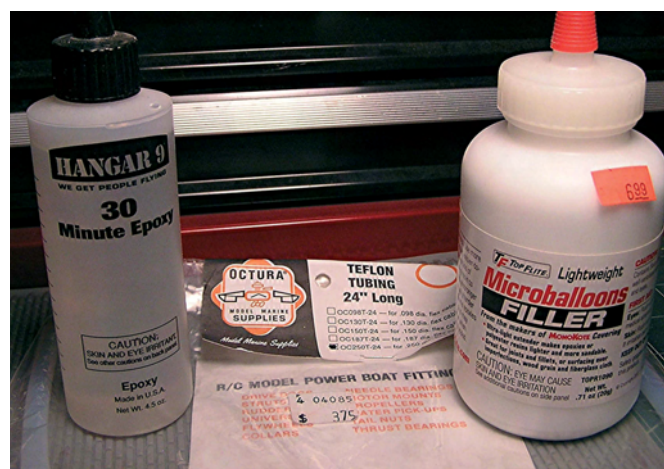
Put out by several companies, a Teflon-like stuffing tube liner material is commonly used on a majority of I/C boats; but, when building a new hull you'll need to pre-determine if you want to use a lined or unlined stuffing tube on your hull
