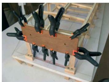
Fixing the mahogany transom in place
