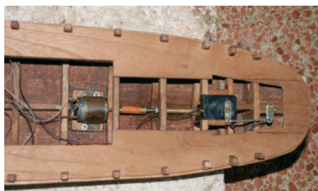
The deck in place and the steering servo installed
