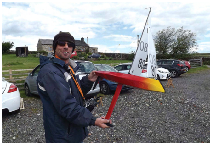
Glen Meekcom downloaded this Esterel 65 design off the Internet and built it from scratch, including the moulded carbon fin
