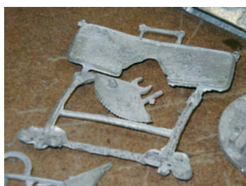
Here are a few of the Bofors 40 mm gun parts. Note the quality of castings
