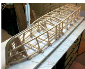
Stringers all glued into place
