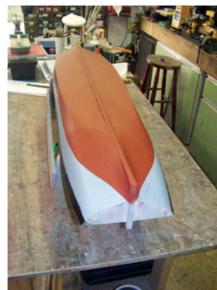
Painting the hull – stern view
