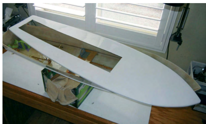
The deck component ready to be joined with the hull
