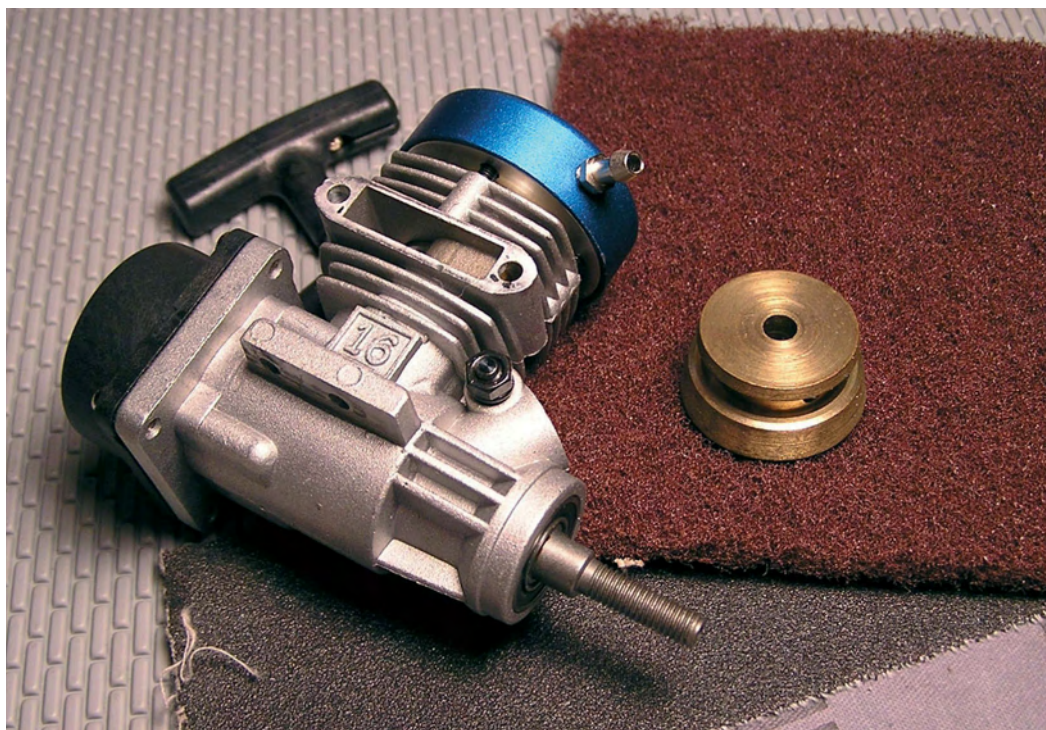
ABOVE: Using nothing more than some emery cloth or a regular kitchen pot scrubber you can add some bite to your engine's flywheel groove that will eliminate belt slip during a start-up of a high horsepower nitro power plant
