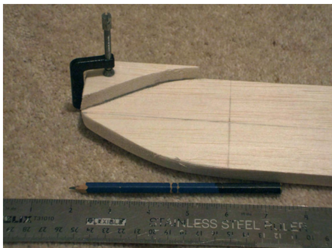
The first cut off bow section being used as a template for the other side
