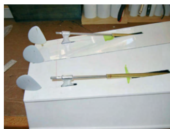
Here the drive train is ready to be secured in place with epoxy glue and fibreglass cloth
