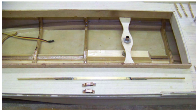
The keel tube support clearly visible with the crosstrees and leeboard rollers on deck prior to fitting
