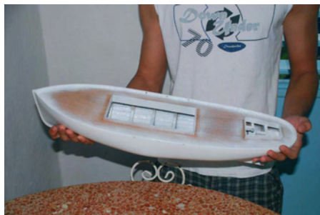
The primed hull clearly showing the hatches for accessing the drive and steering systems
