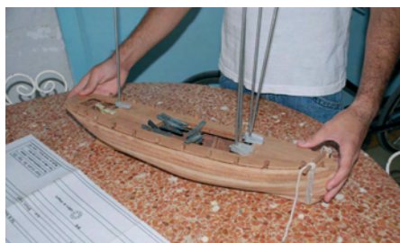
Pegs and clamps used to hold the deck in place while the glue dried
