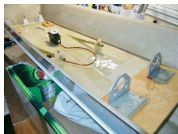
Aligned motor mounts, drive shafts, stuffing boxes and rudder posts shown secured from the inside
