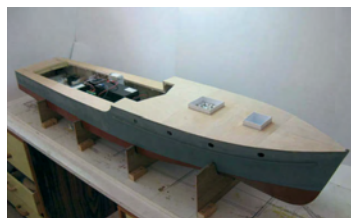
Plywood deck ready for planking
