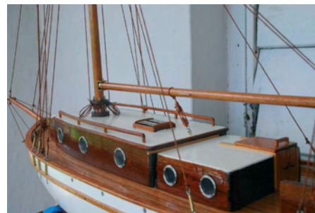
The main cabin showing the round portholes rather than the square frames on the full size boat
