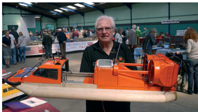
Model of the Griffon 470 SAR Hovercraft H006 (one of seven commissioned by the RNLI) built mainly from 1/64 plywood with GRP ducts by Tony Middleton of the Air, Water, Land Model Group (AWL)
