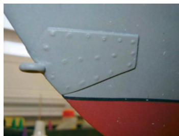
The bow tow hook was detailed with glue dot bolts/rivets
