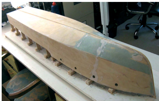
The fully plated hull, with fibreglass coating, ready to paint
