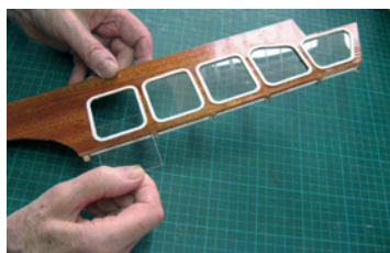
Inserting the glazing sheets
