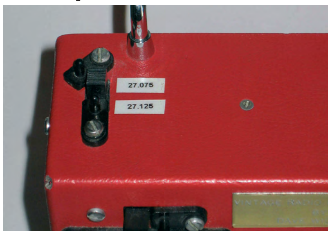
I added dual crystals to mine. This is NOT an original feature, all American radios of that era being single frequency
