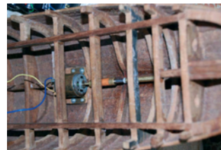
The completed planking clearly showing the frames together with the motor, prop shaft and coupling
