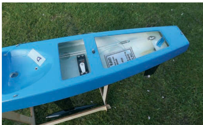
The stern of the MX Goth RG65 shows the rudder servo in position, and the pulley for the underdeck main control line
