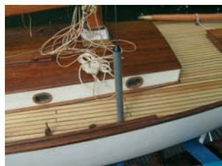
As in real life, some turnbuckles require protection using a tube filled with grease
