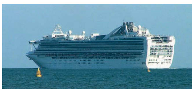
Lead ship of a class of three, Grand Princess was completed in 1998 by Fincantieri and had a 'skyway' aft as seen on Caribbean Princess. This was removed in 2011 when this picture was taken. GT is now 107,517 and normal passenger capacity 2,600 (Peter Anthony)
