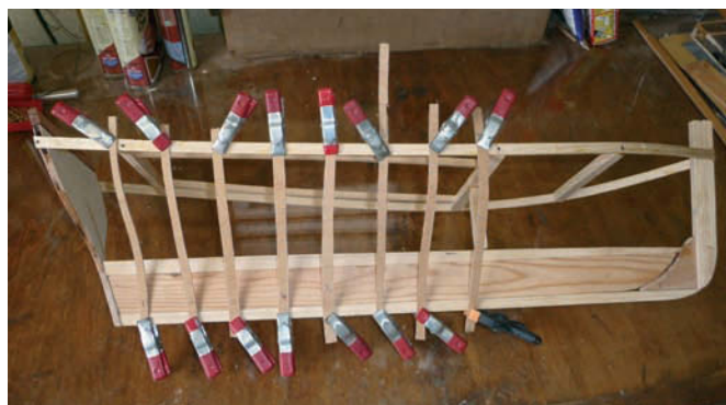
Early stages of the model Dayspring showing frames clipped to hull
