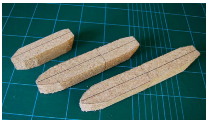
Short (11 cm), medium (18 cm) and long (22 cm) hulls carved to basic shapes
