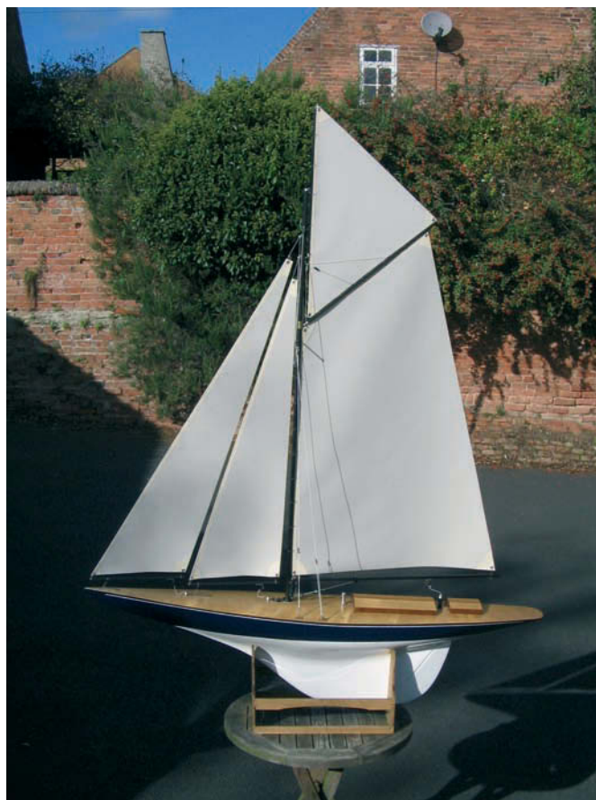
The twin foresail and gaff mainsail rig on the Nottingham J hull is the most recent variation on the standard size 48" length hull
