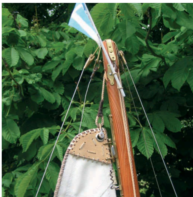
The masthead and details of the top of the mainsail
