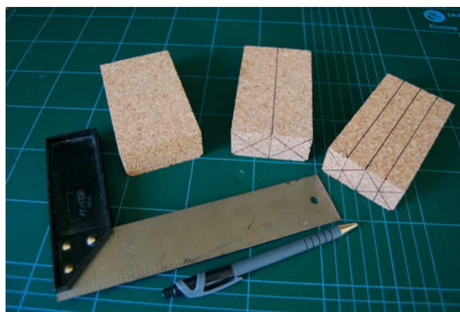
Mark out the sanding block and then draw the centre-line around each half
