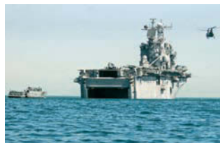
A landing craft approaches the partially flooded stern dock of USS Belleau Wood (courtesy US Navy)
