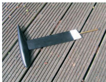
The additional keel weighing 2,700 grams
