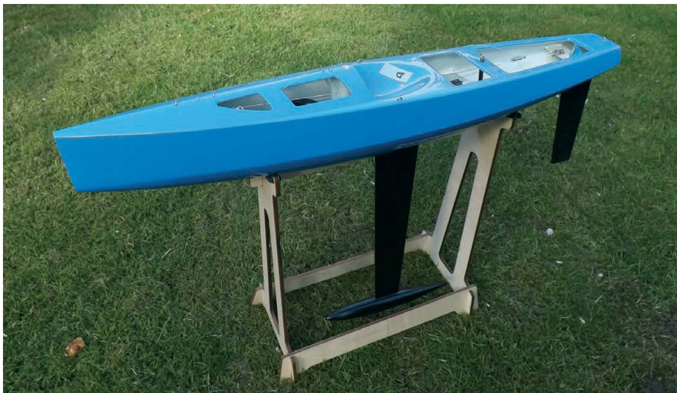
This view of the MX Goth from the bow shows the attractive and modern design of the hull, with a chine moulded into the side from about midpoint to the transom
