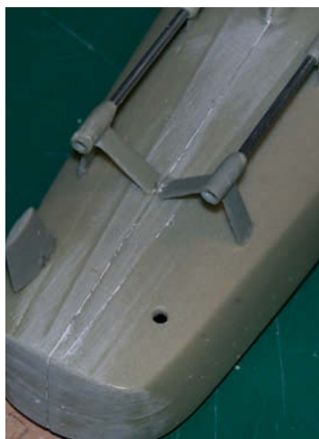
Propeller shafts and rudders being installed, note filler used along some of the hull
