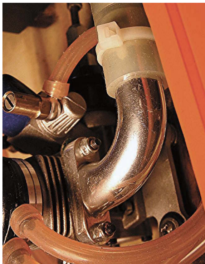
Largely done on nitro-engined boats, adding or subtracting header pipe length on the exhaust can alter the engine's power curve to a point where it gives the modeller the best package for racing or sport running conditions
