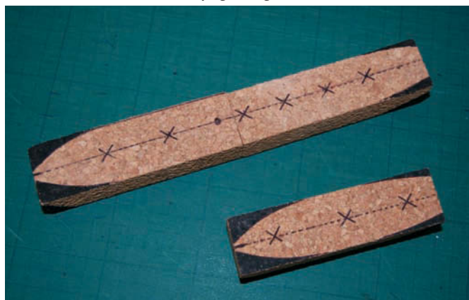
SS Great Britain and HMS Trincomalee hulls marked for cutting out and shaping
