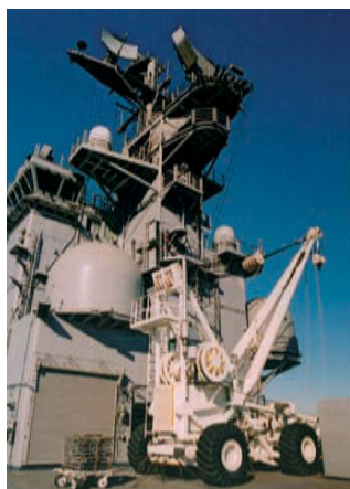
Rear of island structure: note sensors on rear mast, shutter style door and mobile crane unit
