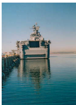
Stern gate on USS Belleau Wood lowered for hovercraft and landing craft to enter and leave
