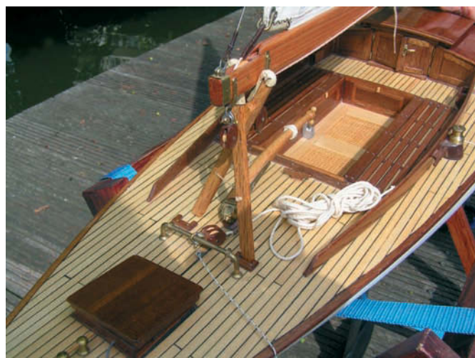
In dock an 'X' frame supports the boom
