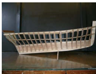
Completed frames and sheer plank
