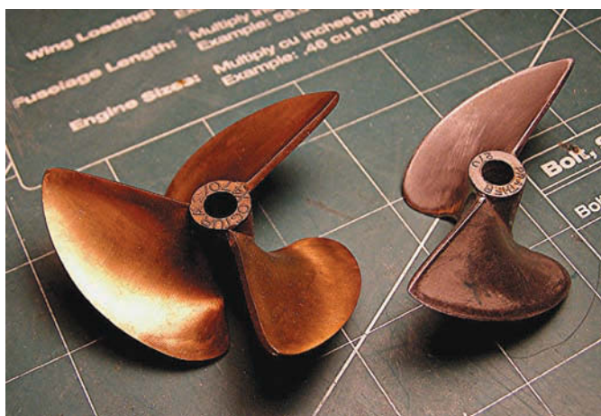
Due to hull lean from propeller torque, changing to a smaller three-bladed metal prop can help the boat run straight and smooth without showing too much torque lean as you accelerate the vessel
