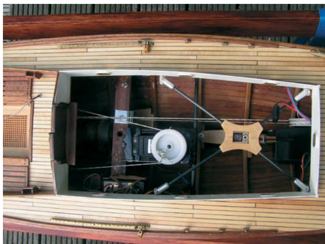
From left to right: the Genoa winch, the connection to the mast and the mainsail hoist
