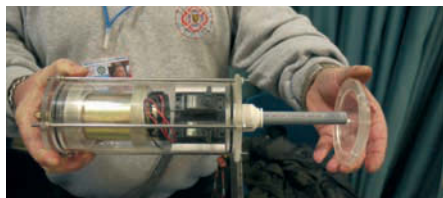
A compartmentalisation system for model submarines using 'push fit' pipe seals
