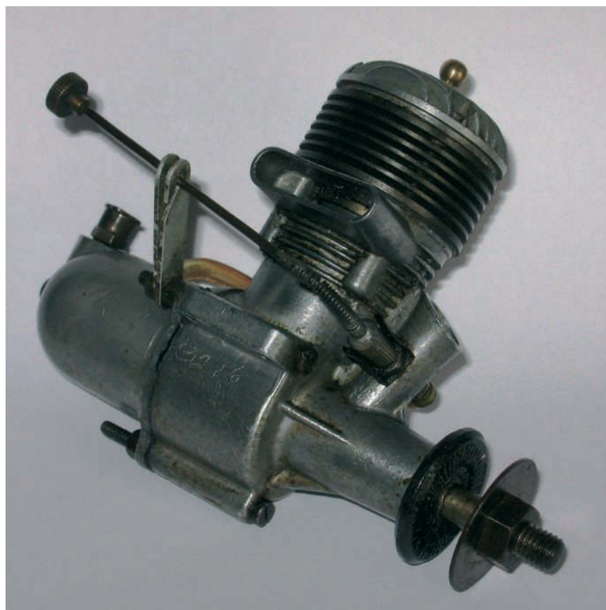
A quality built, early British glow engine – the 5 cc FROG 500. Note the nicely thought out needle valve
