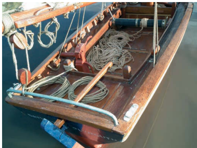
Stern view showing tiller, bilge pump and dandywink winch
