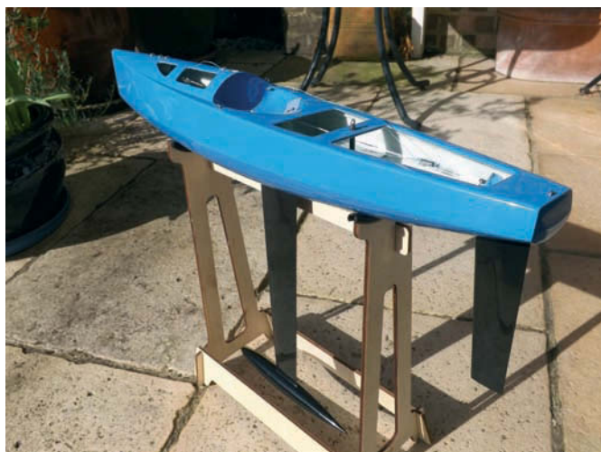
Side view of the attractive MX Goth RG65 hull. Note the deep scallop in the deck to allow the main kicker to be as low as possible
