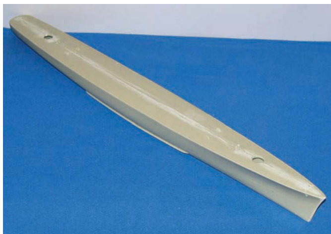
The resin hull comes in one-piece complete with deck
