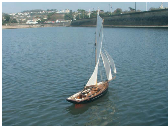
This shows the slot effect headsails correctly sheeted
