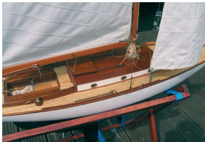
The starboard deckhouse. A Genoa is sheeted behind the mast, which is what makes it different from a jib. This sheet passes outside the shrouds of the mast. The Genoa gives better performance upwind which is very important in this type of craft
