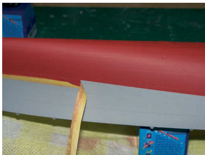
Masking tape was used on the hull during painting
