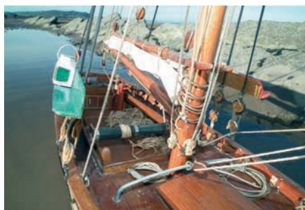
On the water, forward view showing staysail horse and mast
