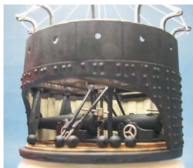
The USS Monitor turret showing the cut-out to view the interior (courtesy CIM)
