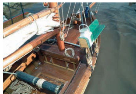
Stern view showing dandywink winch and starboard navigation light
