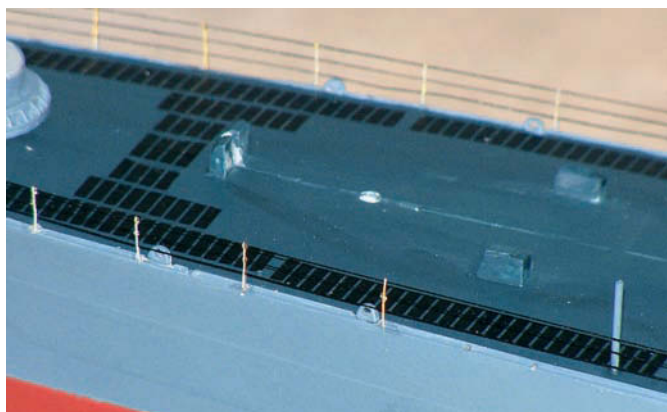
Stanchions fixed in position with black thread to represent the railings, note the anti-slip decals in place
