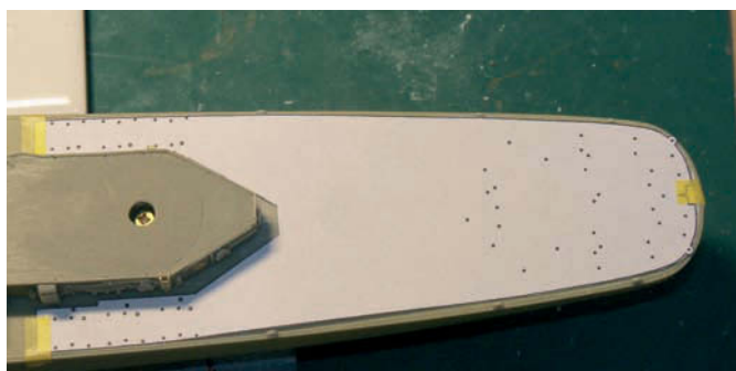
Templates attached to the deck to drill pilot holes for fittings
