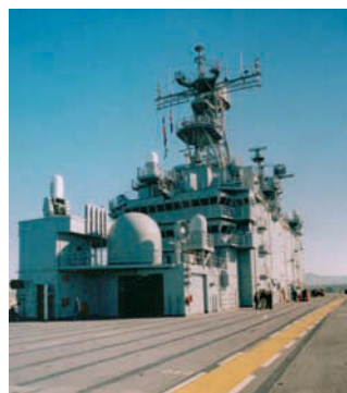
Forward view of island. Note large radome in front of the bridge structure and prominent yellow line running down the flight deck
