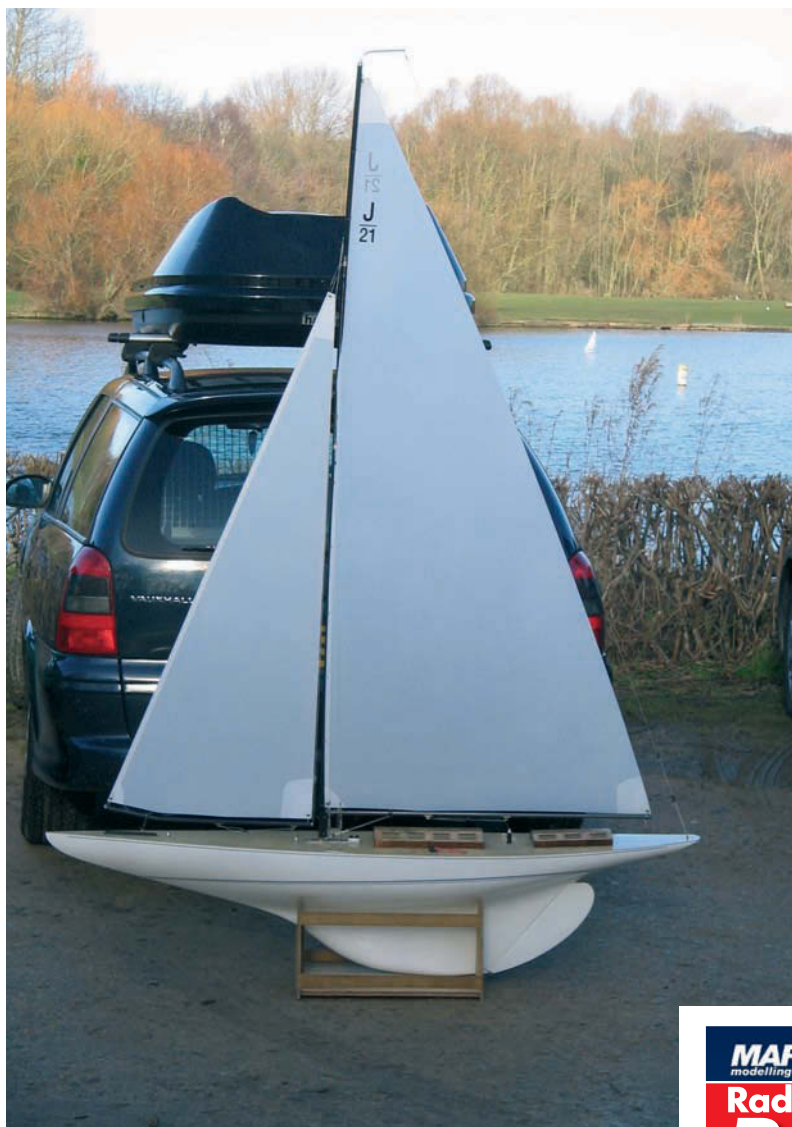
ABOVE: The prototype Nottingham 60 hull shows off its cloud of sail. This rig is deliberately large area to mimic the full size J class, and will be best suited to light wind conditions
