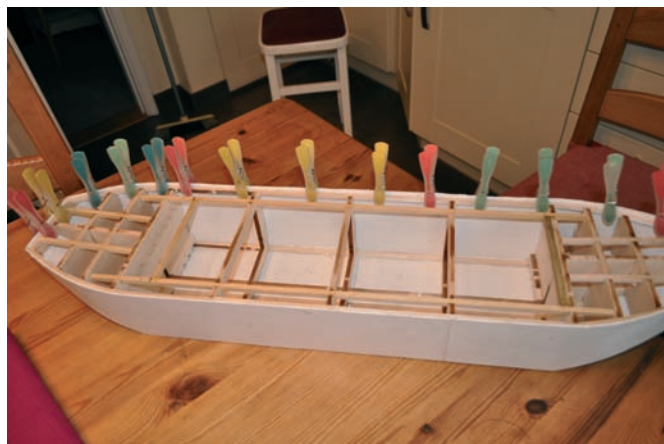
The hull is clad in Forex plastic sheet
