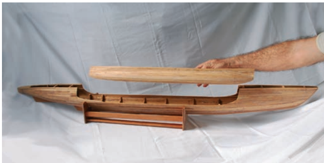
The hull with the detachable section during the construction process
