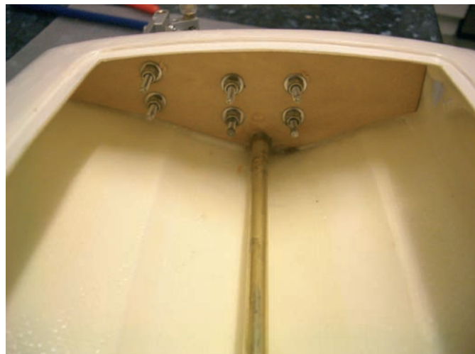
The inside of the transom with strut brackets, rudder a shaft outer tube fitted
