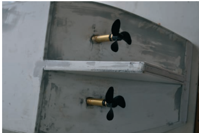
The props are the same handed and contrary to tradition this has little effect on the performance
