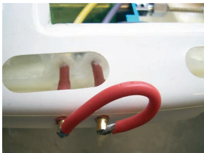
Safety loop fitted through hull side and flood chamber
