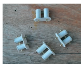
Bollards constructed from plastic tube, plasticard and brass rod
