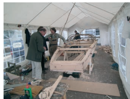
The hazel ribs being fitted
