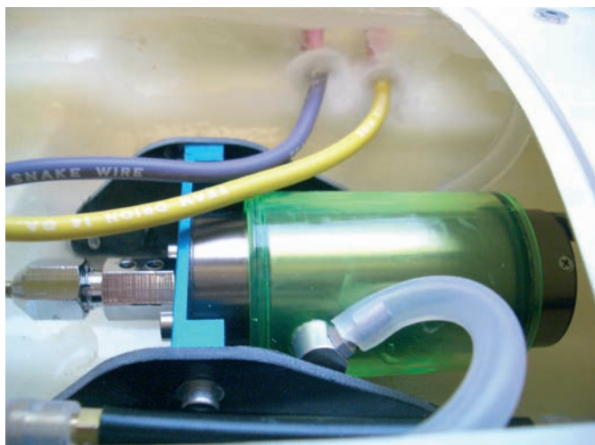
Close-up of motor assembly with water-cooling jacket. Also shows wire from safety loop sockets coming through the flood chamber
