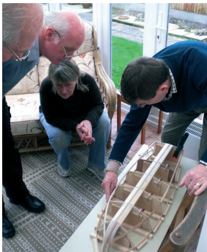
Ken explains to Dean, Dick and Lesley the intricacies of frames, stringers and the sheet building of an Aqua Riva style boat
