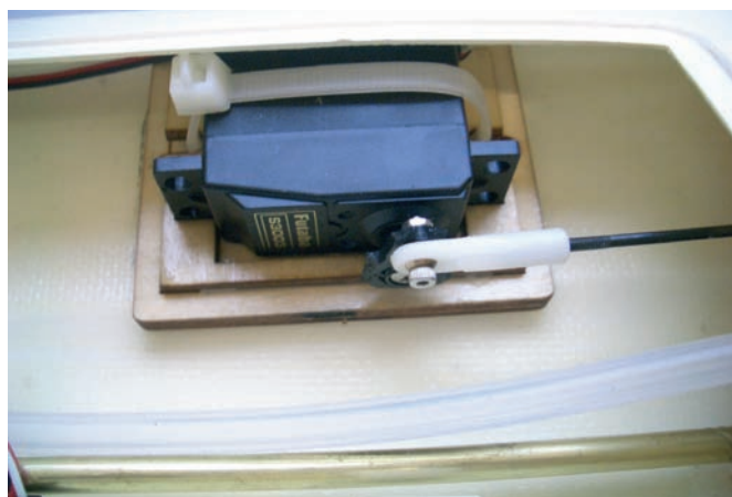
Rudder servo and wooden mount (see text)
