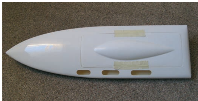
The Mono 1 hull, note the neatly cut flood chamber inlets
