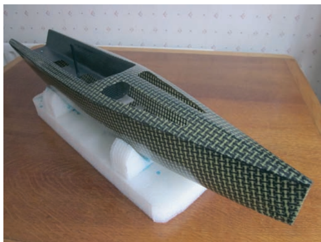
Carbon Kevlar as a hull moulding material
