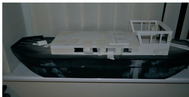
Assembly of the accommodation and bridge
