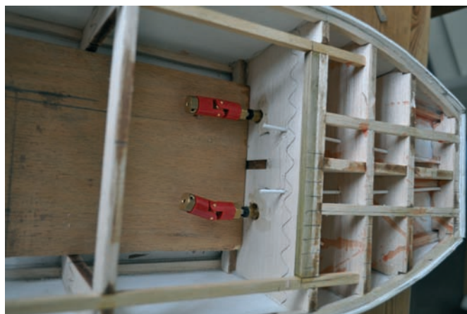
Twin prop shafts now fitted with tubes for the rudder control lines
