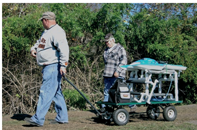
A lot of PVC pipe went into the construction of this cart's stand that doubles as a hot-pit 'workbench' and all four of the cart's wheel hubs are ball raced and turn pneumatic rubber tyres to smooth out the transporter's ride
