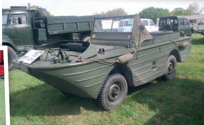
Side view with fenders and side windscreen canvas water deflector
