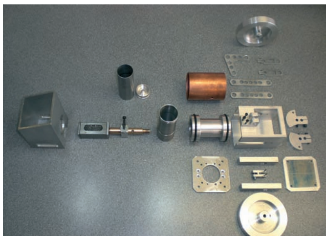
Some of the Stirling engine parts that have been fabricated by Ken on his lathe and milling machine, taken from the plans of Roy Darlington's famous book
