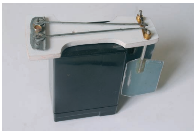
Rudders and linkage on top of a sealed 6 V 4.0 Ah lead/acid battery
