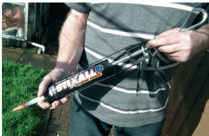
A building adhesive called Stixall was used to adhere the Forex cladding to the wooden hull frame
