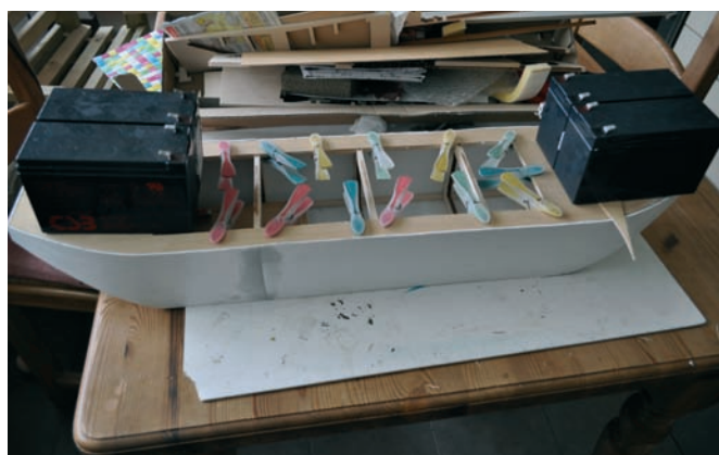
Ply sub deck now being fitted
