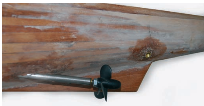
Prop shaft in its place, hole for rudder with metal tube inside
