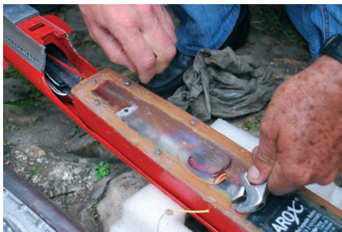
Checking the watertight seal
