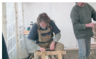
The other professional traditional boat builder, Padraig O Dunnin shapes the ends of the hazel ribs
