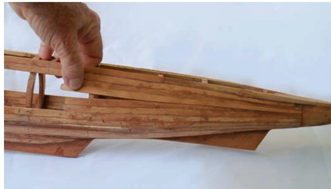
Strake by strake the hull was taking form. Stern detail
