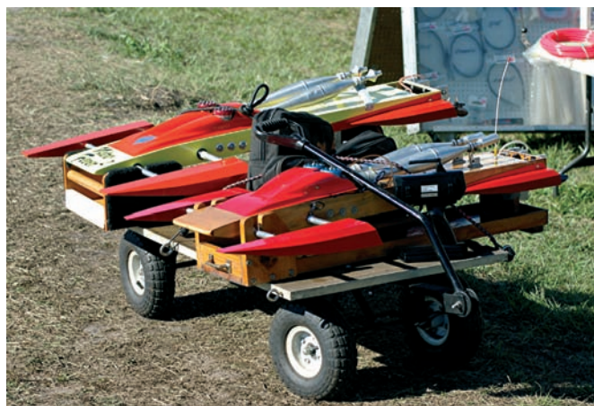
Metal hooks screwed into this wagon's wooden chassis top helps to retain the cradled hulls on the carrier and note how the pull handle has been bent to make it easier to move the cart from place to place
