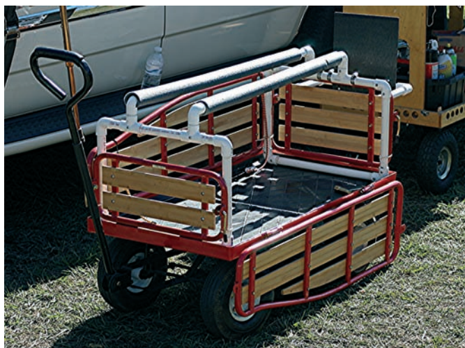
This heavy-duty steel yard cart features large tyres, hinged sides and a separate PVC plumbing pipe hull cradle. The unit also has ample gear storage for such things as starters, fuel cans/pumps and toolboxes
