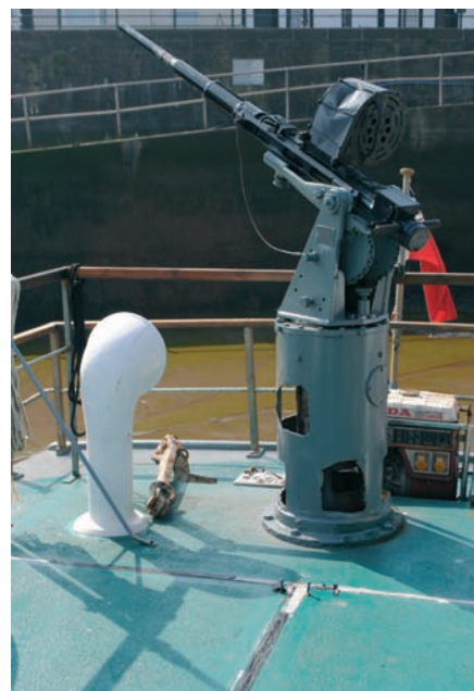
The 20 mm Oerlikon cannon on its mount
