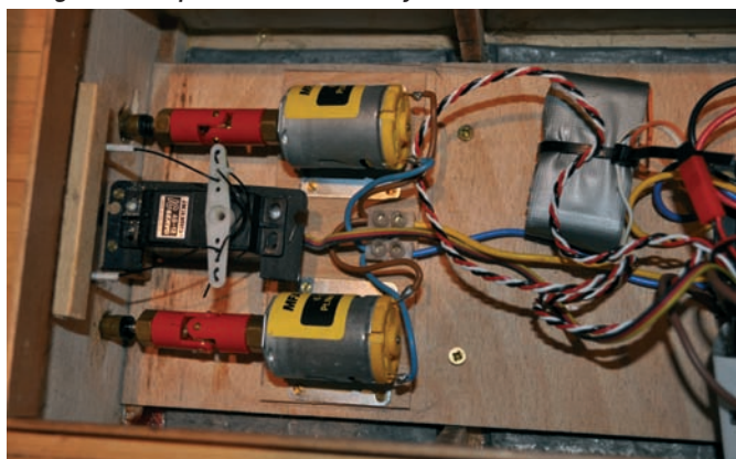
Motors, steering servo and receiver battery fitted
