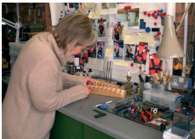
Lesley uses a pin-vise drill to prepare holes for Will Everard's – a Thames barge – plank on frame hull
