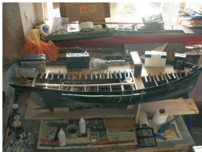
Fixing ply false deck
