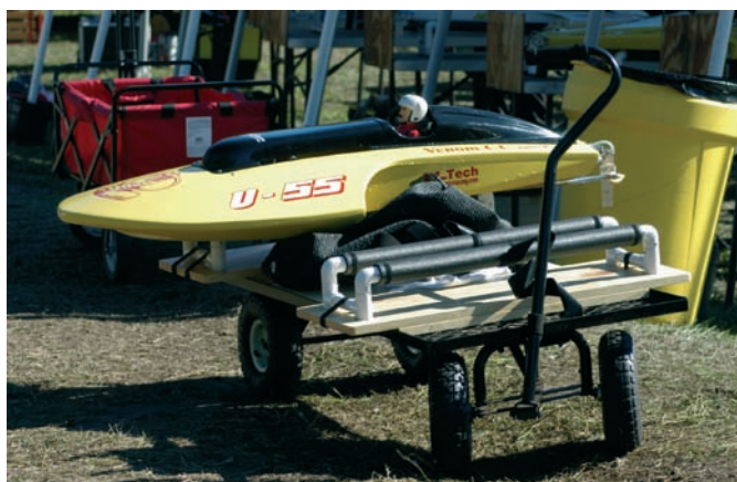
A regular yard cart is a good hull carrier as it comes with a pull handle that also steers the front wheels as you walk your boat to the staging area
