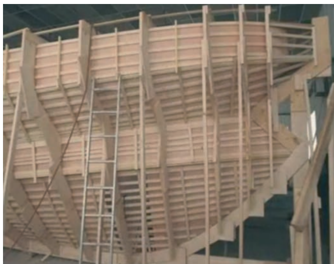
Full size ORC bow under construction (courtesy Bernard)
