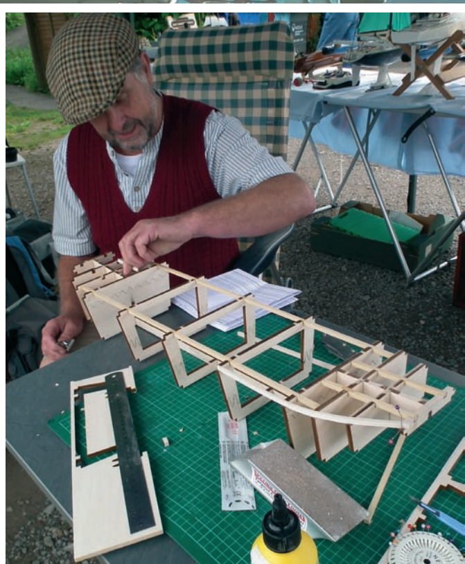
The author building the woodpack of the Lighter used as the hull for Josie
