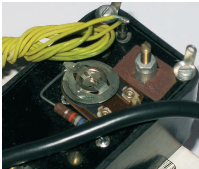
A close-up of the two tuning adjustments. The resistor is a 'sensitivity' control while the tuneable inductor is the RF tuning control
