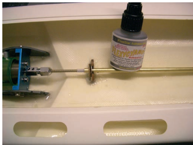
Original fitting of shaft showing unsupported flexi as explained in text
