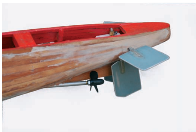
Stern, propeller, rudders and static hydroplane (but it is possible to change the angle)
