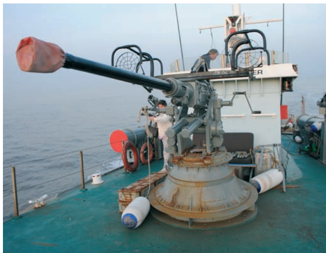
The Bofors 40 mm on its mount with iron anti-aircraft sights
