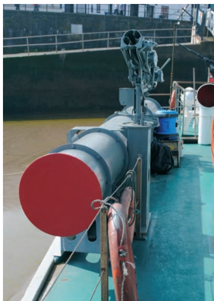
The replaced starboard torpedo tube and anti-aircraft rocket launcher
