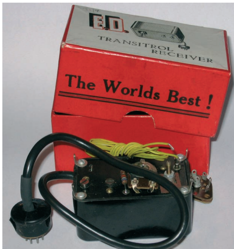
Britain's first 'modern' R/C receiver – a mint and boxed E.D. Transitrol part transistorised hybrid set
