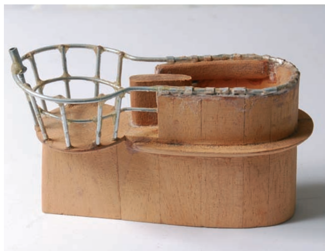
Turret with handrails, again bicycle spokes secured with epoxy
