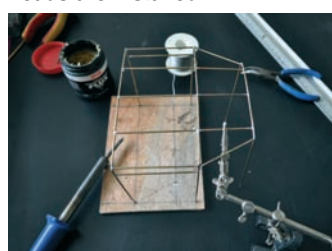
The framework of the rear awning is constructed from soldered brass wire
