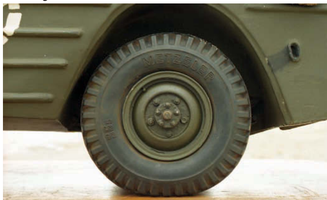
The rims were made in metal from aluminium off-cuts from the components of modern tanks. Tyres, meanwhile, were from ashtrays advertising Metzeler. On the right the exhaust outlet can be seen
