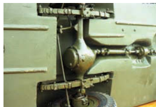
The front axle: from the worm gear a shaft enters the intermediate housing which drives the rear and forward axles. We can distinguish on the steering one of the steering boxes and a constant velocity joint
