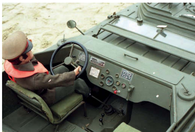
The dials on the relatively simple dashboard are all lit. The system for lowering the windscreen is a faithful reproduction of the original
