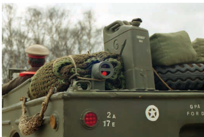
At the rear of the vehicle the brake lights and turn signals are all illuminated by LEDs. The reflectors are from bicycle reflectors
