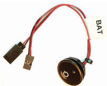
This brand new RMG deck mounted on-off switch and battery state reader was on the RC Winches stand at the MYA Trade Show
