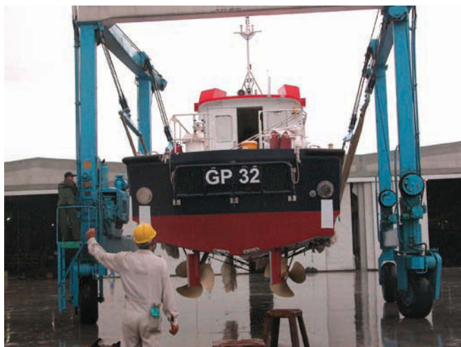
A clear view of the transom that shows exhaust outlets, hinged platform and the stepped chine
