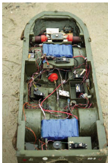
The interior of the GPA; the two motors that drive the worm gear are visible at the front
