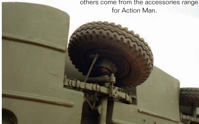
The steering of the vehicle is faithfully reproduced; steering boxes with a constant velocity joint, suspension, leaf springs and fastenings are all shown
