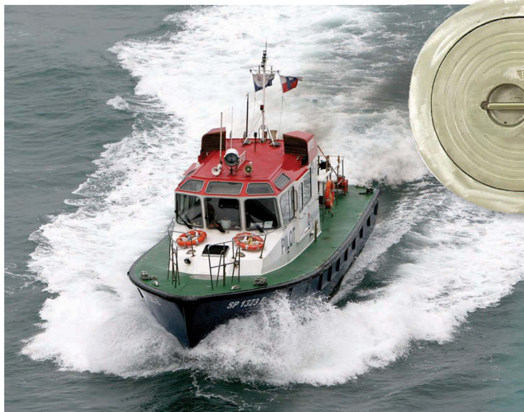
Singapore Pilot Boat SP1323E: this gives a good impression of the profile view of one of the series at speed. It is noticeable that the thickness of the rubber rubbing strake is also carried around the bow (courtesy Felix Toggenburger)
