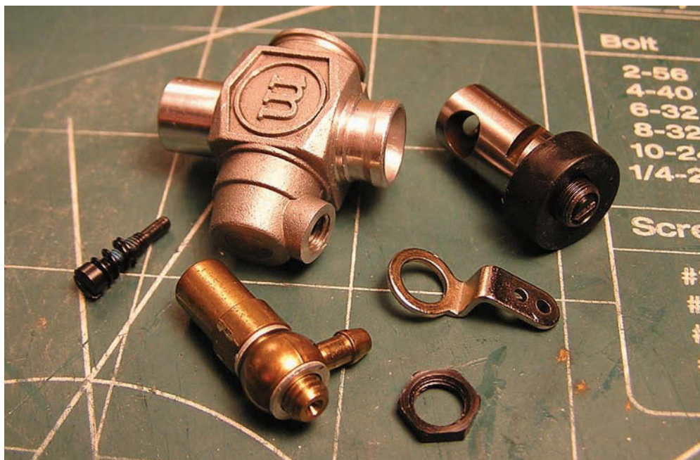
Over time a small marine nitro engine/carburettor assembly can get clogged up with old fuel, especially fuel that uses castor oil as a lubricant; so, a couple of cleaning cycles may be necessary to remove all the residue
