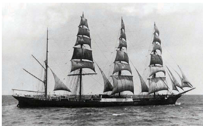
Moshulu again. She is sailing with the wind from abaft the port beam; over her 'left shoulder', so to speak. This is the best angle for the big barque to make progress, and her aftermost canvas has been furled, so as not to blanket the square sails, and to minimise the amount of yawing, about her course, that she would otherwise do
