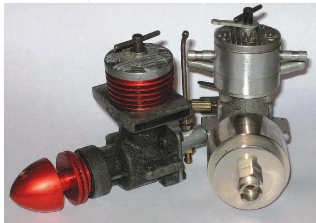
Two versions of the Racer diesel designed by Basil Miles for E.D. – the air-cooled item is a late 1950s engine, the marine version being much later
