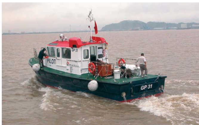
Singapore Pilot Boat view from aft, the twin-engine exhaust outlets and boarding hinged platform fitted on the transom are prominent in this picture
