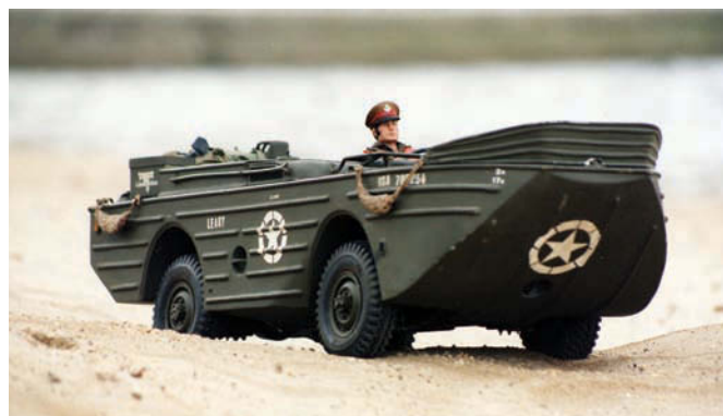
With the breakwater lowered into position the Ford GPA prepares to cross a stream
