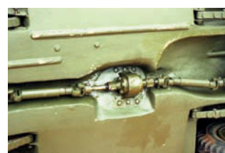
The intermediate housing is bolted directly to the hull and is driven by a shaft mounted on the worm gear. This box actuates the front and rear axles by means of shafts assembled on gimbals and universal joints
