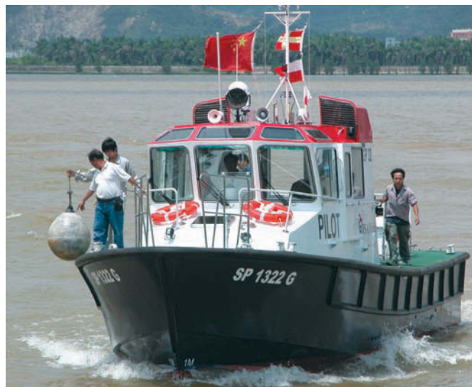
Singapore Pilot Boat SP1322G: bow view, which gives a good view of wheelhouse front, engine room intake vents and protective rubbing stakes along the side
