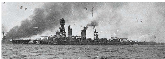
A Nagato class battleship provided with a funnel cap to her fore unit. A temporary measure to help reduce the effects of smoke effecting bridge personnel and equipment (IJN Department of Naval Aeronautics)
