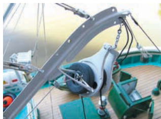
The system of fishing with the diablo (centre winch) operated by compressed air. The hoses can be clearly seen
