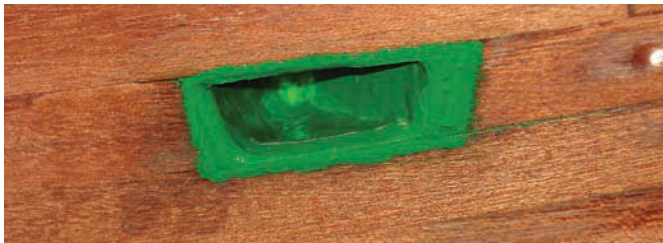
My replica of Altair's inset navigation lamp enclosures; the bulbs do of course need to go in before the deck planking is nailed and glued down
