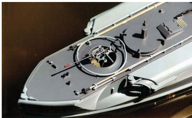
The forward deck section may be removed to access receiver installation
