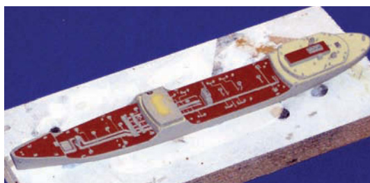
Hull and deck painted, attached to temporary wooden base using Blu-Tack
