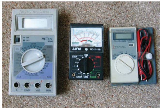
A selection of multimeters. Left my trusty 15-year-old Metex digital, middle is a small analogue meter, pretty accurate and still useful, and a Maplin pocket digital meter
