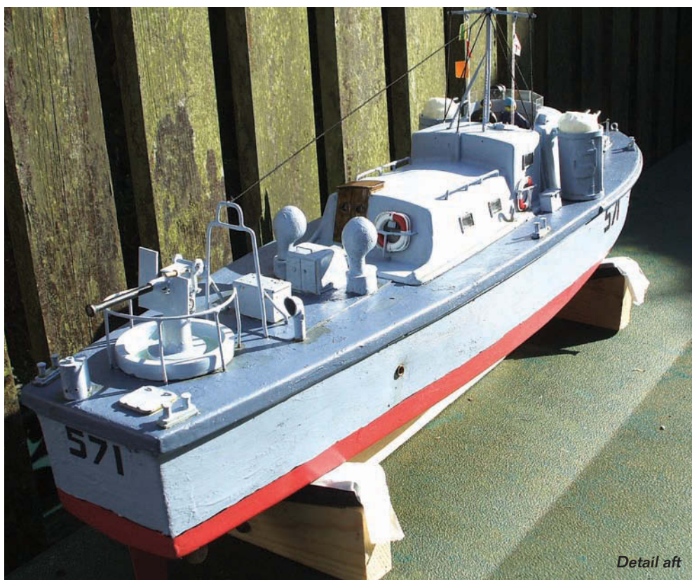
2 pounder and its guard built from scrap bits and domestic earth wire
