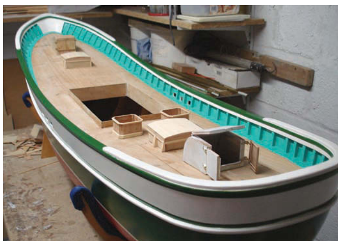
The completed bulwarks and hull strakes together with the under deck in position
