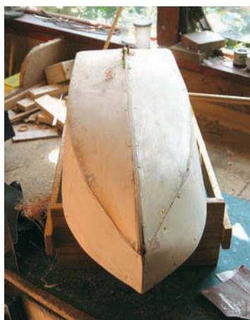
The model of Altair with her hull fully skinned and ready for spray strips
