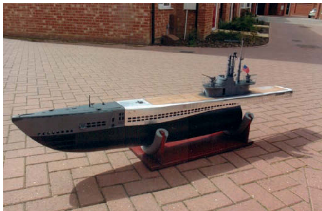
Completed forward deck section
