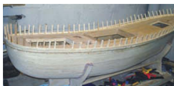
Installation of the bulwark stays
