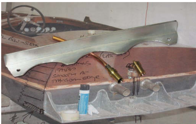
The aluminium deflector plate on Altair and my modelling of it
