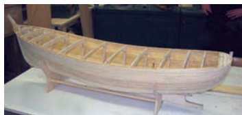
The finished plating gives an indication of the final quality of the construction
