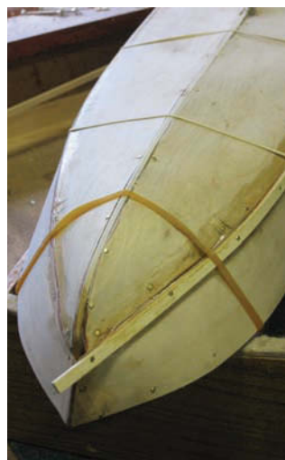
The first spray strip going on
