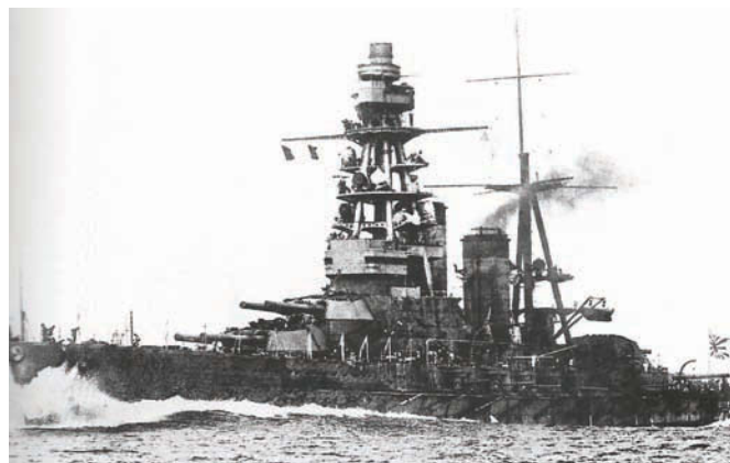
Nagato at sea as built, 20th October 1920 off Ugurujima achieving 26.7 knots on her trials. Her relatively open towering six-legged bridge structure is conveyed to good effect here, a feature well captured by Fujimi in their Amagi. (IJN Department of Naval Aeronautics)
