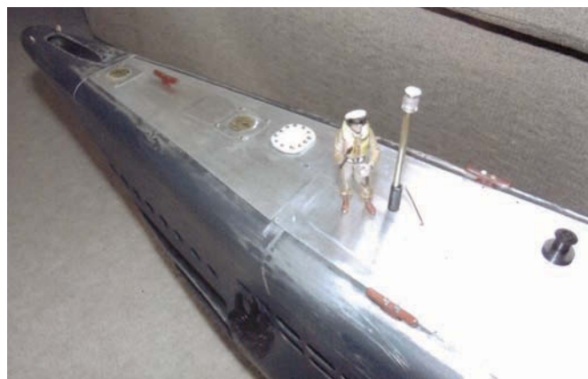
Scale fittings to bow deck section
