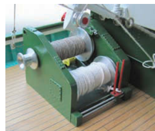
The winch. The caulking of the deck is clearly seen
