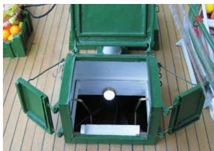
The rear hatch illuminated by ultra-bright LEDs encased in a plastic lampshade
