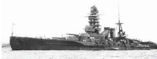
Another fine image of the evolving Nagato. It is noted that a good identification point between her and her sister the Mutsu during this period, was in their slightly different arrangements of steam pipes featured on their fore-funnel (IJN Department of Naval Aeronautics)
