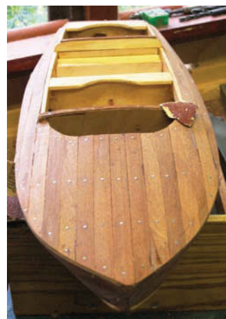
Deck planking going down; the sides have already been planked
