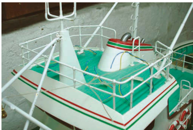
Installation of electrical wiring for lighting to the bridge
