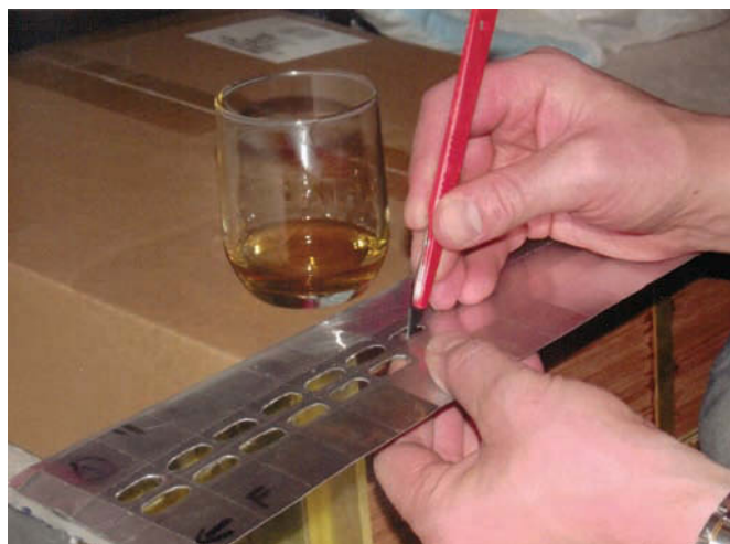
Cutting out the limber holes
