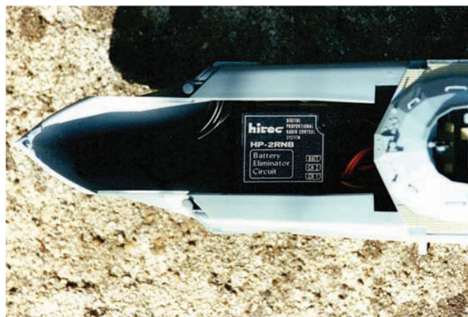
Hitec's HP2RNB receiver and antenna are placed below the front deck
