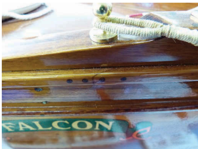
A plain scarf joint on the starboard side rubbing strake – it says it all
