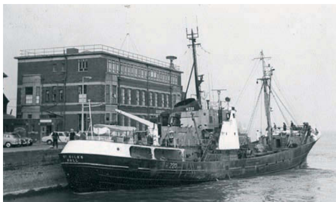
St Giles prepared to cast off at the entrance to St Andrews Dock at Hull. An additional radar scanner has been mounted on top of the wheelhouse, the aft trawl door can be seen stowed outboard of the aft gallows (courtesy of David Buckley collection)
