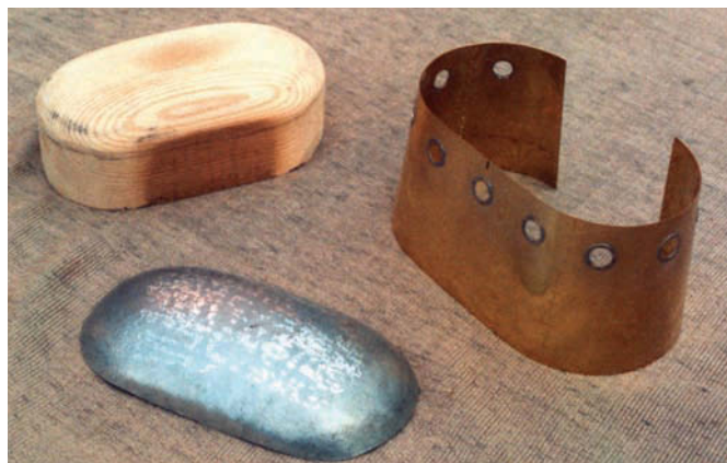
The cockpit of brass. The zinc roof and the wooden former on which it was hammered (R. Lefèvre)
