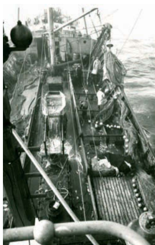
Trawl warp hanging block and attachment to the gallows, also with safety chain loop
