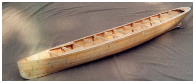
The wooden hull is of conventional construction followed by two layers of fibreglass and polyester resin (R. Lefèvre)
