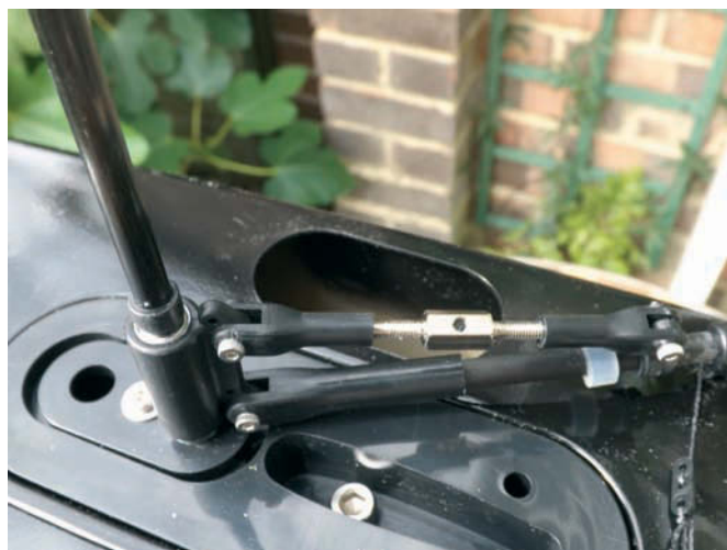
The superbly engineered gooseneck is central to the rig's performance and proved extremely friction free in light winds
