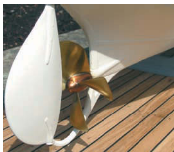
The hand-crafted four-bladed propeller made of copper
