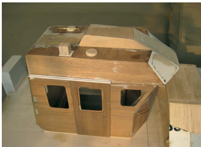
Hull and superstructures were built parallel from spruce
