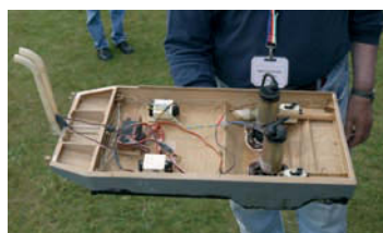
Mike Sheppard's experimental water jet model with butterfly valves for speed and steering. To be developed into a rescue craft for stranded models
