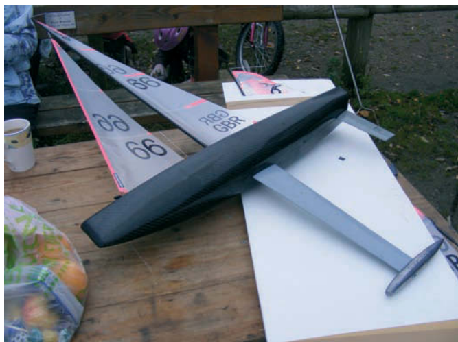
This is the original Ice, moulded in carbon fibre by Robot Yachts and sailed very effectively by designer Mark Dicks
