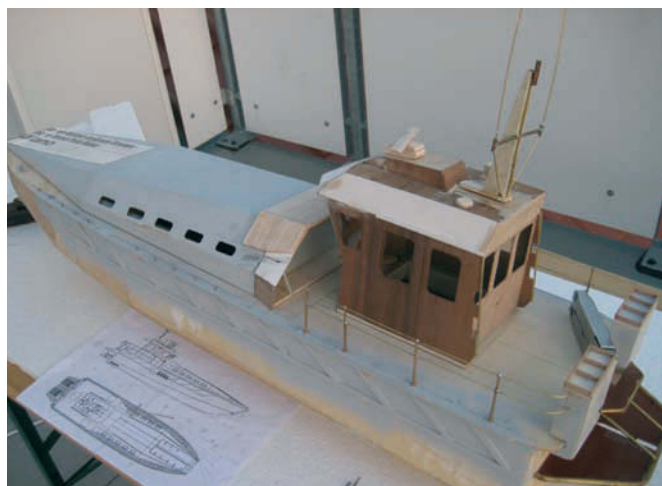
After finishing the construction jobs, spruce and GRP form a formidable craft
