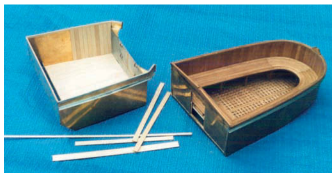
The front and rear seats trimmed with strips of plywood of 1 mm thickness (R. Lefèvre)
