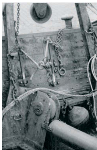
A view of the guide sheave angled at the bottom of the gallows fore leg with cover over the warp which leads to the port centre roller. The trawl door and one of the trawl bobbins should be noted. Just in frame is the warp hanging block
