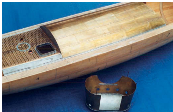
Central superstructure of brass and zinc (R. Lefèvre)
