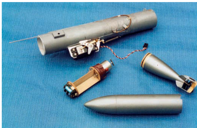
The torpedo tube and torpedo split into its three parts (R. Lefèvre)
