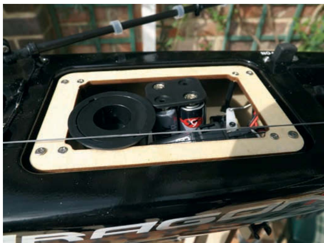
The Dragon Force main hatch open to show the compact installation of receiver, winch, rudder servo and battery pack holder, all of which comes set-up ready to run... just add four AA cells
