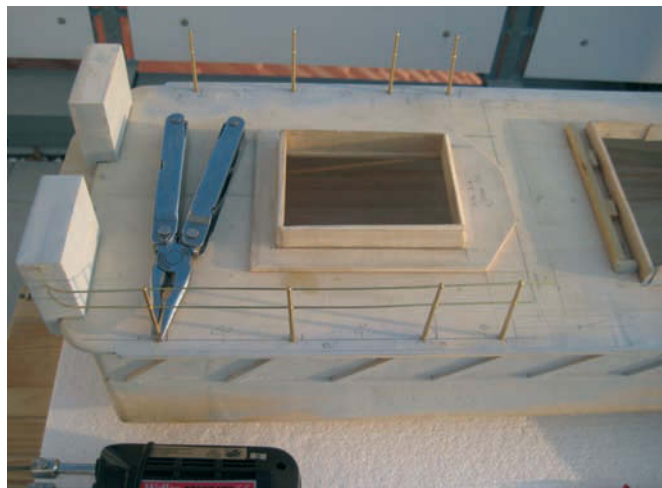
Railings are soldered together directly on the boat
