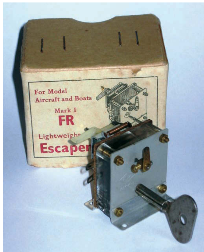
A Fred Rising two-pawl clockwork escapement controller with its winding key and in original box. Another very collectable mint and boxed item from the author's collection
