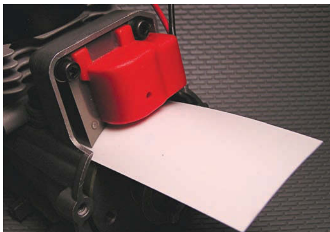
Positioned at the point where the engine flywheel's magnets match up with the module's laminated 'legs', the paper card creates the clearance at which point you can tighten the module screws and remove the card
