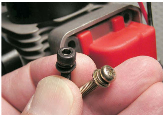
Made from a relatively soft metal the module's twin Phillips-head screws can be replaced with hardened Allen-head fasteners that will be easier to work with when adjusting the module
