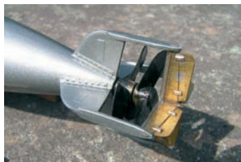
Contra-rotating propellers steer the torpedo via a small radio-control system
