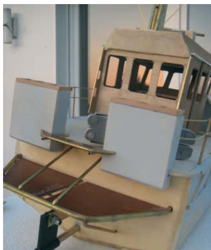
The boat's bow platform was made utilising brass and board material
