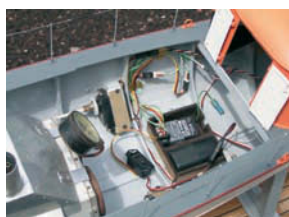
The entire radio is installed in the front of the model to allow maximum space for the installation of the steam engine and its boiler
