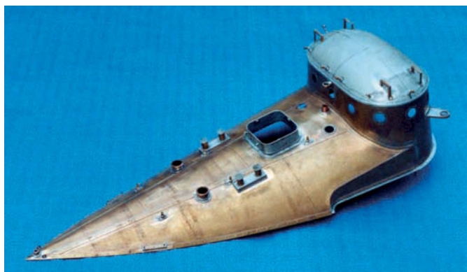
The forecastle almost finished and soldered to the cockpit (R. Lefèvre)
