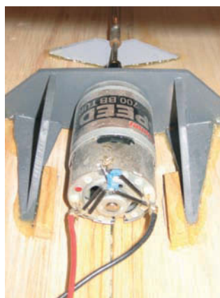
E-Power: Graupner's 700 BB was installed, but is supposed to be replaced by a 6 cc later on
