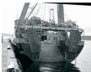
This shows a typical trawl board, on a stern trawler in this instance
