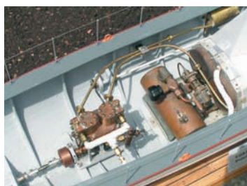
The steam engine, a personally designed vertical-twin classic
