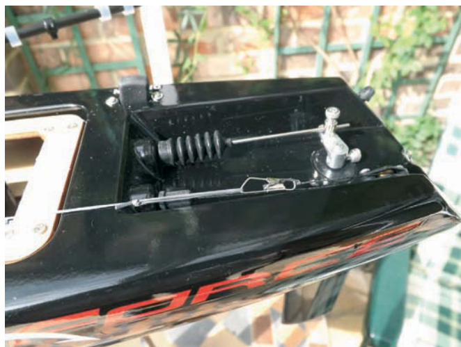
The stern deck layout is neat and follows normal racing RG65 style, note the easily reached on-off switch, and the pulley-block to turn the sheet line without friction
