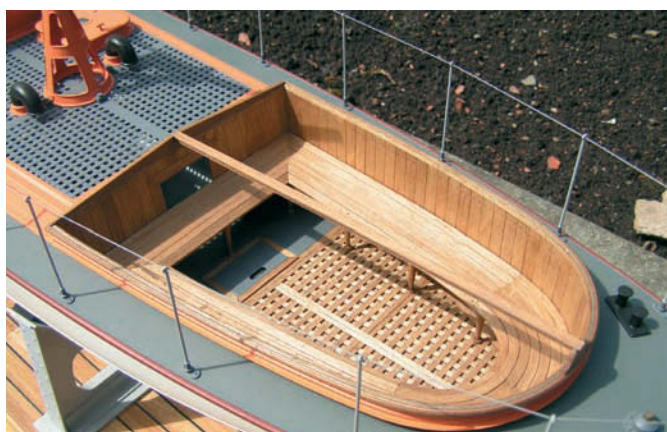
The rear seat and curved slats are cut from a sheet of 1 mm thick plywood
