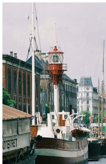
Although built from wood, beacon and superstructures have been made from metal
