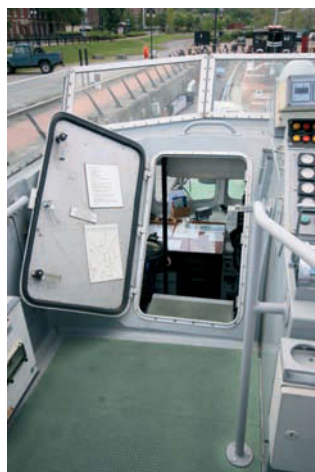
Access door to flying bridge
