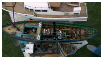
All scratch-built, including the steam plant and engine
