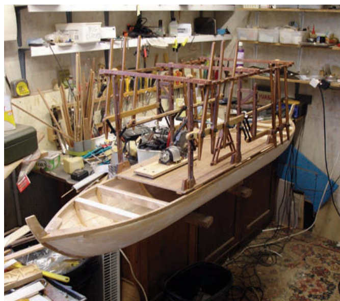
The drive system attached to the hull
