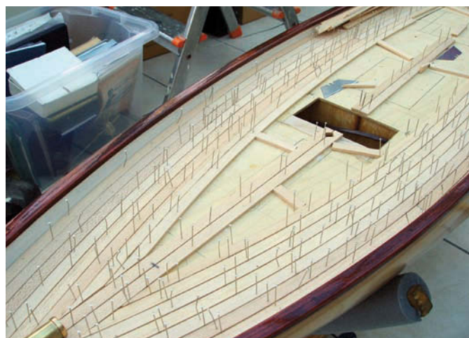
Deck planking underway showing liberal use of pins, and pins used for plank spacing
