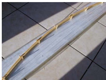
Deck edge capping rail glued (two pieces of wood dry bent and glued/pegged for shape)
