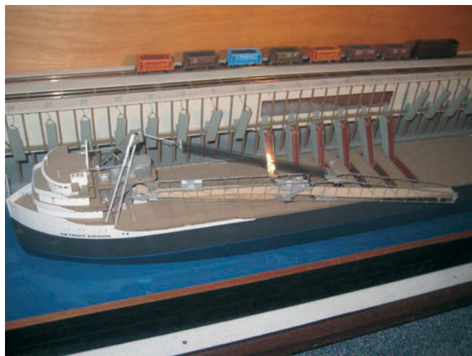
Unloading bulkers was extremely labour intensive. Conveyor belts allow unloading without men working in the cargo hold, as is represented by a model of Detroit Edison
