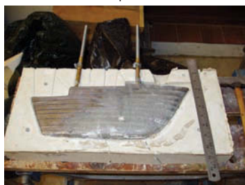
The cast lead keel in the plaster mould showing the fixing bolts
