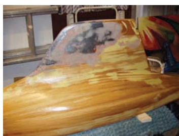
Fibreglassing completed showing the final position of the lead keel
