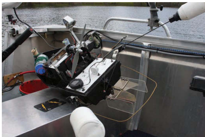
Rear buoys assist in turning the craft
