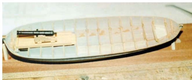
The hull ready to start deck planking
