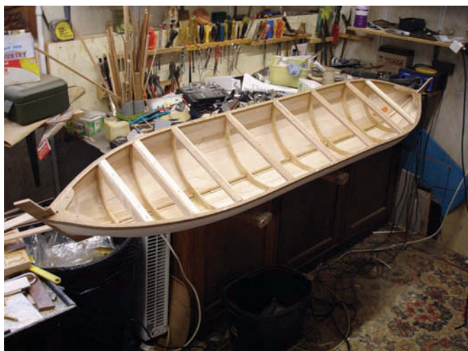
Ready for the fibreglass covering, inside and out
