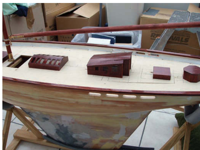
Superstructure underway and main boom joint – note ports for water drainage and hole behind mast for the battery
