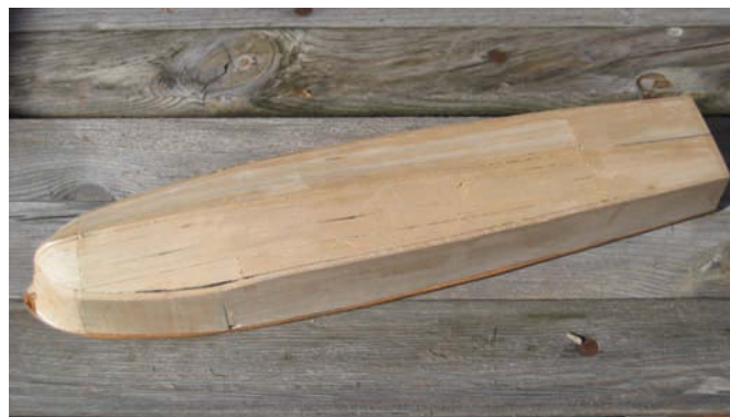
Made entirely from wood, GRP was used to strengthen the hull
