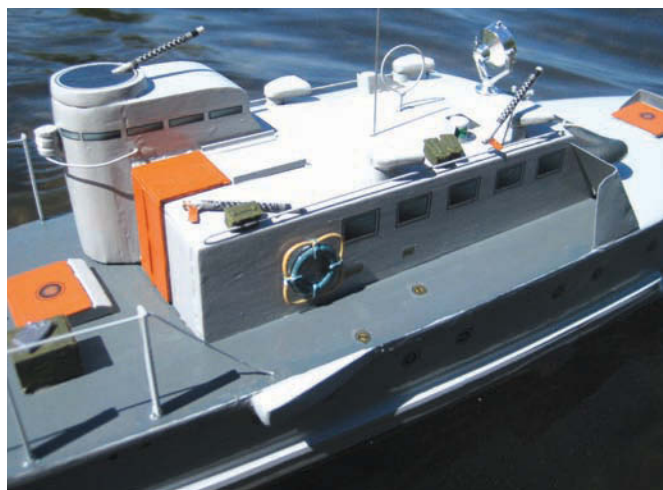
The deckhouse seals off the opening to access the R/C equipment
