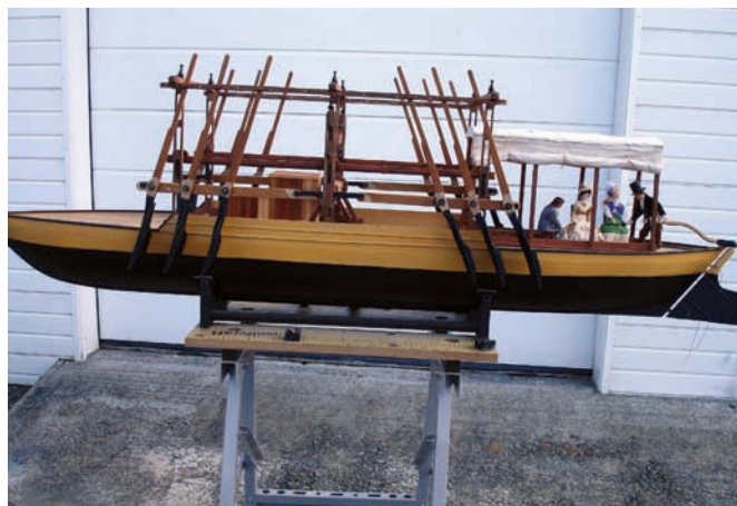
A clear view of the rudder assembly and paddles
