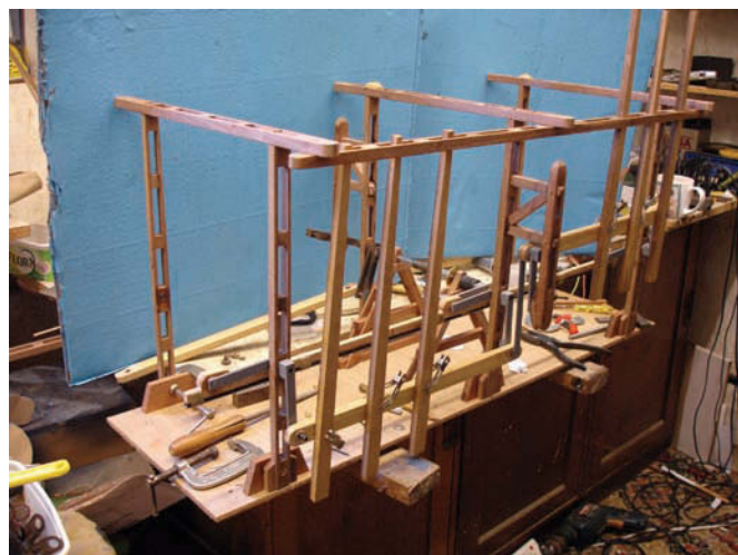
The mechanical unit being built on a board, which is actually the centre deck area
