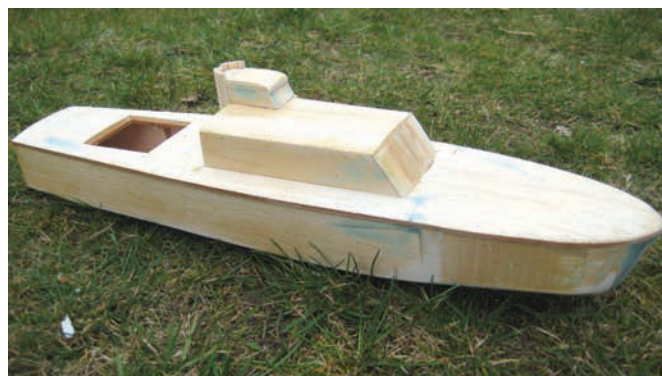
Balsa deck and a plywood cabin give an indication of the boat's future looks
