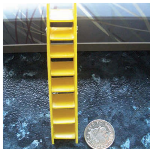
Complete trimmed ladder awaiting final sanding and finishing
