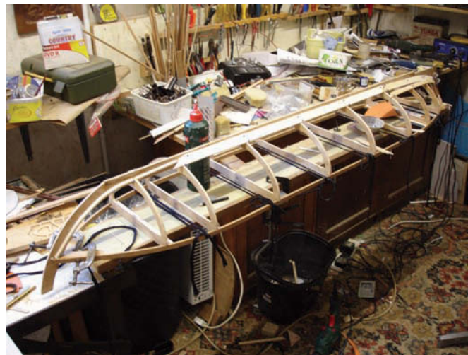
Keel and frames used in the second attempt at a hull
