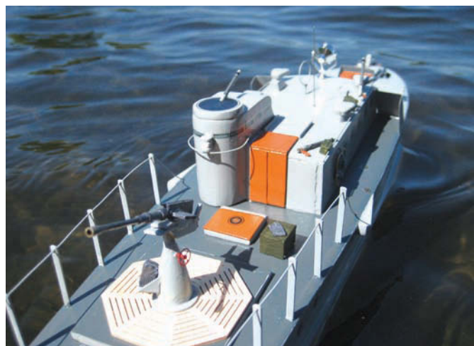
Meant to protect the crew from spray and mist, the deflectors keep the model dry, too
