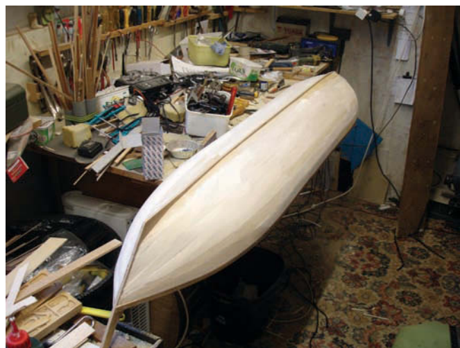
The hull is planked in balsa strips
