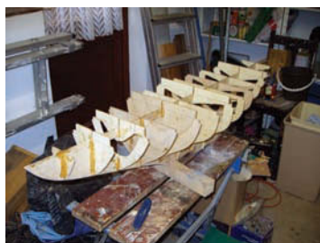
Early frame construction showing solid bulkheads in line with the main shrouds
