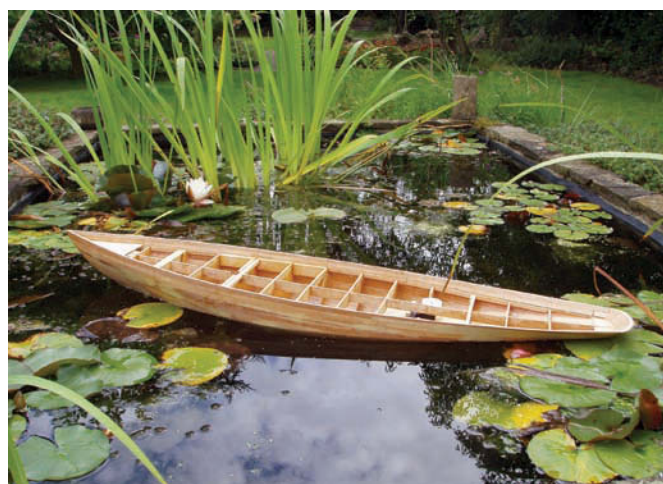
First floatation test showing unanticipated bow up angle and the Hi-tec sail winch
