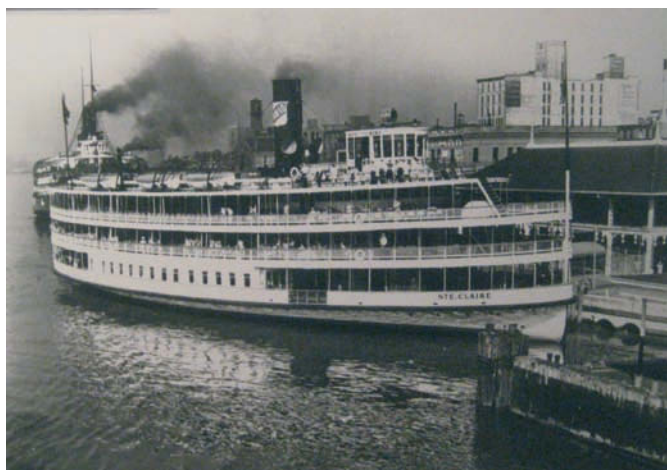
Built in 1910 and measuring (L x W x D) 181 x 50 x 15 feet, Ste. Claire was the last of the large Bob-Lo boats built for the Detroit, Belle Isle and Windsor Ferry Comp
