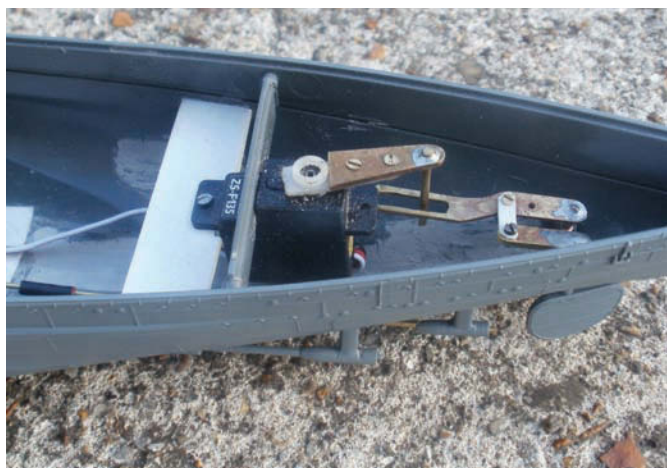
Owing to the narrow stern a different method was adapted for Kirishima. A single tiller arm with a slot for an activating pin connected to the servo arm. The two rudders are connected with a flexible arm
