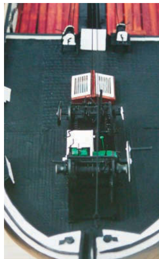
Overhead shot of the forecastle with all engine driven winches and two operated by hand to control the net booms
