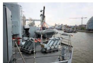
Portside looking aft at rear superstructure – note chaff launchers
