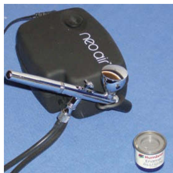
Neo Air miniature compressor with airbrush holder in place, the paint pot gives an indication of size
