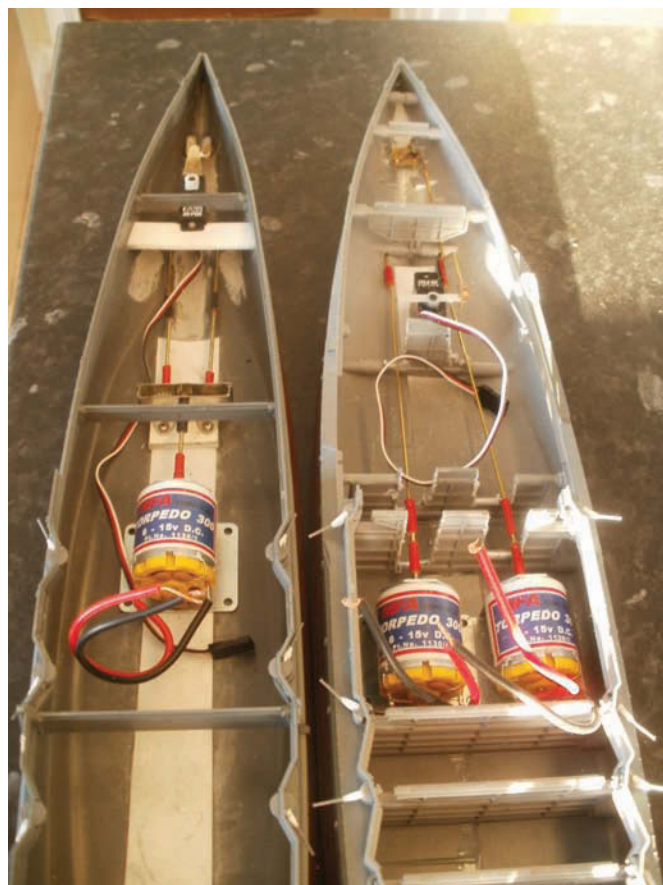
Nagato and Kirishima side by side for comparison with Akagi. Nagato has a similar layout as Akagi but owing to the narrowness of Kirishima's beam only one motor was used with a suitable gearbox connected to the two propeller shafts
