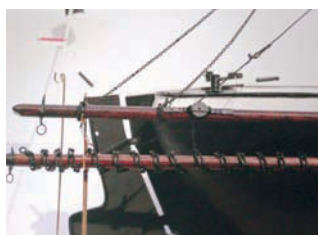
To ease operations, net booms had been weighted with chains
