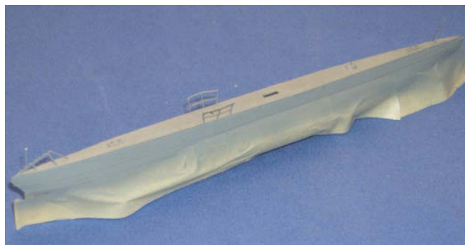
Lower section masked, next colour has been applied
