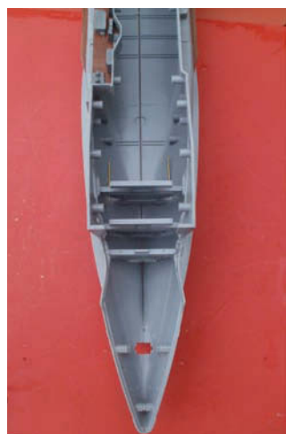
The halves temporarily joined showing the slot for the rudder insert and the new propeller shafts. The retained bulkheads are also visible
