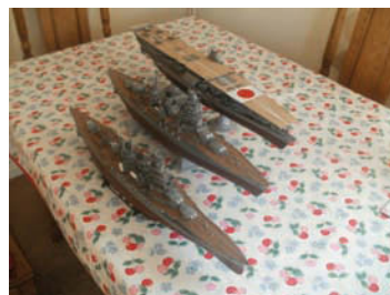
Nagato and Kirishima side by side for comparison with Akagi. Nagato has a similar layout as Akagi but owing to the narrowness of Kirishima's beam only one motor was used with a suitable gearbox connected to the two propeller shafts
