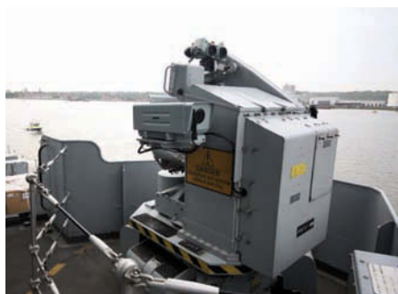
Electronic sights on bridge wing port and starboard
