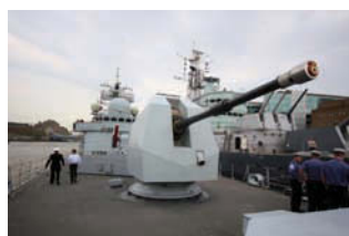
Vickers 4.5 inch Mk.8 Mod 1 Kryten semi-automatic main gun
