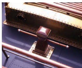
Over 3,000 lace pins are necessary to reproduce the riveting
