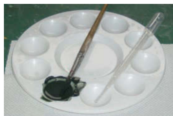
Pipette used to add thinners a drop at a time when mixing
