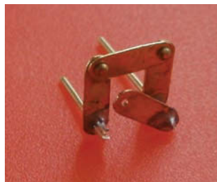
The rudder paralleling device for Akagi ready to be fitted
