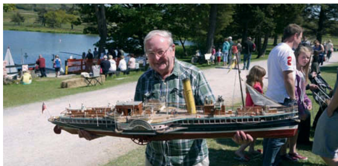
Graham Charles' Dutchess of Fife (1903-1953) paddle steamer. Mostly scratch-built with seven or eight layers of 'gum paper' strip and varnish to cover the hull. Thin plastic was then used to simulate the plating
