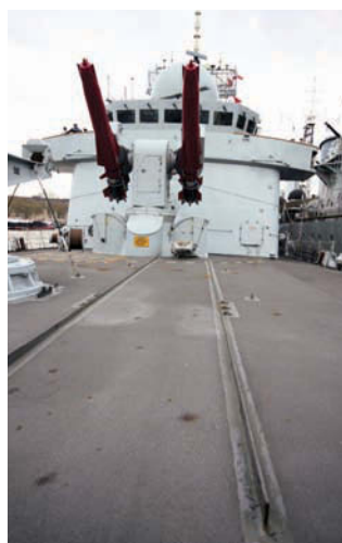
Forward superstructure and Seadart launcher
