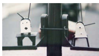
Different in size, but serving the same purpose. Two small winches allowed control of the net booms on Aranka
