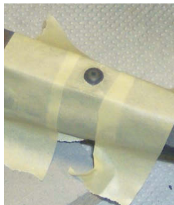
Masking tape in place around dome
