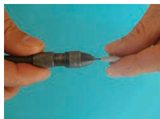
Drilling out the outer propeller supports for new brass propeller shafts
