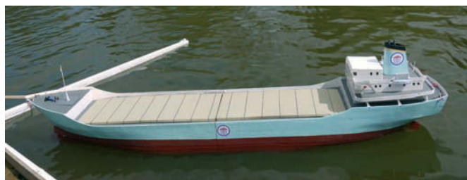
Challenger is 10 ft 6" long and uses a water ballasting system. Built by Tony and Jon Simons and Roger Keep of the Mid-Thames Model Boat Club
