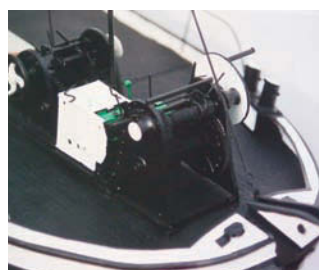
The forecastle was dominated by winches. Left to right: windlass, diesel and gearbox, capstan
