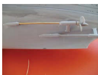
The outer propeller shafts in place with the attached propellers
