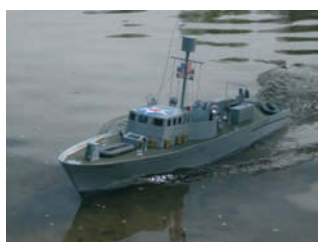
Twin props and low weight due to the GRP hull clearly increases the model's performance
