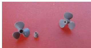
Propellers for Akagi showing the experimental polystyrene inserts to match the new shafts
