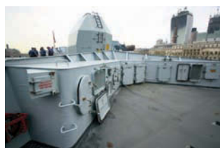
Breakwater positioned between main gun and Seadart launcher
