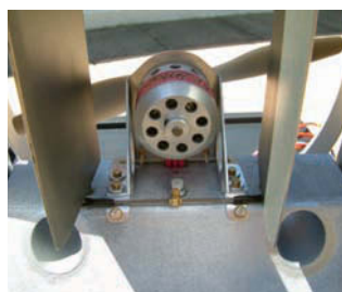
Rear view of duct shows motor, rudders and blast holes
