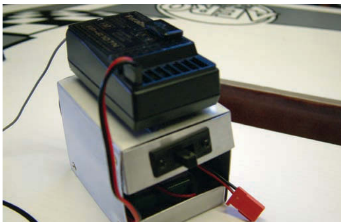
Small aluminium module housing, receiver and battery, and later the gyro
