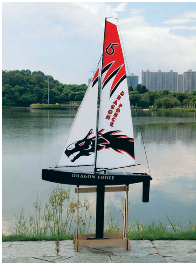
The Joysway Dragon Force has a 300 mm depth keel and high ballast ratio, which should ensure excellent performance
