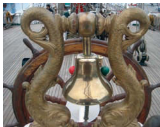
The bell atop the helm. All sail signals, obstacles seen and the time are communicated via this bell aboard Sedov
