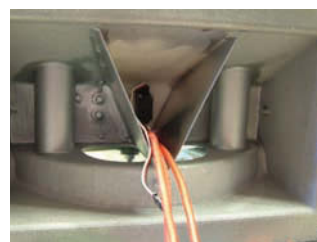
Underside of duct support shows embedded rudder servo and aluminium splitter plate
