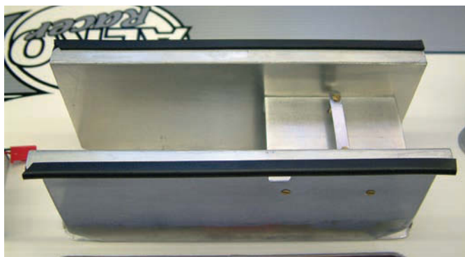
Aluminium module for housing battery and speed controller
