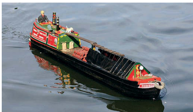
Built using the plank on frame method Steve Johnson's narrow boat features a traditional narrow boat finish
