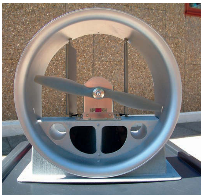
Front view of duct showing blast holes and first attempt at air bag openings
