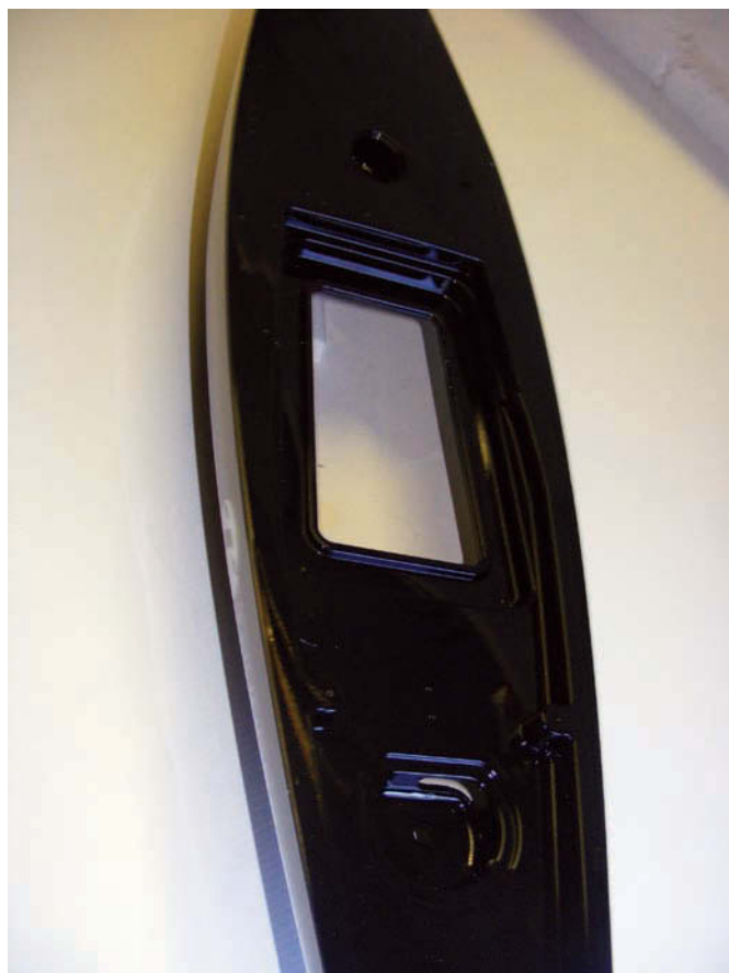
The deck has a well-moulded central access, which allows the builder to get to some of the fittings as they are secured before inserting the radio tray assembly
