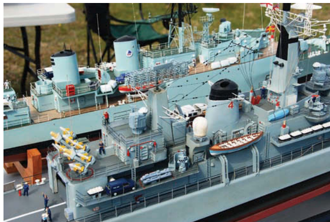
Detail on HMS Cleopatra, a Batch 2 Leander class frigate, shown with the Exocet anti-ship missile system installed
