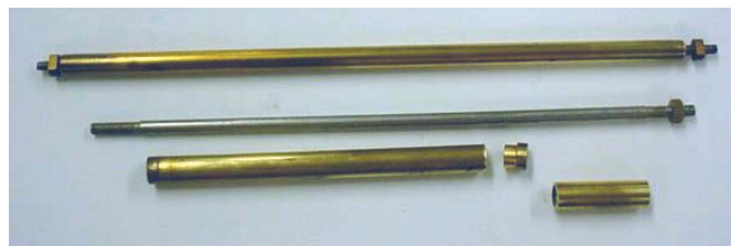
Evolution of an exposed shaft using a commercial prop shaft. Photo shows a standard enclosed shaft, below it the shaft removed and the outer tube cut to length. Also shows the bearing removed from the waste tube ready to be fitted in the shortened outer
