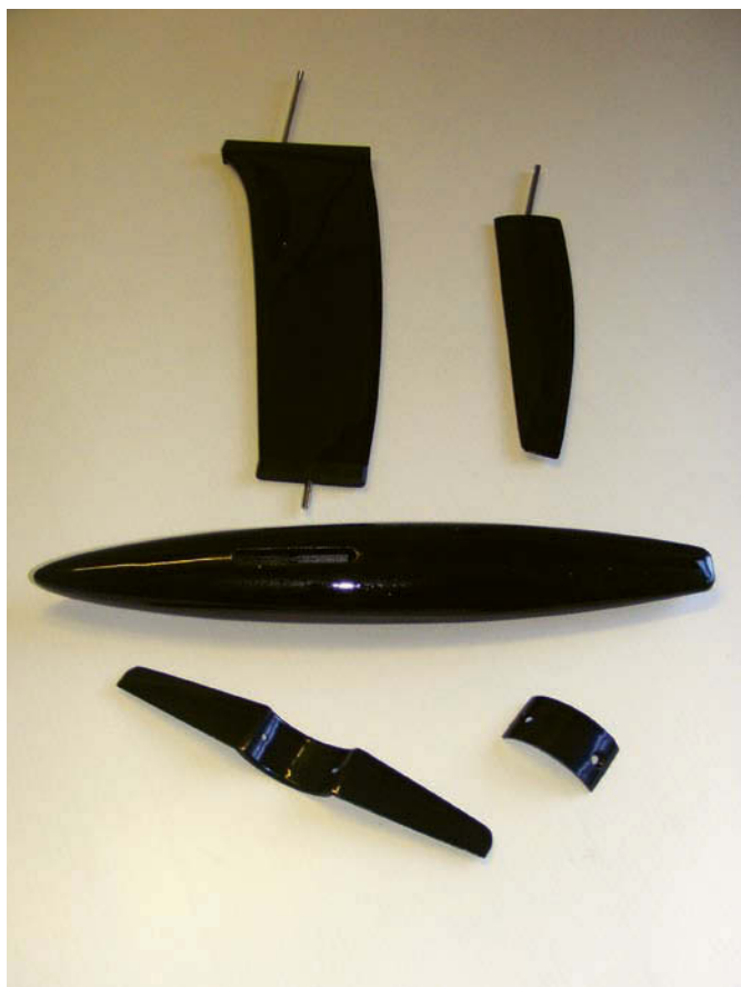
The keel blade with rod for hull attachment, threaded rod for ballast bulb, and both alternative keel accessories, plain and the wing aileron
