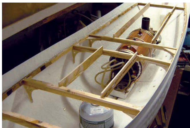
Rigidity of the hull improved after fitting whales
