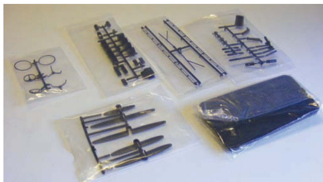
The main plastic parts are moulded on sprues much like a giant plastic kit
