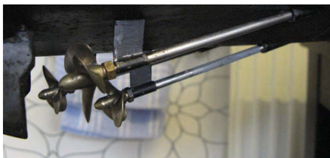
Triple shaft set-up on my MASB (see text)
