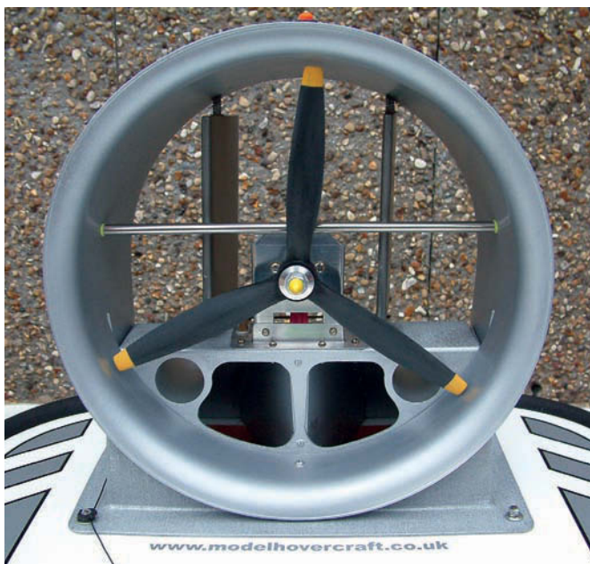
Modified duct air bag orifices are larger to obtain correct bag inflation and three-bladed prop fitted
