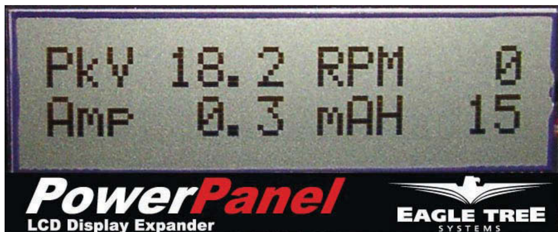
LCD PowerPanel showing the 'live' values being logged
