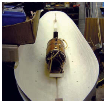
Trial fit of steam plant
