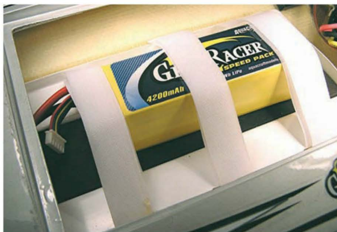
Using three loops of Velcro strip the hull's 4S LiPo pack was secured to the inner battery tray. However, any pair of NiMH or LiPo packs can be put side-by-side or in a stacked position using the tray/Velcro set-up
