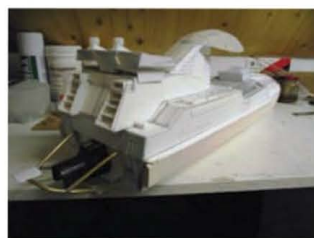
A shot showing the addition of louvers to the two stack engine exhaust outlets, and the fixing of the square section balsa to the side rails. Scribe lines can be seen on the body panels (Photo – Chris Scott)
