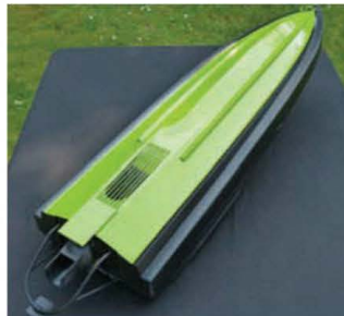
The underside reveals detail and finish. Note the small rectangular plate attached to the water jet protection bar – Chris moved and adjusted this a number of times on different waters, to keep the 'rooster tail' spray to a minimum and the propulsion low and to a maximum
