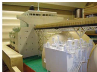
Top walkway starts to meet the superstructure. Also showing loose fitted reliquefaction plant, pipe work made from sprue, (scrap from old plastic models)
