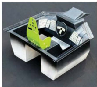
The cockpit with the windscreen now attached, also note the sloping front face to the seat now
