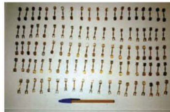
Mass produced Harland & Wolff patent rigging screws. Each consists of seven separate parts
