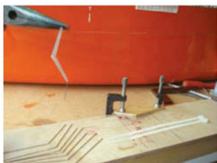
Showing two of the tapered ends of small cable ties joined together with piano wire to form hydraulic arms for fenders
