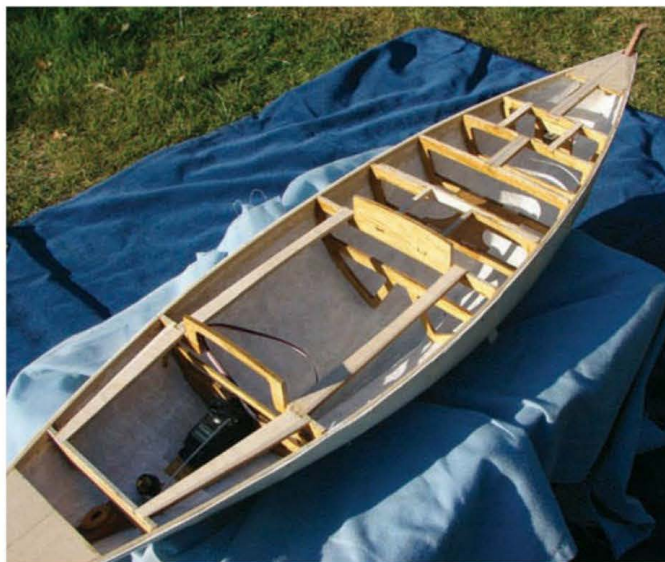
The servos are scribed and the hatches take shape
