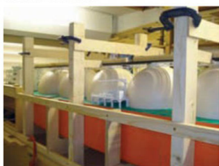
Cradle made to hold ship hull and to line up top walkway. Gives a centre line to measure from
