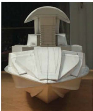
Head-on clearly shows the stepped stages and thicknesses of styrene card used. The centre line is paramount to any build and can be seen on many of the components in the build photos (Photo – Chris Scott)
