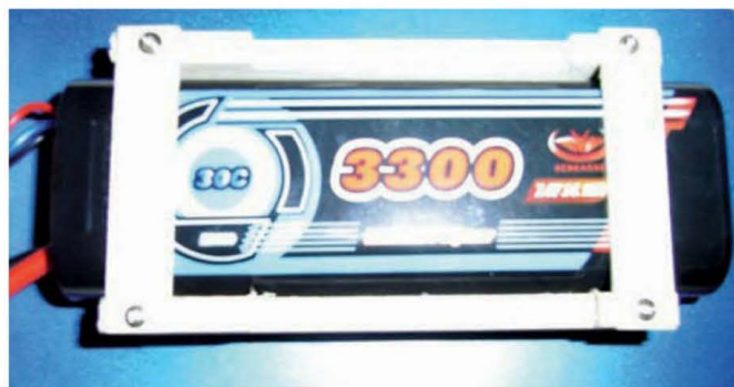
This 3300 mAh LiPo is rated at 30C, which implies it could deliver an impressive 99 amps
