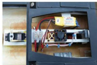
A sub-frame has now been added above the motor to take the cooling fan, electrical connection and Spektrum receiver. Balancing lead weights can also be seen on the bottom of the hull
