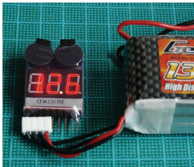
A LiPo Voltage alarm fitted and displaying the total pack voltage
