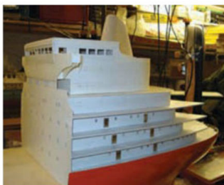
Rear superstructure loose fitted and made from plasticard and foamex sheet. Funnel carved from balsa wood
