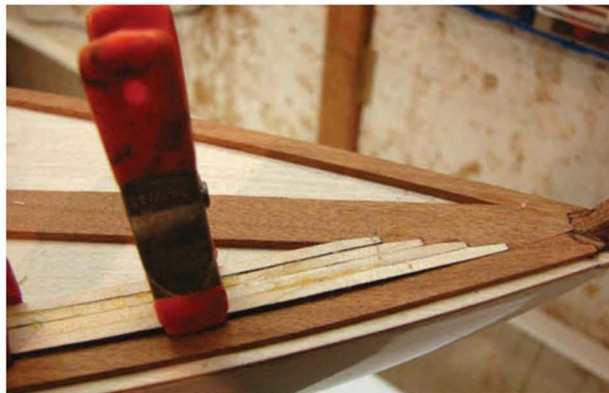
Planks were joggled in, four or five at a time
