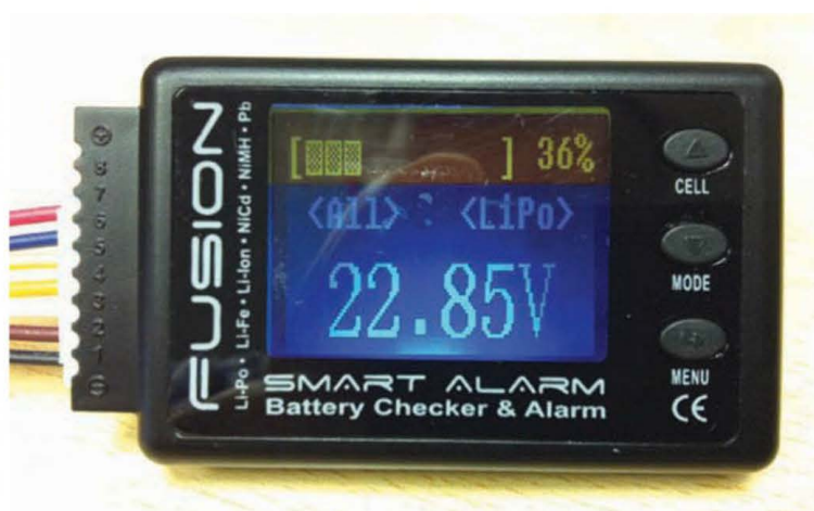
The bright display can show many functions, this one is showing voltage
