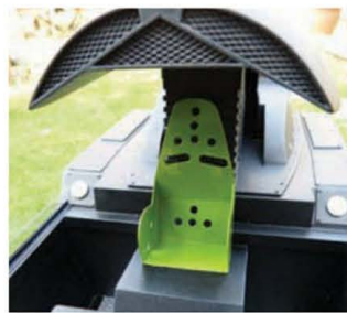
The front of the rollover bar canopy showing the detail on the air inlets, made with car body repair aluminium mesh
