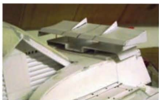
The rear mounted, two layered aerofoil section wing being styrene sheet cut to shape, sometimes gently heated and shaped, before gluing in place. Humbrol filler was used and Peco track pins to give simulated bolt heads – much used by Chris to good effect (Photo – Chris Scott)
