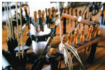
Foremast with spider band and fife rail
