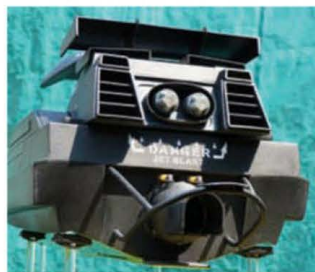
This stern shot shows the exhaust nozzles, above the signage, which Chris cast in resin
