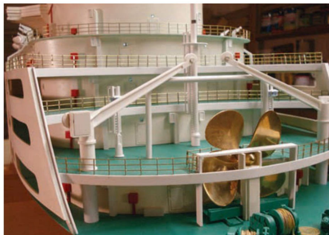
Showing spare propeller and lower working deck
