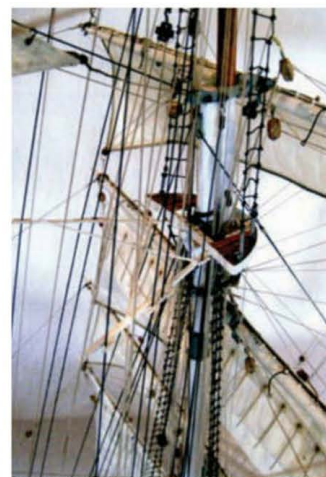
The topgallant mast doublings and spreader centre left
