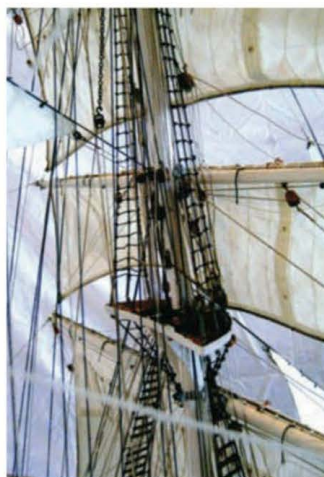
Just over 1600 feet of rope was needed to rig this model. The futtock shrouds are clearly visible
