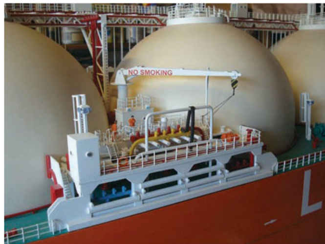
The goal post is the handle to lift off these loading/discharge terminals that conceal the deck joint underneath
