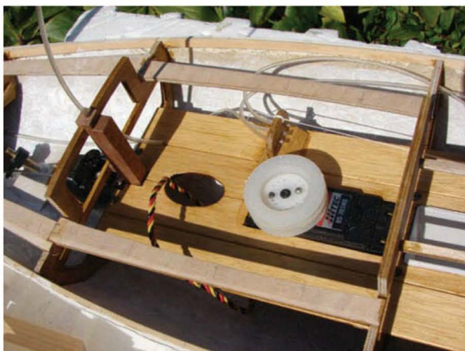
Plastic tubes route the sheets to the sails
