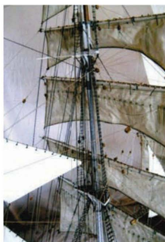
General view of the square sails; the model is rigged exactly as was the original
