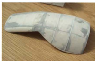
The rear canopy engine air inlet cover in its early stages of construction; notice the balsa wood in-fills between the styrene sections and the use of P38 car filler compound (Photo – Chris Scott)
