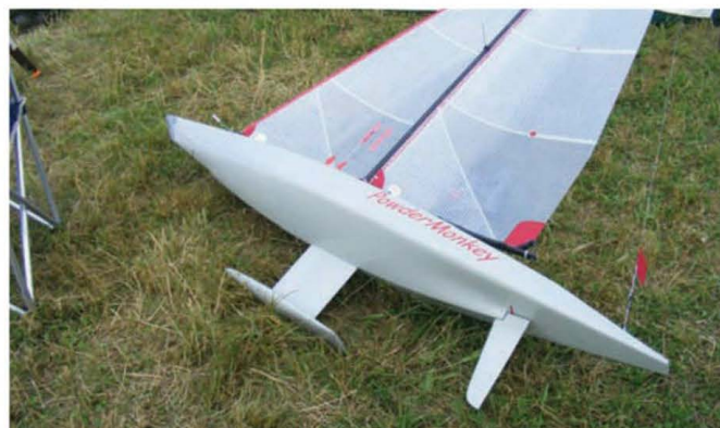
Chris Durant's Gunboat, produced off a CNC cut styrene plug and male moulded shell, lots of hard work to produce this quality of finish
