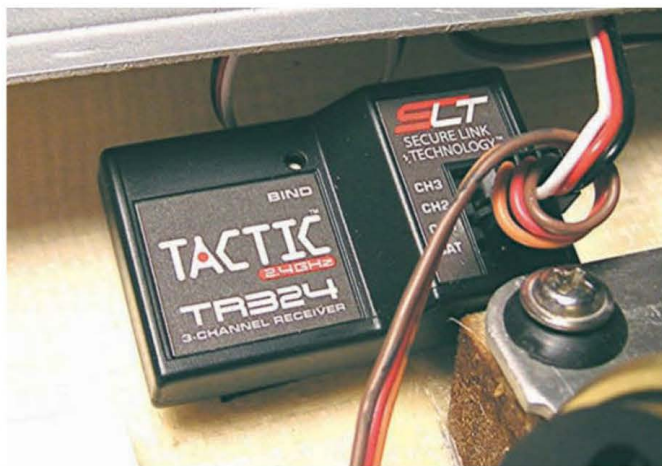
Small in size the boat's Tactic 2.4 GHz receiver doesn't require an external antenna wire/tube and the Rx is joined to the transmitter without any major setting-up procedures
