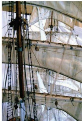
The chain halliard can be seen at left with the cross gin block at its lower end
