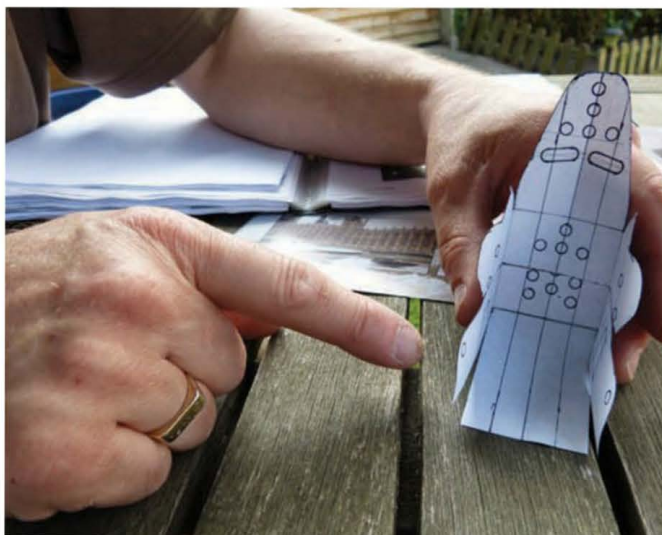
A thin styrene card cockpit seat was cut using this cardboard template
