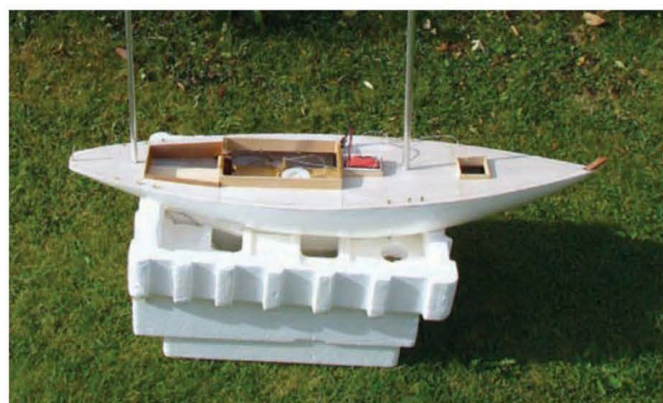
A thin ply sub-deck finally seals the working parts
