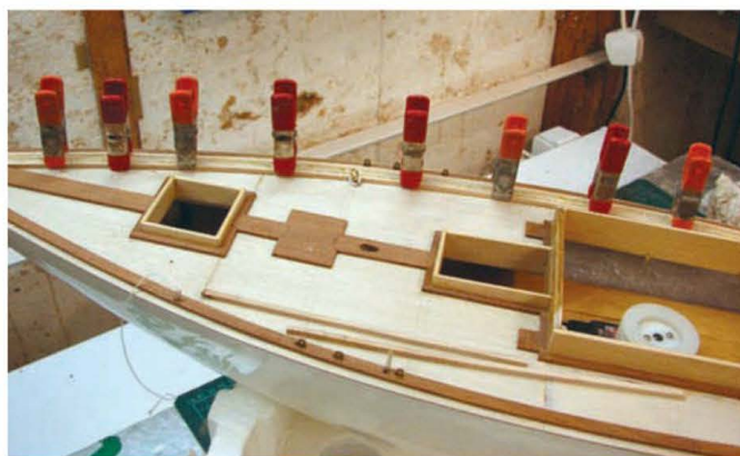
Cover boards, king planks and deck planking
