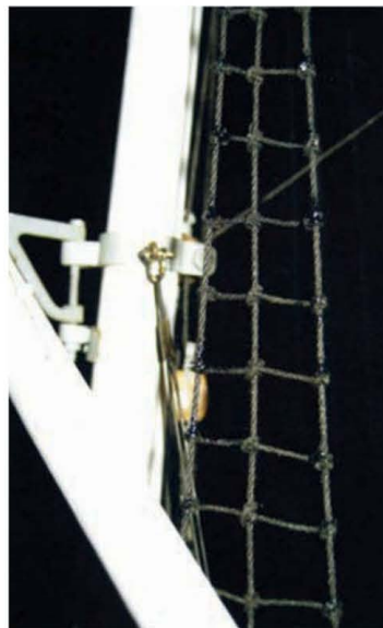
Some of the 1510 clove hitches needed to rig the ratlines
