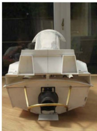
An early stern area shot with the brass protection bar for the 28 mm water nozzle in place (Photo – Chris Scott)
