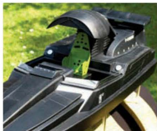
With seat finished, painted and in place a number of other processes can be seen here. The scribe lines are now more visible, drawing pin heads have been added and painted white to give detail on either side of the seat and all edges have been 'highlighted' using the Tamiya dry painting powders described in the text
