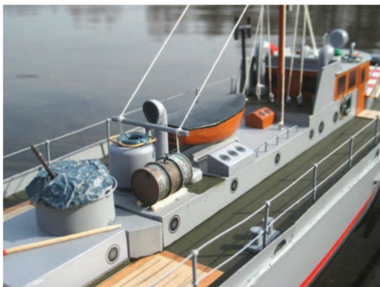
To gain space needed for the machine gun position, the vents for the Büchi chargers had to be redesigned
