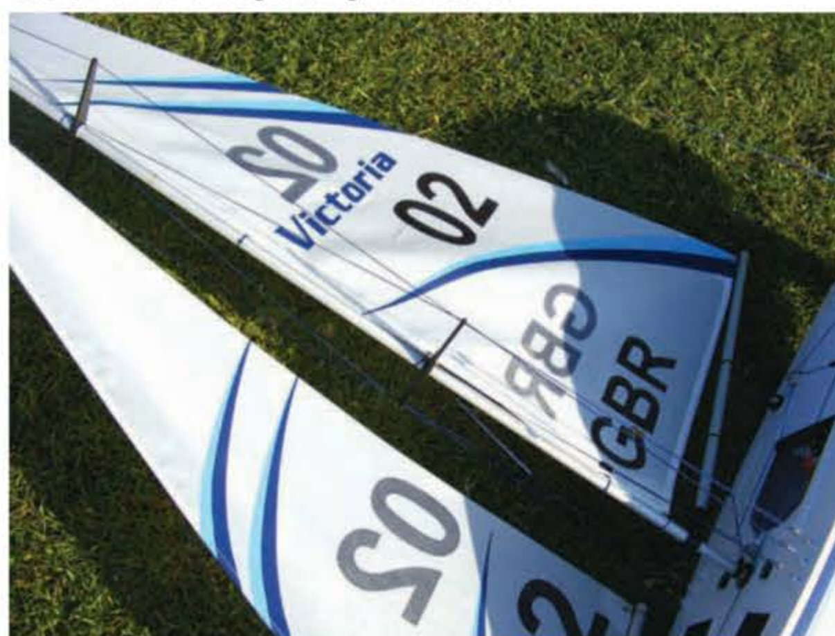
The double spreaders hold the aluminium mast well, and offer insurance against failure of any single cord shroud
