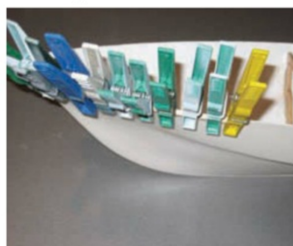
Since the original GRP hull came without any sheer rails, these had to be built from balsa
