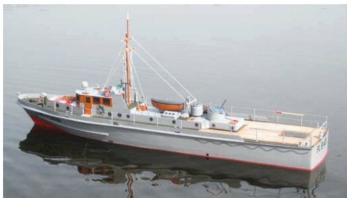
The arrangement of vents at the aft end of the boat deck is a characteristic of later Seeteufel IV-boats
