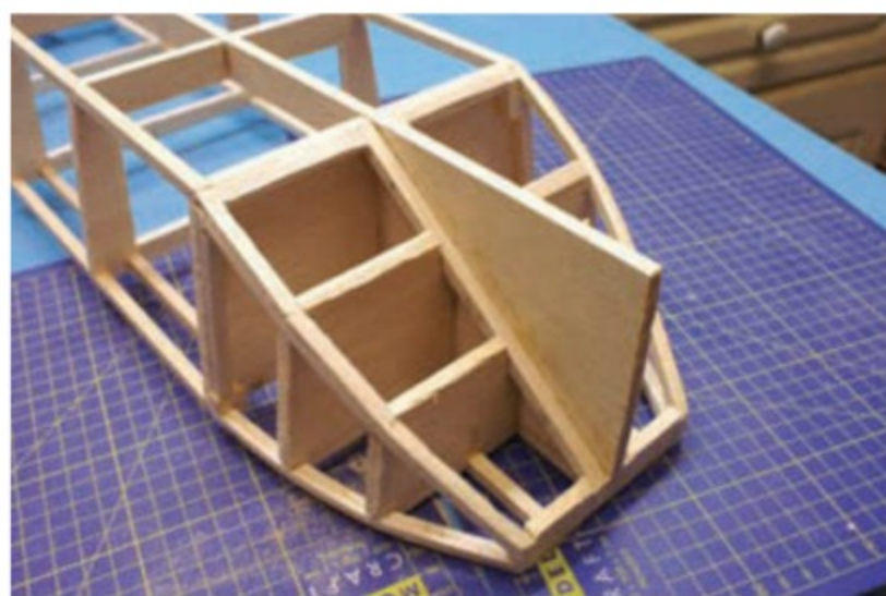
Aft end showing fixed rudder
