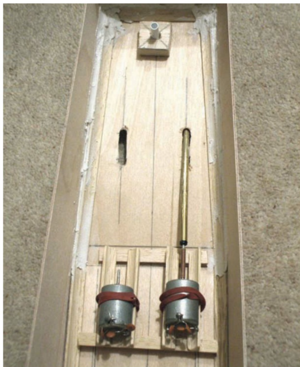
Slots cut in hull bottom and one shaft being lined up. Rudder tube and support block glued in place
