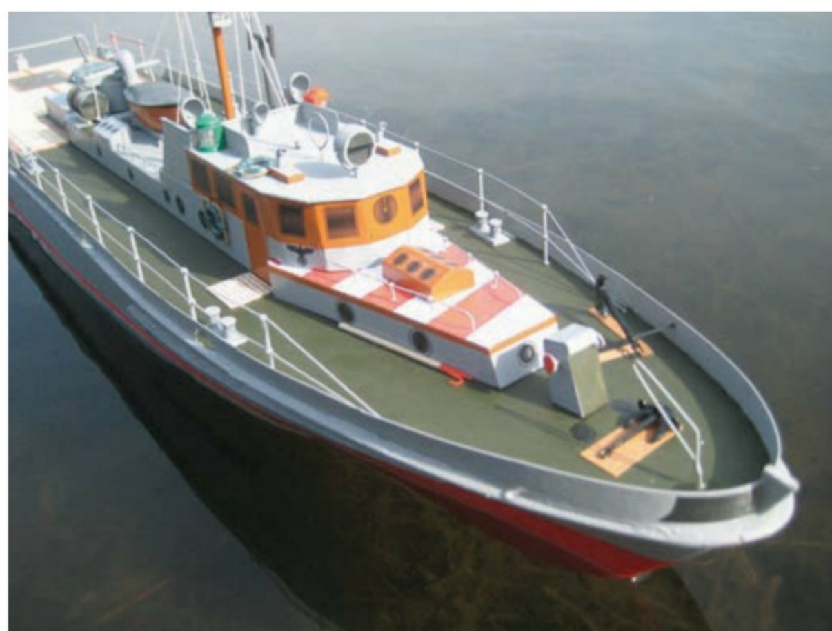
After applying Glasurit filler, usually used in automotive body shops, grey spray paint was used for vertical surfaces
