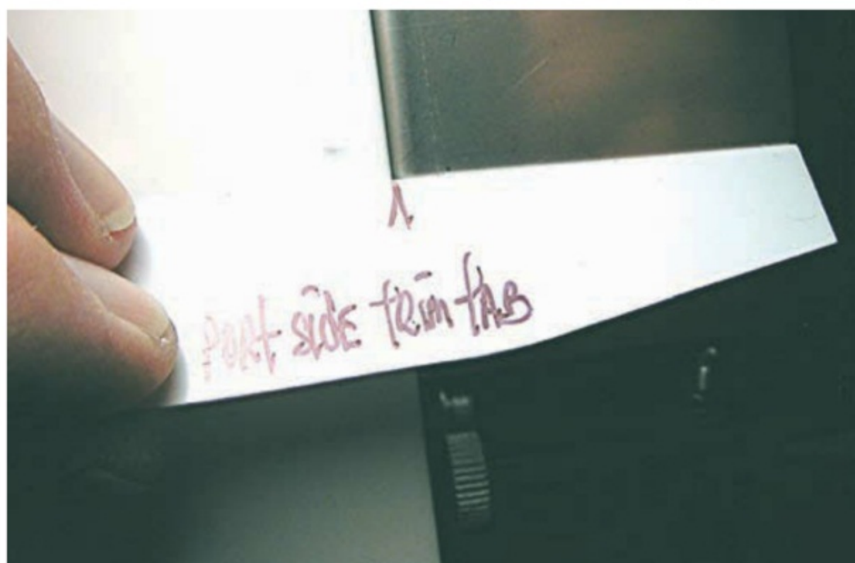
Made up from pieces of scrap plasticard a set of trim tab angle gauges will allow the boater to quickly/correctly determine if his/her hull's trim tabs are set correctly at all times
