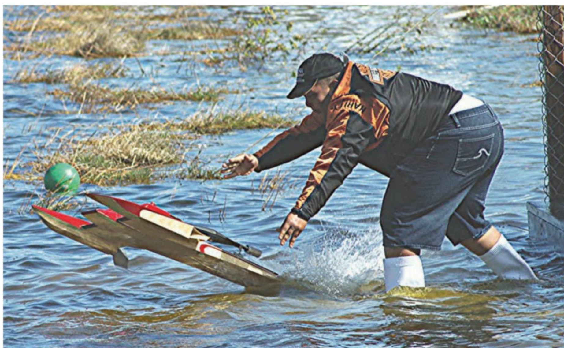
Dropping a boat stern-first, especially on a hull sporting a large-diameter surface drive propeller can result in a 'wheelie' or a quick torque roll each of which means a non-start during your day at the races
