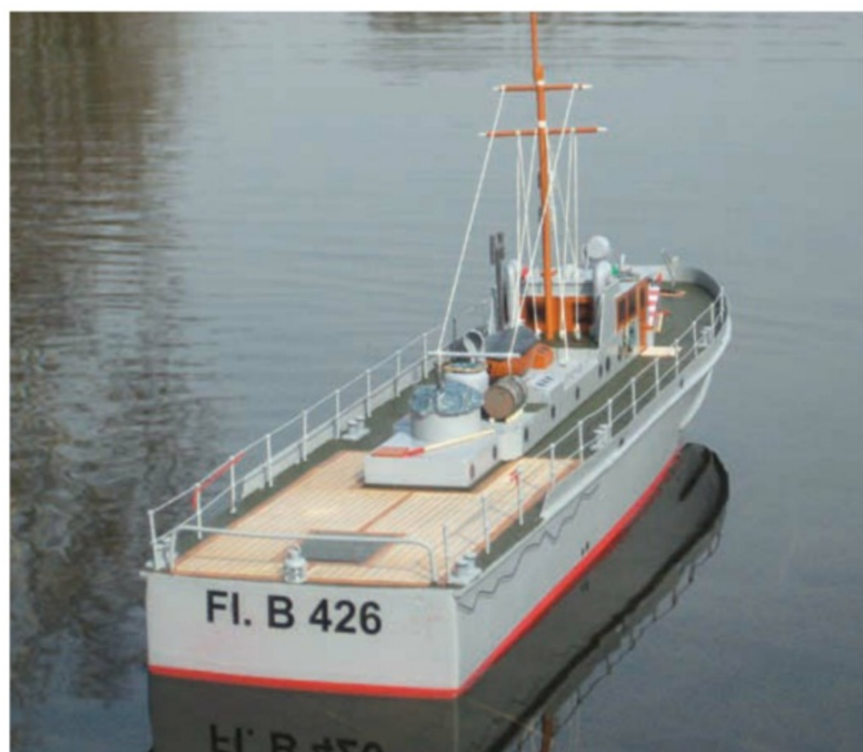
The model sports a grey hull and dark green horizontal surfaces, with a wooden deck aft. To avoid the wood from looking too even, its pieces were dyed in coffee
