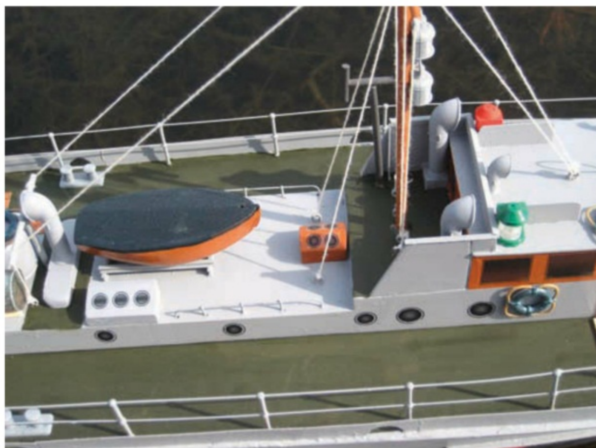
Searching for downed aircrews was difficult due to the low silhouette of the boat. A flybridge increased the visibility
