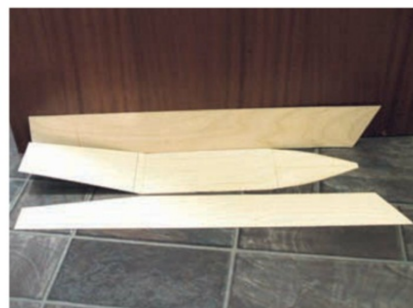
The two hull sides with the hull bottom, its after portion canted up
