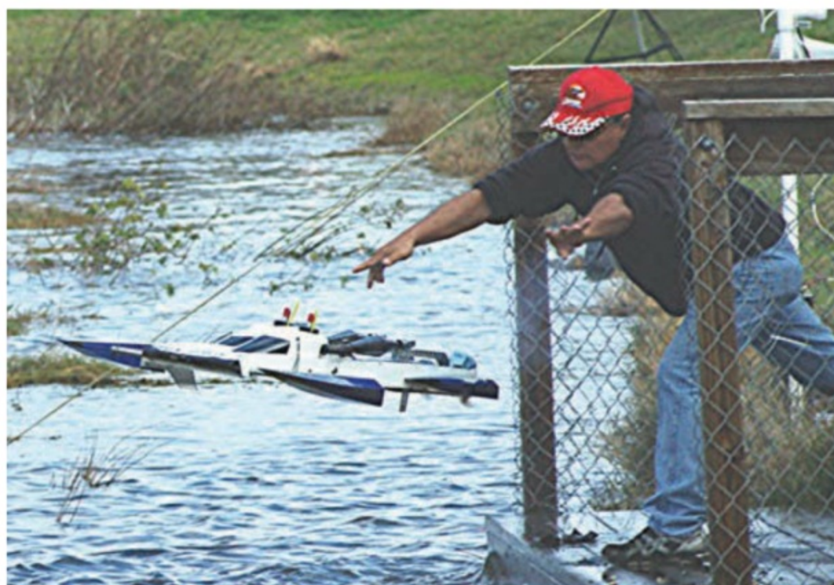
Dock-launching an I/C vessel could end up adding a bit too much altitude to the toss and the result could be an engine stall out or a snapped drive cable once the running hull contacts the water
