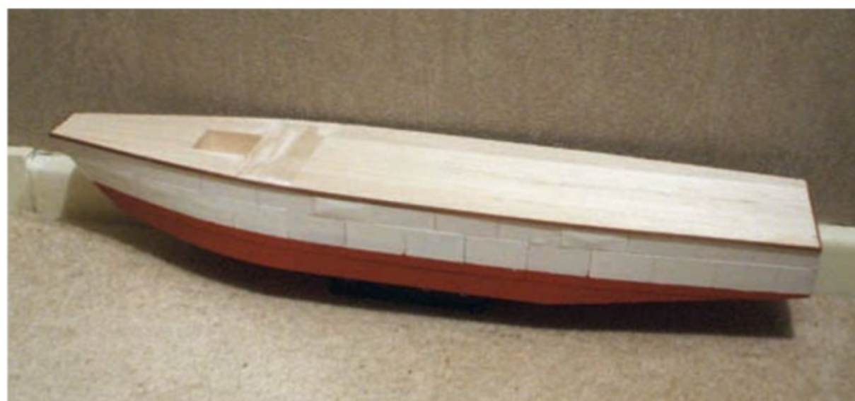
Decking complete. Smoke bomb mortar pit installed and mahogany rubbing strip fitted around deck edge
