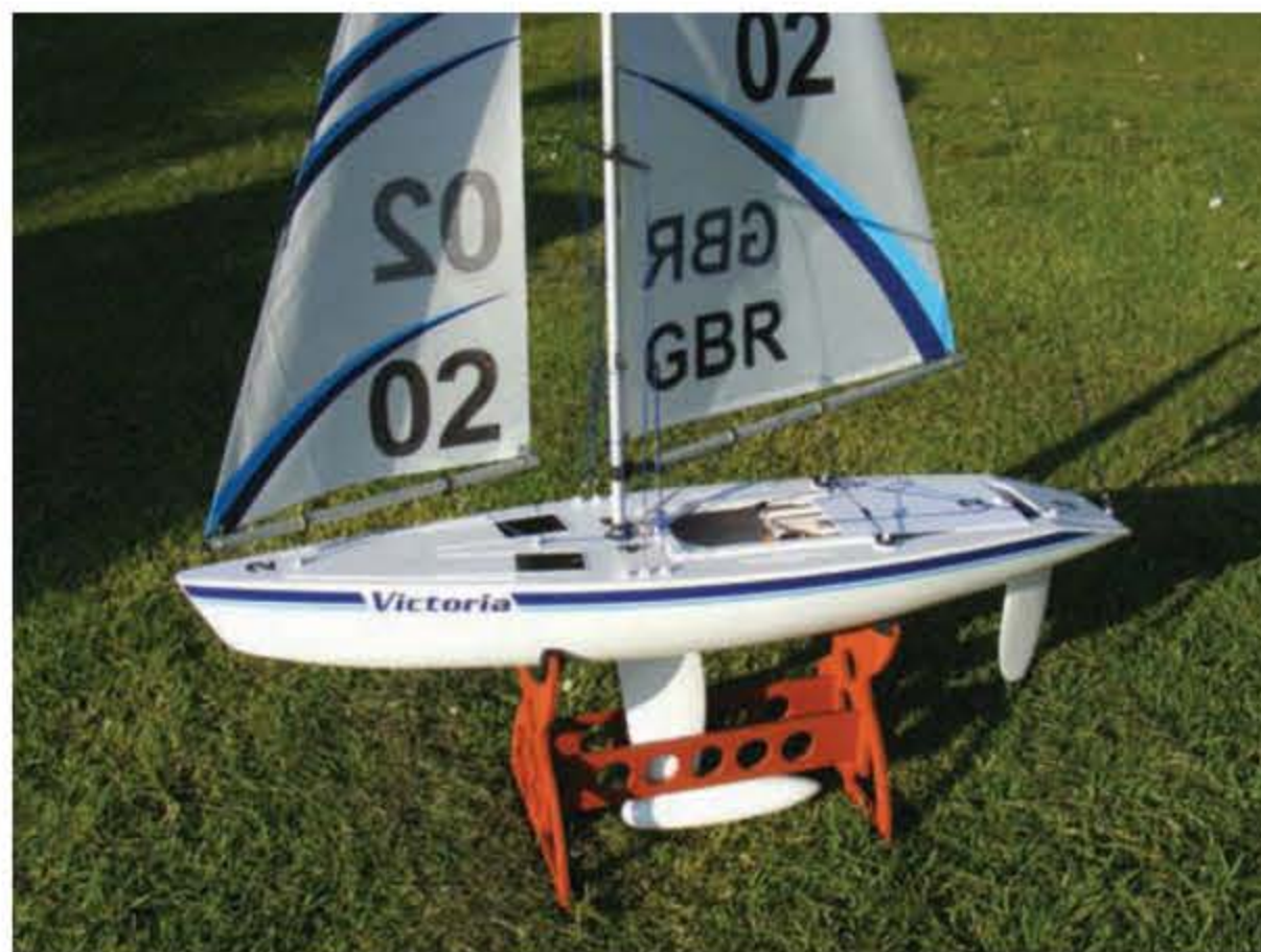
On its kit supplied display stand you can see the moderate keel depth and classic hull lines of the Victoria
