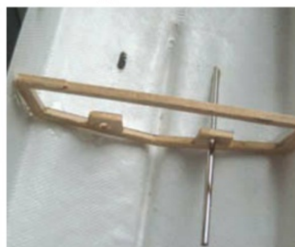
Twin shafts are glued in place after alignment with aft frame
