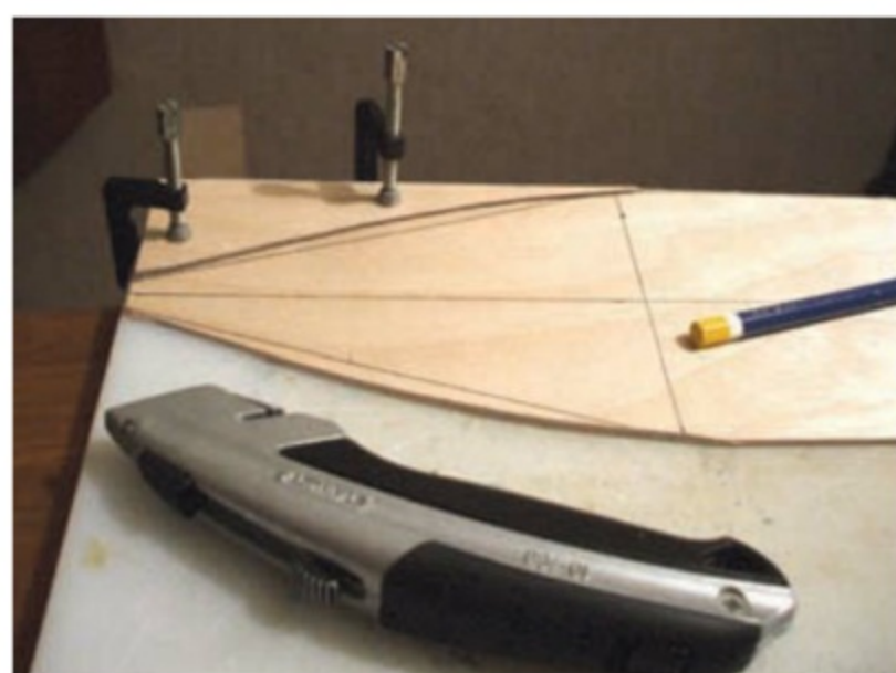
A bow section cut out being used as a template for the opposite side
