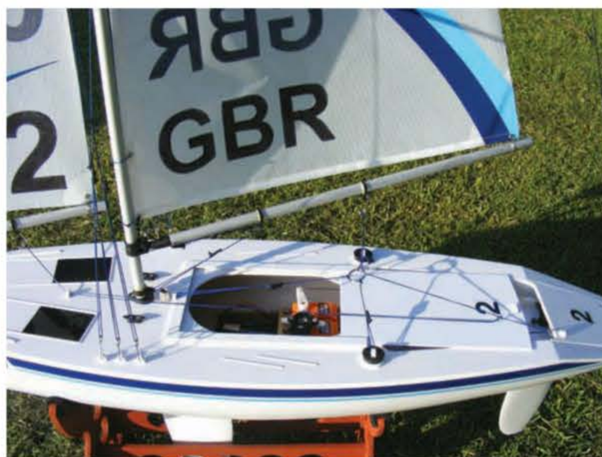
The mainboom has a cord kicker, which works acceptably and is very sound in design
