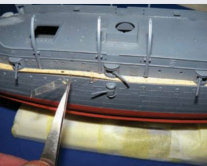
Film being removed to allow self-adhesive deck to be securely fixed
