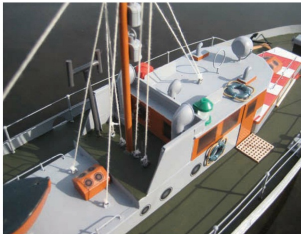
The rear side of the wheelhouse had two windows, which could be opened to ease communication between helmsman and spotters
