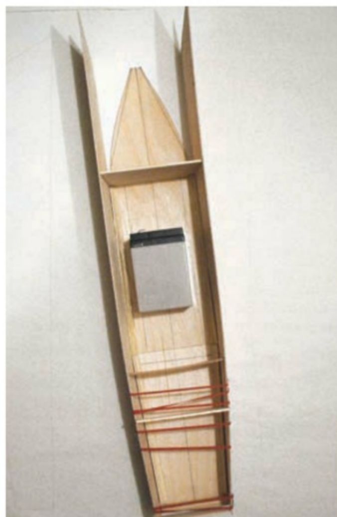
With the main bulkhead in place the aft sections of the hull sides are glued to the bottom (the crossbeams aft are temporary)
