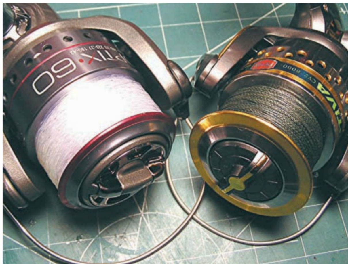
Both mono-filament (left) and braided (right) fishing line can be used on a rod/reel recovery set-up; however, the extra-strong braided fishing line will be a lot more difficult to remove should it get tightly wrapped-around a boat's prop shaft/stuffing tube area
