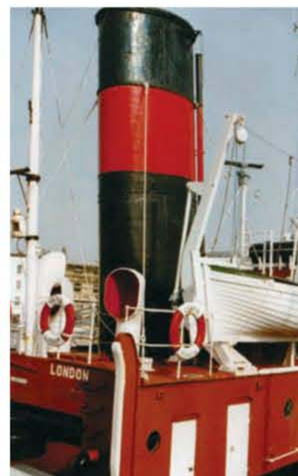
Funnel and engine room ventilators
