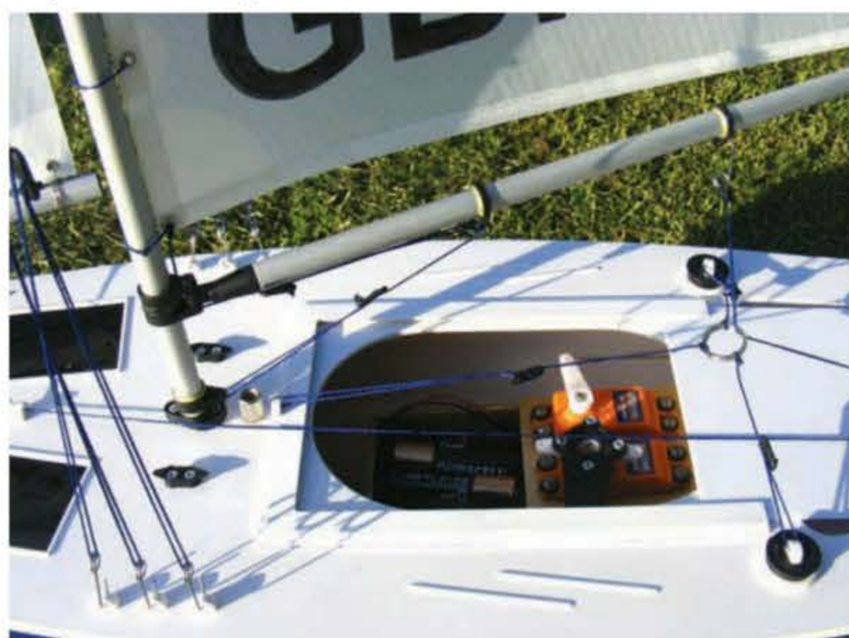
The R/C gear is held in a timber box to avoid water ingress and is located under a long sliding hatch cover
