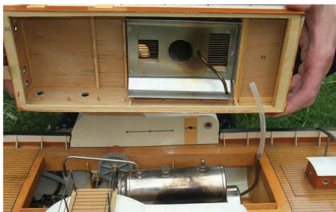
Fitting the superstructure
