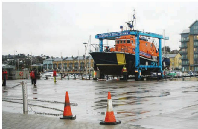
Lifted – an expensive removal to take off the starboard propeller for repair and anti-foul the lower hull
