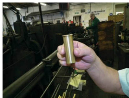
Funnel of a steam engine just off the production line
