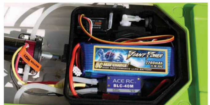
The radio/power box layout
