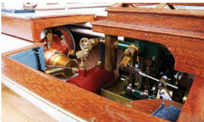
The power behind the model. On view the steam power plant for Consuta, a triple planked Umpire's Launch from the River Thames, built by Tony Woodford
