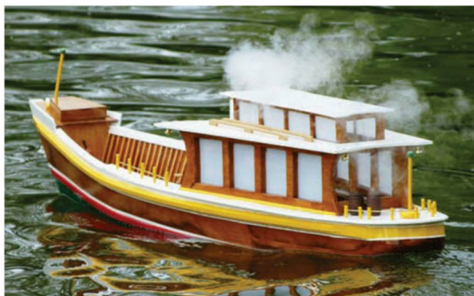
Trevor Tallent's 1/8th scale gas powered steam river launch underway
