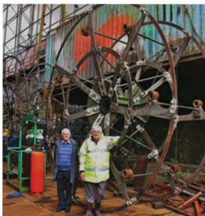
Paddle wheels being constructed for PS Medway Queen (image by Bob Stokes)
