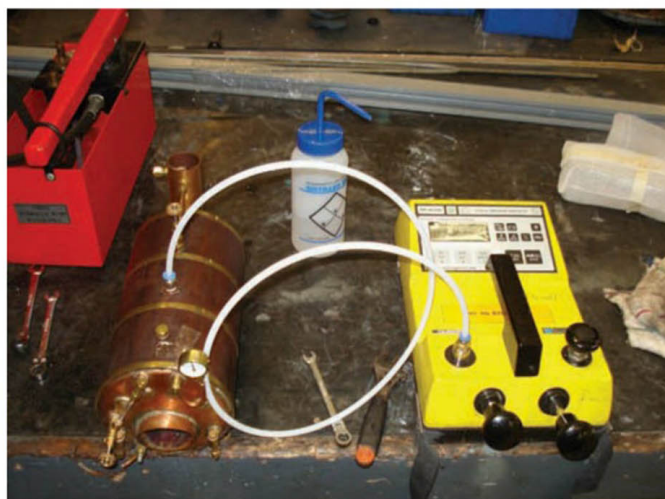
A 5½" boiler being prepared for its hydraulic test. Pressure and water level gauges may need removal for safety
