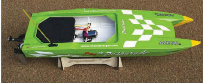
The magnetic top removed revealing the brushless motor and sealed radio/power box
