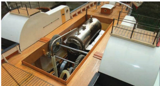
More detail of the drive train for the paddles
