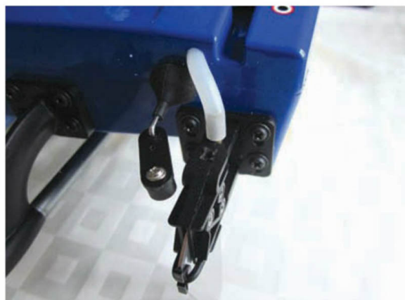
The damaged rudder assembly on the first blue model
