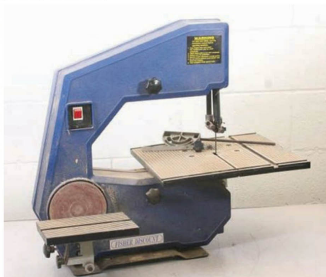
A more typical modeller's bandsaw. This one extra useful as it has a built in disc sander, cheaper too
