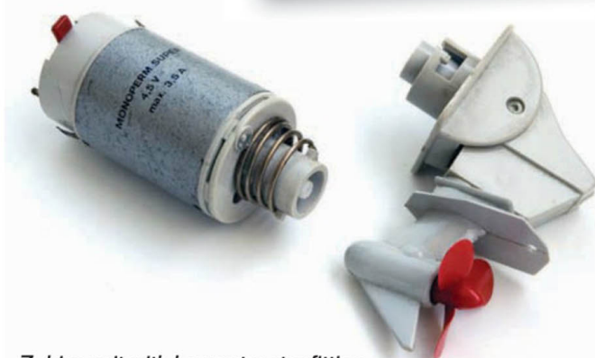
Z-drive unit with bayonet motor fitting
