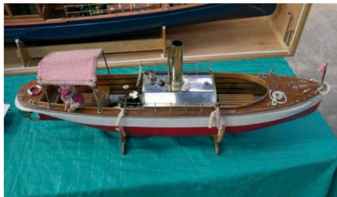
Arthur showing the meths fuelled boiler and engine
