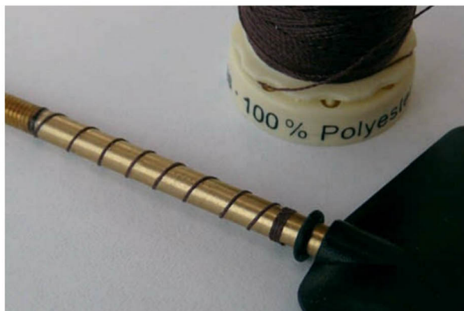
Polyester cotton and a small 'O' ring are added to the rudder to provide a watertight seal
