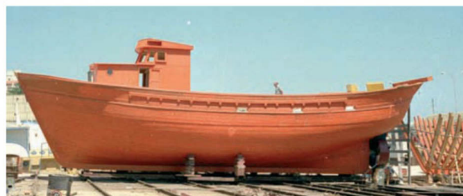
Another broadside view. The overhanging section of bulwark amidships is noteworthy, but do not know the reason. She has been fitted with a kort nozzle around the propeller, so I assume she is intended for trawling
