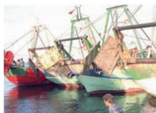
This shows the typical rig aft of the trawlers, with extending towing gantry with cross beam and round cross beam carrying the warp hanging blocks and stern roller
