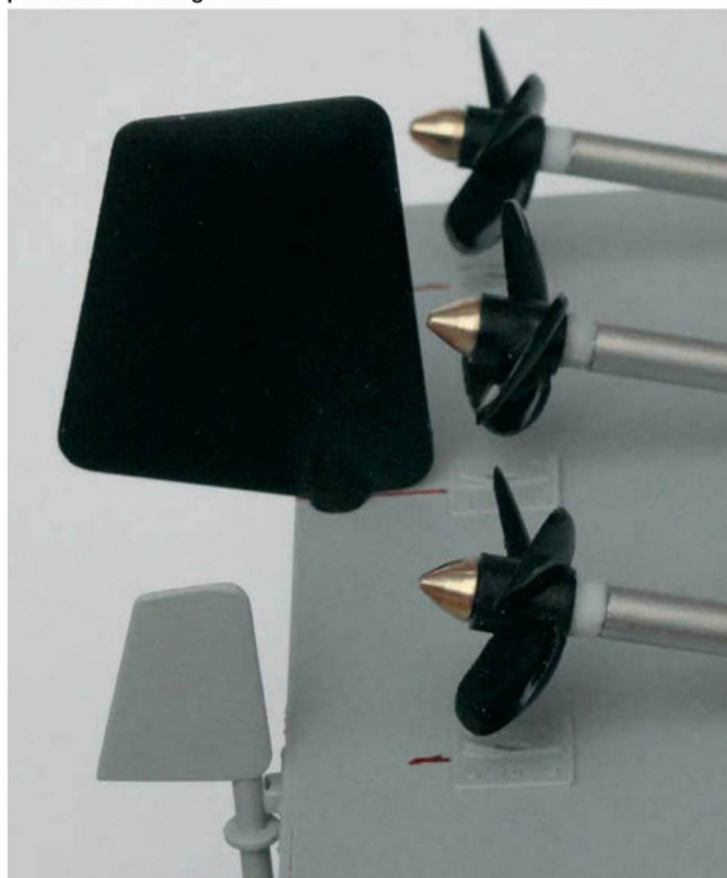
The rudder is installed close to the stern – leave room for propeller removal!
