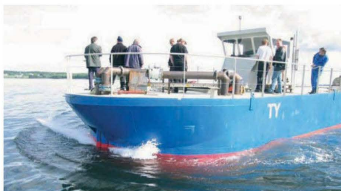
Hydrodynamic flushing test vessel – note pipes running to the rounded bow
