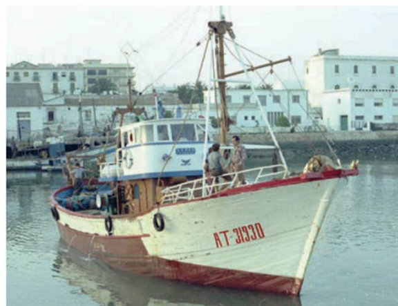
Bow quarter view, showing the short derrick mounted high up on the mast with short crossrees, note the beam across the bow with fairleads at ends
