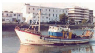
Another trawler leaves port, the trawl winch and the towing gantry and trawl doors can be seen clearly at the stern
