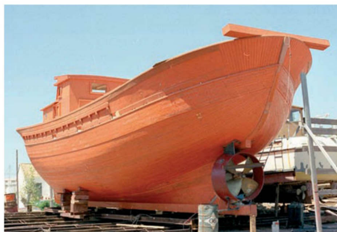
Another view of the same boat, from aft completely planked this clearly shows the different run of planking aft referred to above. I am not sure what is the purpose of the cross beam on the stern, some boats have a similar fitting on the bow with fairleads at each outboard end
