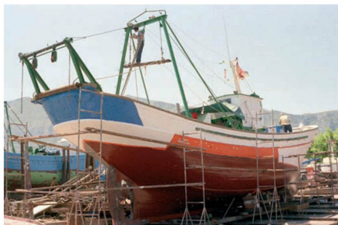
Small trawler hauled up for repairs. This gives a clear view of the towing gantry with round bar cross beam and hanging blocks mounted on swivelling collars on the beam and stern roller
