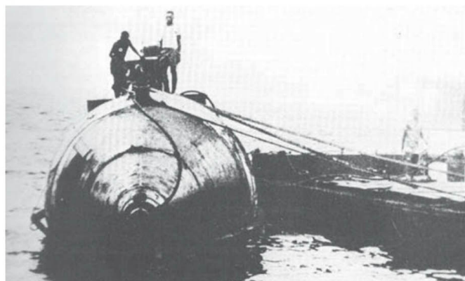
A captured (washed ashore?) Unkato supply canister. The Polynesian natives give scale to this craft, while this bow perspective confirms its very basic cylindrical form
