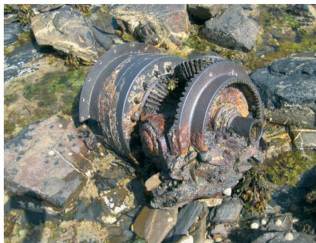
Remains of S-89's transmission, originally belonging to the centre prop
