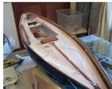
Showing decking and rudder servo mounting
