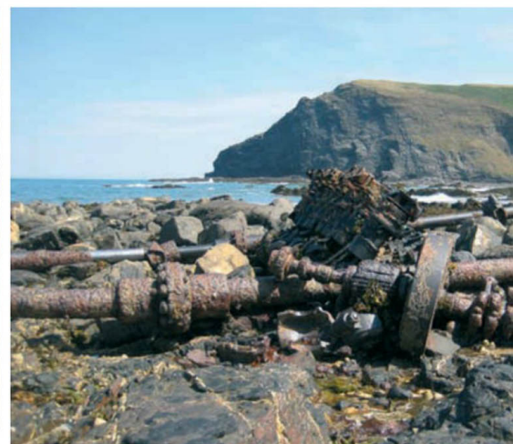
Shafts and engine positions reveal the position of the boat when running aground
