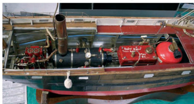
A good view of the boiler, engine, fuel tank and reserve water tank
