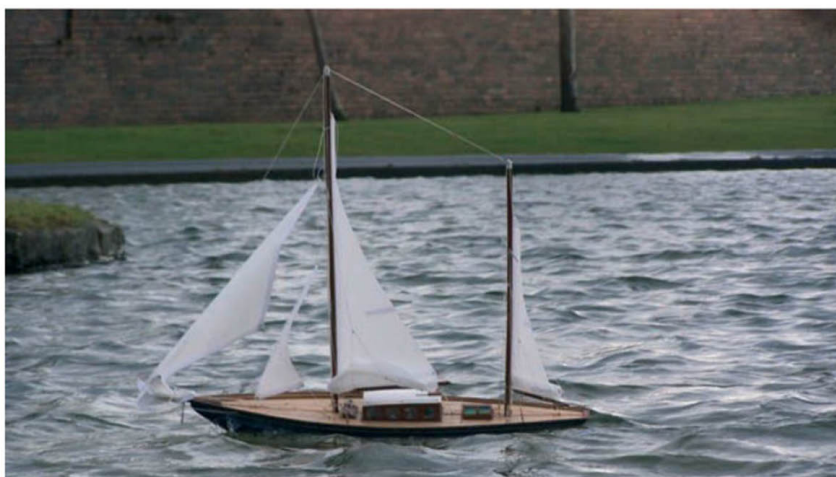
Reaching with the flying jib tacked to the bowsprit and a reefed mainsail and mizzen
