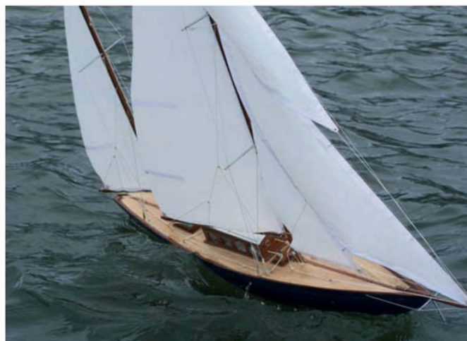
Full sail and note wired boom inside the foot of, No.1 jib
