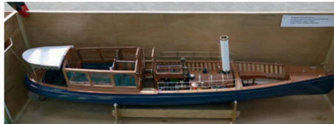
Superstructure removed to give access to the steam plant
