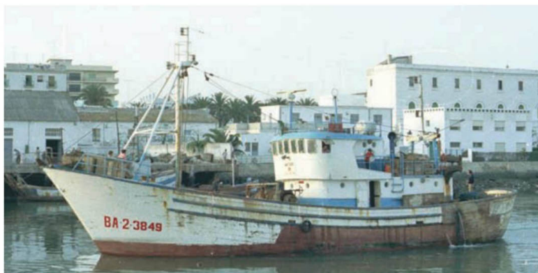
Another trawler at Puerto de Santa Maria with rig more akin to British trawlers. She has hinged towing gallows mounted on aft end of deckhouse and trawl winch forward of the wheelhouse, it would appear that the wire span between fore and after mast is used to carry a hoist rope handy for the foredeck
